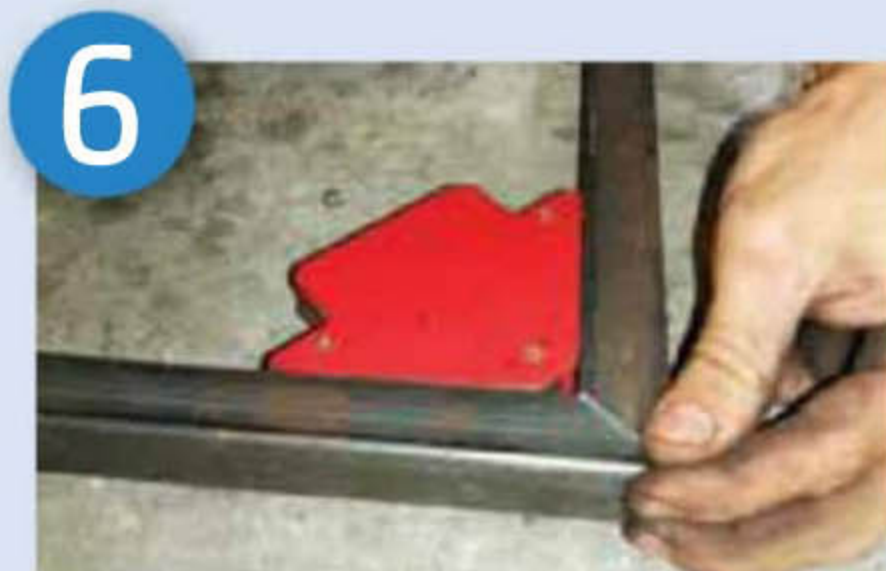
Use a welder's magnet to keep points together
