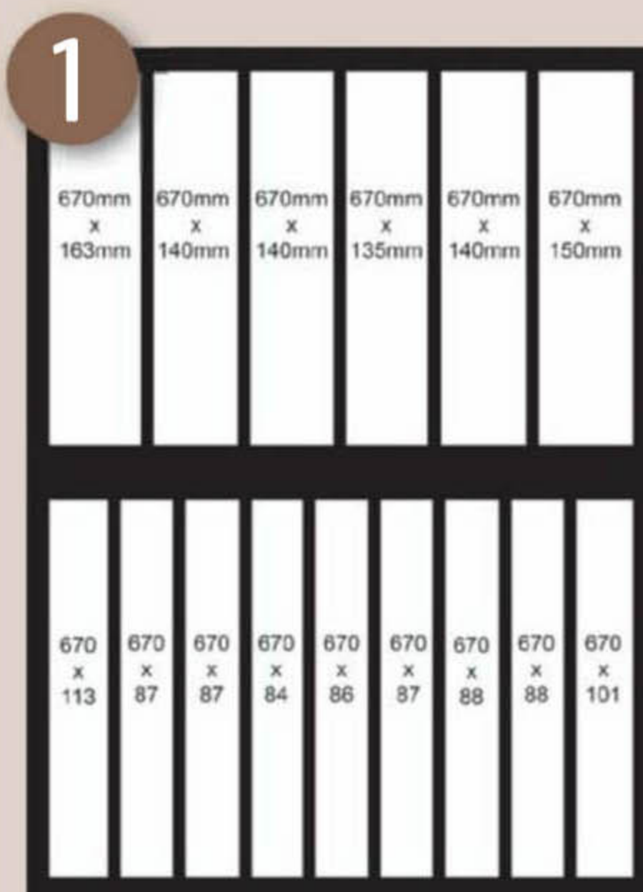
The planning diagram with the measurements of the slats
