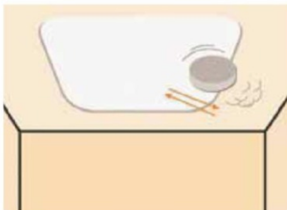
Sand the patched seams smooth to the ceiling, using a fine-grit sanding block
