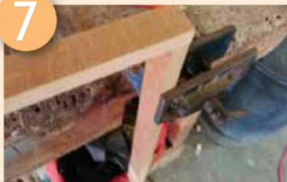
Place in clamp and glue pieces together
