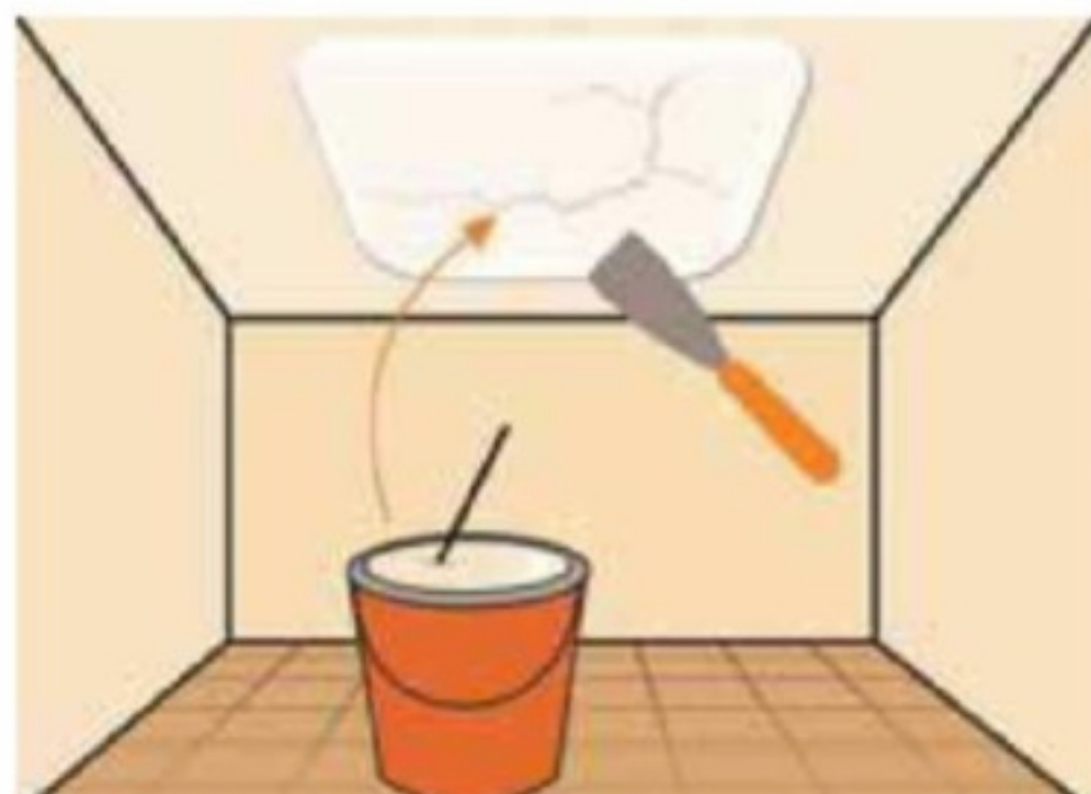
Apply a thin layer of drywall joint compound
