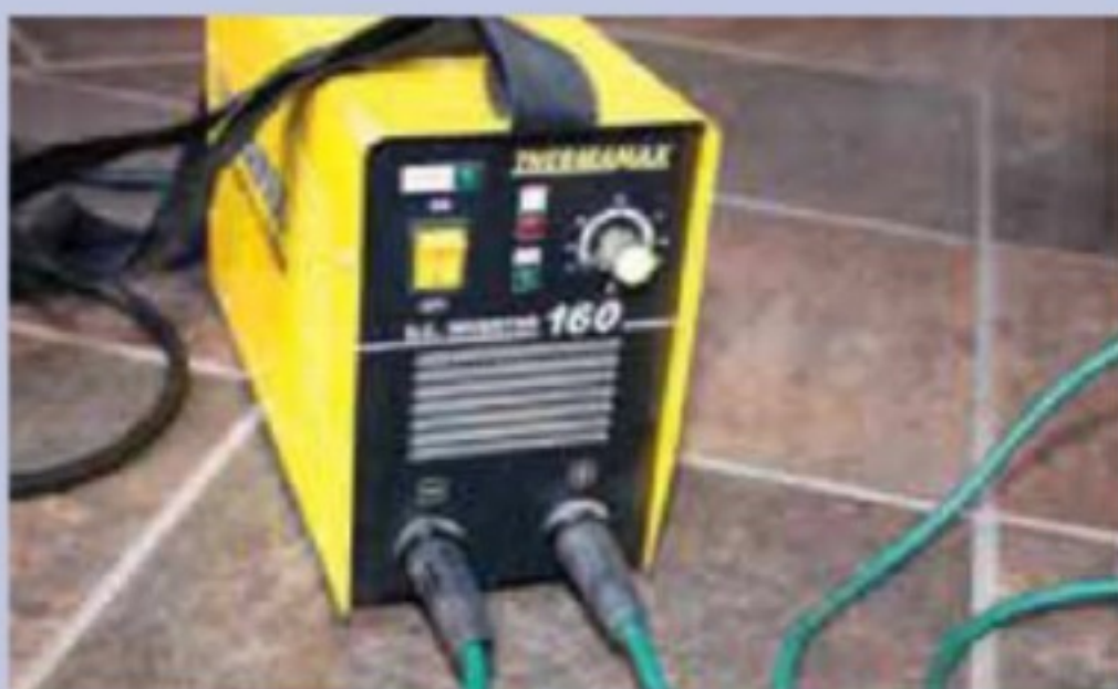
An example of a suitable welding machine for DIYers – lightweight, compact and easy to use
