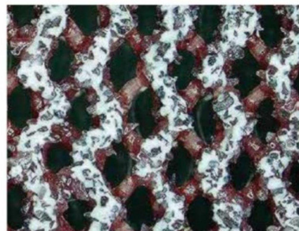
A close-up of a small part of the upper side of a sanding screen. On the diamond pattern of the mesh, white glue appears in zig-zag streaks in which the silicon carbide crystals are embedded ( \pm 20X magnified).
