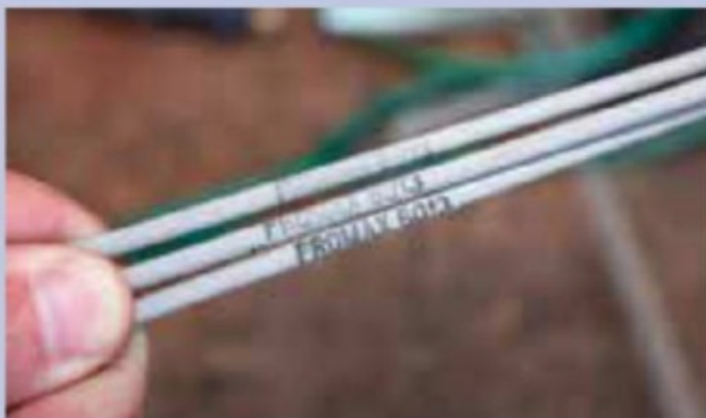
The numbers on the welding rod follow an international standard which indicates what type of metal these rods are suitable for
