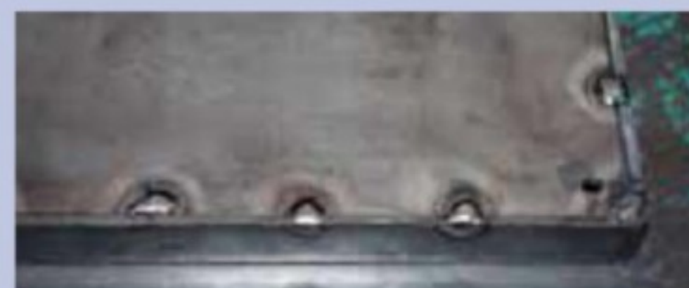
Spot welding is used when attaching sheet metal or angle iron or square tubing
