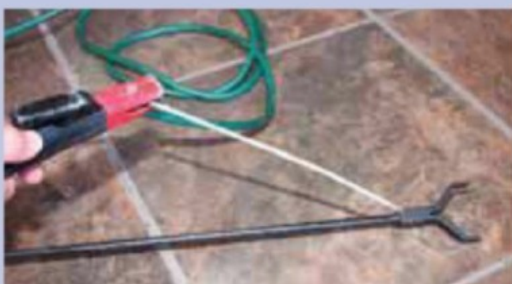
The welding rod in position clamped into the positive cable
