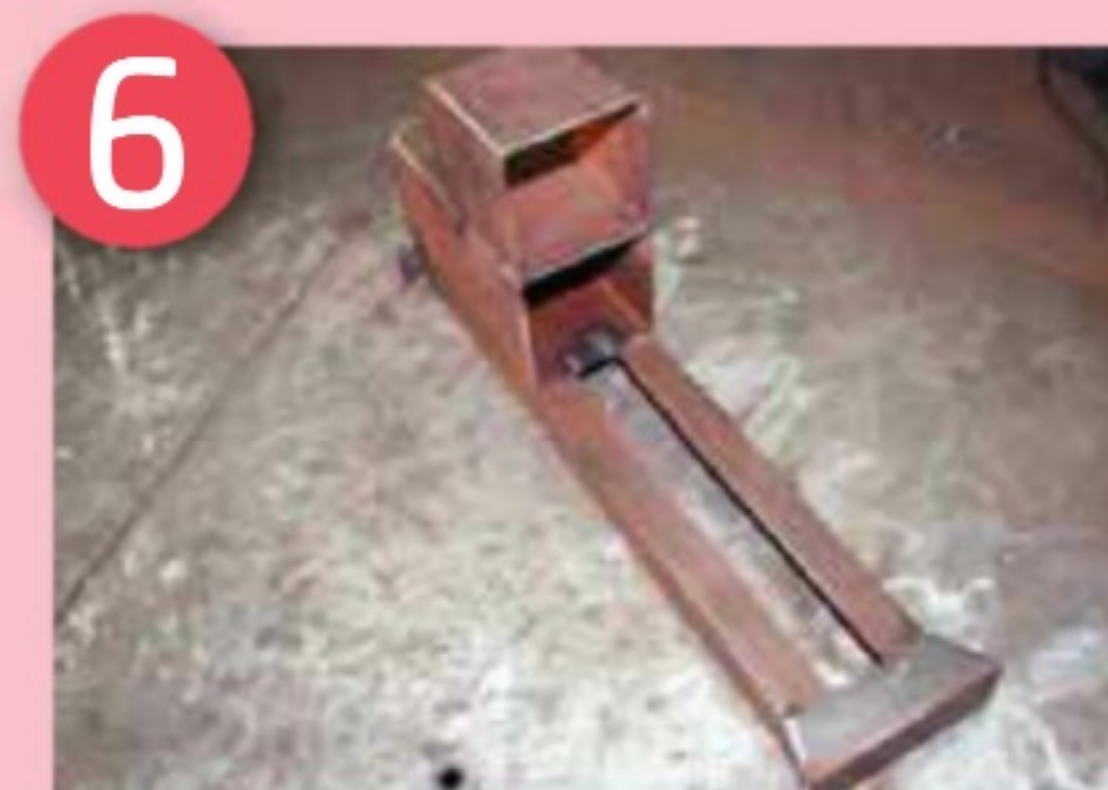
Cut 130mm of 25mm angle iron for the rear bumper
