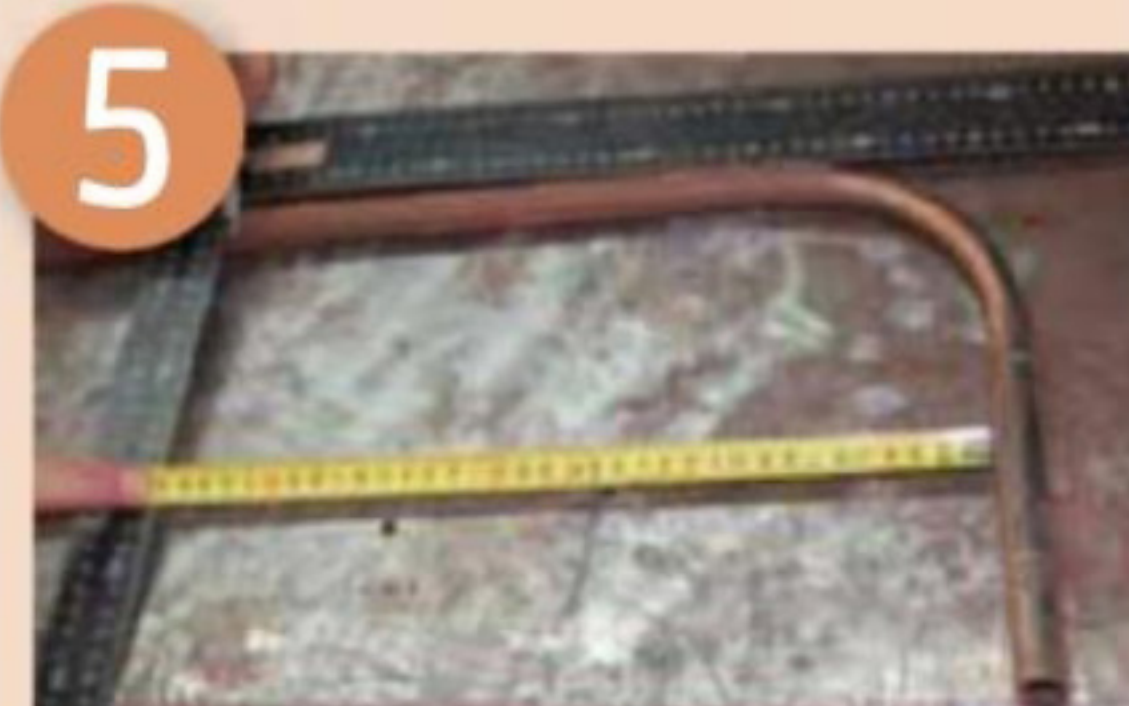
Measure 350mm for the second bend
