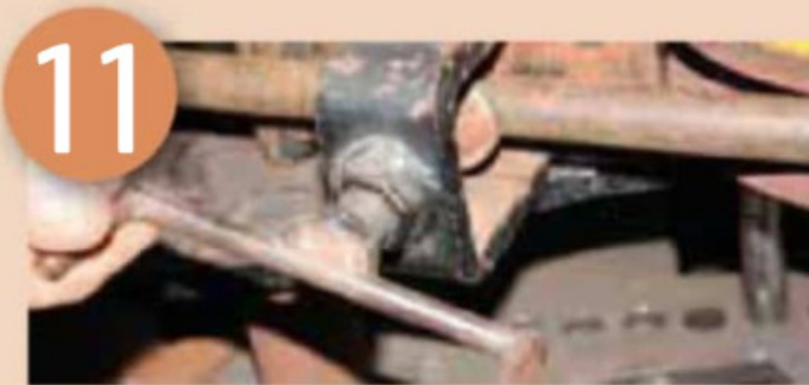
11 150mm was measured to make sure there is enough body for the pipe to fit into the vice of the pipe bender
