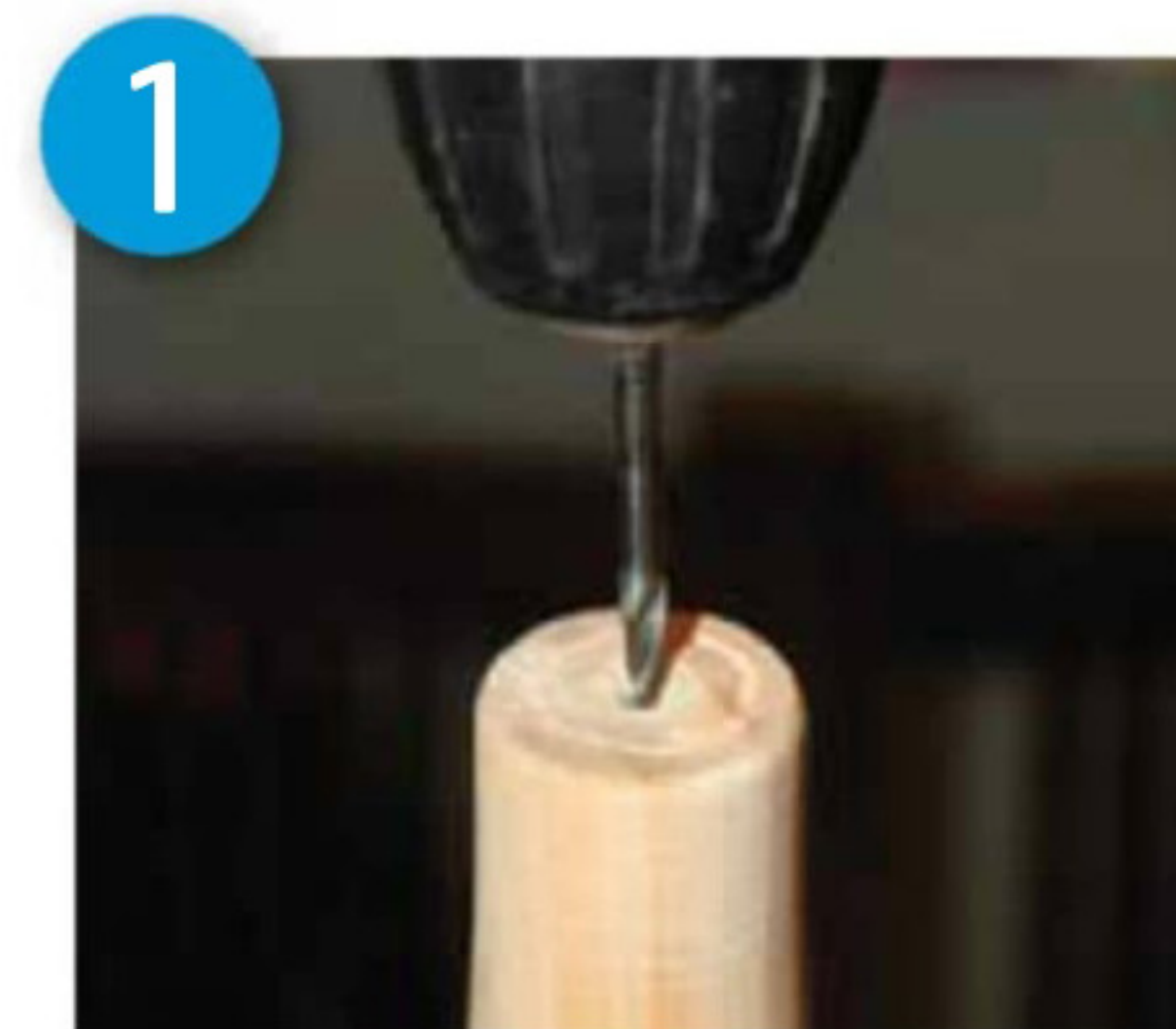
Drill straight down into the base of the leg
