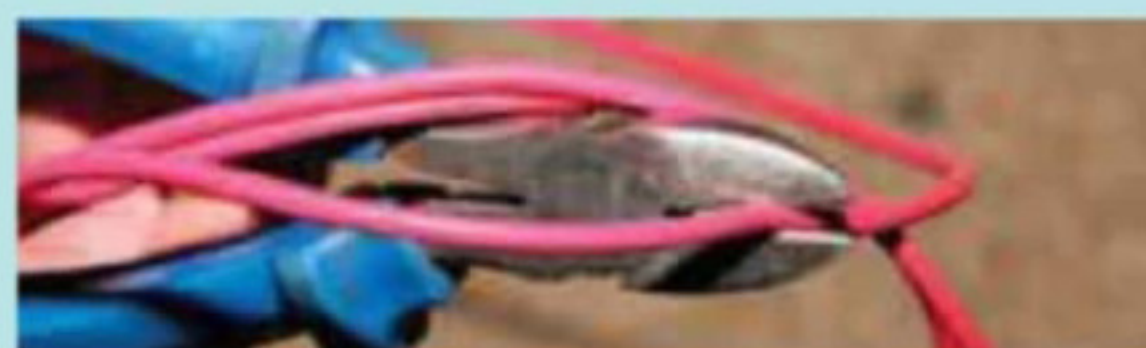
A side-cutter is useful for cutting strands of wire
