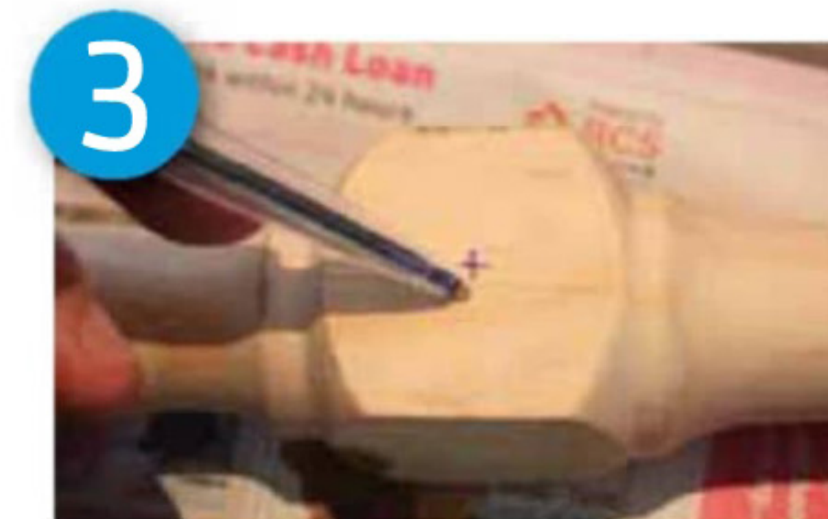
Carefully mark where to drill for the dowel
