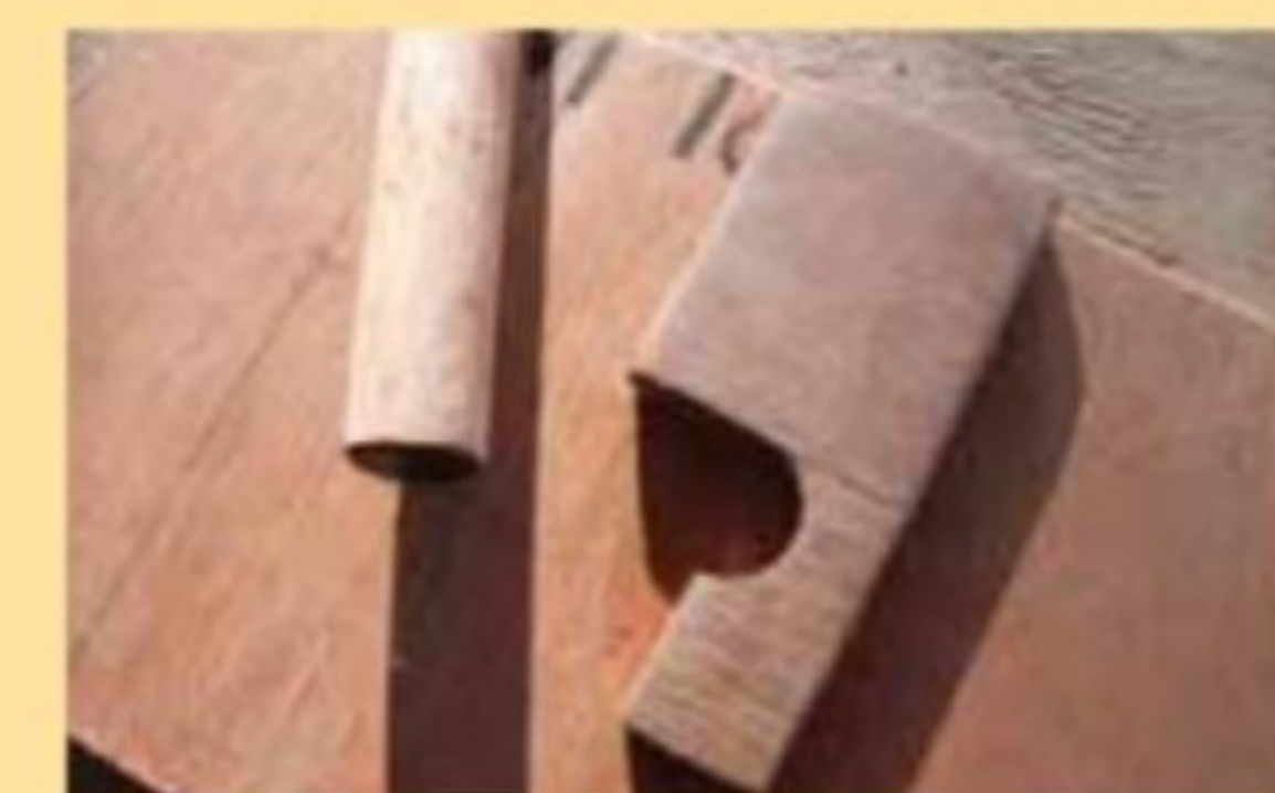
To cut down on weight, dowel rods were used for the fronts of the bottom shelf
