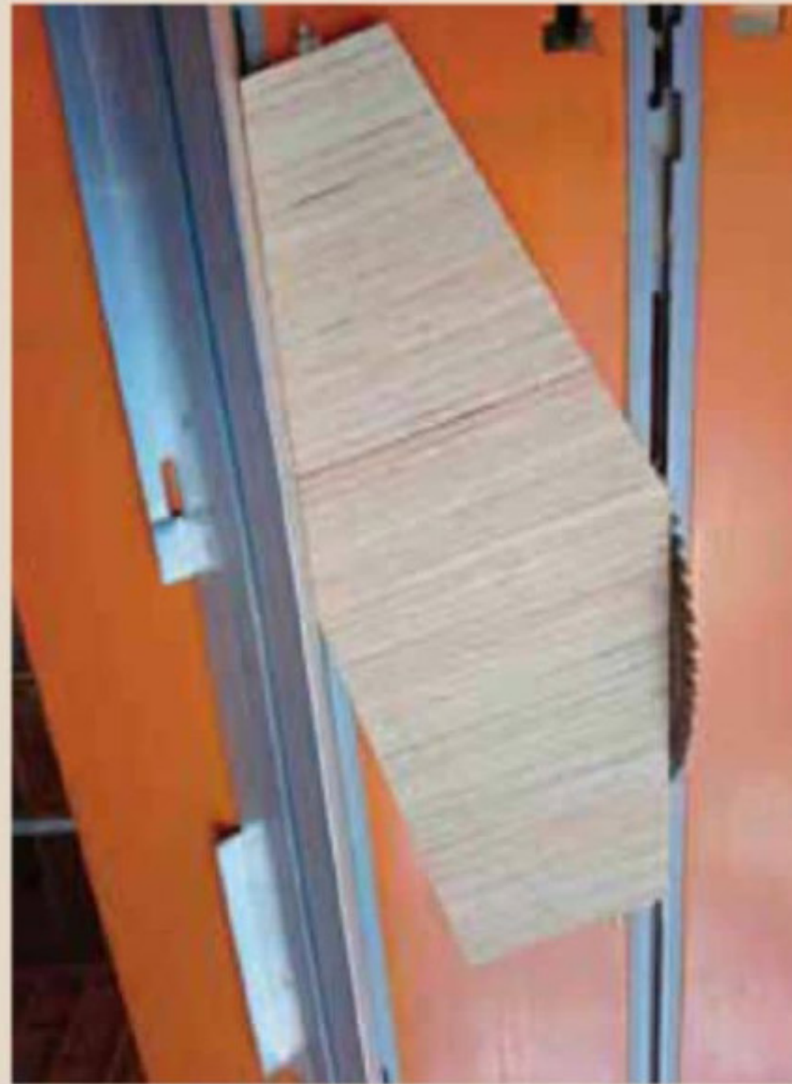
Cut along the lines to get the taper profile of the spinner
