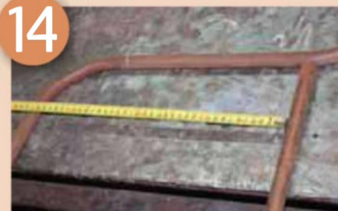
14 Measure 360mm (inside dimension)
