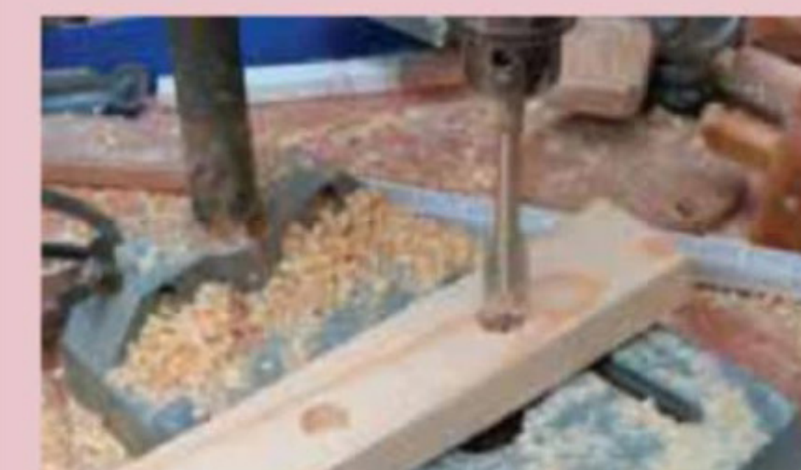
A drill stand facilitates square drilling
