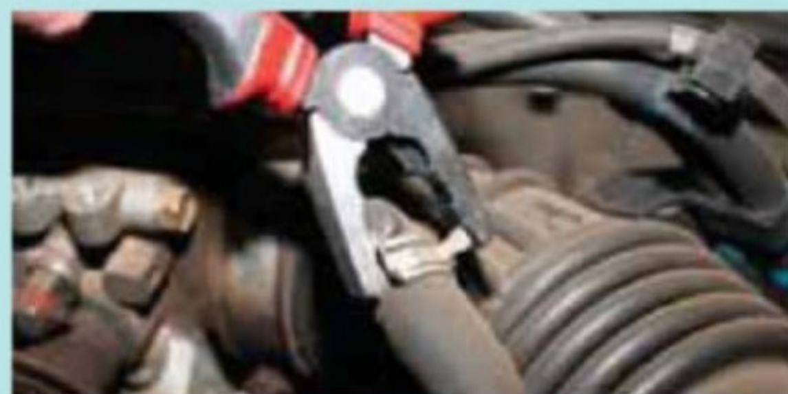
The combination pliers can be used to cut, grip and extract items and is an essential pliers to have in the toolbox
