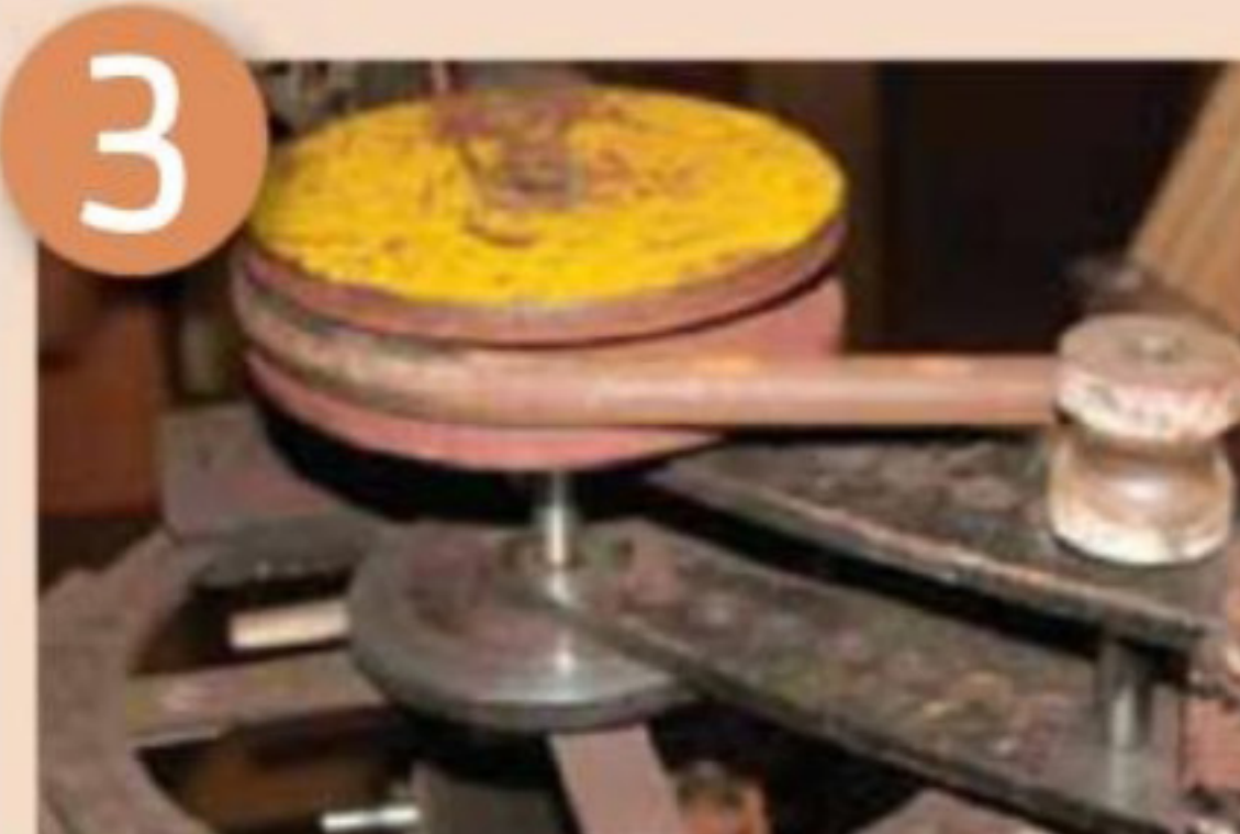
Bending the first 90° bend
