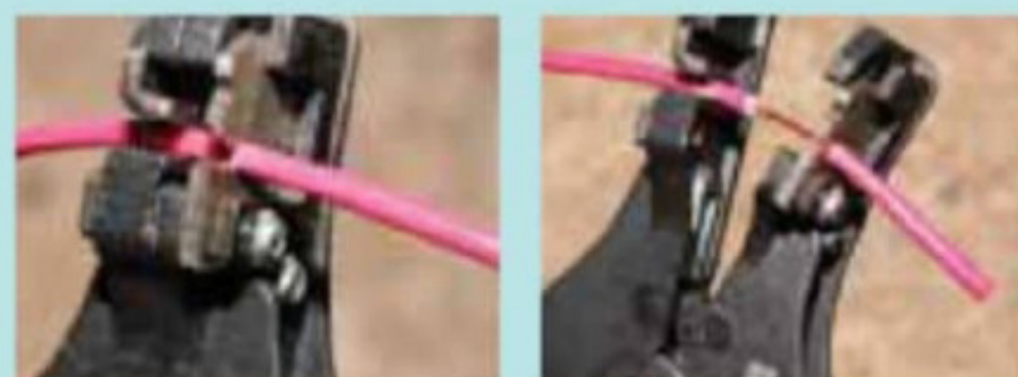
A wire-stripper is used to remove the outer insulation without damaging the copper
