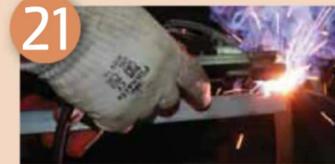
21 Weld the flat bar in place for the seat and back rest
