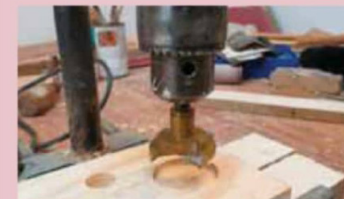
Clamp your wood together and use a Forstner bit to cut half-rounds for the bottle necks
