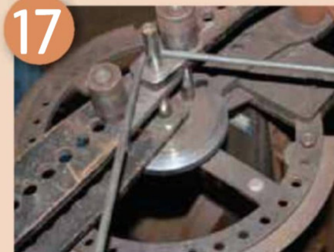
17 The 90° bend on the 8mm round bar
