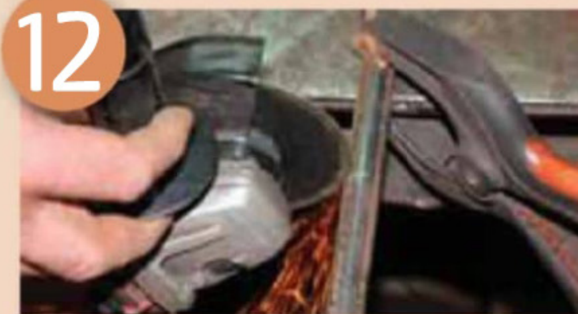
12 Cut off 80mm of the original 150mm measurement
