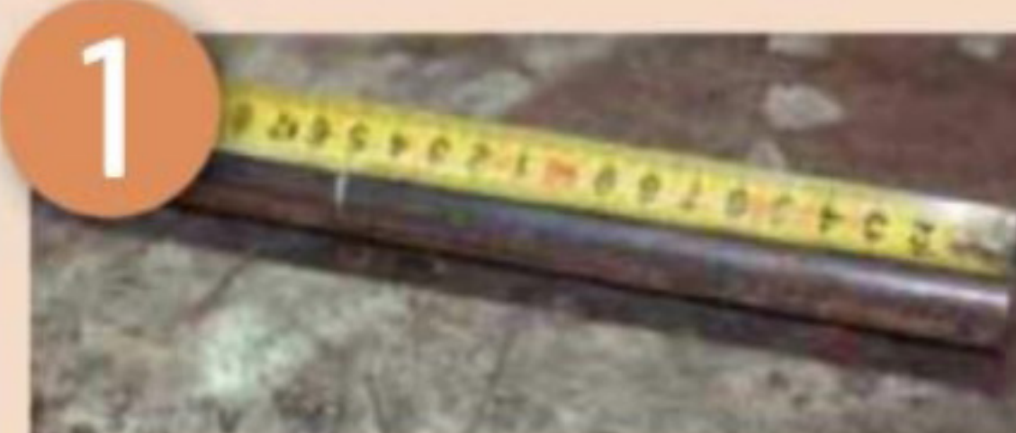
Measure 150mm of the round tubing
