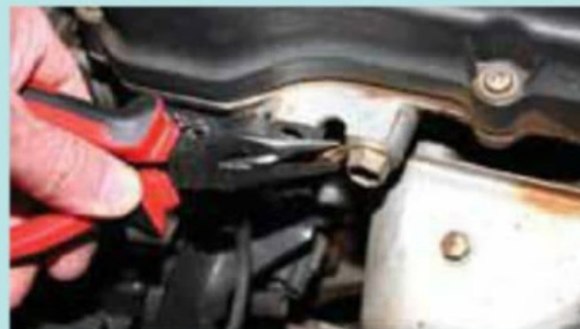
Long-nose pliers are useful when working in tight spots for extracting or holding items in place
