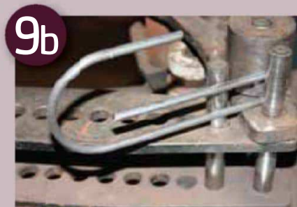
Bend 45° to prevent the toilet roll from slipping off
