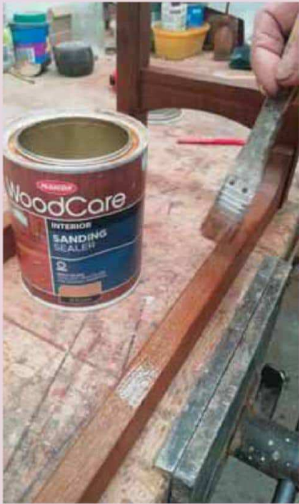
Seal the wood after it has been sanded and assembled in the frame
