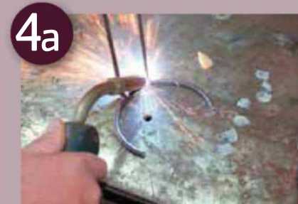
Cut two 350mm of 6mm round bar and bend a 135mm diameter circle
