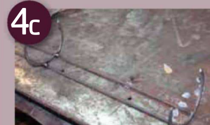
Weld the 'horse shoes' in place
