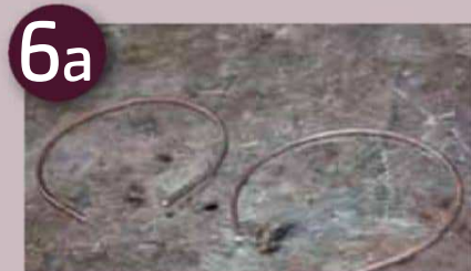
Cut two 350mm of 4mm round bar and bend two circles
