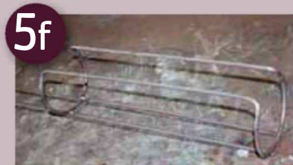
Cut the 6mm round bar and bend 90° on both sides
