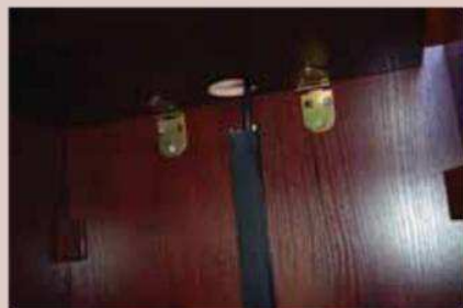
Attach the tilting projector shelf to the back panel using two butt hinges
