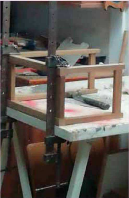
When you've assembled the construction and glued the joints in place, use a clamp to hold it all together while it dries
