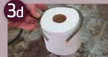
Cut two 350mm of 6mm round bar and bend a 135mm diameter circle
