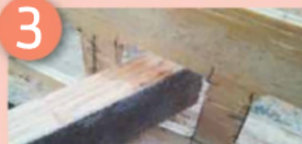
To simplify the sanding job, make a sanding stick that can easily get into those nooks
