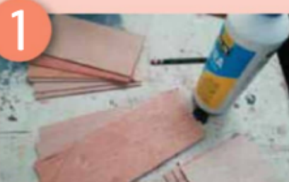
We recycled off-cuts of laminated wood, gluing them together to the 10mm thickness we required
