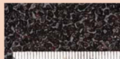
Medium-sized grit, in this case 60. Scale bar in mm
