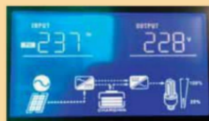
Input/output screen – showing solar panels charging the batteries and running the office
