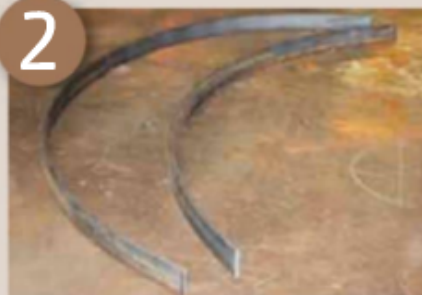
Bend the flat bar to form a half circle
