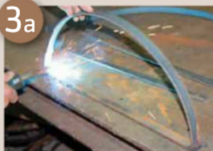
Bend the flat bar to form a half circle
