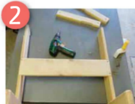
Fitting the legs, base and cross member
