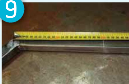
Measure intervals of 200mm for cross beam
