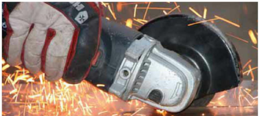
Always use appropriate PPE like gloves and safety glasses when operating an angle grinder
