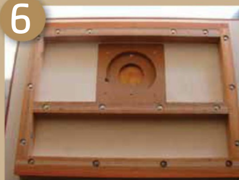
Bracing to prevent sagging
