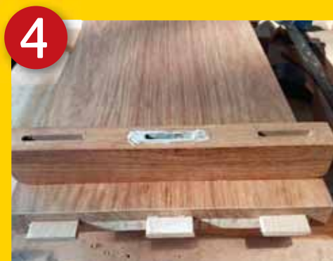
Gluing breadboard end
