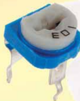
Variable resistor, called a potentiometer
