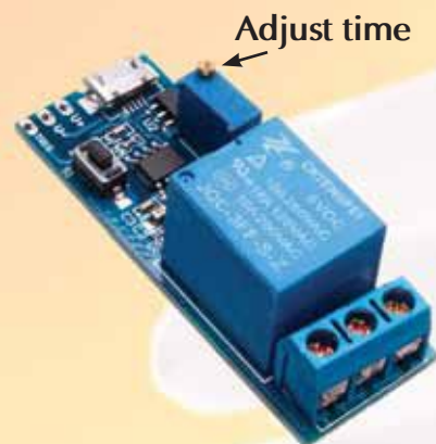
A timer relay board allows you to set the time a relay will be open once a signal is received
