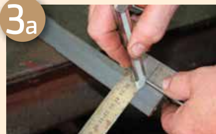
Measure for the cut-out joint
