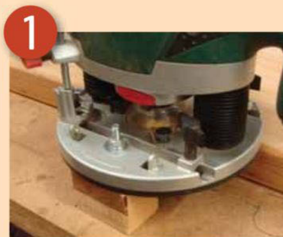
Stabilising a router
