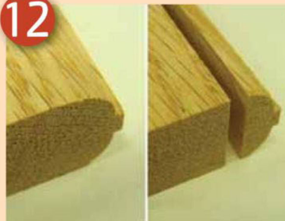
Making small applied mouldings
