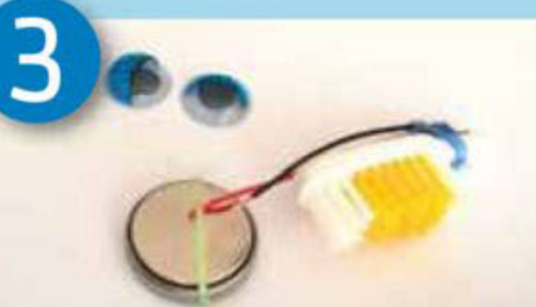
Secure one of the motor wires to the battery
