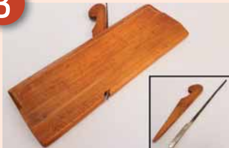
Wooden body and a matching profiled steel blade
