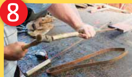
Fit the wood over the other end of the scoop to serve as the handle
