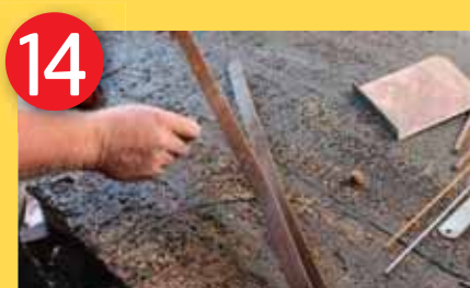
Measure 400mm downward from the bend and bend the flat bar in again to give it some spring action
