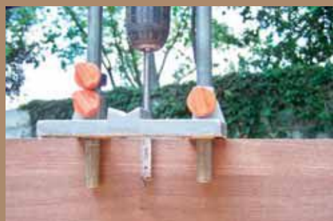
Our Wolfcraft comes with a set of collar adapters to ensure that the drill bit is precisely aligned with the posts
