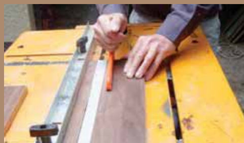
Set your table saw up to rip away the 30mm strip marked out in step 1
