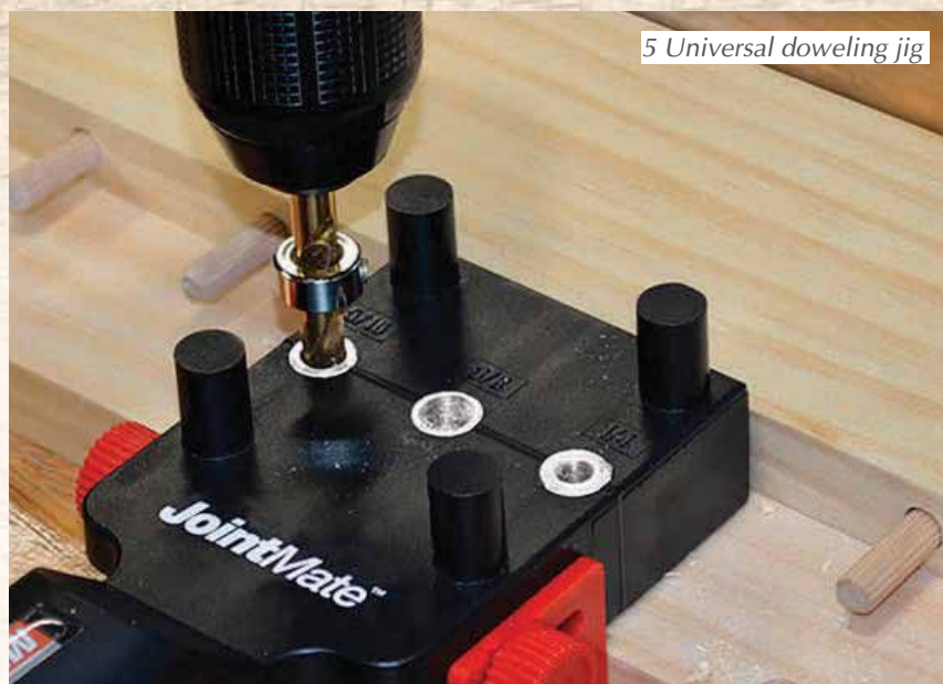
We used a Wolfcraft drilling attachment which allows accurate drilling
