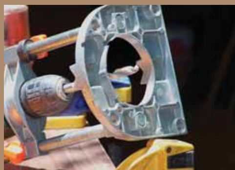
We used a Wolfcraft drilling attachment which allows accurate drilling
