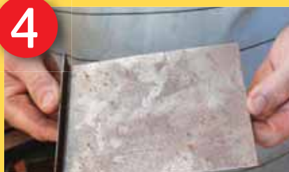
Make a 90° bend 20mm inwards on one of the 150mm sides
