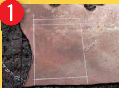
Mark out the rectangle on the sheet metal
