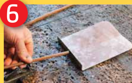
Weld a 760mm length of round bar to the scoop
