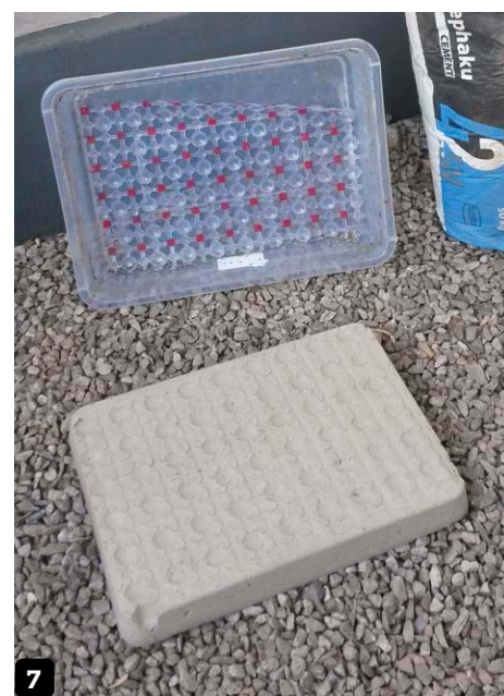
7 Leave the stepping stone in the mould for four days to allow it to dry before removing it
