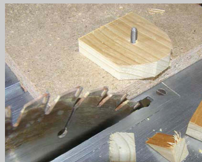
Drill a pilot hole in a block of wood and screw it onto the sled
