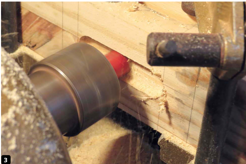
3 We used a 12mm router bit on our lathe to prepare the tenon at the base of the trunk to take the mortise of each foot
