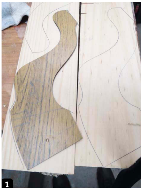
1 Begin with a plan. We had to laminate planks to get the right thickness
