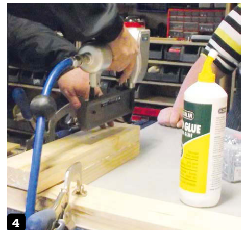
Each layer was attached to the next with glue and the insertion of screws and nails
