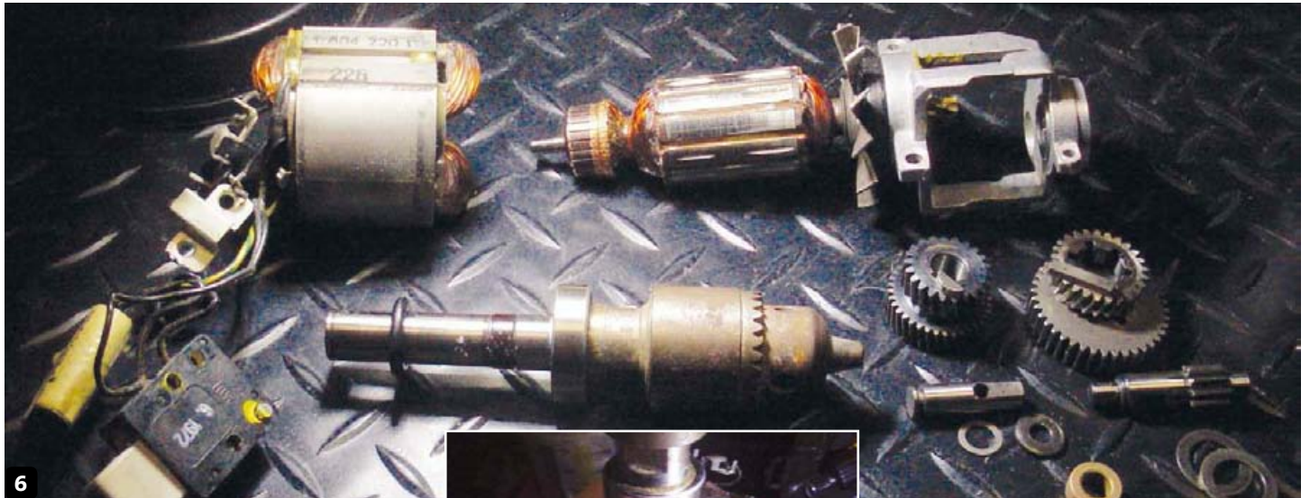
6 The basic components of the drill including the armature, windings, gears as well as the chuck and main shaft
