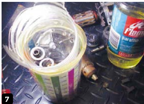
7 Washers, bushes and other small parts were washed in paraffin
