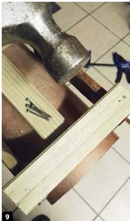
9 Nails can be used to secure the top and bottom frames
