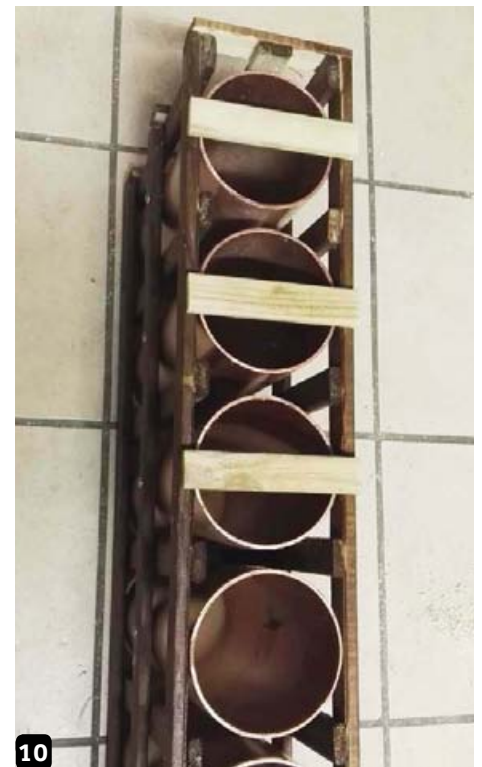
10 Use offcuts to create stoppers at the back side of the wine rack
