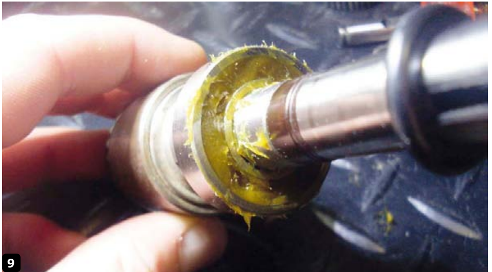
The bearings were repacked with fresh grease
