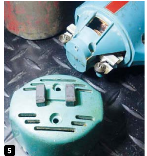
5 Removal of the brushes revealed worn out brushes
