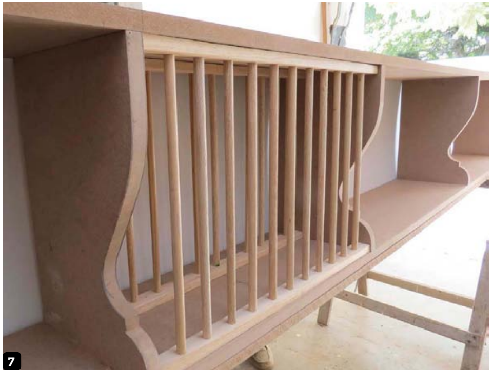
Fix the dowels in place with two screws in each support
