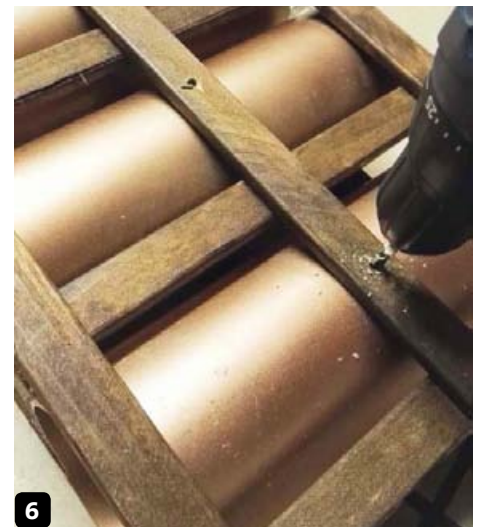
6 Line up the sections of pipe with the trellis and drill holes
