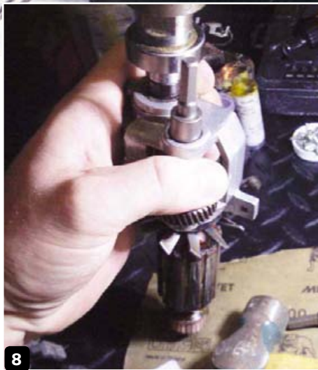
8 A hex drive was used to press bushes back in place after cleaning
