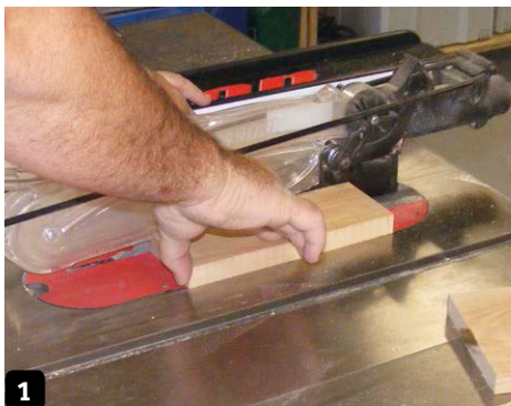
1 Rip the lengths of wood as per the cutting list
