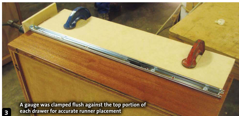
Mock up and testing of the drawer dimensions and trial fitment of the chosen rails
