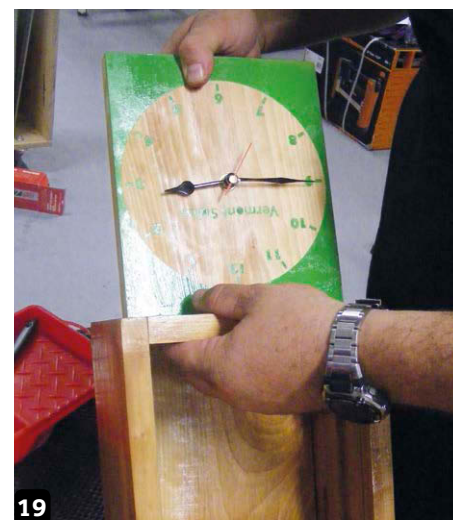
19 Slide the clock face into the carcass before fitting the base
