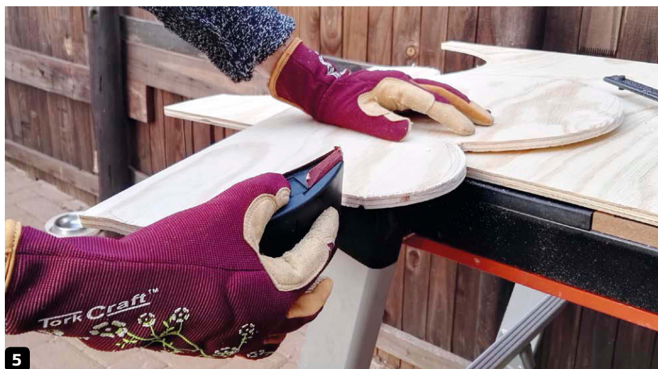
After the cloud and sun shapes have been cut, sand the edges with some fine grit sandpaper
