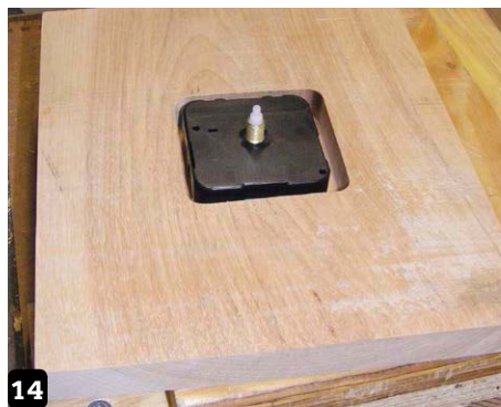
14 Fit the clock mechanism to the clock mount
