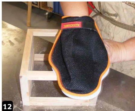
12 Use a hand sanding glove and smooth the clock carcass
