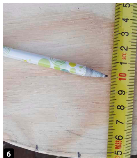
Measure along the curved edge above the sun and mark the spacing for the dowel sticks
