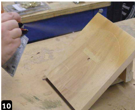
10 Use an airbrush to spray over the stencil and allow for about 15 minutes of drying time
