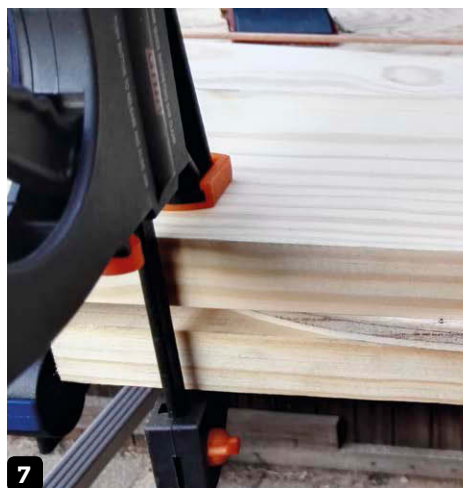
To prevent drilling into my hands I chose to clamp the 'sun' in-between two offcuts
