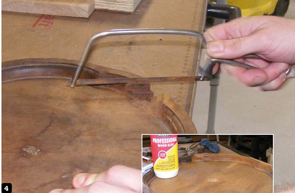
4 A hacksaw was used to cut away the ragged edges from the lip
