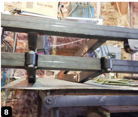
8 The end truck guide wheels were positioned inside the C-profile of the runway beam
