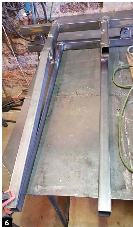
6 The end truck was placed on the workbench and bolted on one side before being welded on the other
