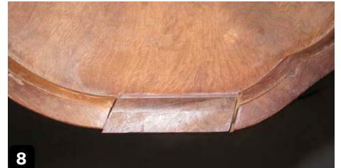
8 Some gaps remained on either side of the inserts
