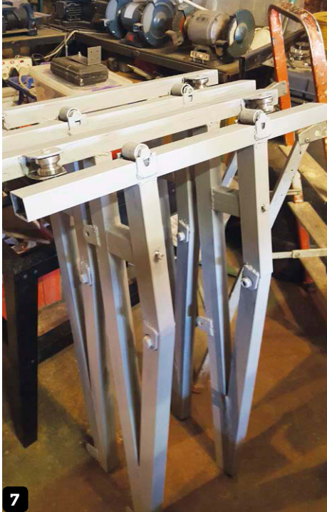
7 The completed end trucks, along with the guide wheels, form a triangle structure, enhancing stability of the crane
