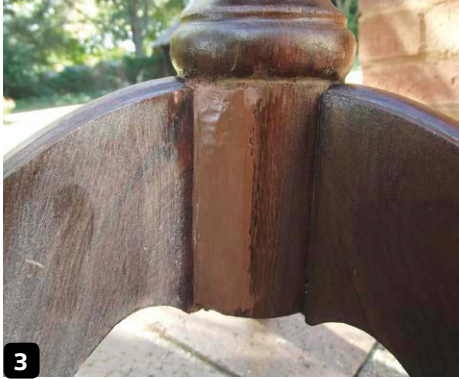
3 Flexible wood filler was used to fill the gaps where wood was missing
