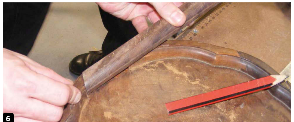
6 A length of leadwood was placed on top of the lip to gauge the angle and lengths required
