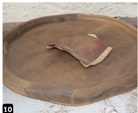
10 The inserts were sanded by hand in an attempt to match the existing cove more accurately
