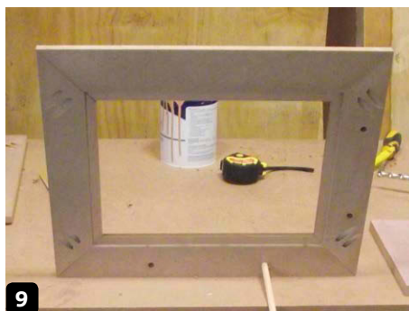
9 Cut two dowel rods as supports for the frame
