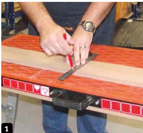
1 Mark the length to be cut in half
