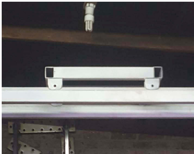
4 The end truck was 600mm long and the extensions seen here form part of the structure needed for the addition of the guide wheels
