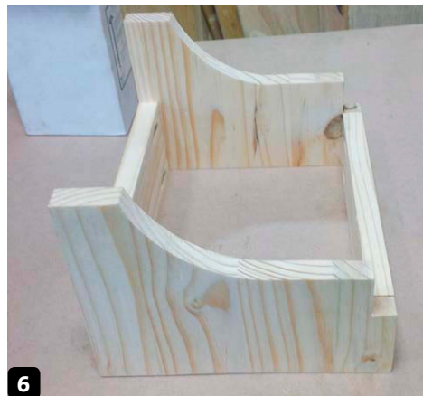
6 The assembled lower step will fit inside the main frame
