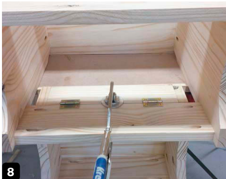
8 Hinges allow the lower step to fold into the top step to save space
