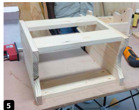
Flip the stool over and fix the rear support rails to form a frame
