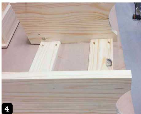
The first step in assembly is attaching the front support rails to the larger sides of what will be the top step
