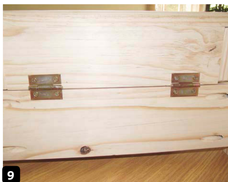
9 Ensure that the hinges are 30mm in from each end
