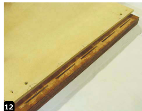
12 Biscuit slots in underside of top
