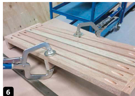
6 The side and middle pieces were glued onto the slats and held in place with sash clamps
