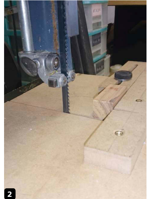
2 The top and bottom half of the pen was trimmed from the machined 'strips' of wood
