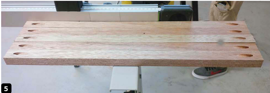
5 Once the pocket holes were completed the slats were laid out before the insertion of screws
