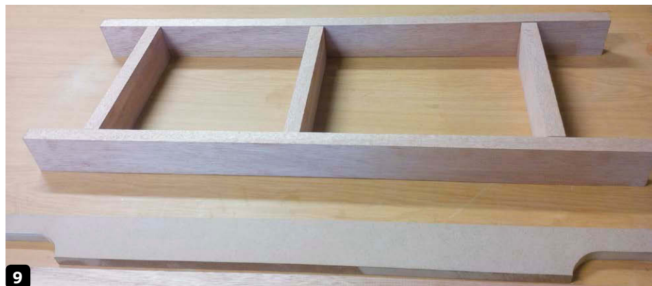
9 The 75mm overhang was cut using a jigsaw and neaten on the router table
