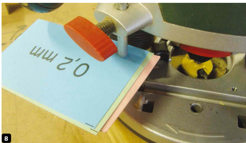
8 Setting jointer depth of cut
