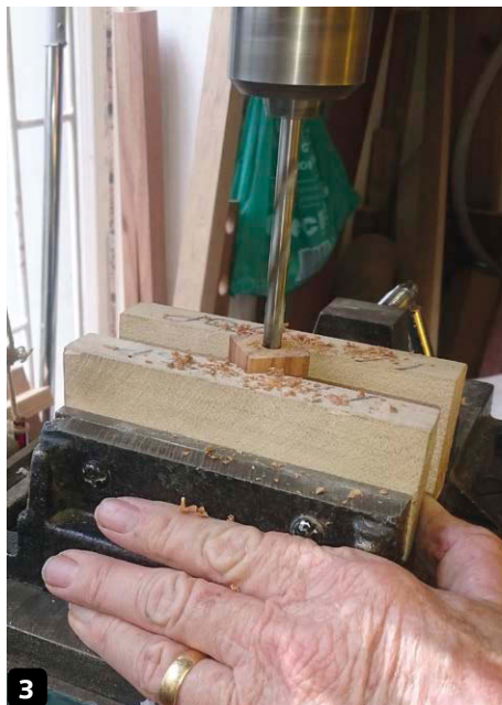
3 A hole for the pen kit insert is drilled down the centre of each half of the pen
