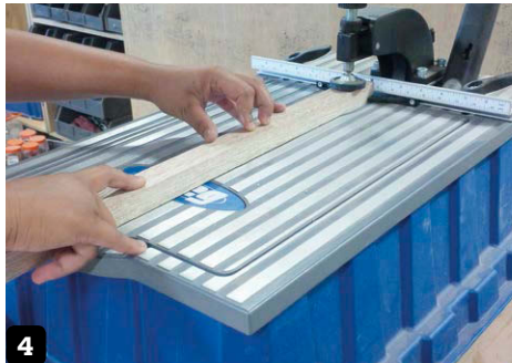
4 A Kreg jig was used to create the pocket holes for each slat
