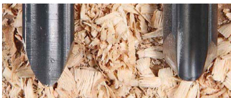
▲ Spindle gouges (left) have a profile that is flatter than bowl gouges. Bowl gouges (right) have a round profile, allowing for a deeper flute
