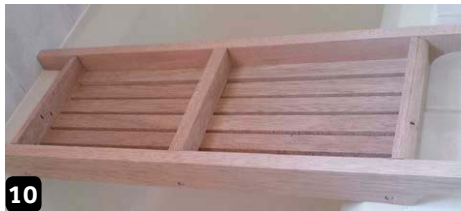
The finished pieces were screwed together
