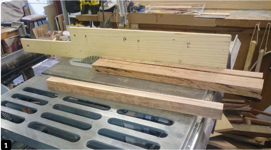
1 A table saw or bandsaw is used to cut the sizes needed from a larger piece of wood
