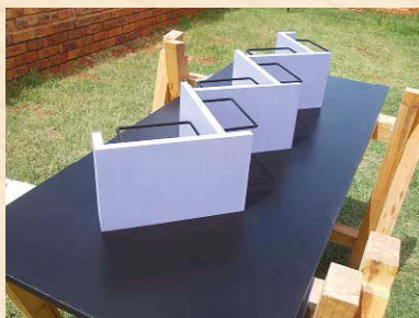
▲ Ian De Jager received the most 'likes' for his media storage centres for compact disc storage and won himself a Kreg Jig Master System (K4MS). The shelves were made from 16mm MDF and were painted with Rust-Oleum, and a sheet of black laminated pressed wood formed the base
