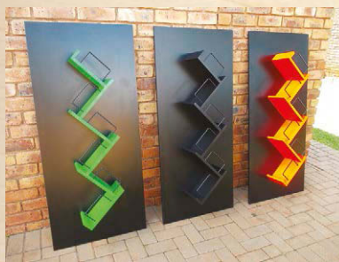
▲ Ian De Jager received the most 'likes' for his media storage centres for compact disc storage and won himself a Kreg Jig Master System (K4MS). The shelves were made from 16mm MDF and were painted with Rust-Oleum, and a sheet of black laminated pressed wood formed the base
