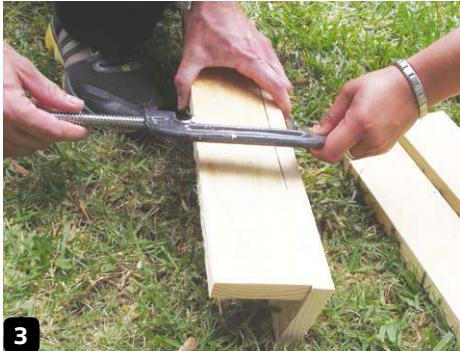
3 Our G-clamp came in handy when butt jointing the base to the sides
