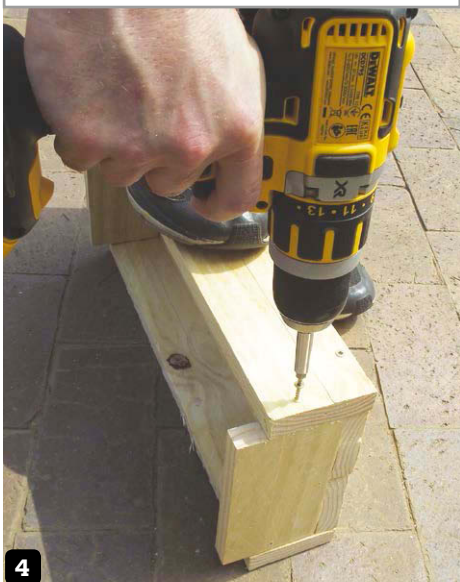
4 The shorter lengths are inserted in-between the sides creating the bottom of the box
