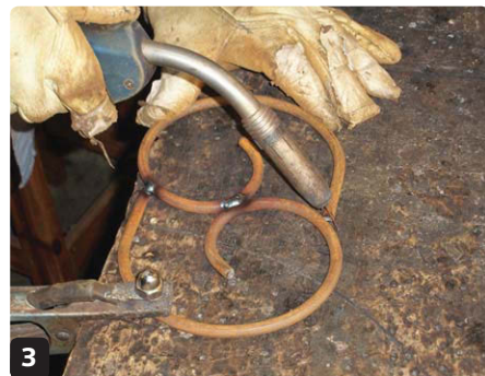
3 Weld the feet together
