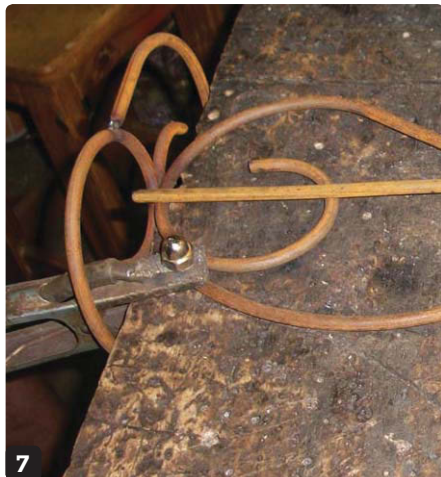
7 Weld the 470mm length of round bar onto the back of the lamp's body
