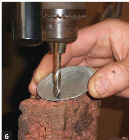
6 Drill a 6mm hole in the metal cap
