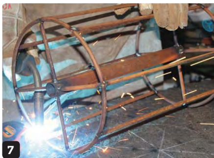
7 Position the axle correctly and weld it onto the four round bar pieces on each side
