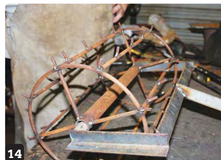
14 Weld the 44 spikes onto the roller
