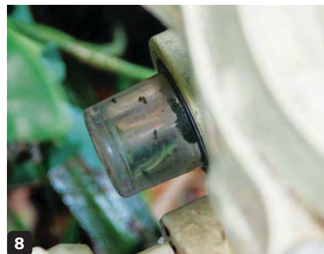
8 Do a backwash water clarity check
