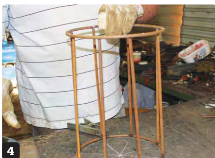
4 Weld the second ring onto the other ends of the round bar lengths
