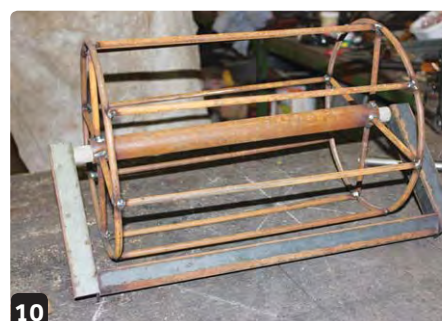
10 Weld the entire bracket onto the outer ends of the 20mm pipe
