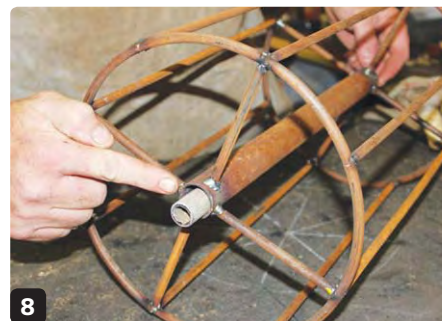
8 Slide the 20mm pipe into the axle
