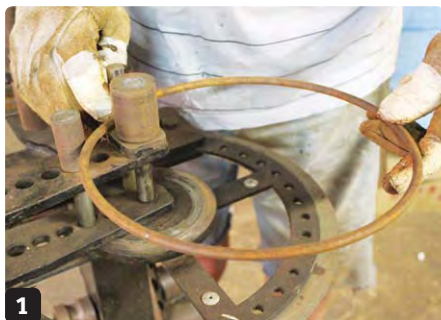
1 Roll two rings from the 800mm lengths of round bar
