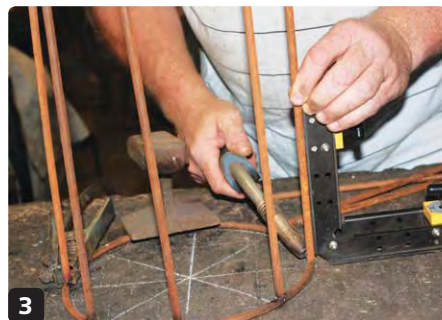
3 Weld the eight 380mm lengths of round bar onto one ring
