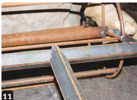
11 Cut one end of the 700mm angle iron at 45° and weld it in place in the centre of the 470mm angle iron
