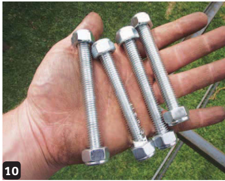
10 Cut four pieces of threaded bar, each 90mm long
