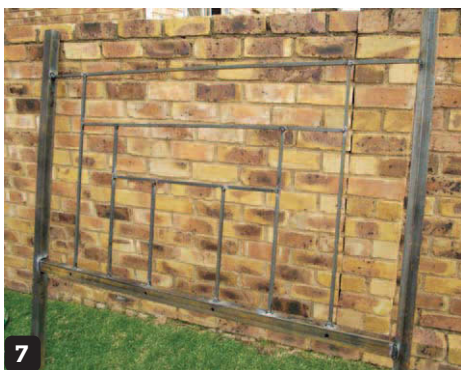
Use the 12mm square bar lengths to construct the headboard design in-between the two pillars
