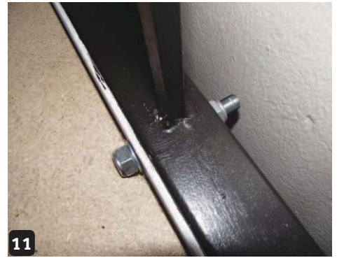
11 To assemble the bed simply fasten the headboard and the frame to each other by means of the threaded bar
