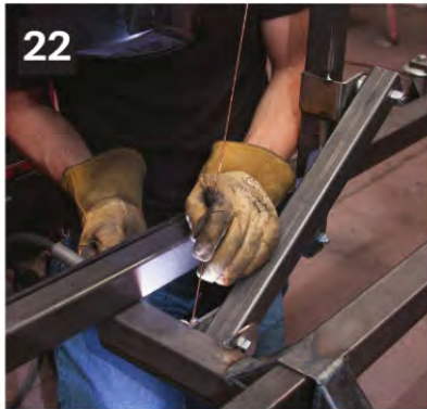
▲ After testing the operation of the lift mechanism, I welded all of the brackets.
