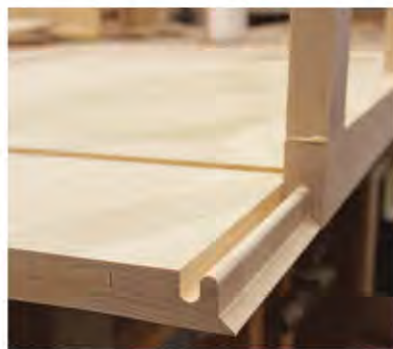
▲ A locked miter joint consists of male and female components that, when glued together, prevent slipping.
