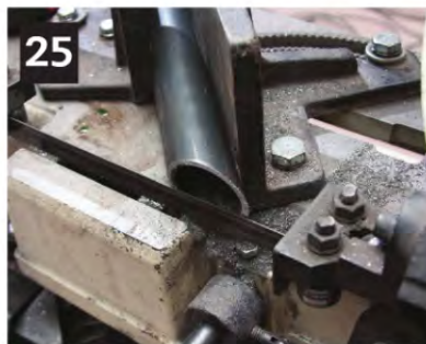
▲ The handle is made of 1/8-in. x 1-1/2-in.-dia. round tube. I mitered the ends using a horizontal band saw.
