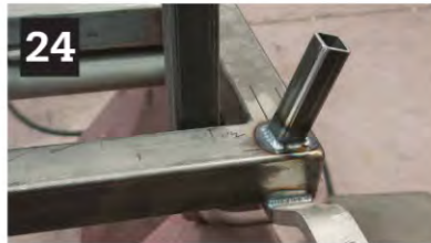
▲ To make mounts for the removable handle, I cut two 3-in.-long pieces of 1-in. square tubing and angled one end 15 degrees; then I welded them to the base section.
