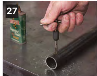
▲ To lock the handle in place during use, I drilled and then tapped 1/4-20 threads 1 in. from the end of the tube.
