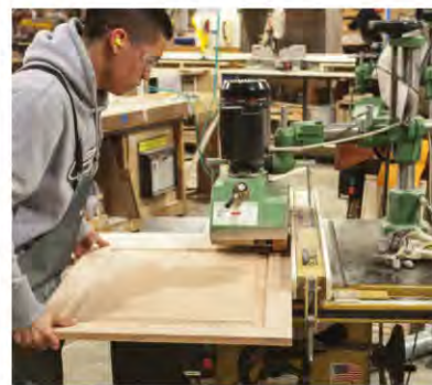
▲ The assembled door frames and panels are sanded smooth and level with a special belt sander.
