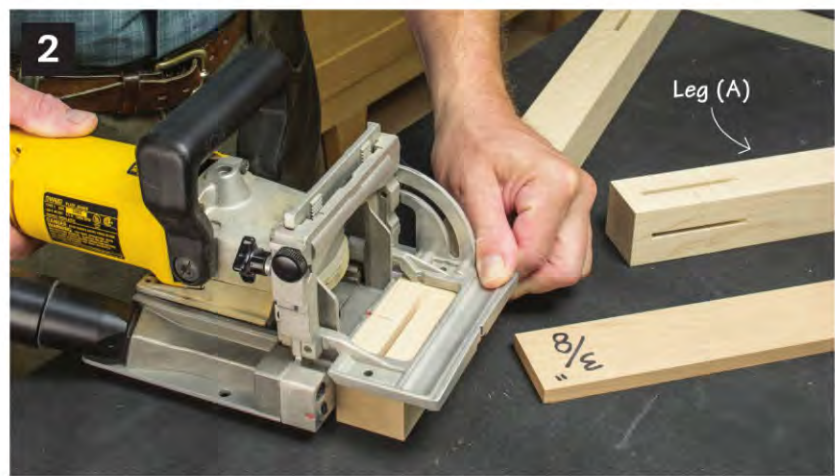
▲ Cut the offset biscuit grooves in the legs (A). Don't change the height of the biscuit joiner's fence, and don't use the spacer. This setup creates the 3/8-in. offset of the parts.
