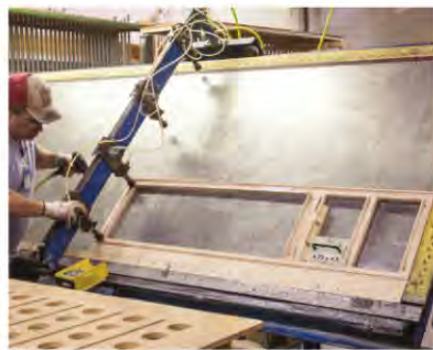
▲ Face frames are built on large-scale jigs. Spacer blocks ensure accurate placement of components, and pocket screws are used to hold everything together.
