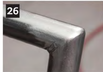
▲ I welded the upper corners of the handle and then ground, radiused and sanded them smooth.
