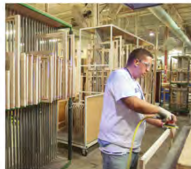
▲ Once the glue has cured, each face frame is inspected and sanded. Large industrial sanding machines smooth the faces; the edges are sanded by hand.
