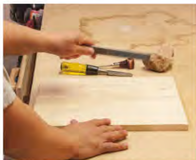
▲ Distressing is done by hand using a variety of old-fashioned implements such as rocks, chisels, files and awls. As a result, each panel is unique.
