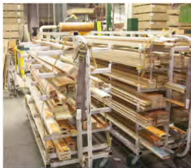
▲ Stacks of plywood and sticks of hardwood will soon become cabinet components once they are cut to size and milled with profiles.
