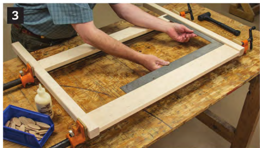
▲ Assemble the base sides. Make sure the frames are perfectly square. This is very important to the success of the table. I use an old framing square that I know is exactly 90 degrees.
