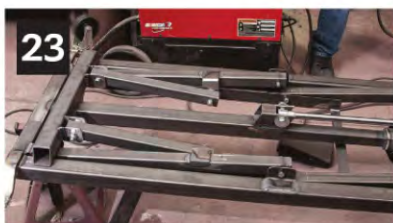
▲ To complete the final welds, I turned the cart over. (This enables you to see the entire lift-arm assembly and how the parts work together.)
