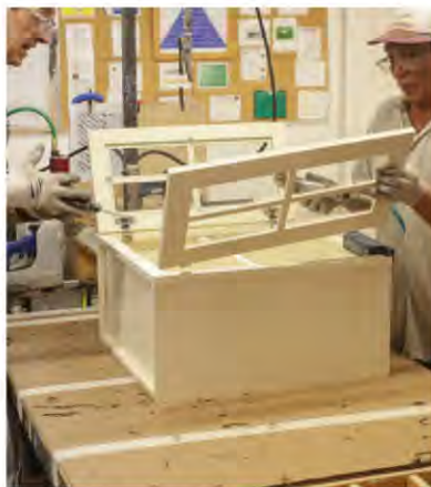
▲ Two-man teams assemble all of the components into cabinets. Here the doors are being installed on a wall cabinet.
