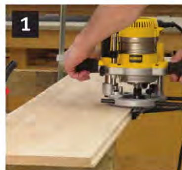
▲ Rout the rabbets in the rear edges of the sides (A). Use a straight router bit and an edge guide. Make the cuts 1/2 in. deep x 1/4 in. wide, and cut from end to end.
