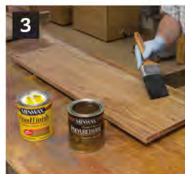
▲ After applying the stain with a rag and letting it dry for a couple of days, brush on three coats of polyurethane. Smooth the finish between coats using 220-grit sandpaper.
