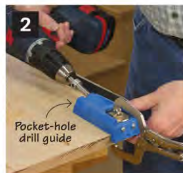
▲ Drill the pocket-screw holes in the undersides of four of the shelves (B), the top side of the cubby shelf (B) and the backs of the cross braces (D) and toe kick (E).
