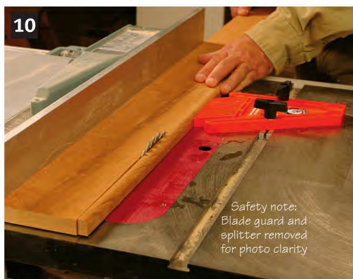
▲ Next, rip the base shoe molding to its final 3/4-in. width. Repeat the routing and ripping process to create multiple pieces of molding. You can use the same technique with any thin stock molding.
