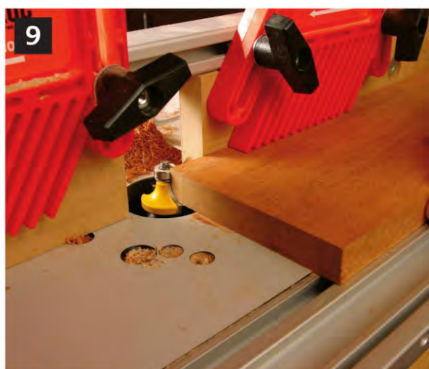
▲ To make the base shoe molding, first rout a 3/8-in.-radius roundover on a piece of trim stock lumber that is wider than the final base shoe width.
