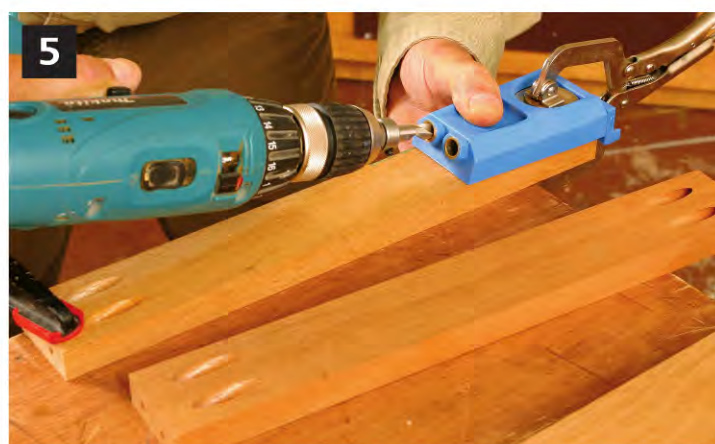
▲ Use a stepped drill bit and pocket-hole jig to drill the pocket-screw holes in the rails.
