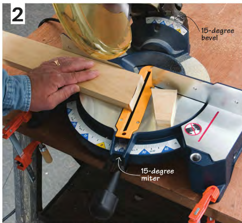
▲ Set your miter saw to cut a 15-degree miter and bevel. Cut the ends of the legs at this compound miter angle.
