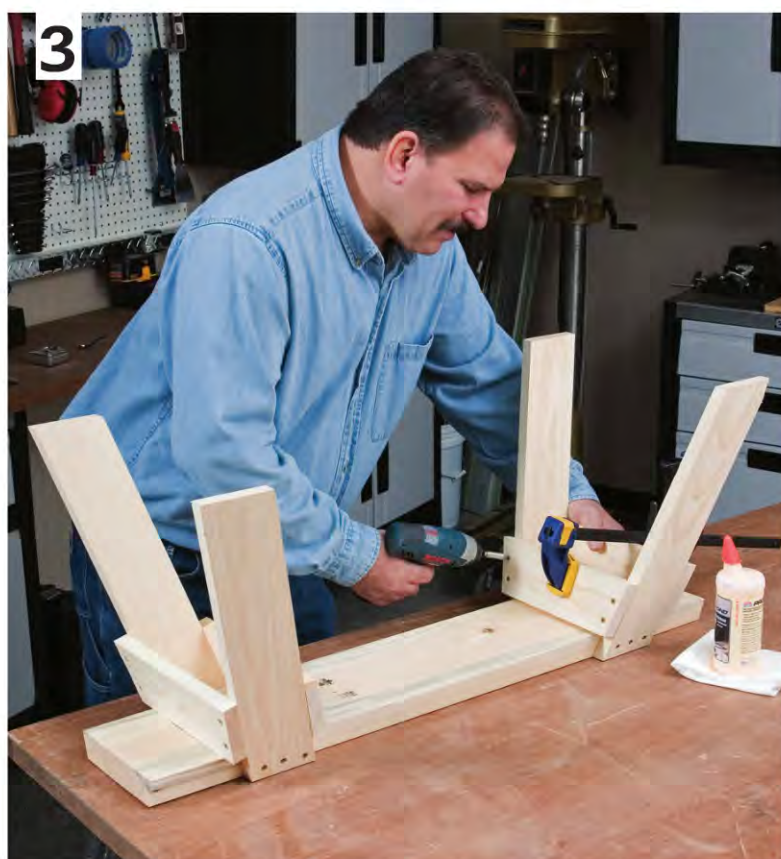
▲ Attach the legs to the top board with 2-in. screws and then attach the gussets to the legs with 2-in. screws.
