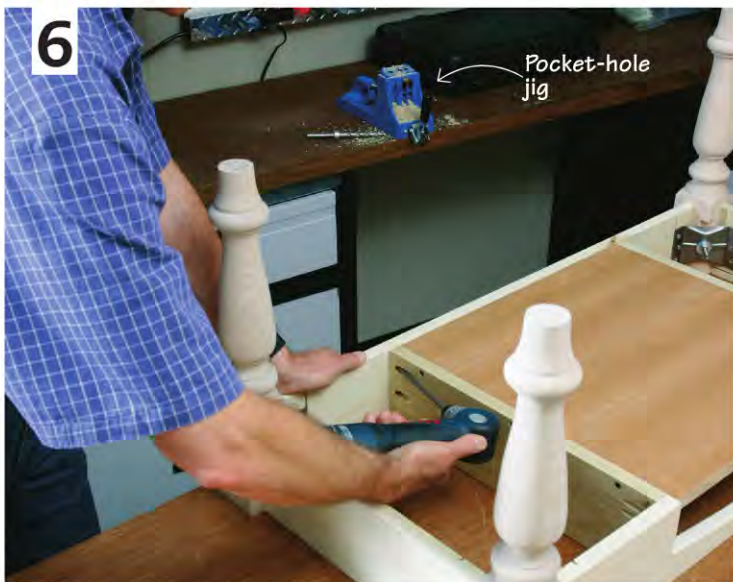
▲ Fasten the brackets to the skirt boards with No. 8 x 3/4-in. wood screws. Then fasten the legs to the brackets with washers and bolts.
