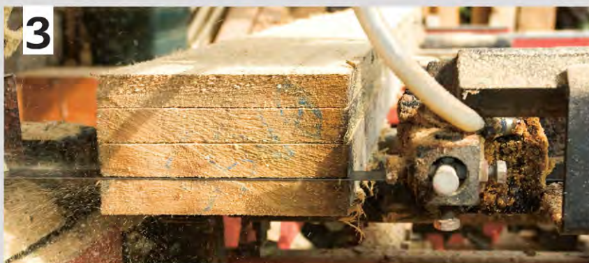
3 ▲ Beams are milled on a band saw mill into 1-in.-thick boards.
