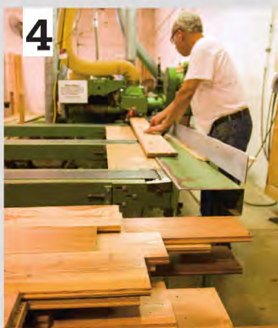
4 ▲ A commercial mill then planes the boards to final thickness and cuts the tongue-and-groove edges.
