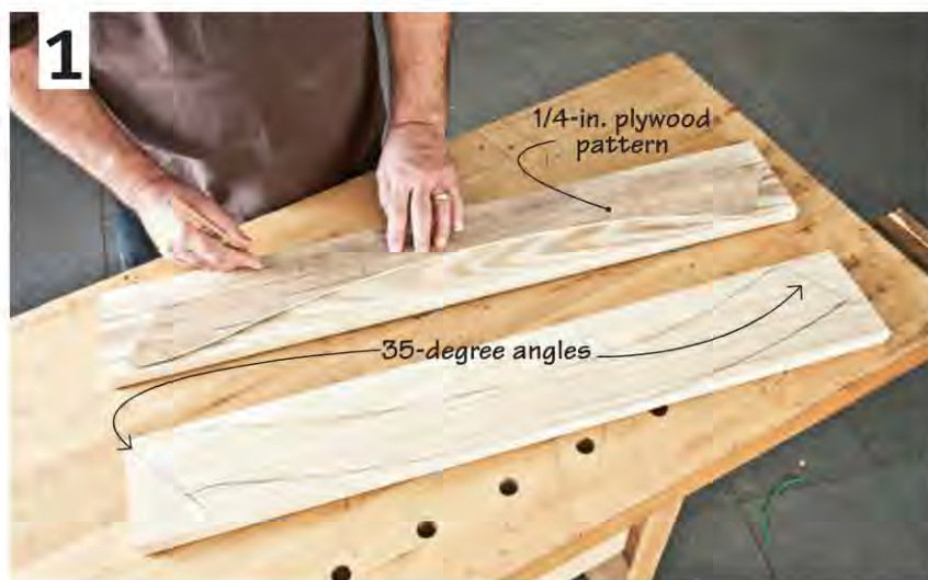
▲ Make full-size templates for the curved pieces so you can trace the contours on the actual parts.
