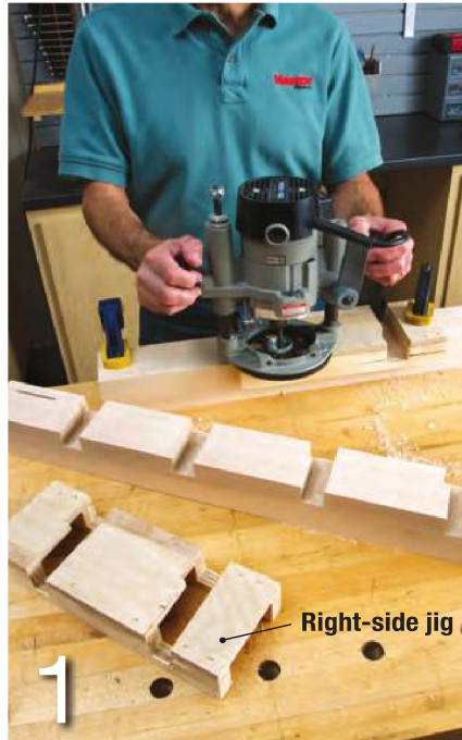
1 Use a jig (see illustration, p. 10) and a router with a straight bit and a guide bushing to cut the bench-dog holes in the two outside bench-top laminations.
