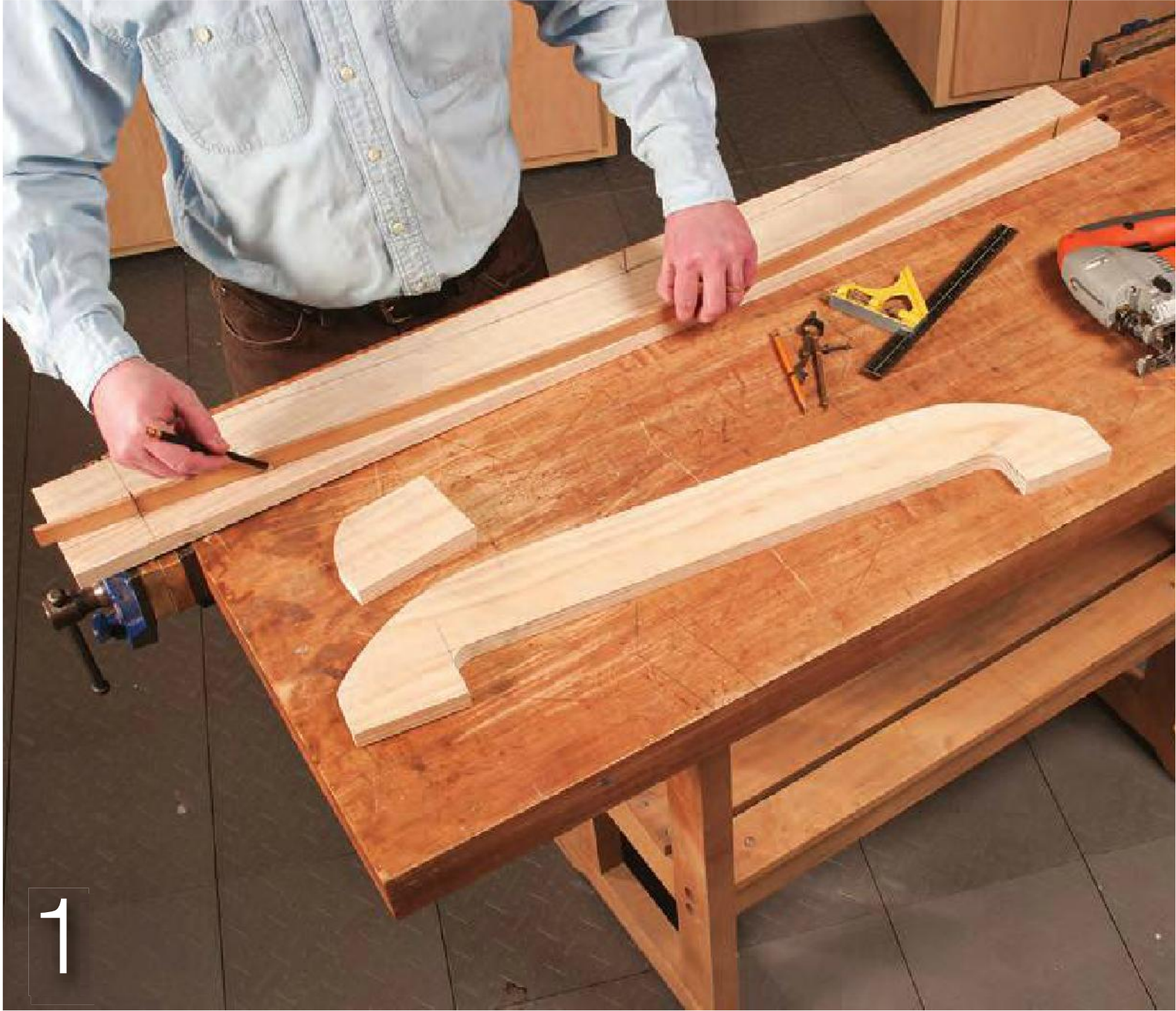
Make templates for the cross-support ends, feet and trestle. Flex a thin piece of scrap wood to lay out the arc profiles on the top and bottom of the trestle.
