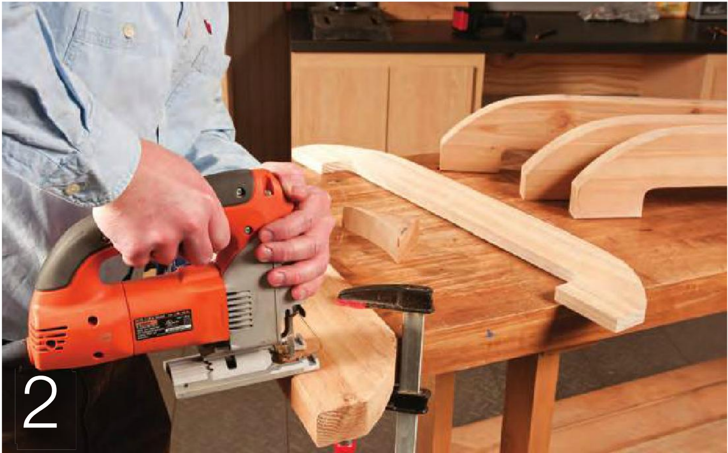
Trace the templates on the actual stock and then cut the parts with a jigsaw. Use a file and sandpaper to remove the saw marks and ease the edges.
