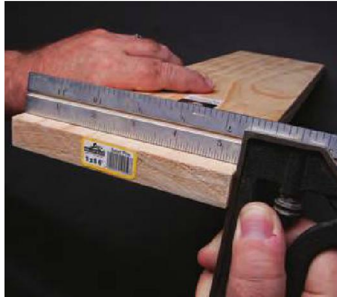
Dimensional lumber never matches the printed measurements. This 1x6 board actually measures 3/4 x 5-1/2 in.
