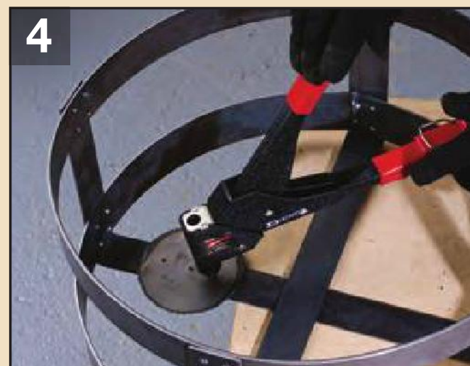
4 Once you've attached the top hoop to the straps, use rivets to fasten the candle bases to the straps.
