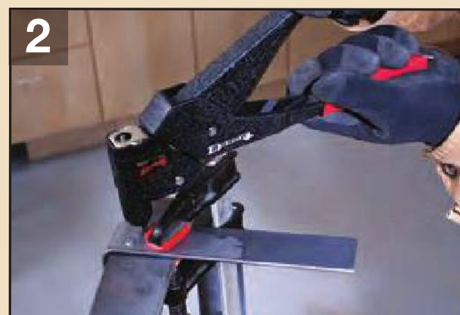
2 Clamp the bottom hoop and the support straps together. Use the holes you've already drilled in the straps as guides for drilling holes through the hoop. Insert the rivet into the hole, slide the rivet gun onto the rivet's mandrel and squeeze the gun handles together.
