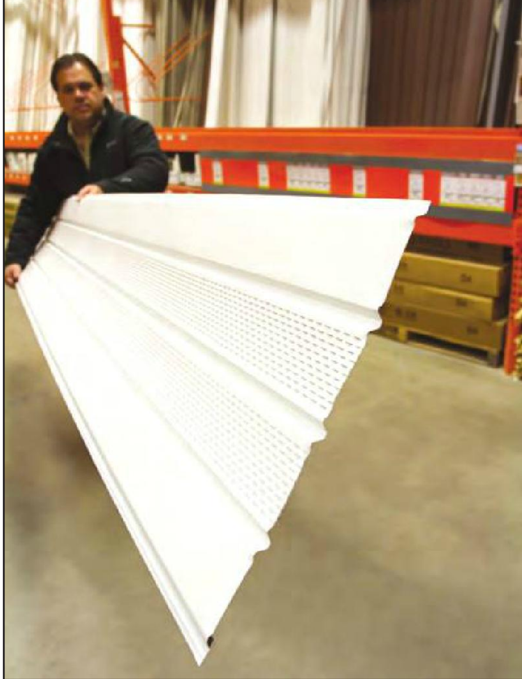
Vented aluminum soffit panels are sold in 12-ft. lengths and have thousands of tiny holes that allow air to flow up into the home's attic space.
