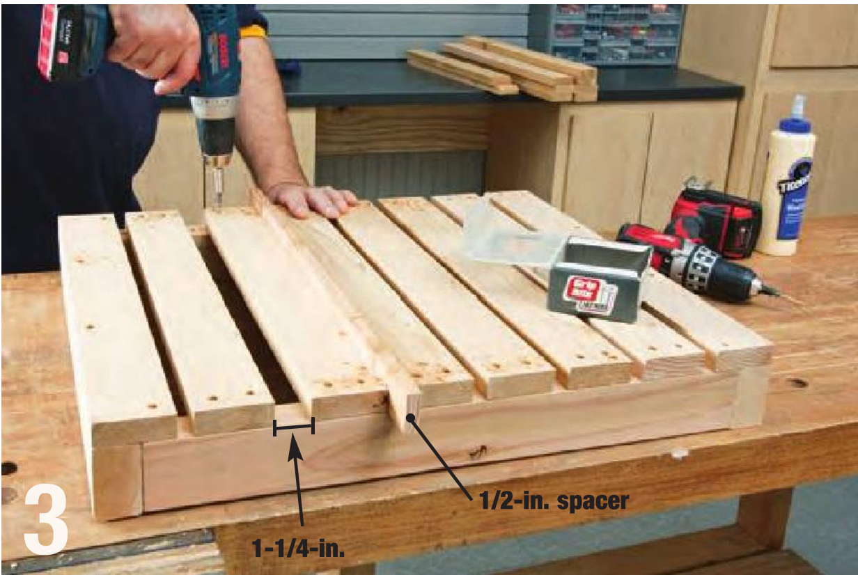
When attaching the seat slats to the side seat supports, use a 1/2-in.-thick spacer. Drill pilot holes and 1/4-in.-deep counterbores; then drive 1-1/4-in. screws.
