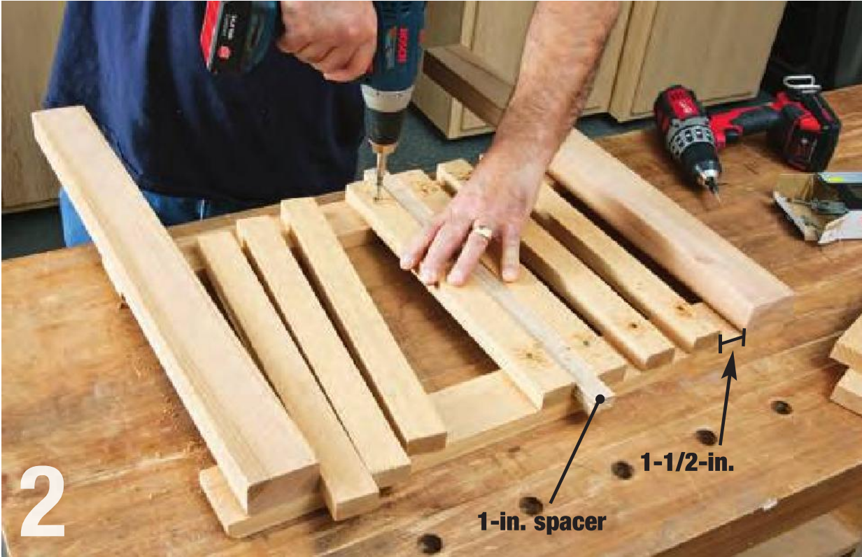
For uniformity when attaching the side slats, use a 1-in. spacer between them as you bore the pilot holes and drive the screws. Tip: To save time changing bits on one drill, use two drill/drivers: one to bore and one to drive.
