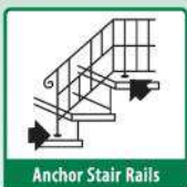
Anchor Stair Rails
