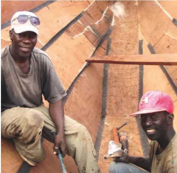
Senegalese boatbuilder and the internal caulking
