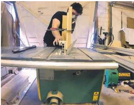
4 The undersides of the desk top were cut vertically to achieve the required mitre angle
