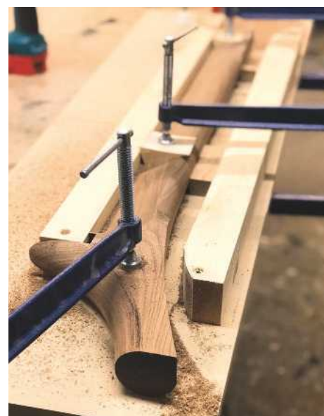
Softwood jig to support the router at the correct height when cutting the rounded profile of the leg
