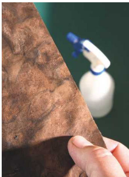
9 Burr veneers are particularly prone to buckling when they are dry and, being brittle, they need dampening with water before they can be flattened
