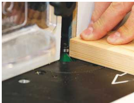
14 Before making any cuts, check the fence is correctly positioned and the height is set
