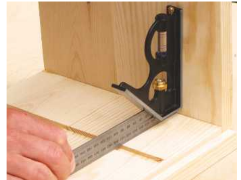
15 Check everything is square before nailing the joints, adjusting the clamps if you need to
