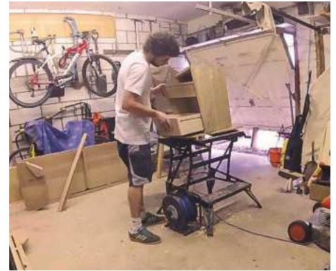
29 Here the drawer slides are being screwed to the inside of the cabinet. Nylon tape was later added to the top of the slides to reduce friction
