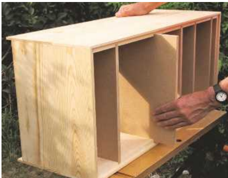
19 Make the vertical dividers from 12mm MDF. Slide these into place without using glue
