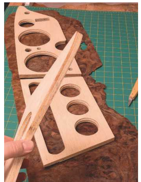
10 More complex shaped groundwork like this dashboard can be glued up before details are cut in the veneer
