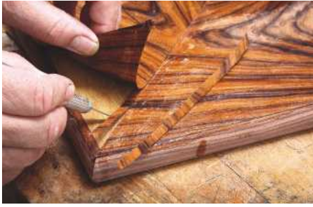
4 Pre-cut oversize the veneer is laid in hot glue, cut through with a craft knife then lifted at the edge to remove offcuts
