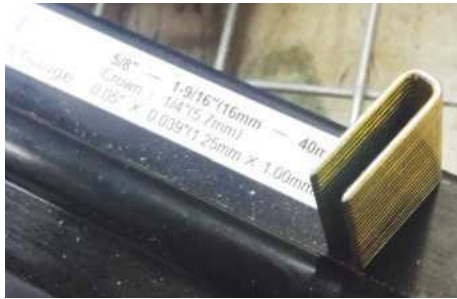
13 The 19mm narrow crown staples used
