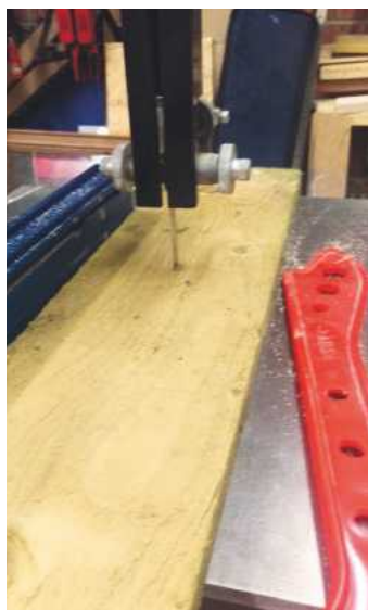
4 Resawing gravel board to give 75mm wide planks
