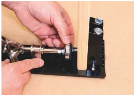
4 The toggle clamp features an easily adjustable pressure foot with a soft rubber facing
