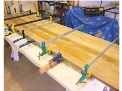
3 The desk top glued up and clamped together
