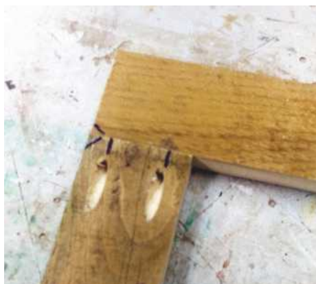
11 The joint once assembled
