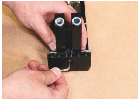
2 The guides can be adjusted using the hex wrench. A scale on the jig allows quick setting to specific centres
