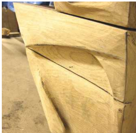
31 In tighter areas, such as the pocket in the top drawer, I used a Dremel with a carving burr
