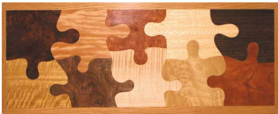
14 Bandsawn veneer sheets have been scrollsawn to make this interlocking pattern
