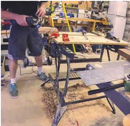
30 Starting to sculpt the drawer fronts using a grinder fitted with a Kutzall carving disc
