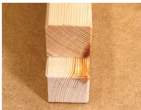
18 The legs can also be left square on the top edges. A chamfer on the bottom helps prevent the legs from splitting away if the piece is dragged along the floor
