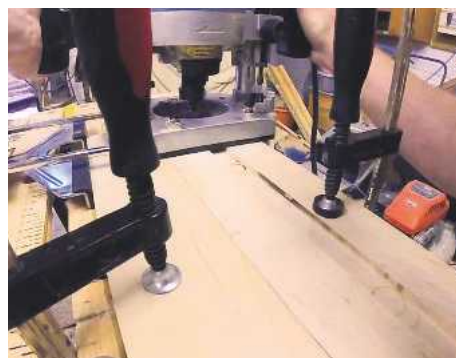
26 Routing a dado for the drawer slide to sit in
