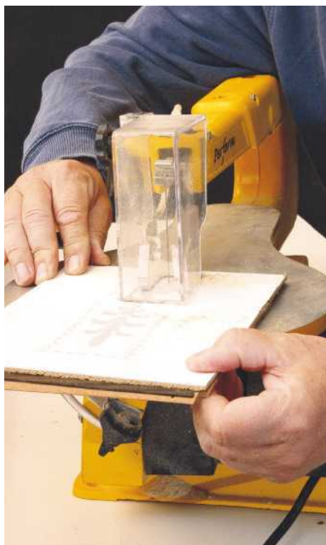
13 Multiple layers of veneer can be cut with a fine-bladed scrollsaw
