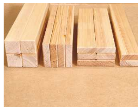
19 The components should now have the end-grain and long edges chamfered, ready to go to the pocket hole stage
