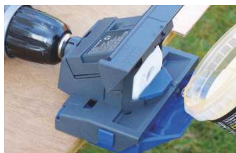
Before grinding it's necessary to fill the trough with water – a maximum level line helps to prevent overfilling
