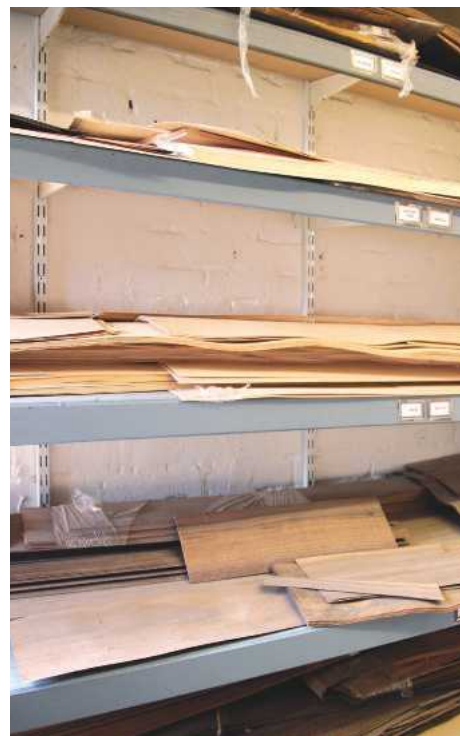
2 Veneer sheets, typically 0.6mm thick and 50mm to 400mm wide, are bought and stored in the sequence in which they were cut
