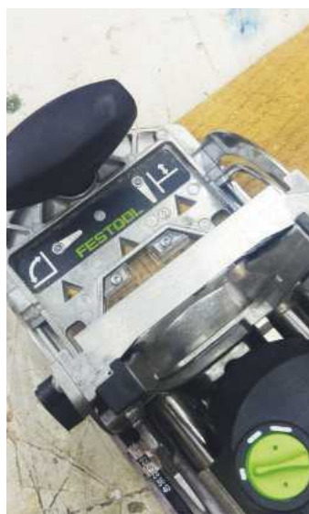
5 Cutting the rail mortise
