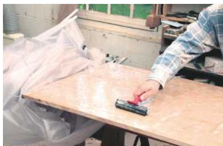
11 Glue is applied to a large substrate board using a rubber roller
