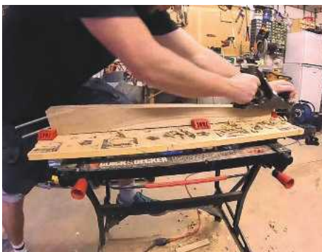
10 Planed smooth after tapering on the table saw
