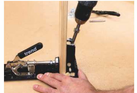
6 The drill should be withdrawn occasionally, which will help prevent the waste building up
