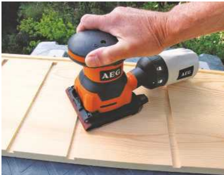
13 It's easier to sand the inner surfaces before gluing the carcass sections together
