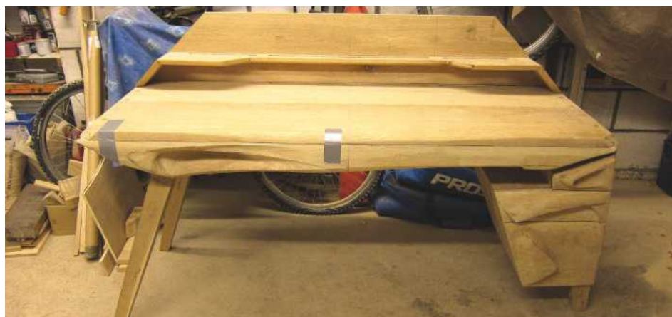
39 Hand tools (block planes, spokeshaves and rasps) were then used to refine the form before finish sanding
