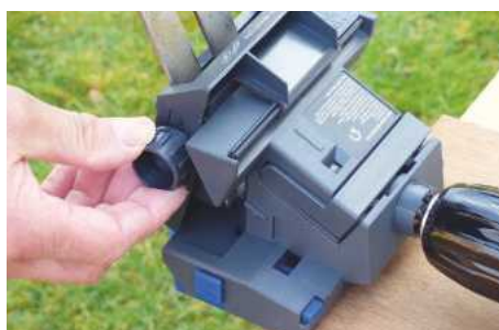
The blade holder is hooked over the rail and you insert the blade, which is clamped firmly and tightened with a knob
