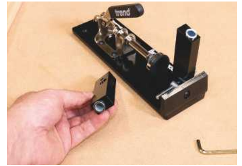
3 The guides can also be removed for use in repairs, to work in situ, or on thinner stock
