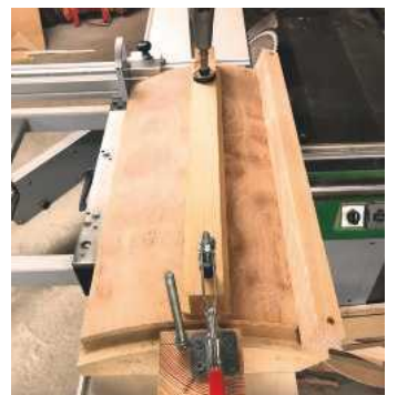
Jig made from the original curved former, which clamps the panel in position when cutting it to width
