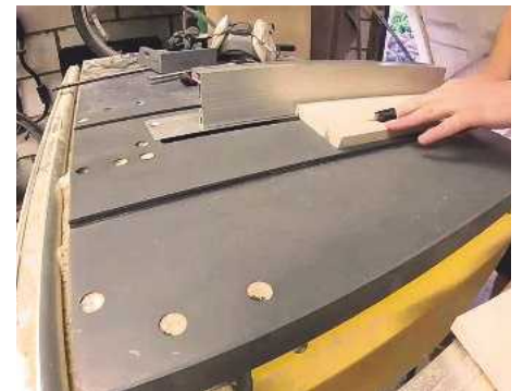
25 Groove cut for floating drawer bottom
