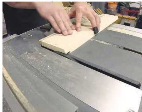
24 Rebate cut by multiple passes on the table saw
