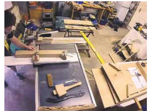
9 The legs were clamped to the jig and run through the table saw to cut the tapers
