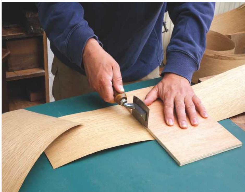
1 A veneer saw run against a straight edge is ideal for cutting across the grain
