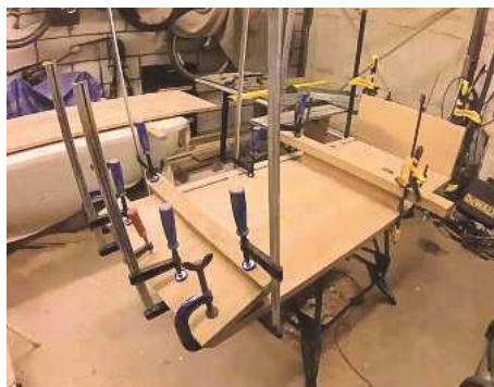
11 Both sides and supports glued in place
