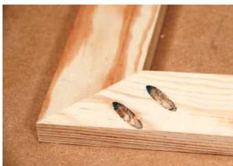
10 Other joints, such as mitres, are equally easy to secure with a couple of fixings from the unseen face
