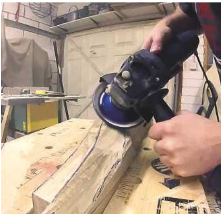
30 Starting to sculpt the drawer fronts using a grinder fitted with a Kutzall carving disc
