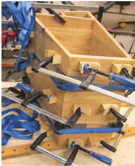
21 Glued blocks allowed the clamps to work properly. These were later chiselled off
