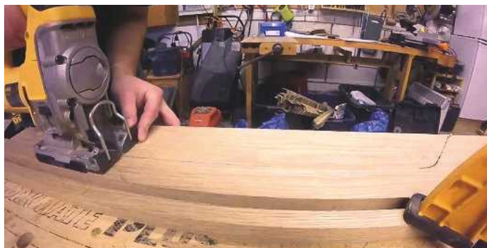
14 A section was cut out to allow a PC monitor to sit within the shelf
