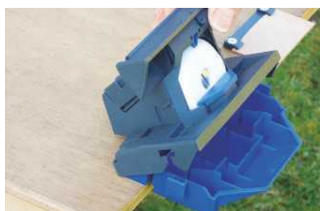
This incorporates a water trough and enables the wheel housing to be clipped into place
