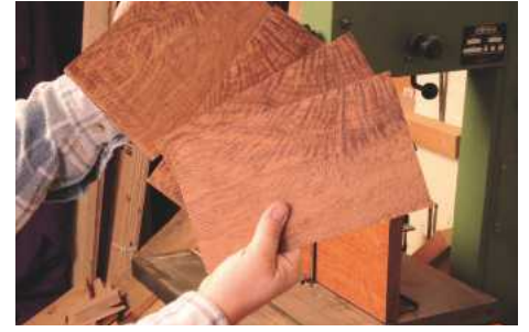
6 Veneers cut on the bandsaw to a thickness of 1.5mm
