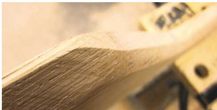
16 The chamfer along the shelf front was refined using a spokeshave and files
