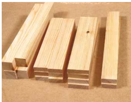
12 The cut sections should now consist of four legs, six short slats and four aprons of the same length, plus two longer slats
