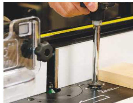
13 Fit a chamfer cutter into the router table and adjust the height to take a very fine cut; this will ease the component edges
