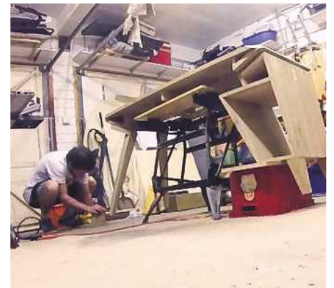
23 Bolts go through the top of the cabinet and into the underside of the desk top. Here I am also marking up to the required height
