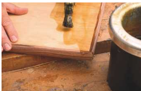
3 Traditional hot animal hide glue being spread on a plywood substrate with lipped edges ready to take the veneer
