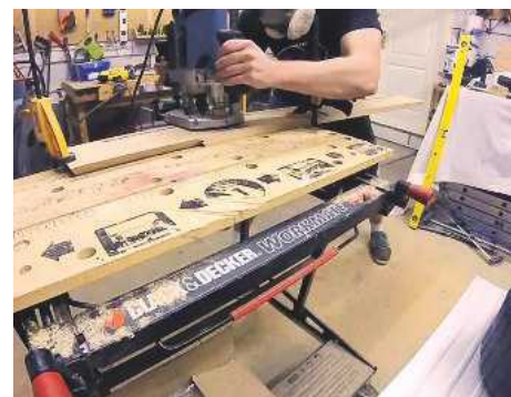
13 Routing the cable channels
