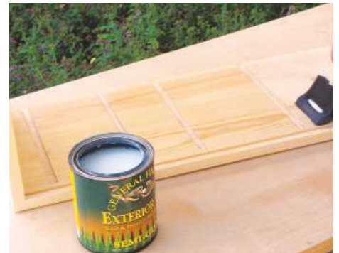
21 Finish the interior with a suitable exterior varnish. Yacht varnish is best for the outside of the box
