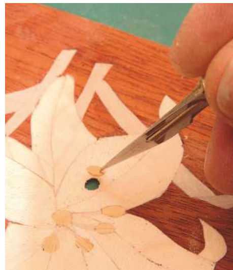
16 In order to build up a picture, individual components of the marquetry pattern are inserted and glued one inside the other
