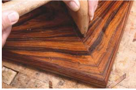
5 The joint is finally pressed down firmly using a veneer hammer
