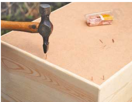
22 The rear panel is from 6mm MDF. Cut it to size and fix it to the rebate with hardboard pins
