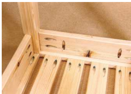
8 Viewed from below, the pocket hole configuration shows how they secure the various components
