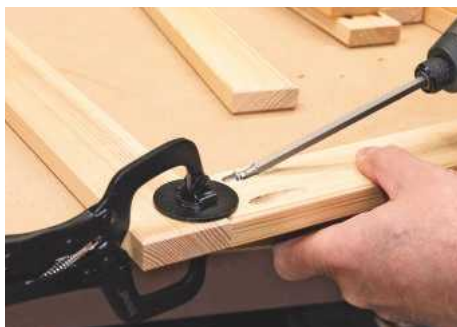
7 The face frame clamp ensures stock of the same thickness is perfectly flush once screwed together
