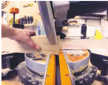
5 A compound mitre was cut at the top of the legs, allowing them to splay out
