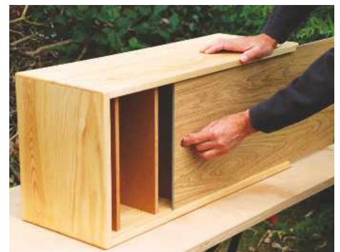
24 Check the front panel slides properly and drill a 22mm diameter finger hole
