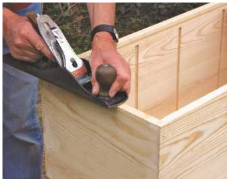
17 Clean up excess end-grain from the lap joints with a plane, then shoot the front and rear edges
