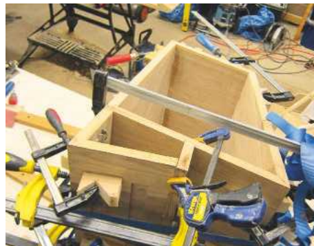
22 To add strength, three dowels were later drilled and inserted across each corner. The spacer sits in the recess shown in the bottom middle of the photo and holes were later drilled to allow bolts to connect the cabinet to the desk top
