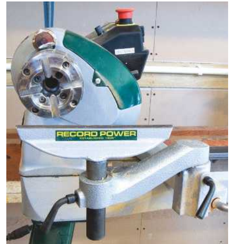
The headstock swivelled through 90° for larger work, and the toolrest fitted with an additional crank
