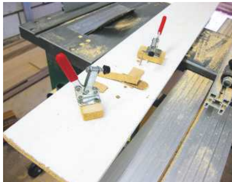
8 I created a simple tapering jig from scrap timber and toggle clamps
