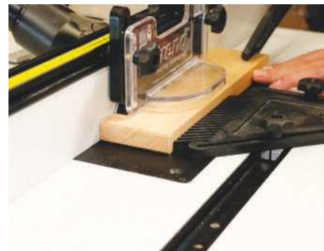
16 Set up the side featherboard and to ease the corners, run the pieces through on the long-grain edges
