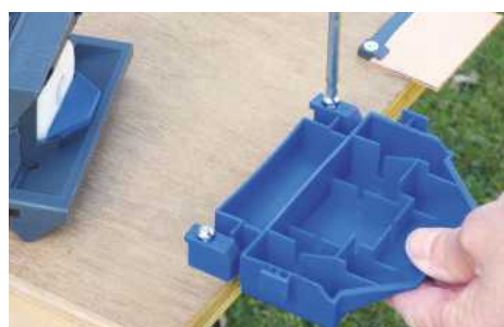
You first need to screw a plastic baseplate to the edge of a board or bench top
