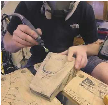
31 In tighter areas, such as the pocket in the top drawer, I used a Dremel with a carving burr
