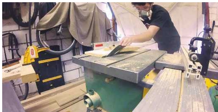
15 Cutting the shelf sides with a taper and chamfer along the front edge
