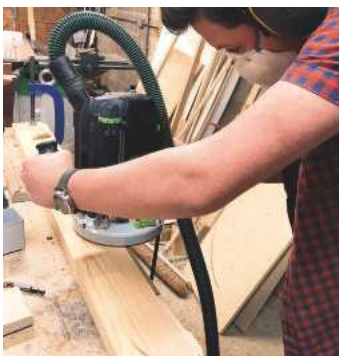
My keen apprentice Owen shaping the glazing beading with a router. Carefully positioned small screws hold the beading from beneath
