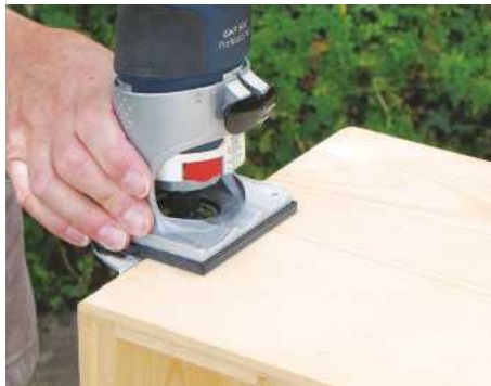
20 All outer edges are routed with a round-over bit to soften the cabinet
