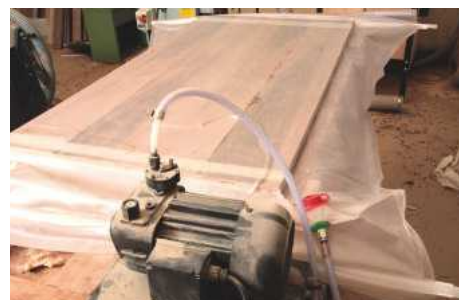
12 With veneer carefully laid in the glue the board is inserted into a vacuum bag press
