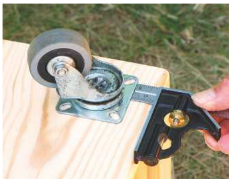
23 Mark castor positions and screw to the box. These will be replaced with larger wheels
