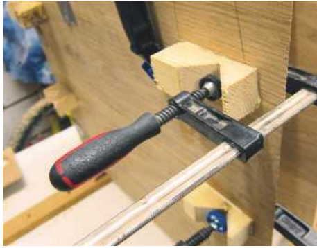
20 Sacrificial blocks were placed near the corners to allow the cabinet panels to be glued properly. These were later chiselled off
