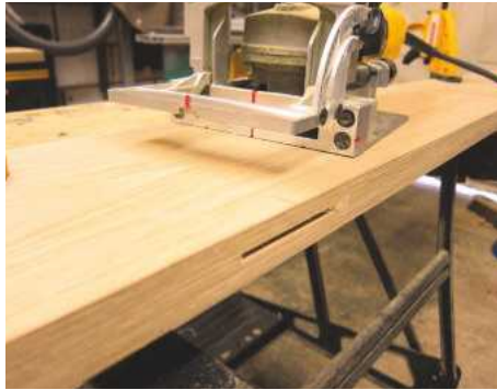
2 Biscuit joints were cut into the boards; these would make up the desk top
