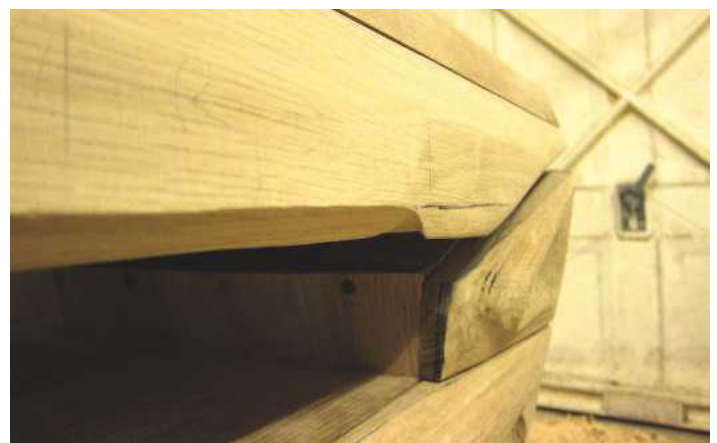
33-37 The photos here and above show the stages of progression for sculpting the drawer fronts
