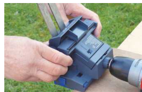
It's simply a case of moving the tool sideways along the rail for grinding
