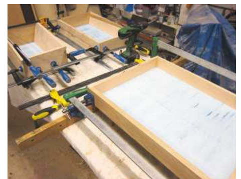
27 One of the drawers clamped up: here you can see a rebate on each side and the floating drawer bottom panel
