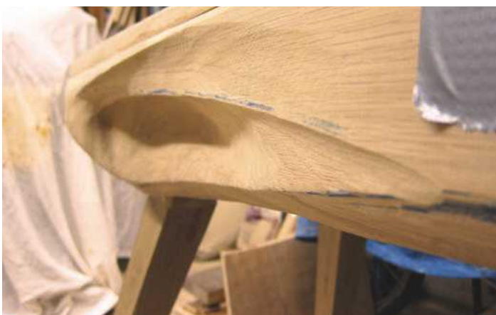
33-37 The photos here and above show the stages of progression for sculpting the drawer fronts
