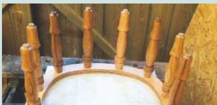
Tenons are placed into the pre-drilled holes and glued in place
