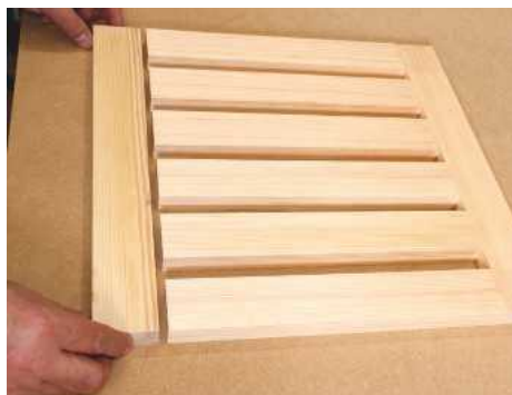
11 Using the rod to mark and make the cuts in this way will give a square top profile, which can easily be checked before assembly
