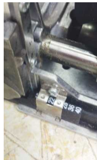
7 Setting the Domino position for the 22mm timber
