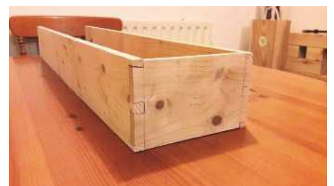
21 Loose joints due to sawing on the wrong side of the line
