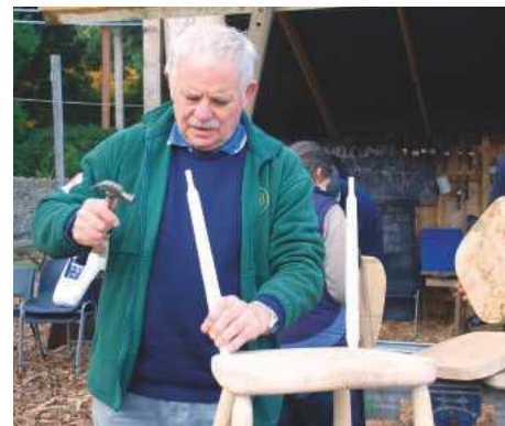
Hammering the two outer spindles snugly into the seat
