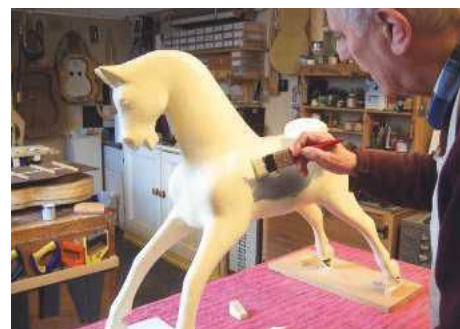
13 The cupboard paint is applied
