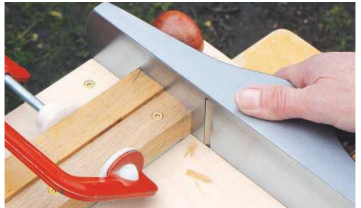
8 Before use, trim the end of the planing stop. Cramp a backing piece to this in order to prevent splching
