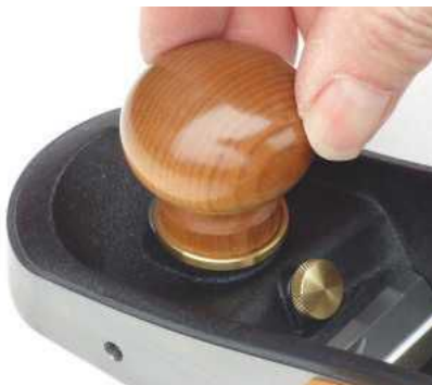
Veritas recommend that you set depth of cut first, then close up the mouth and tweak the stop
