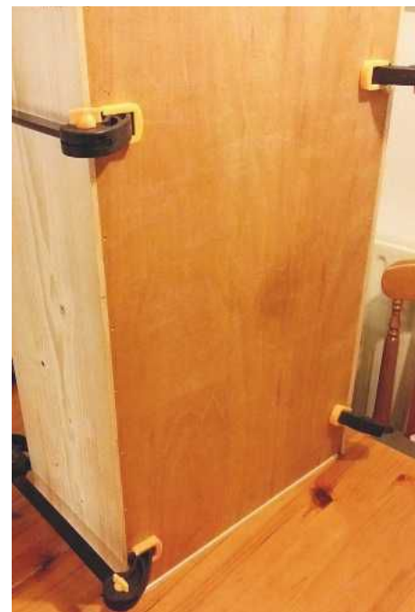
13 Here you can see the corner gap, which needed to be filled in, the plywood lip that needed to be planed down, and the pin holes, which were still to be filled
