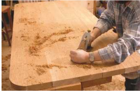
5 Planing diagonally across the grain flattens out any irregularities in the top
