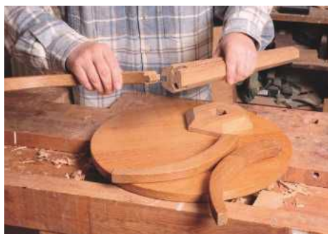
8 A round-topped tripod stand side table assembled from carefully jointed components
