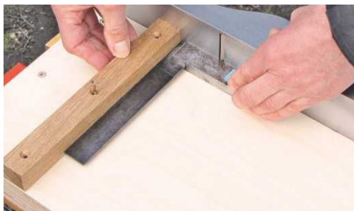
4 With the plane tight against the top, align the stop with a square. Glue and cramp before screwing
