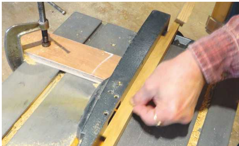
4 Scalloping. Again, several fine cuts are better than one hefty pass. I set up the ply stop so that I could always arrive at the same finish. Back in the right angle frame (shown in Pic.3 ) I glued the strips together and lightly cramped them
