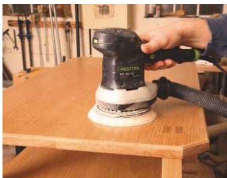
6 A random orbital sander smooths away any tracks or roughness left by planing
