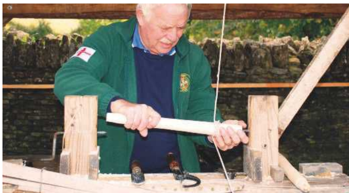
Once he'd got the hang of it, mounting a spindle on the pole-lathe and winding the string is easy enough for Paul
