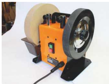
The leather stropping wheel to the fore; the support arm will fit in either orientation for maximum range
