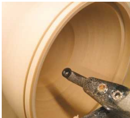
17 As I was working further into the piece, I found that the spindle gouge became less effective due to the overhang on the toolrest. The Simon Hope hollowing tool is stronger and easily copes with the extra depth
