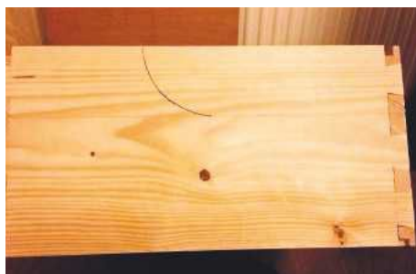
9 The curved lid edge is cut with a coping saw, matched on both sides, and the dovetails are spaced to allow the lid to be cut free
