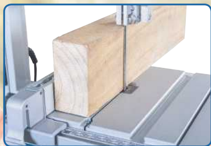
Allows sawing of large work pieces at a cutting height of up to 120 mm
