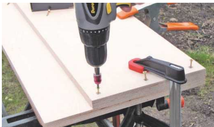
3 Drill and countersink the upper surface. Align both of the boards, then cramp and screw them together
