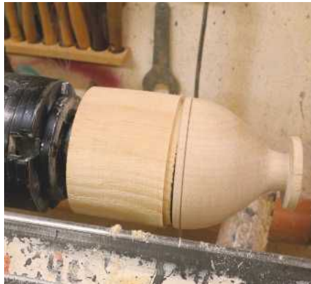
23 The neck section will need to be turned to shape and the best way to do this is to make a jam chuck out of pine to accept the recess on the base
