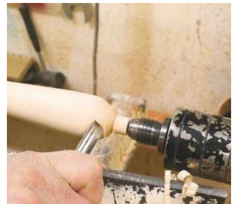
27 As always, leave enough waste at the tailstock end – here I have left a good 10mm. The skew creates a fantastic finish across the end-grain, which requires little or no sanding
