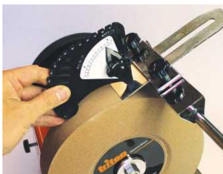
Checking the correct grinding angle
