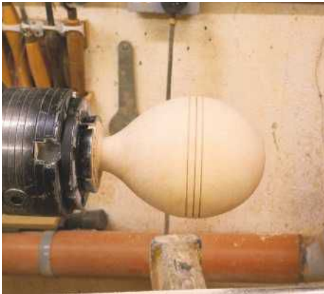
19 The best description I can find for the shape is a balloon. As it gets thinner near the chuck you may experience some vibration, so make sure you finish each section as you go along
