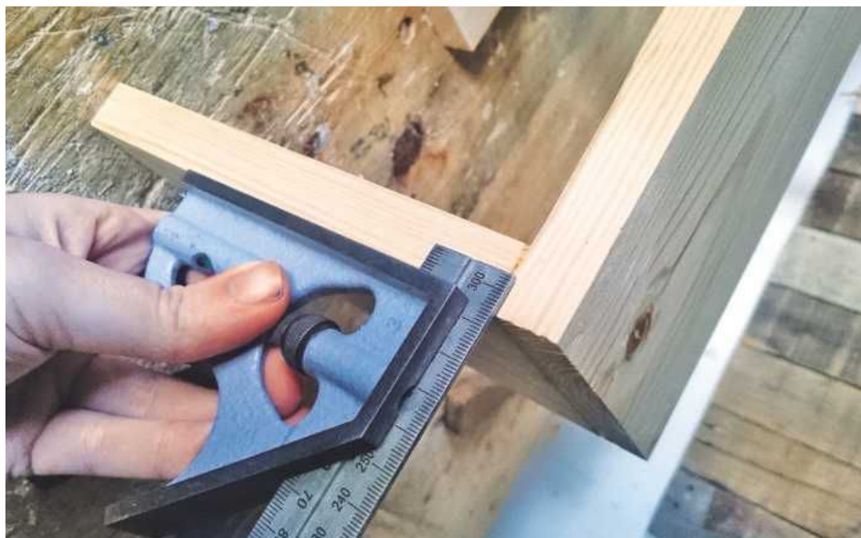
8 To correctly place the dowels, I measured half the width of the boards with a combination square
