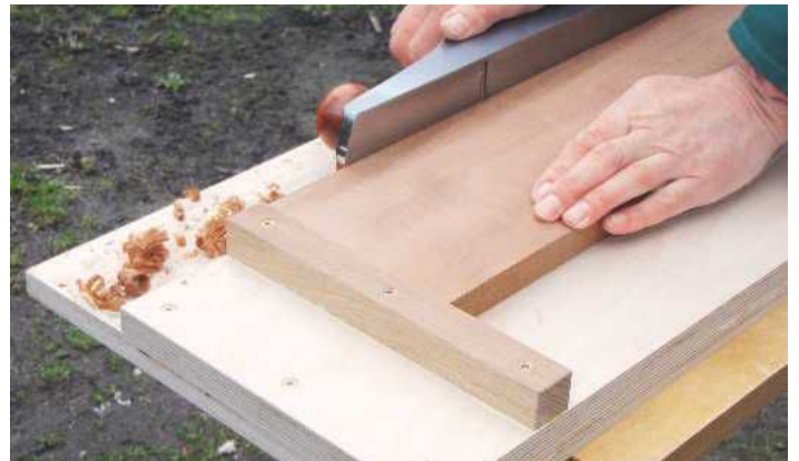
10 To shoot an edge just hold the board against the stop and move the plane
