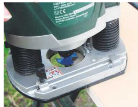
2 Rout a chamfer on the underside of the top board to give clearance for shavings and dust when planing
