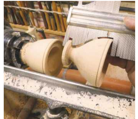
21 These profile gauges are absolutely essential when trying to match profiles. I find the metal ones suit the fine detail from turned shapes better than the plastic gauges
