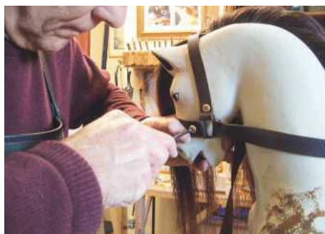
22 The bridle is screwed into place
