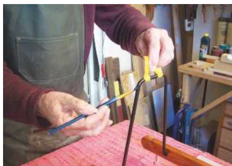
25 The swing irons are painted with satin black enamel paint
