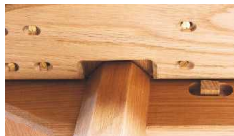
16 Looking up at the underside, the support frame of this table is loosely screwed to the top, allowing for seasonal wood movement
