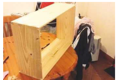
8 Here the dovetails have been trimmed flush
