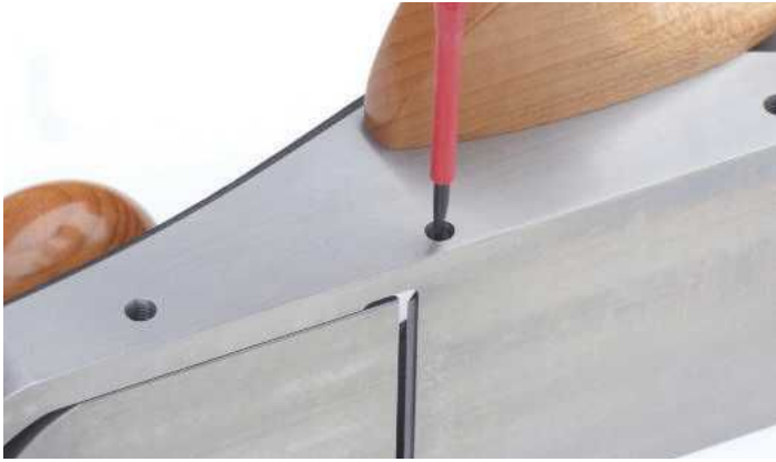
Screw guides are adjusted so there's no side play with the blade in position
