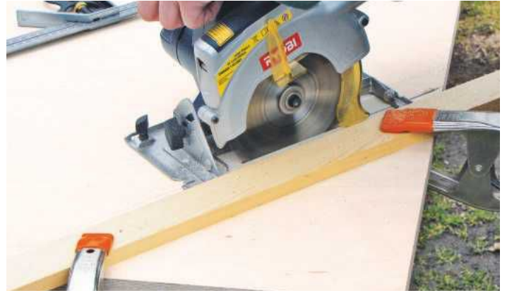
6 Cut a right-angled triangle to form the mitre shooting board. Plane up the sawn edge
