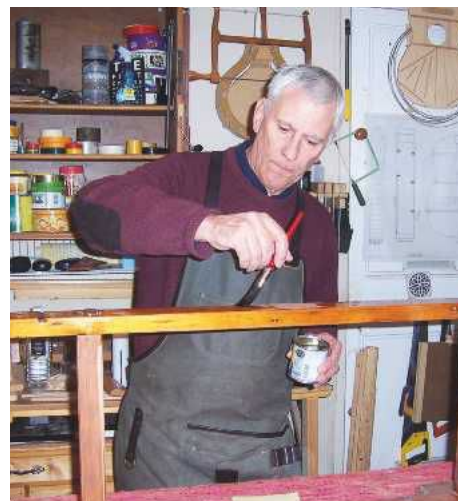
3 Polyurethane varnish provides a tough finish
