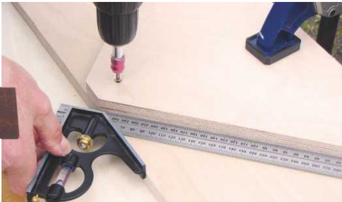
7 Ensure that the mitre board pivots slightly. Insert extra screws for accuracy, or cramp when shooting
