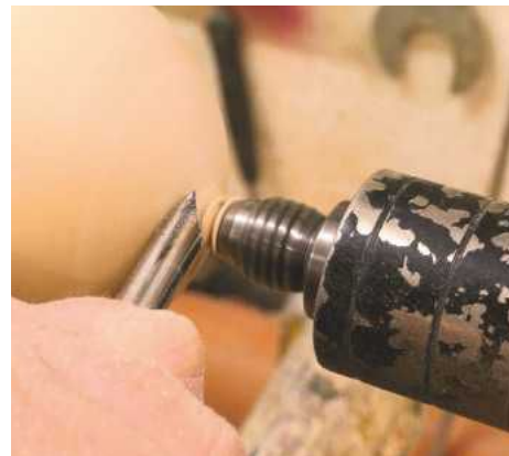
15 The curve on the top can now be turned by following the shape all the way down to the live centre. Make sure you allow for about 5mm of waste on the top, which will ensure you don't end up with a mark from the centre
