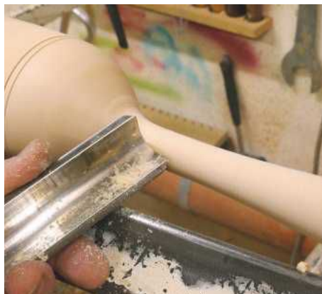
26 Sweeping cuts with the spindle roughing gouge are fine for these types of flowing shapes. I angle the tool slightly, which eliminates any chance of the tool running back on me
