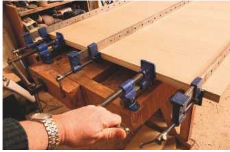
4 Sash clamps alternately above and below prevent buckling as they press the boards together while the glue sets
