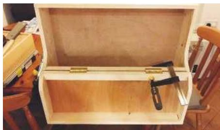
18 The hinges installed
