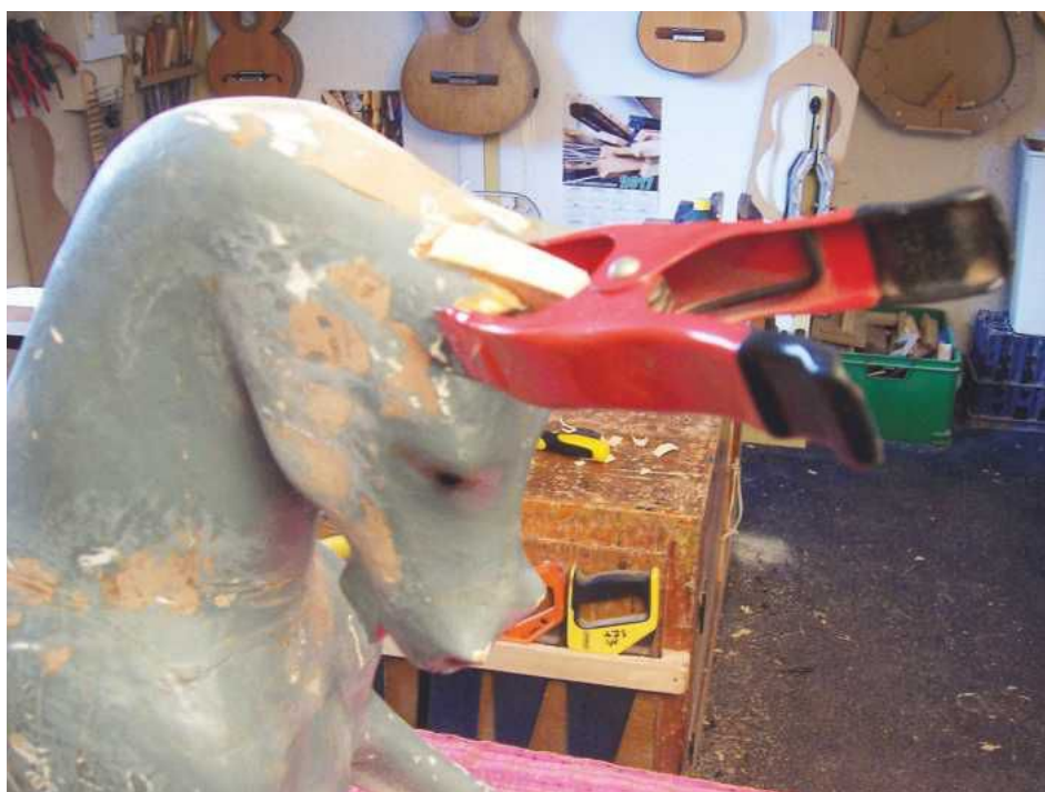
6 A small pine block is glued into place
