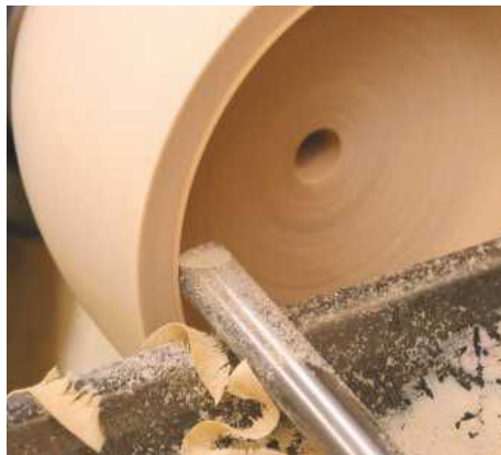
14 It's now time to fit the lid by making really small cuts using a 10mm skew chisel. It will need to be a tight fit as you are going to jam the top on; this will allow you to complete the shaping of the maracas
