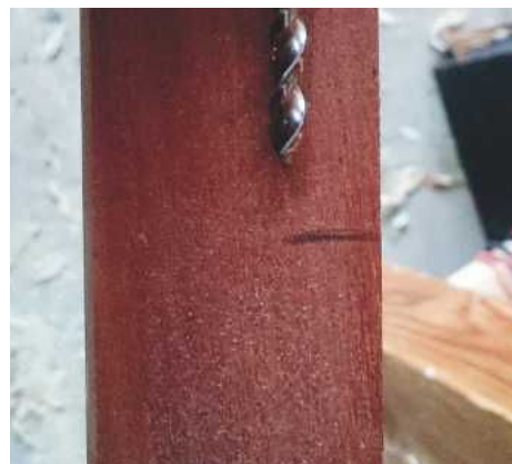
11 Holding the drill bit up to the sapele, I marked a little bit longer than the depth of the holes
