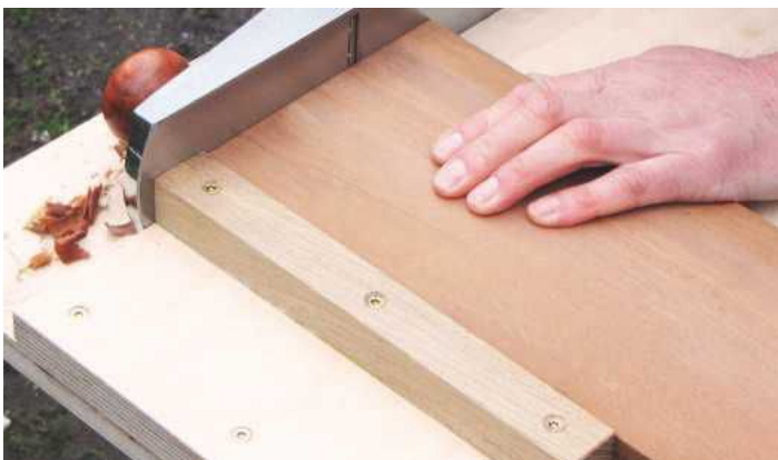
11 You should adjust the plane for a very fine cut when trimming end-grain square
