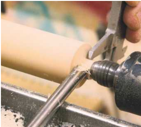
22 When you are happy that the bodies match each other, mount the stems between centres and make them round. An accurate 10mm diameter spigot about 10mm in length needs to be created on one end
