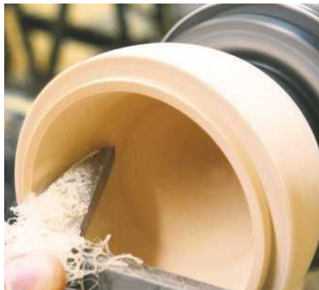
11 A negative-rake scraper is the tool of choice for cleaning up the inside. You're looking for a wall thickness of around 5mm maximum; if it's too thick, it won't make a decent sound
