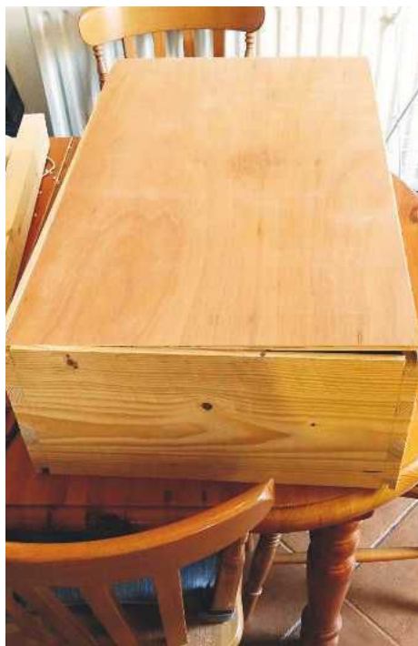
11 The plywood skin, roughly cut to size
