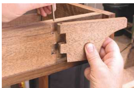
12 The extending flaps of a drop leaf table are supported on swing brackets pivoted on hinges cut in the wood
