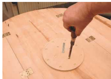
11 This folding round table top rotates on a central disc screwed to the underside
