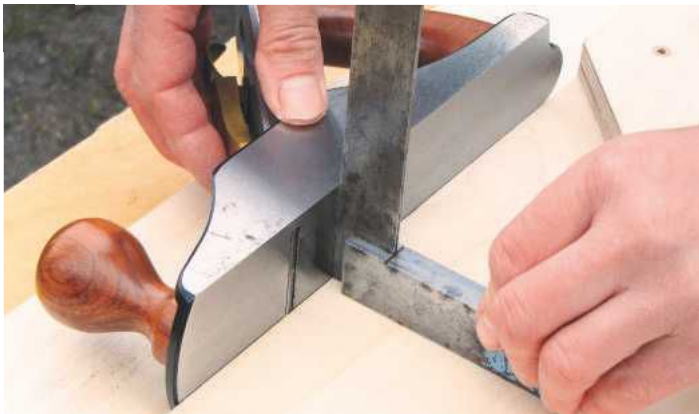
9 It's important that the sole of the plane is square to the top board. Check with a square
