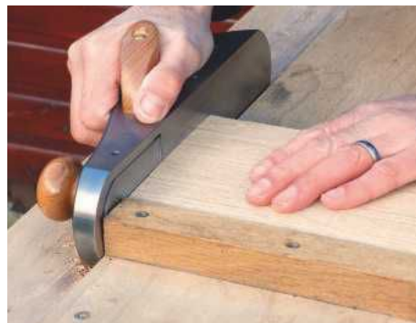
Used with a shooting board, it's far easier to use than a regular bench plane
