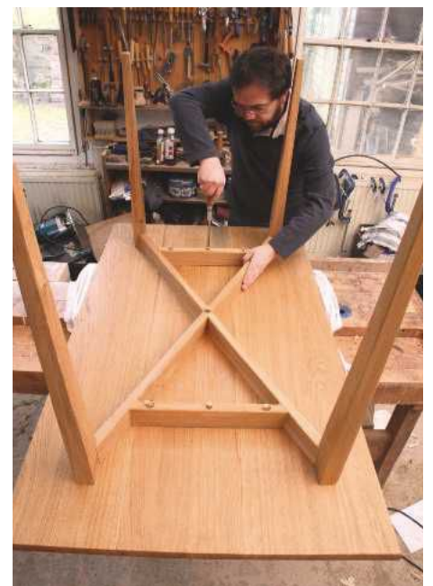
7 The simplest of straight leg support structures is braced by a hidden diagonal frame beneath the table top
