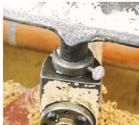
18 All my toolrests in the workshop have these locking collars on them; this means that I can move them from parallel to the lathe bed to right angles, without altering the height
