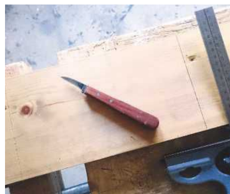
3 When working the pine, I decided to cut all the lines deeply with a knife
