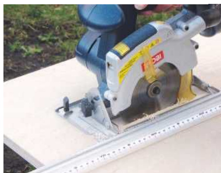
1 Start by sawing the ply to size using a guide rail. The top board is about 90mm narrower than the lower one
