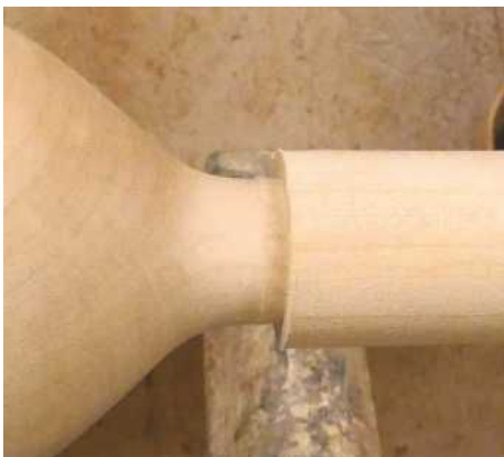
25 The surfaces where the handle meets the body need to be cut square or you can end up with a gap. For added security during the turning process, you can glue the handle in place at this stage
