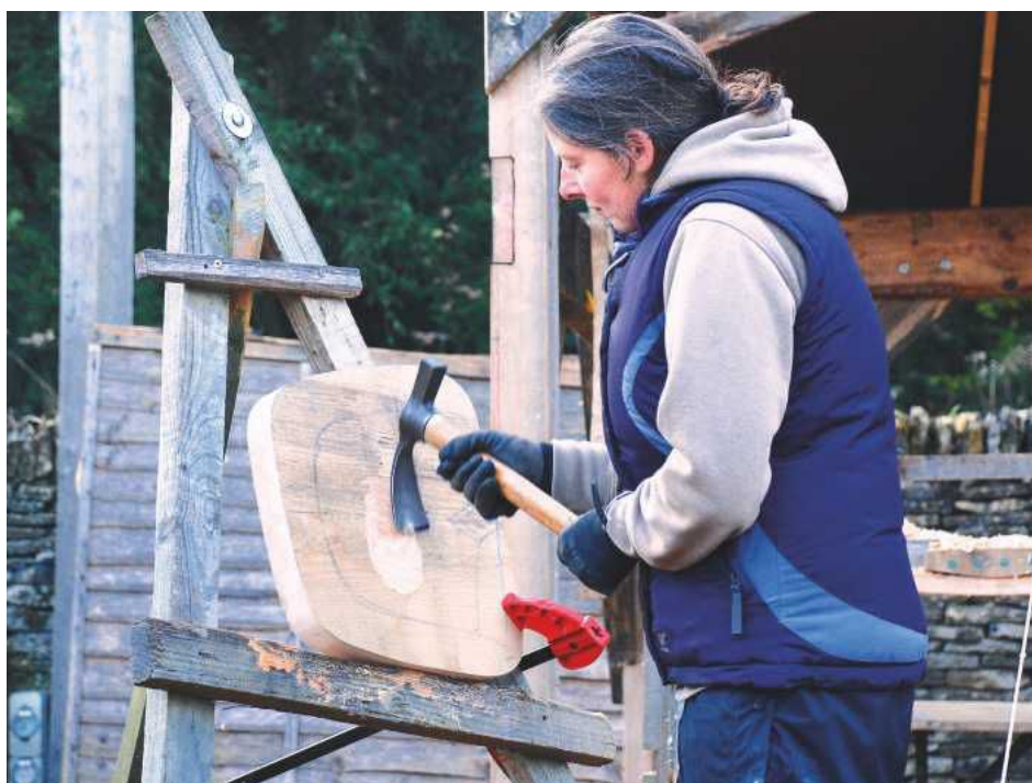
Using an adze to hollow out an ash seat blank. Many participants have never used woodworking tools before, let alone attempt specialist chairmaking techniques
