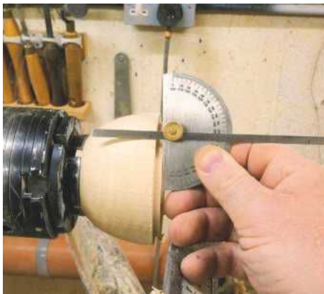
10 A simple depth gauge will show how you're progressing. I ended the hollowing just short of the chuck, which allowed me to clean up the end of the piece
