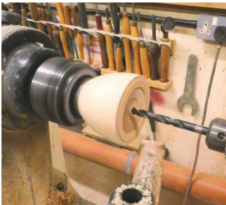
13 Next, mount the other half in the chuck. This piece will have a hole all the way through it, which you can make using a 10mm drill bit. Remove the drill frequently so it doesn't bind up with shavings
