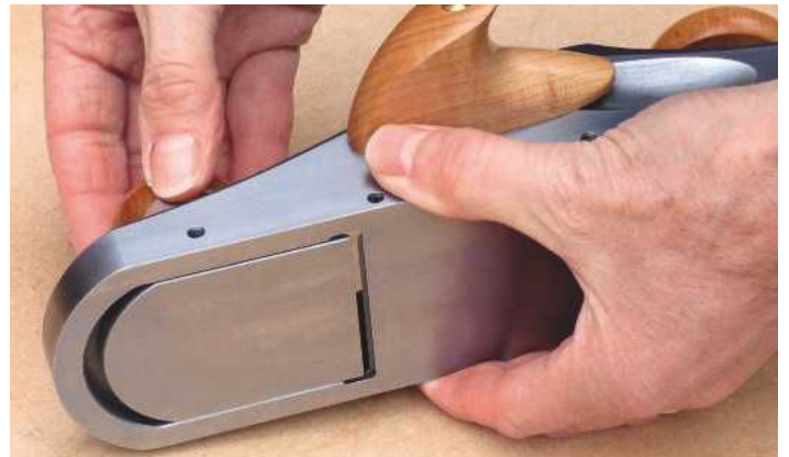
Slackening off the front knob enables you to slide the front shoe back, with up to 7mm of travel
