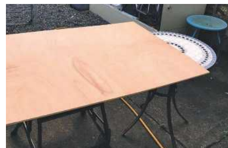
10 Half a sheet of plywood was used for skinning the frame
