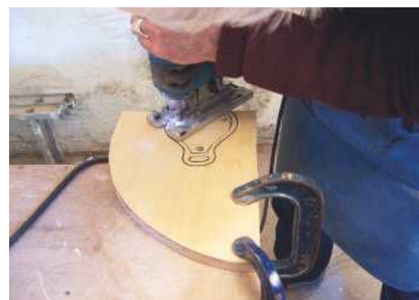
23 The inside shape of the stirrups is cut out with a jigsaw
