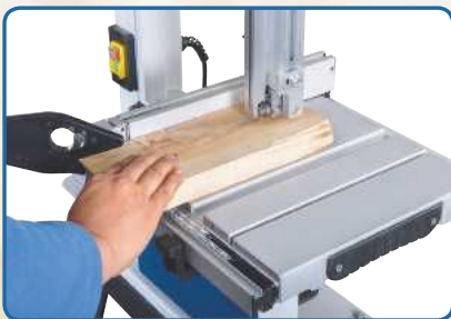
Rigid ripping fence allows for perfect straight cutting
