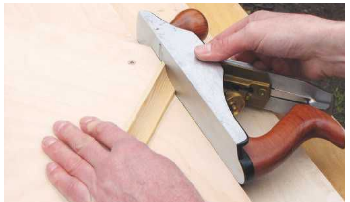
12 This is a multi-purpose jig, as trimming 45° mitres precisely is frequently necessary when making picture frames
