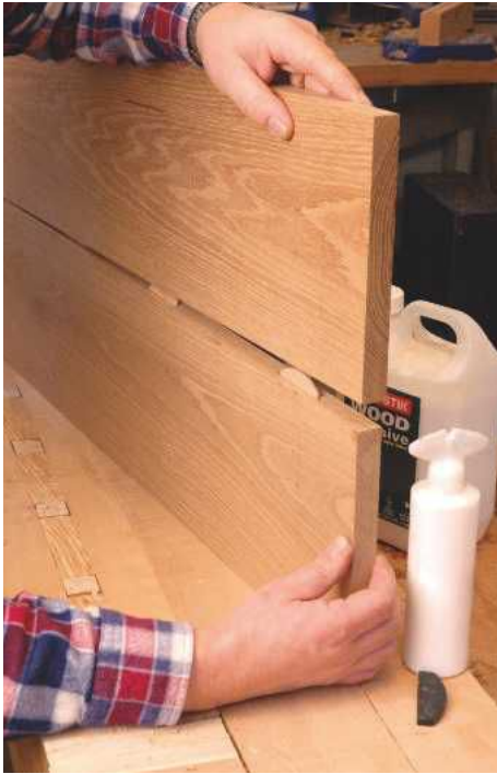
3 Wooden 'biscuits' are glued into each slot as the boards are brought together edgewise
