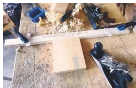
5 I set up a plank on my workbench to push against; this would allow me to work each piece down with a smoothing plane
