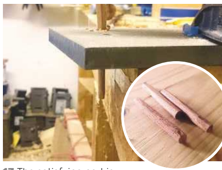
13 The satisfying part is tapping the dowels through the dowel plate
