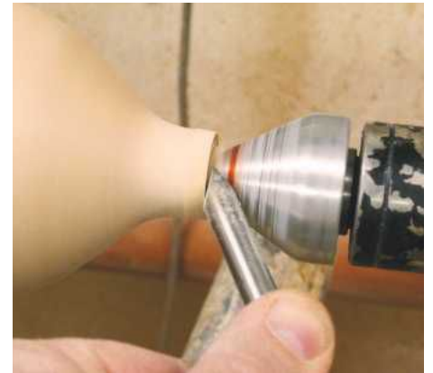
24 You will find that you will need tailstock support all the way through this part of the process. The aluminium cone on my live centre allows me to cut right up against it without damaging the edge of the tool
