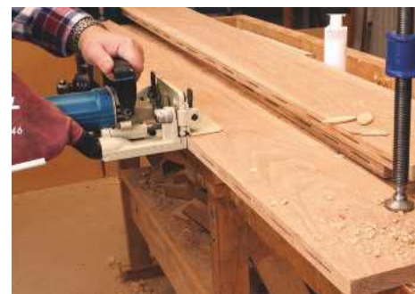
2 The biscuit jointer cutting a series of slots is a great tool to help edge joint boards
