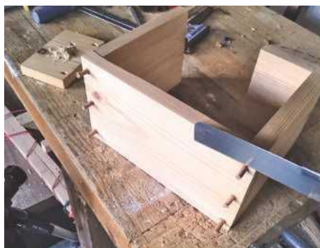
16 Using a flush cut saw to trim off the dowels
