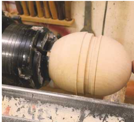
20 The other one is turned in the same way and here I am offering the first top up to the second one so I can get the sizes similar. It's a good exercise to try and get them both exactly the same
