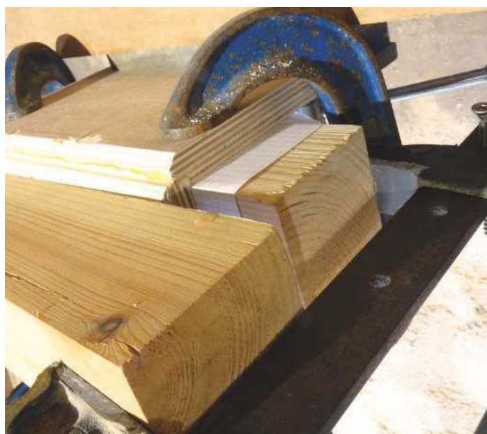
6 How to cut for a spline? I thought of a cradle to run over the table saw. It needs to be made accurately. Here I'm using polyurethane glue to bind the two wings of the jig at a definite 90°...
