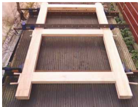
15 Use heavy-duty sash cramps when gluing up, making sure that the work surface is flat to avoid the gate twisting
