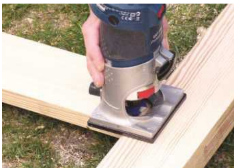
23 Rout a matching chamfer along the inner edges of the stiles and top rail. Both outer boards will also need chamfering
