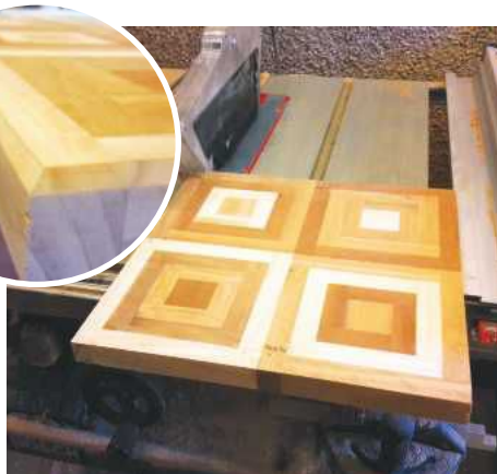
11 Skim the edges on a table saw to straighten
