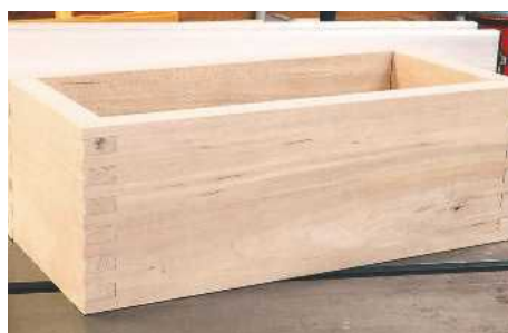
2 The box sides cut and test fitted, waiting for glue to be applied
