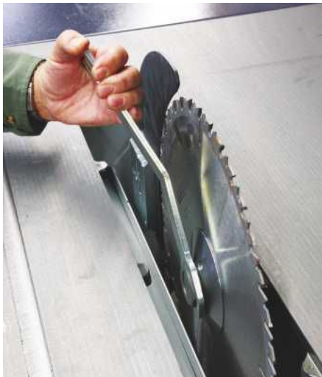
5 To change the blade, the rotating arbor is locked in place and the securing nut removed
