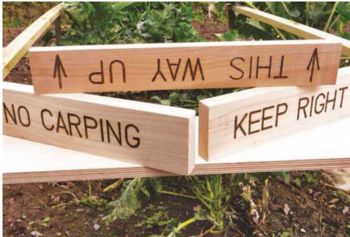
2 The larger the letters, the less noticeable their irregularities. Poplar and beech (top) worked well
