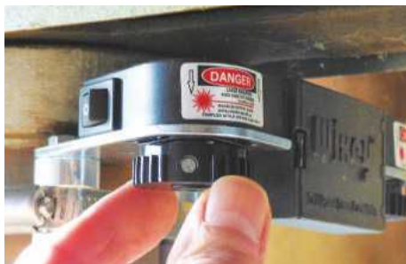
Twin plastic thumbwheels are used to adjust the laser lines vertically
