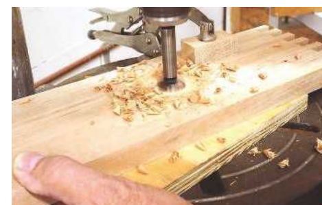
3 Cut the sound hole a bit smaller than the bouncing balls used on the drumsticks (32mm)
