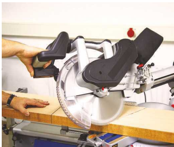
12 An alternative to a saw bench is a high performance cross-cut sliding arm cross-cut saw
