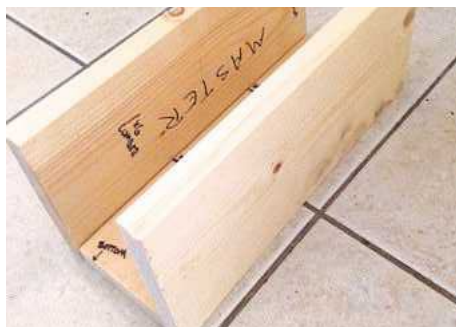
5 The first step is to nail the back wall and side pieces together
