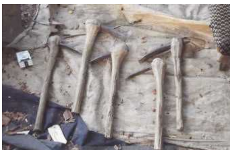
A comprehensive set of adzes made from vehicle springs with handles of neem wood
