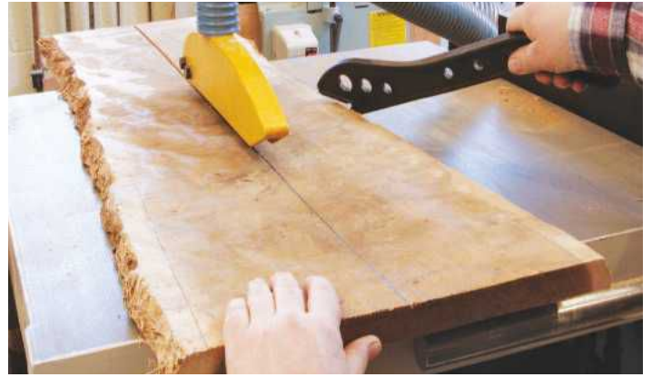
4 Here I am rip-sawing down the centreline of a board
