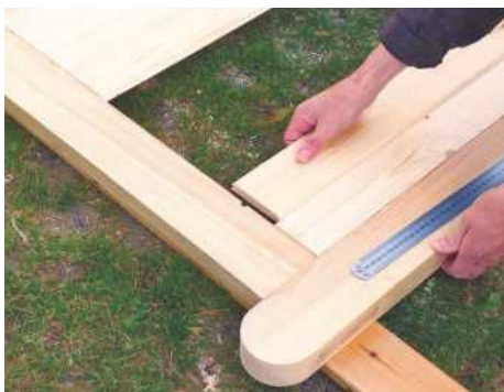
20 Rout rebates along the outside edges of both outer boards to match the grooves in the stiles. These should not be too tight
