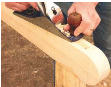
17 Trim the tenons flush with a bench plane. Check both stiles with a long straightedge and true up if necessary
