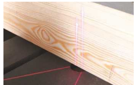
With the block stood on edge on the machine table, you then adjust each line via their respective thumbwheels until they're parallel to the pencil line
