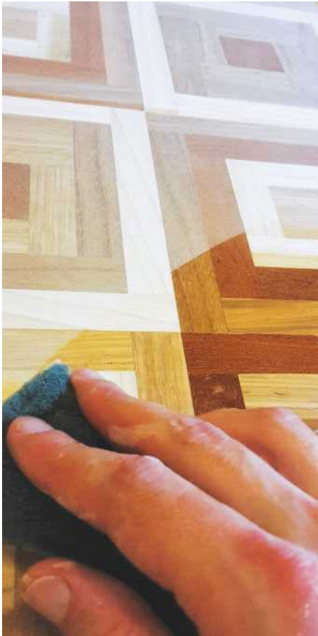
16 Wet the surface of the table to raise the grain between sandings
