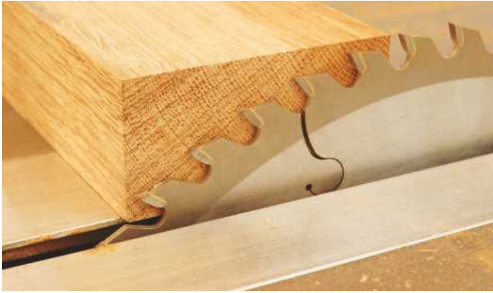
3 The blade height is adjusted slightly higher than the thickness of the wood, so the maximum number of teeth are in contact
