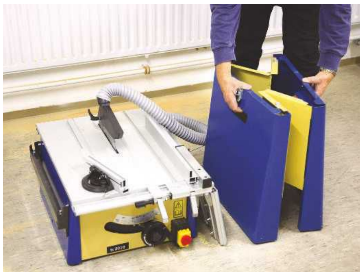
9 A folding stand allows this small cabinet saw to be carried in pieces by one person and taken in the boot of a car
