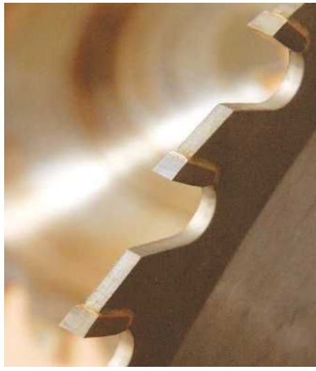
6 Most blades nowadays are tungsten carbide tipped and have expansion gaps, curiously shaped to reduce noise
