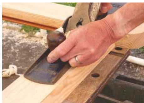
24 Making sure the gate is cramped securely, clean up both faces with a long bench plane, checking for true with a straightedge
