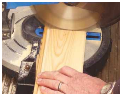
18 Saw the T&G matchboarding oversize. They will be cut again once the boards have been nailed to the gate
