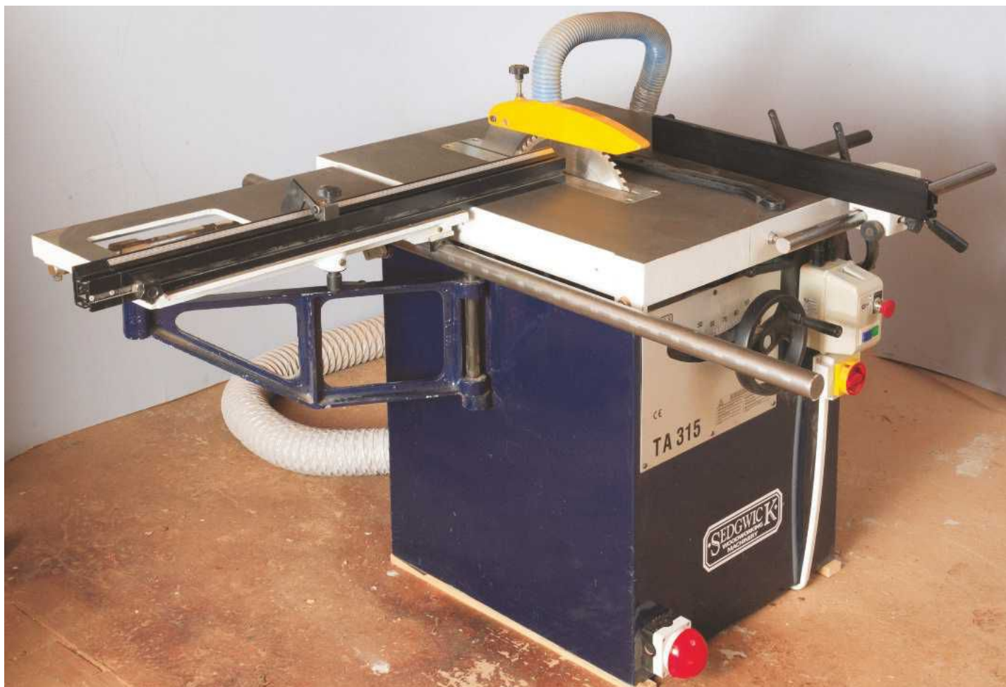
1 A medium-sized table saw with sliding cross-cut carriage on the left and ripping fence on the right. The yellow crown guard on top is fixed onto the riving knife behind the blade
