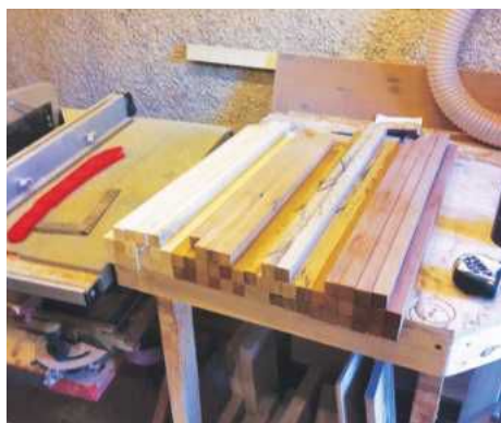
3 Cut them into rods around 25mm wide – 4.5m is needed
