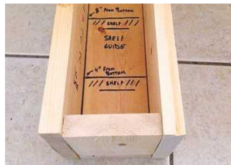
6 Nail the bottom shelf flush with the other pieces
