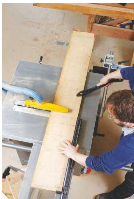
2 Seen from overhead, here I'm cross-cutting a board on the sliding carriage using a push-stick in my right hand
