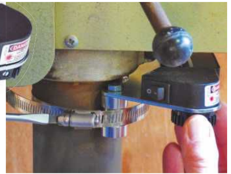
The Jubilee clip column is plenty long enough for the biggest of machines and simple enough to tighten in place with a screwdriver
