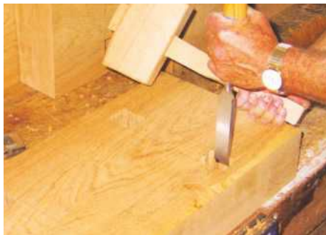
Hand cutting holes in oak with a mallet and mortise chisel
