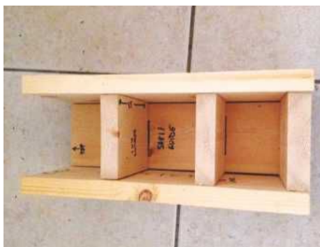
7 The shelves are then nailed in to place
