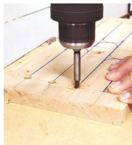
9 Drilling the holes through the top, where each tongue starts
