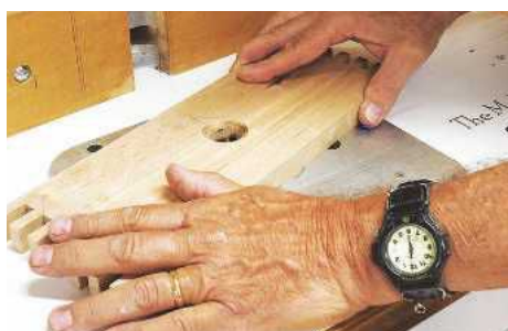
4 Rounding over the edges of the hole with a router
