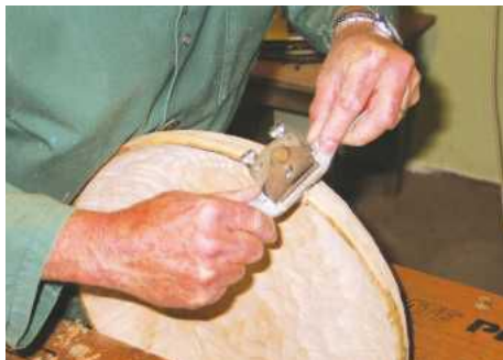
Finishing the edge of a 'rough-cut' chestnut bowl with a spokeshave
