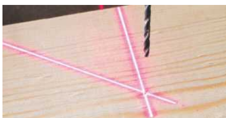
Lower the bit so that it makes an indent, which is dead centre
