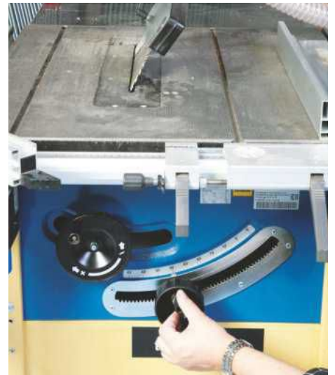
7 The whole rotating mechanism is mounted on a swivel bracket, allowing it to be tilted up to 45° for mitred cuts
