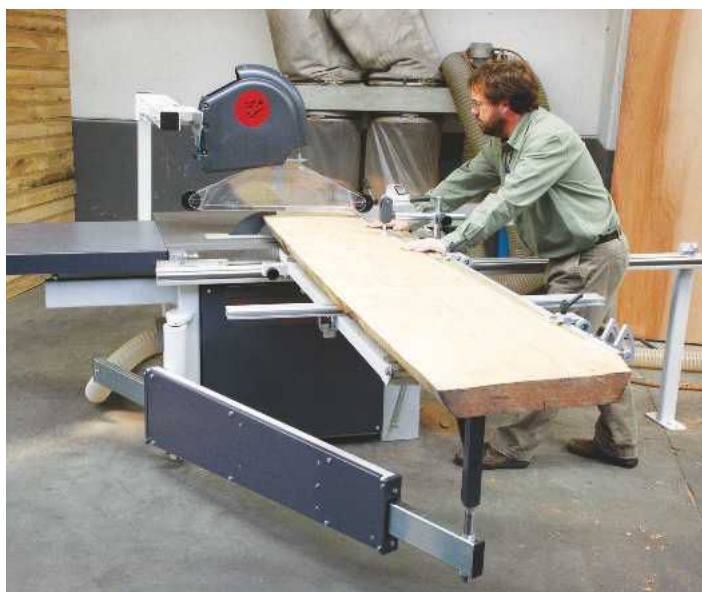
11 This seriously heavy-duty dimension saw is the size and weight of a small car while its swinging arm support helps me cross-cut a large piece of timber
