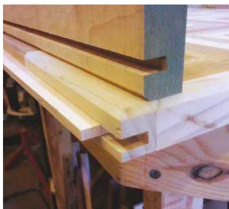
14 Add rails using splines
