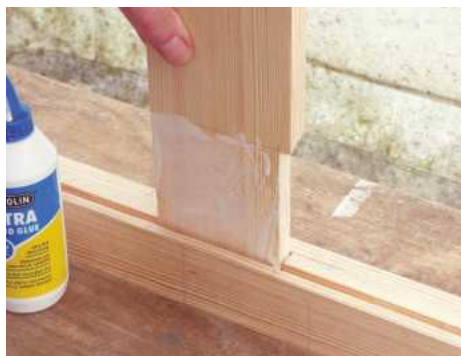
13 Assemble the gate dry to check everything fits correctly, then apply glue to joints with a suitable exterior adhesive
