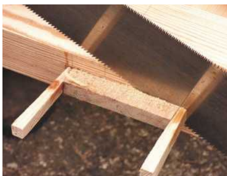
16 Once the glue has dried, saw the excess material from tenons and wedges, leaving the surface slightly proud
