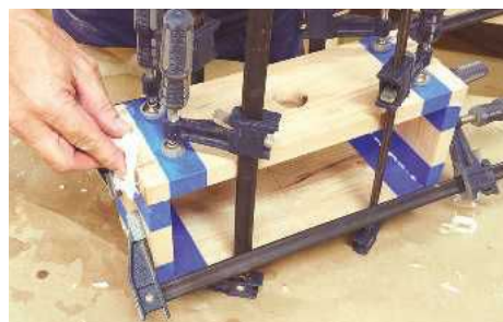
7 When you've finished adding all the clamps, the assembly should look like a porcupine
