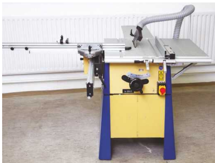
10 When the folding saw is assembled it is to all intents and purposes the same as a rigid machine for light duty work
