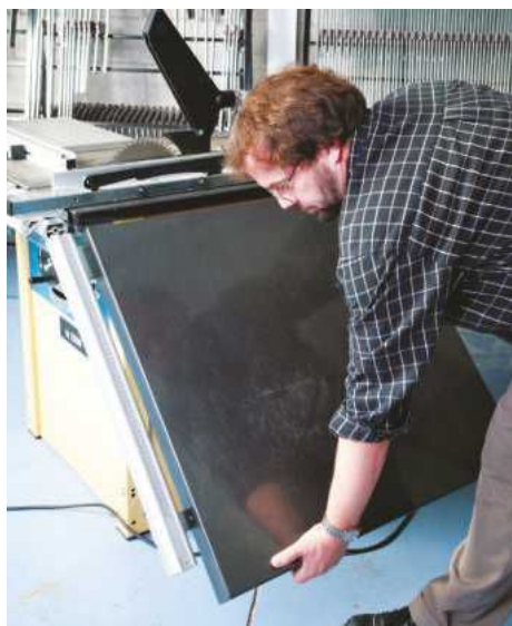
8 Small saws may come with table extensions either fitted or as optional extras to allow larger boards to be handled
