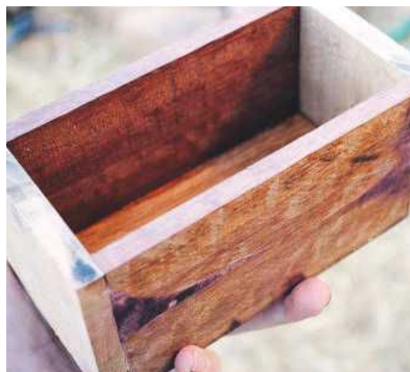
PIC 8. Glue panel D to the bottom of your box
