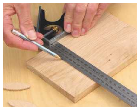
STEP 5. With the box components planed to size, mark out positions for No.10 biscuits
