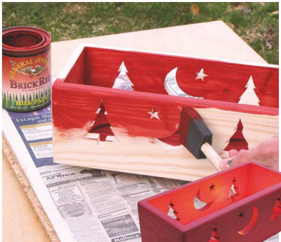
STEP 23. Either stain or paint the pine box. Milk paint doesn't need a primer coat first
