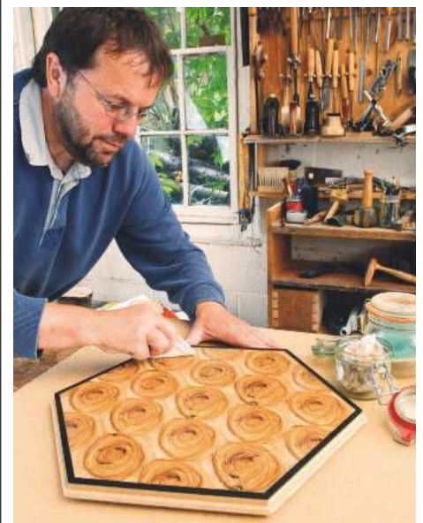
John Bullar demonstrating how traditional French polish, a natural shellac lacquer, can be worked into the surface in layers using a folded cloth and absorbent wadding known as a 'rubber'
