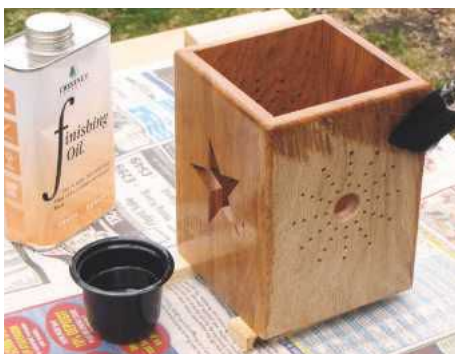
STEP 22. Brush on two coats of oil, denibbing between them. Sand and finish with wax
