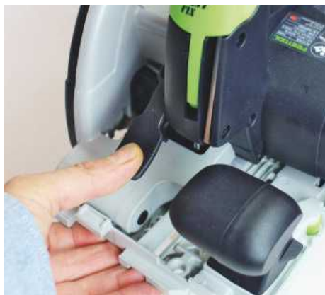
This lever controls the blade guard and will flip it back with ease
