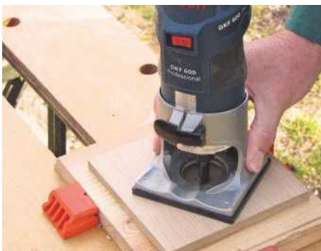
STEP 18. Mark the centre of the base and use a router or large Forstner bit to cut a recess
