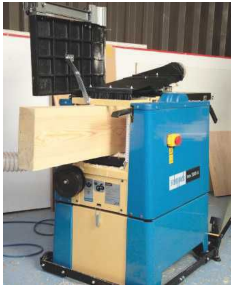
PIC 7. This compact machine is thickening large section timber with one planer table flipped up
