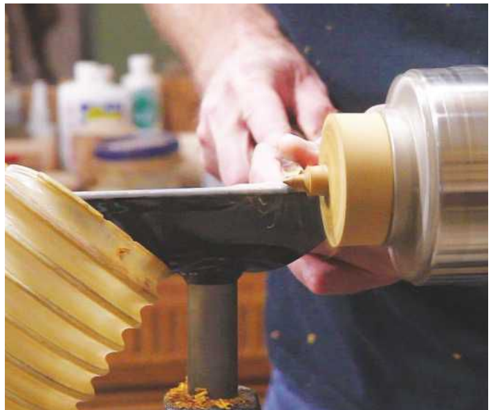
PIC 16. Turning the noses from scrap hardwood using a skew chisel
