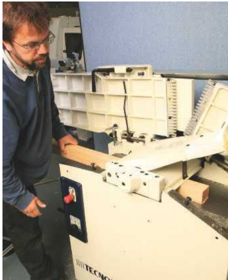
PIC 6. This larger machine has both planer tables flipped up, allowing you to see more of the wood being thickened
