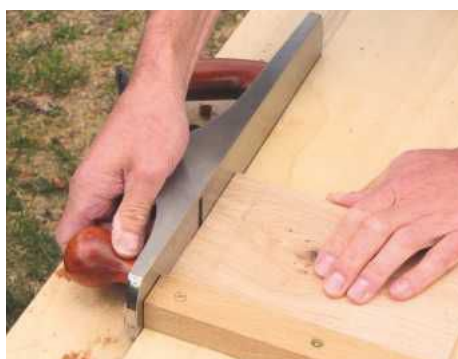
STEP 4. Trim the ends square using a shooting board and bench plane for accuracy
