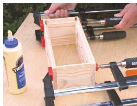
STEP 14. Assemble the box, checking everything is square as you tighten up the cramps
