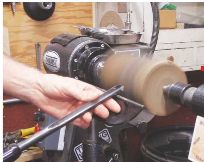
PIC 3. Using the bowl gouge with the lathe speed set low, begin to form the basic features
