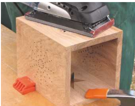
STEP 21. Sand with 120 grit abrasive, finishing with 240 grit. Moisten the oak and re-sand
