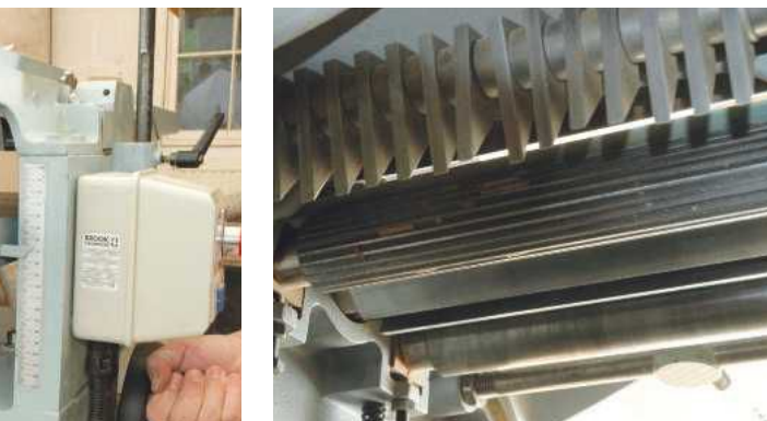
PIC 5. Timber is passed from left to right beneath anti-kickback fingers, grabbed by the serrated infeed roller, passed under the cutterblock, then out beneath the smooth outfeed roller
