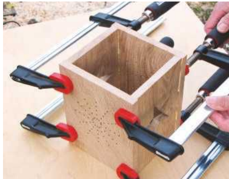
STEP 16. Glue up the oak box in a similar way to the pine version. Wipe off excess glue
