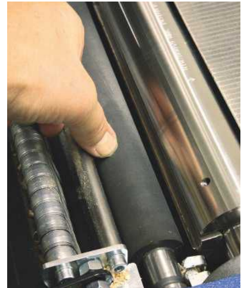
PIC 8. The compact machine has a rubber infeed roller rather than a serrated one before the cutter
