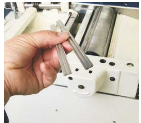
PIC 11. Laminated Tersa knives can be slid into the cutterblock on this machine without adjustment
