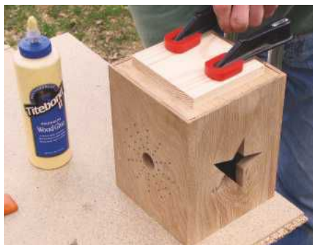
STEP 19. Cut the base to size and glue it into the rebate around the bottom
