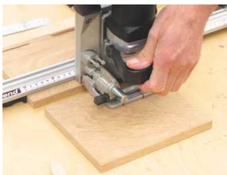
STEP 6. Cut slots for biscuits. If using wood less than 10mm-thick, rout rebates instead
