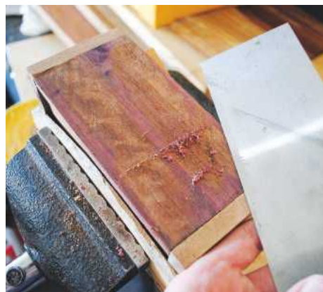
PIC 9. Use a scraper and/or hand plane to clean up the outside
