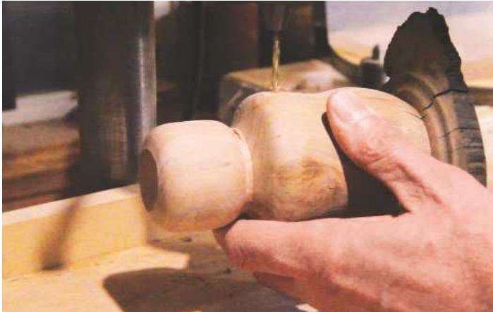
PIC 18. Drilling holes to accept the arms...
