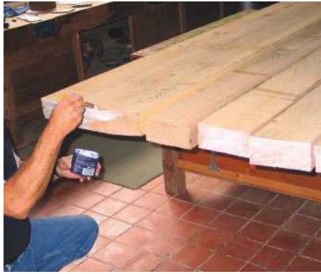
Sealing end-grain with glue
