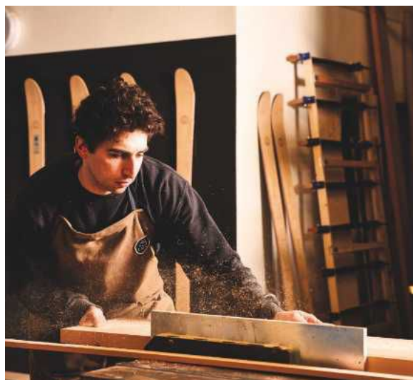
Ripping the beech to make the laminated cores
