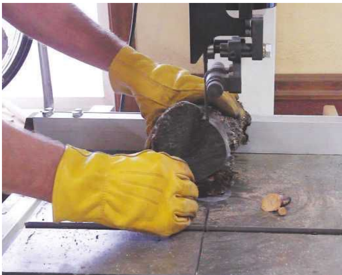
PIC 2. Cutting out the shape requires using the bandsaw
