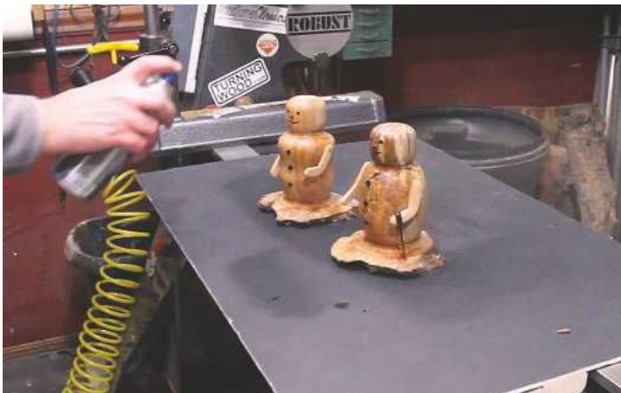
PIC 22. Finishing the pair with several light coats of spray lacquer
