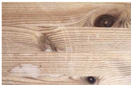
PIC 3. Claw marks, water-damage, and a tired wax finish make for a fair test of steam's ability to revive damaged timber
