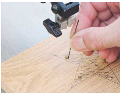
STEP 9. Slacken off the scroll saw blade, feed an end through the workpiece and re-tension
