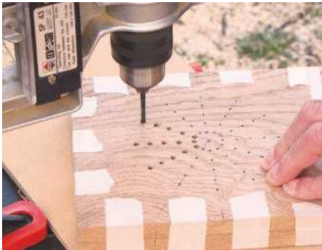
STEP 15. Mark the starburst design and tape opposite sides together. Drill with scrap beneath
