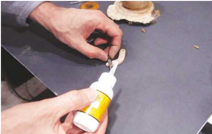
PIC 20. Applying glue to the holes drilled in the arms
