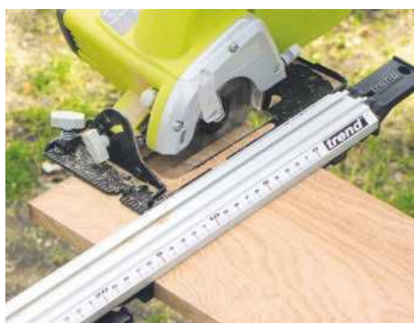
STEP 3. Plane the timber to width and thickness, then saw the box components to length
