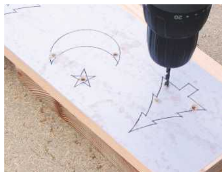
STEP 8. Apply with spraymount and drill a series of holes to enable you to start the internal cuts
