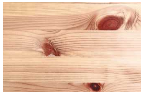
PIC 5. Even allowing for variations in lighting on different days, the steaming and a light sanding has worked wonders in erasing damage from the re-polished lid
