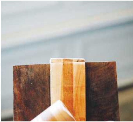
PIC 25. Aligning the edges of the bow to ensure they correctly continue down the side of the box
