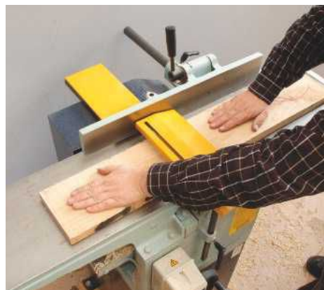
PIC 3. Timber is fed slowly from right to left, over the planer tables and cutter beneath the yellow guard
