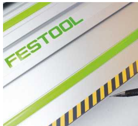
The guide rail, showing the plastic edge strip – a darker colour would have shown up better
