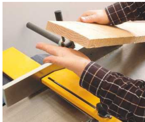
PIC 2. Dried timber often has a hollow or cupped surface, which must be placed downwards on the planer so it will not rock
