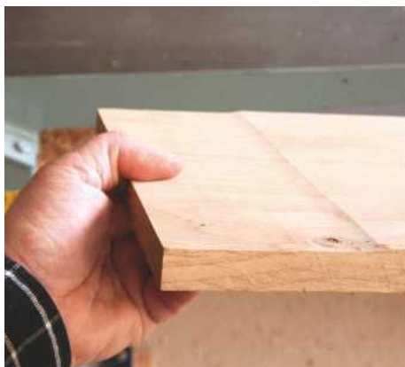
PIC 9. End snipe is a common problem when using a thicknesser. Snipe results from the board drooping as it leaves the machine
