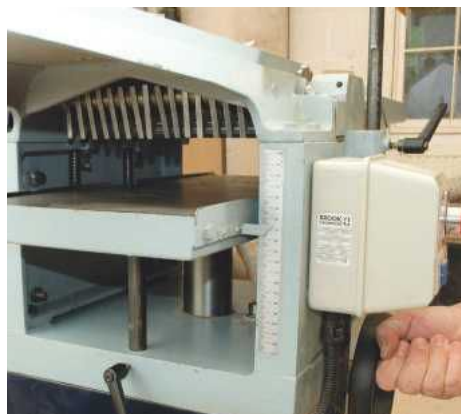
PIC 4. The thicknessing table can be raised or lowered in height with a handwheel
