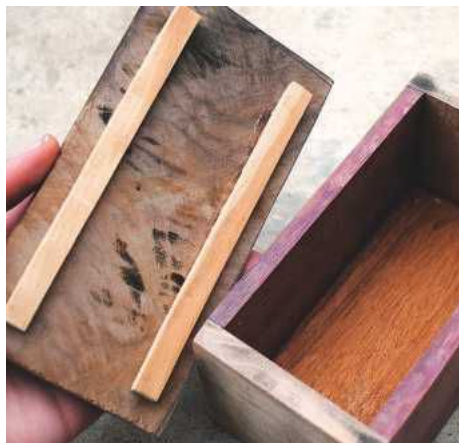
PIC 20. Make sure the lid fits snugly into the box before the glue fully sets
