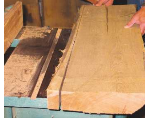
Straightening a wane-edged board
