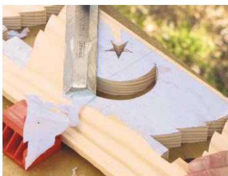
STEP 12. Use a chisel or cabinet scraper to remove the paper pattern after sawing
