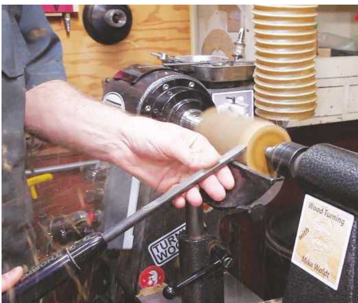
PIC 6. Forming the basic shape using a spindle gouge
