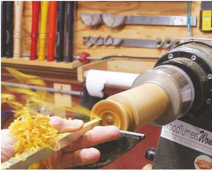
PIC 8. Turning a recess inside the hat to accept the tenon on top of the head
