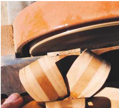
PIC 27. Sanding the strip to bring it down to the required size
