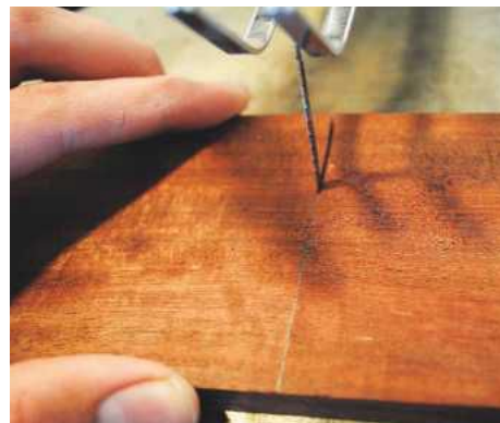
PIC 3. Cutting the wood using the scrollsaw
