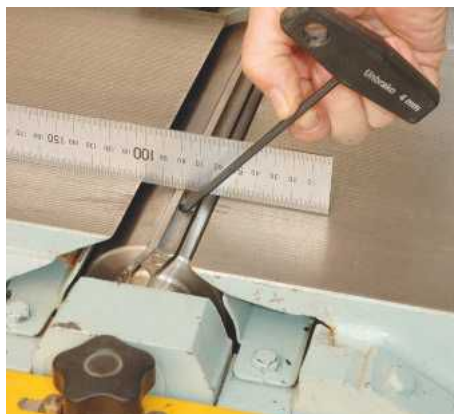
PIC 10. Conventional flat, wide blades – 'knives' – are fitted in a cylindrical cutterblock where they can be adjusted in height or removed for sharpening
