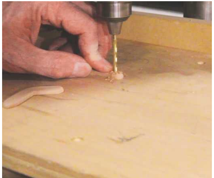
PIC 14. Drilling the holes for the mounting pins
