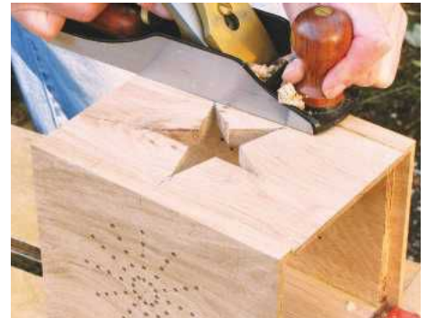
STEP 17. When the glue has dried, trim protruding edges flush with a finely set bench plane
