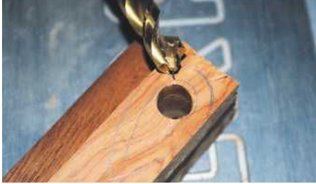
PIC 12. Drilling the ribbon hole
