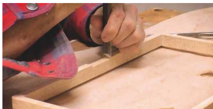
PIC 43. Using a chisel to square up the corners
