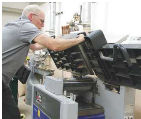
Lifting and lowering a pair of huge tables is surprisingly easy when big, powerful springs are helping
