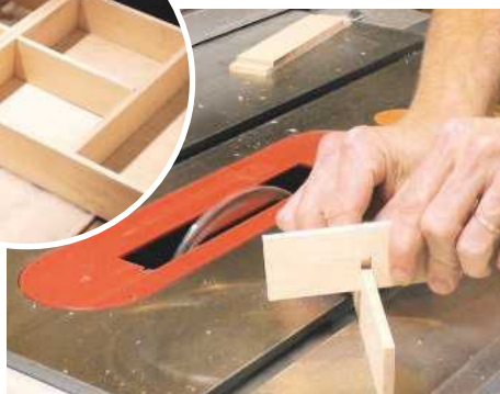
PIC 38. Assembling the cross-pieces once cut
