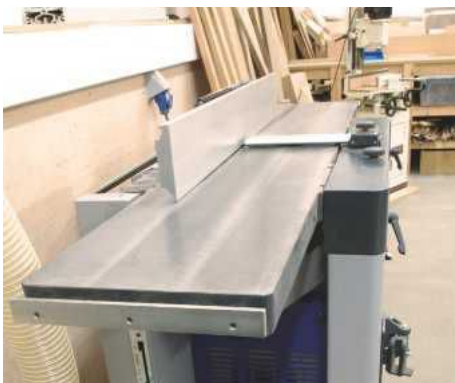
The long, wide tables on the AD 941 give excellent, accurate results on long, wide pieces of timber
