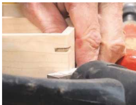
PIC 40. Inserting the walnut splines into the slots using wood glue
