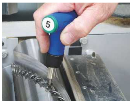
The spiral cutterblock is a real game changer. Changing the blades is a bit of a fiddle but accuracy is guaranteed and the quality of the cut is exceptional
