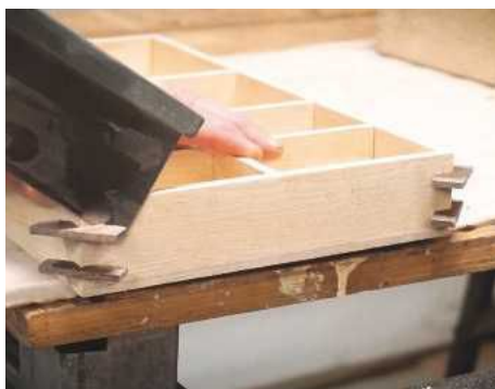
PIC 41. Trimming the splines using a flush cut saw
