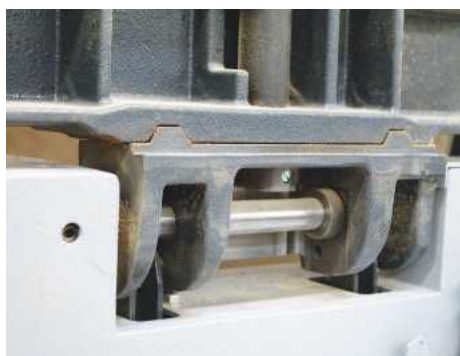
Meaty hinges and Felder's 'prism' table adjusting system all help maintain planer accuracy
