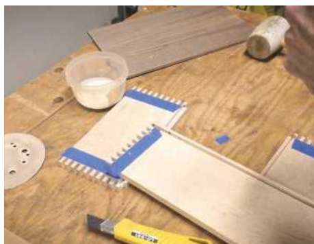
PIC 17. Applying tape to prevent any squeeze-out from sticking to the wood
