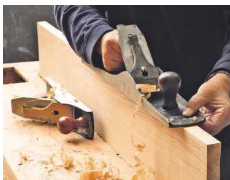
PIC 12. The longest plane you have is best for levelling and straightening edges
