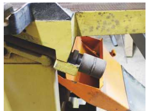
PIC 6. On my machine this knurled winder adjusts the height of the outfeed table
