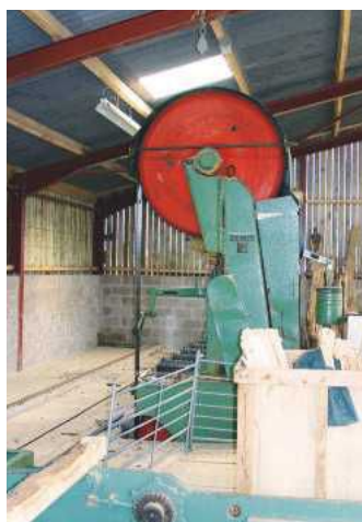
LEFT: The Stenner 60 bandmill has a 229mm x 10m blade. When in use it has 10 tons of tension and the motor requires 150Kva to start the saw blade – certainly an impressive machine!
