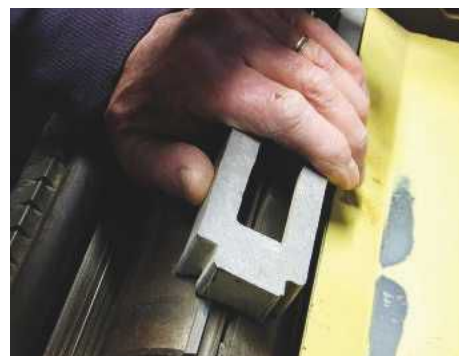
PIC 3. Using the setting jig, each new, sharp cutter is fixed in place
