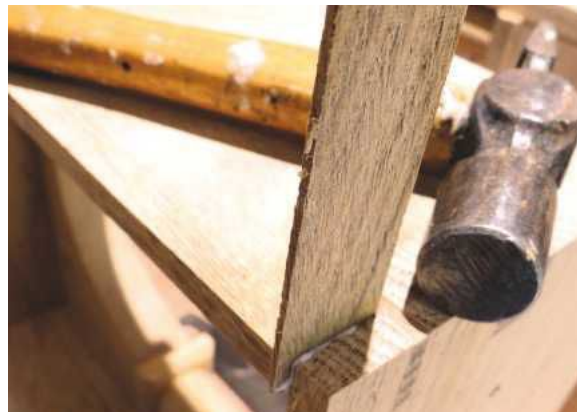
PIC 11. So too with the inaccurate joint. Saw the waste off proud; allow the glue to set, then sand the infill flush. I would never use filler here. Filler has a bland eye-catching colour, and, whatever it says on the label, it tends to sink
