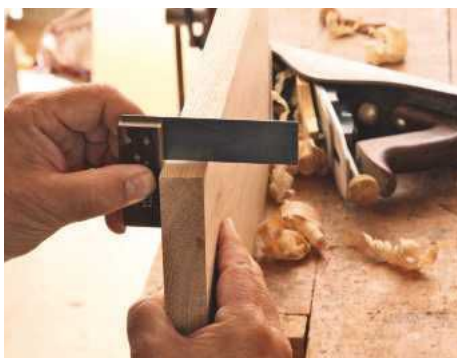
PIC 11. Using the face as a reference surface, I hold a try-square against it to check if the edge needs adjusting to a right angle
