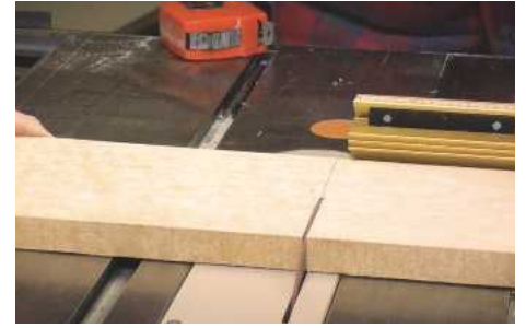
PIC 3. Cutting the maple sides
