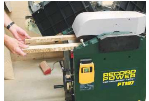
The thicknesser produces a really good finish and will happily handle more than one workpiece
