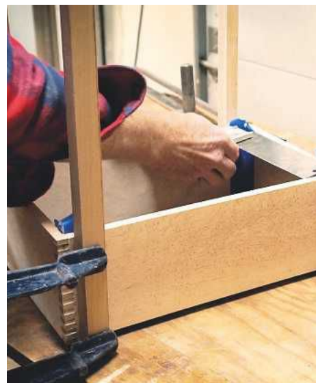
PIC 19. Clamping up the box and checking for square
