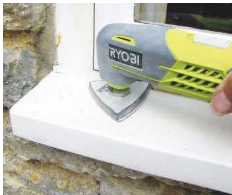
A detail sander, such as this Ryobi version, handles awkward areas with precision
