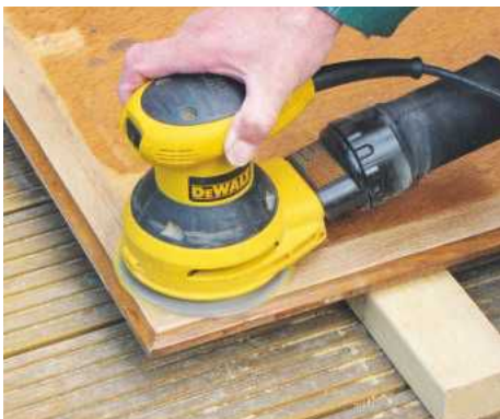
A random orbit sander should be your tool of choice for flat areas
