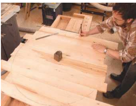
PIC 14. I lay the planed boards edge-to-edge so as to match them up, then I use a string and pencil to roughly mark out the circular tabletop edge
