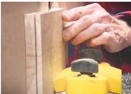
PIC 6. Re-sawing the box sides
