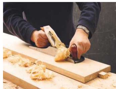
PIC 10. After sawing slightly over-size, the boards' best face is flattened using a medium length broad plane
