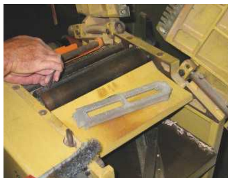
PIC 2. Take the old ones out and clean up all the wedges, springs and housings
