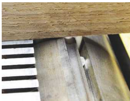
PIC 5. With a wooden straightedge, off the outfeed table, the cutter height is checked
