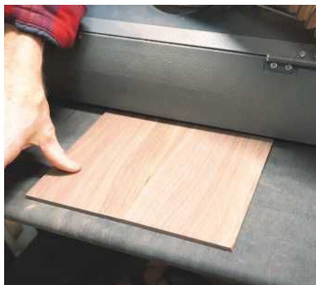
PIC 11. Passing the bottom through the drum sander to remove any excess glue
