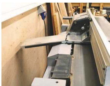
The cutter guard behind the fence is a flimsy collection of bent metal and nuts and bolts – very disappointing on a machine of this quality
