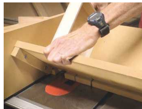
PIC 39. Cutting splines into the corners of the trays
