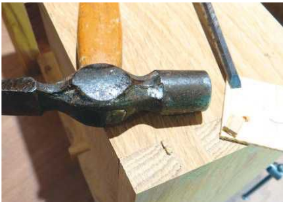
PIC 10. One remedy. A fiddly but simple matter of cutting infill pieces, chiselling a slight taper, smearing with glue and tapping home. It is worth getting the grain to match as well as you can. If the match is perfect, the mend will be invisible
