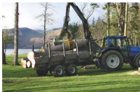
LEFT: This tractor with Botex forestry trailer is capable of lifting 2.5 tons
