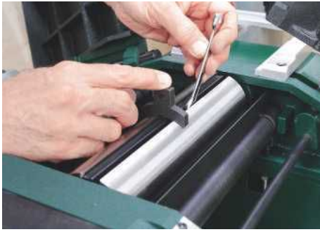
Accurately setting the PT107's blades with the single 'Cutter Block Gauge' can be a bit of a challenge
