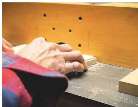
PIC 16. Routing a 6mm dado to fit the bottom panel
