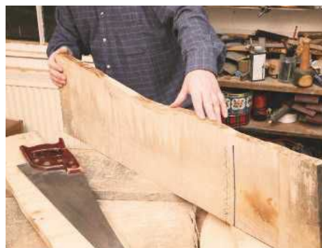
PIC 8. A waney edge on each board can be ripped off with a handsaw or on the bandsaw or saw table
