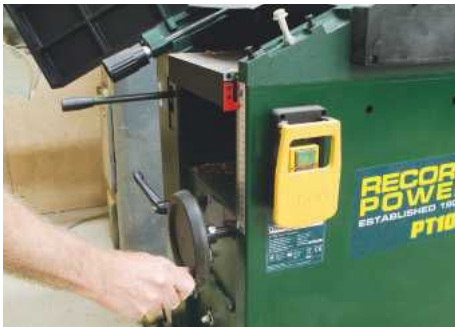
Thicknesser adjustment is achieved using a standard winder handle. Half a turn = 1mm
