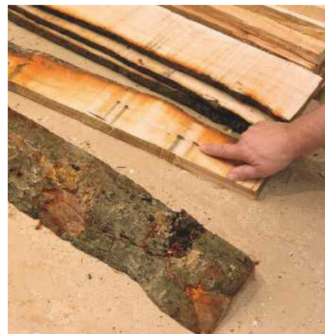
PIC 5. Nails hidden in wood were not visible through the bark but blunted the bandsaw teeth
