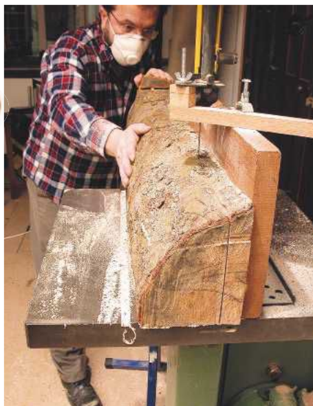
PIC 4. On the bandsaw table I ripped the half trunk into quarters before 'quartersawing' boards from alternate sides
