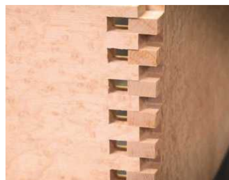
PIC 15. Box joint test fit revealed – nice and tight, which is what we're looking for
