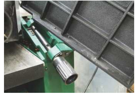
Nice sturdy hinges and a simple, effective adjuster for the chunky cast-iron planer tables
