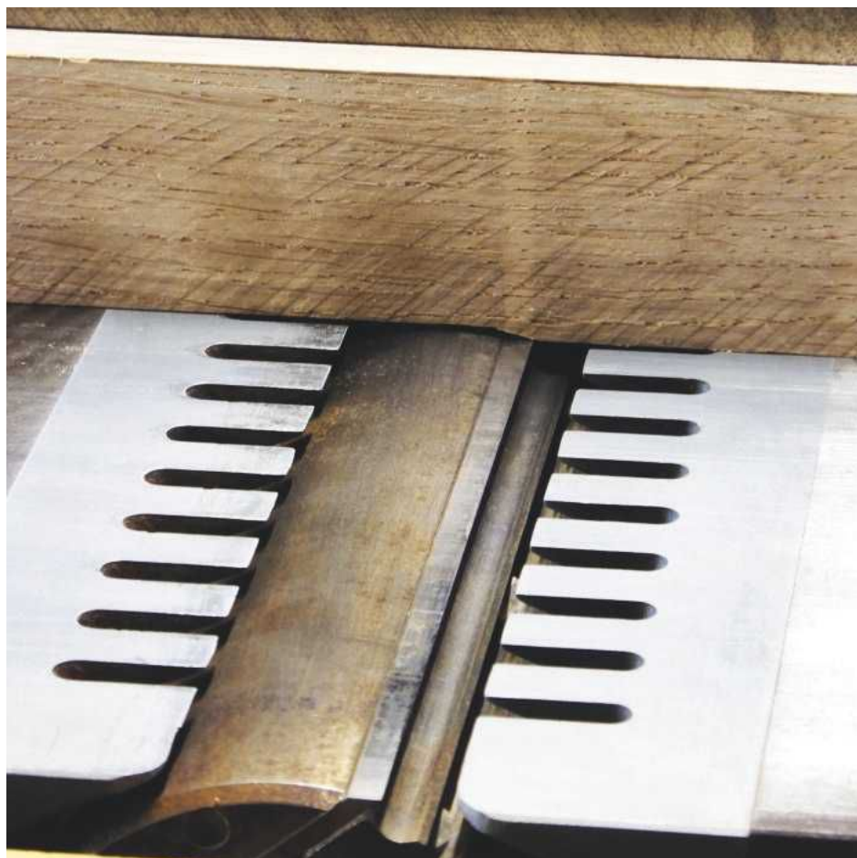
PIC 7. A cut partly made. You can clearly see that both bottom edges of the workpiece are in contact with their respective tables
