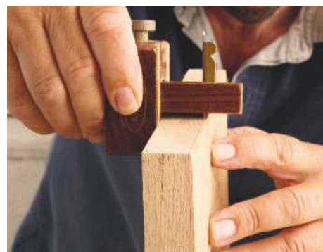
PIC 13. With one face and both edges planed, I use a marking gauge to score a line ready to plane the second face down to final thickness
