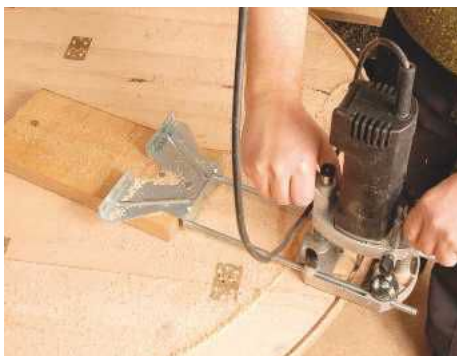
PIC 15. After gluing the boards together, I use a small trimming router to cut the top as a true circle
