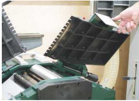
It's easy and quick to change from planing to thickening with one hand
