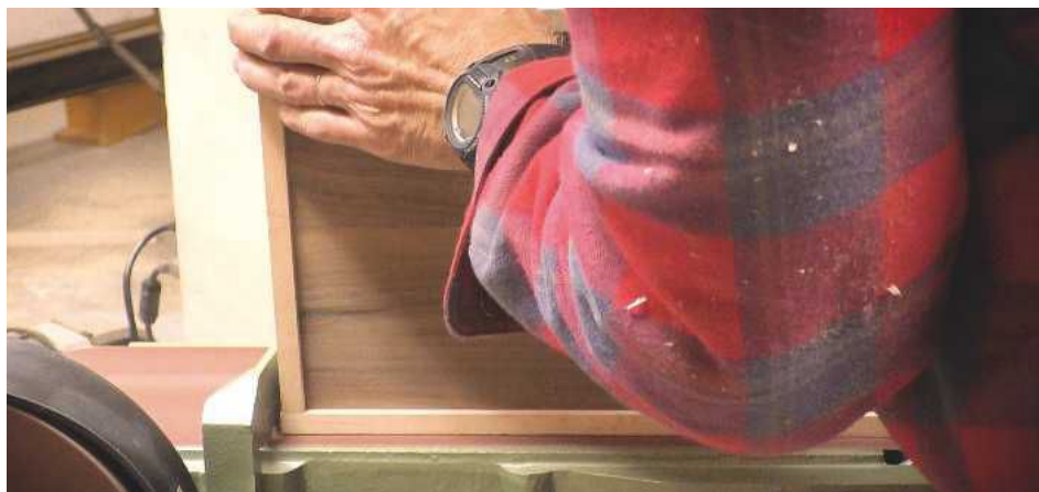
PIC 20. Sanding the joints in order to remove any excess material
