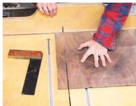
PIC 24. Cutting the top panel to the correct size in order to fit into the rebate
