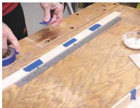
PIC 35. Taping the tray pieces together using masking tape
