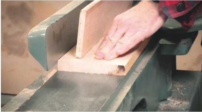
PIC 4. Joining the maple face
