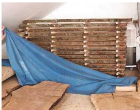
PIC 6. I stacked the 'green' boards with 'stickers' to separate them in the warm workshop loft, initially helped along by a dehumidifier
