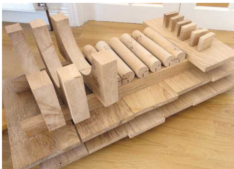
PIC 5. Component blanks full of promise; satisfying in their own right. Notice the quadrant grooves in the pillars. I'd intended to complete these cuts later to form a \frac{3}{4} in cylinder pillar to clip round a square board, but this didn't happen. The grooving did, however, come in useful
