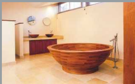
The rings forming the blanks for William Garvey's round, teak baths are built up brick-fashion, glued together, and then turned to shape – no mean feat
