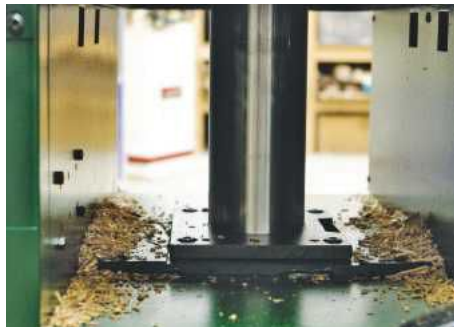
Single pillar support for the thicknesser table, which should be locked after each adjustment
