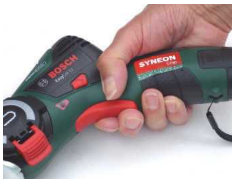
To activate the large trigger you first depress a lock-off button, accessed from either side
