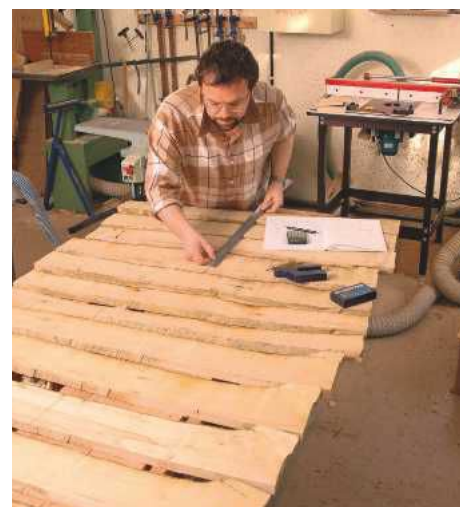
PIC 7. The dried boards are laid out in sequence to check for straightness, twisting or cupping
