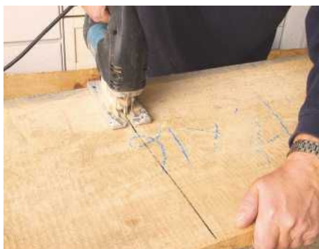
PIC 9. I find the hand-held jigsaw versatile for roughly cutting larger boards down to size
