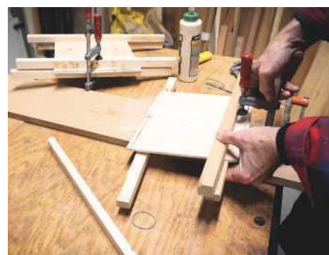
PIC 33. Gluing and clamping the tray pieces
