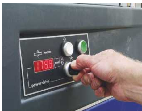
'Power Drive' electronic table height adjustment is a bit of an indulgence but it guarantees repeatable accuracy to 0.1mm
