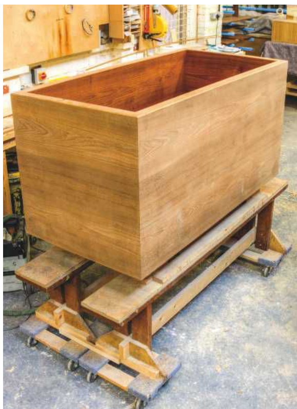
PIC 3. Teak veneers conceal the work of the marine ply core of William Garvey's bath; those mitred corners hold back half a ton of water
