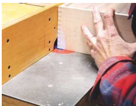
PIC 22. Cutting a 6mm wide rebate along the top edge that is 5mm deep
