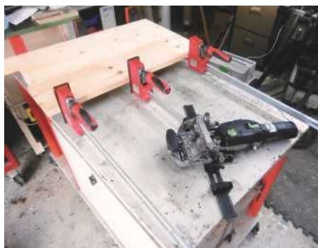
PIC 2. Building up the headboard panel
