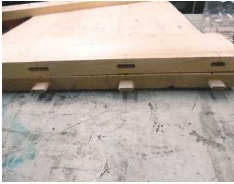
PIC 7. Leg mortises cut wider for movement
