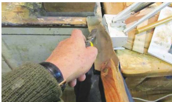
PIC 16. A few strokes against a stiffish piece of leather put a final polish on the edge and remove any loose metal particles left over from the grinding
