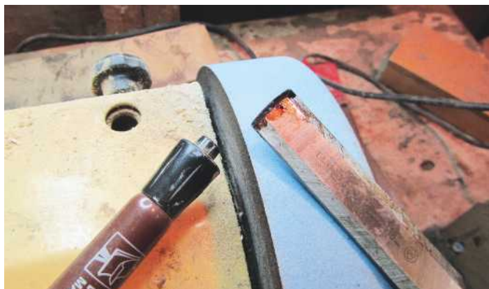
PIC 6. Professional woodturner Mick Hanbury recommends rubbing ink over a bevel before grinding. When you later inspect the blade, the ink marks give you an instant guide as to whether you're grinding evenly
