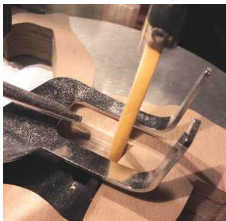
PIC 15. You can now mount the self-made sanding strip in your scrollsaw and sand down the sides of the warrior...
