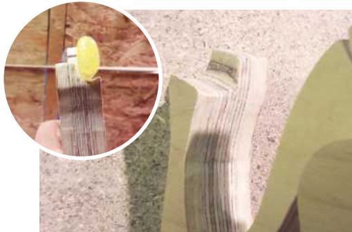
PIC 8. The warrior's hand needs to be shaped to ensure it properly accepts the knife handle you intend to place in it
