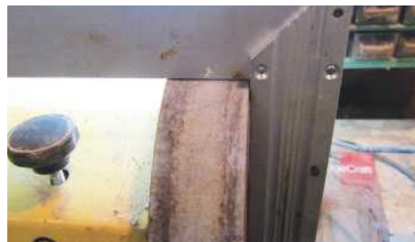
PIC 3. A set-square helps to make sure that you don't inadvertently create a slope on the wheel
