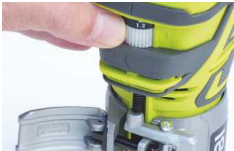
Open the large locking lever for fine adjustment via a threaded steel rod
