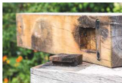
PICS 4&5. Visible fixings have been kept to the bare minimum; those that can be seen are discretely placed and neatly pocketed. This coach bolt ties the back of the arm to the seat; to avoid using a second bolt in the arm, however, the front is retained by an oversized button – the sort of thing you'd normally find fastening a tabletop to its apron – that keys into a mortise in the arm
