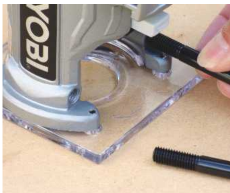
The alloy guide fence is fitted to the base with a pair of 7mm threaded steel rods
