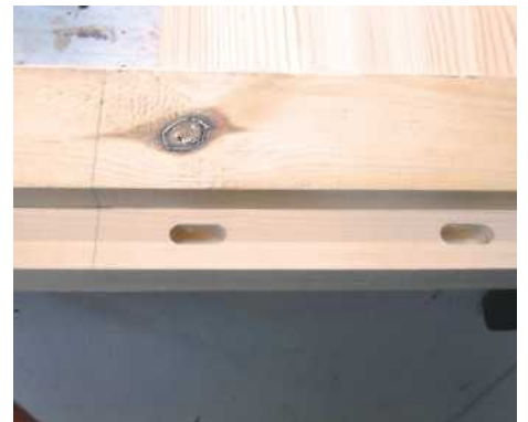
PIC 11. Side rail Domino locations in leg
