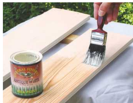
STEP 24. Remove the shelves and brush on a couple of coats of suitable paint. This milk paint does not need a primer
