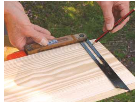
STEP 3. If the corners of the room are out of square, use a sliding bevel to mark the timber before cutting
