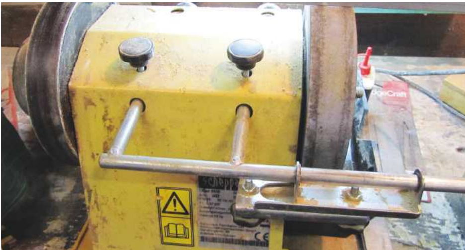
PIC 1. Most grindstones – like this ageing Scheppach – have a water-cooled stone at one end, and one or more leather wheels at the other
