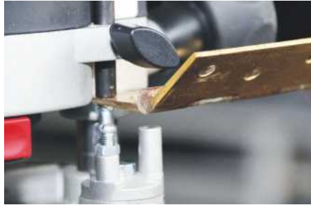
You can use the turret to gauge against fittings such as hinges...
