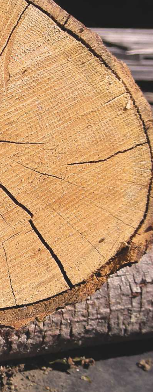
FIG 1. The way in which wood shrinks
