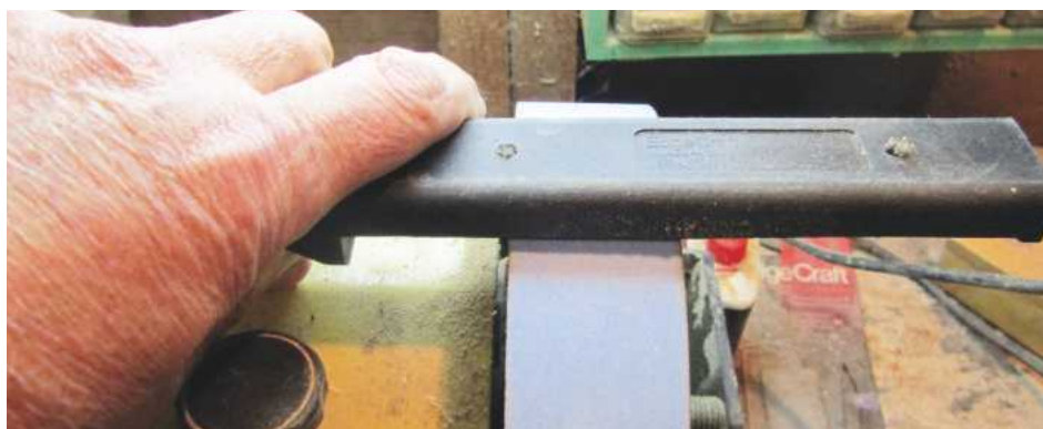
PIC 4. Any strong file or diamond-embedded abrasive plate can be used to flatten the wheel by hand
