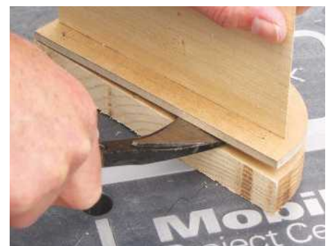
STEP 12. Prise the template carefully off after routing, then repeat for the remaining brackets
