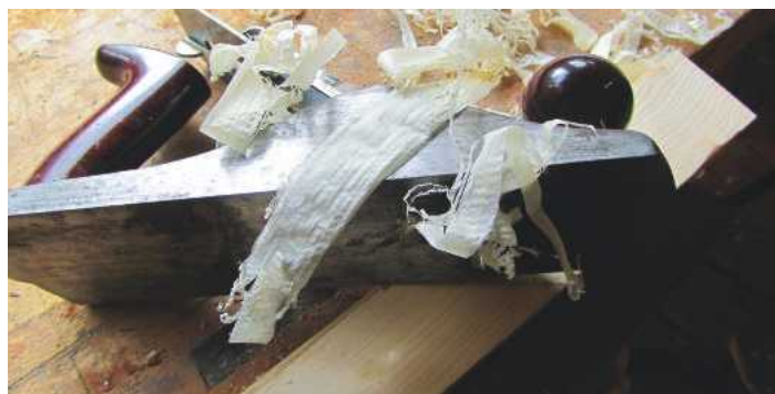
PIC 21. Clean, evenly translucent shavings are good evidence that the plane's blade is now square to the sole and scarily – if not terrifyingly – sharp
