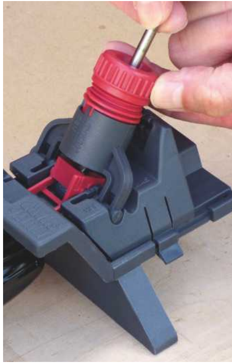
Left and right options for the carriage align the bit with the appropriate wheel
