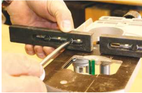
The sliding fence facings allow full support for different sized bits and applications
