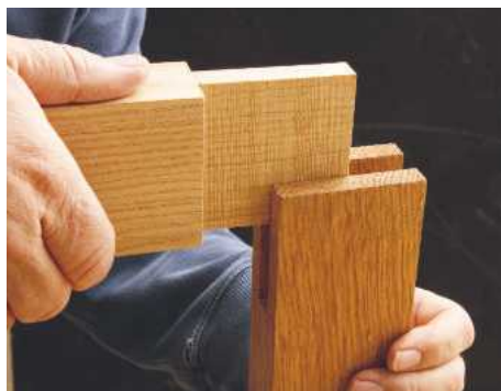
PIC 11. After spending some time setting up, the slot or 'bridle' joint is quickly repeated with four shims on the bandsaw and fits together snugly every time
