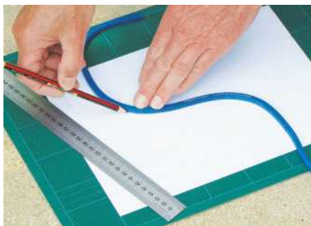
STEP 5. Design the bracket first on paper, using a flexible or French curve to obtain smooth, flowing radii
