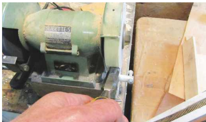
PIC 15. A felt wheel is a quick way to polish up the face or back of a blade, but remember to hold it tip-down against a wheel which is spinning towards you, and remove it frequently so that the blade doesn't overheat and lose its 'temper' – hardness
