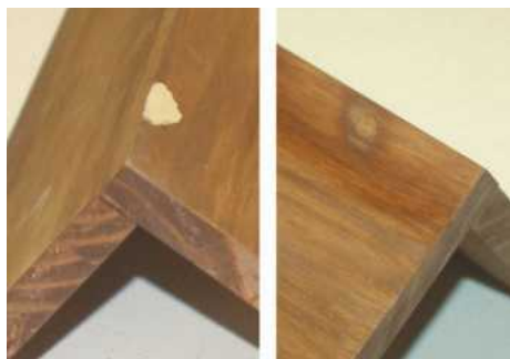
PIC 7. Drill two countersunk pilot holes through the lid back and into the lid front
