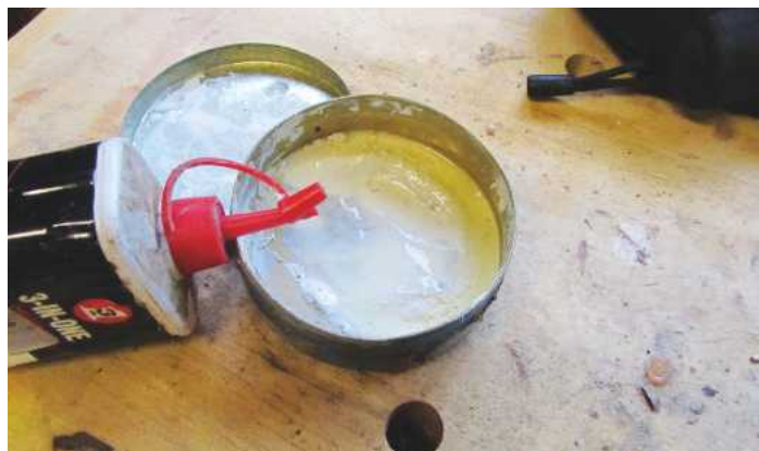
PIC 13. Jeweller's paste, used on leather wheels to polish an edge, often dries out in a workshop. It can be revived by mixing in a little oil
