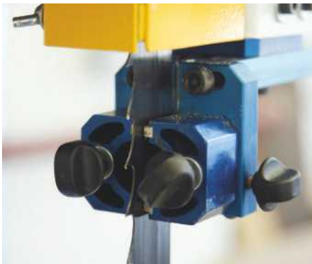
PIC 6. Cool blocks are low friction guides that provide an alternative to roller bearings
