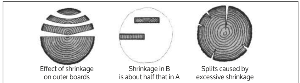
FIG 2. Basic shrinkage in the log
