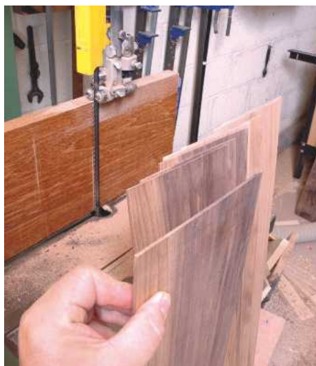
PIC 10. With a high fence mounted parallel to the blade and a millimetre or so away, the bandsaw can cut thin sheets of hardwood for veneering or laminating
