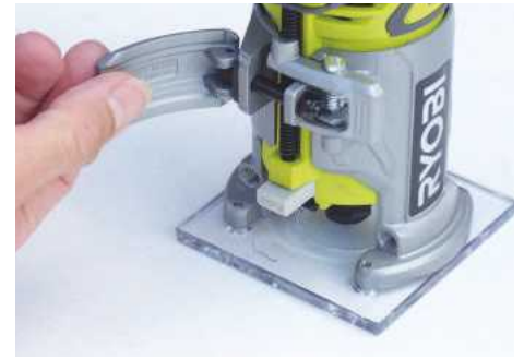
Depth setting is clever, with coarse and fine adjustment combined in a two-way lever
