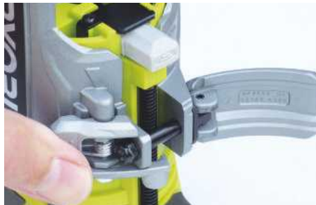
Depressing the spring-loaded secondary lever underneath disengages the rod
