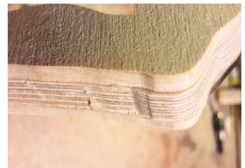
PIC 10. If a lot of glue leaks out of the sides during gluing, you may want to remove the dried glue with a knife before you start the sanding process
