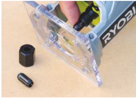
Two collets are provided (1/4in and 6mm), plus a 6mm straight bit
