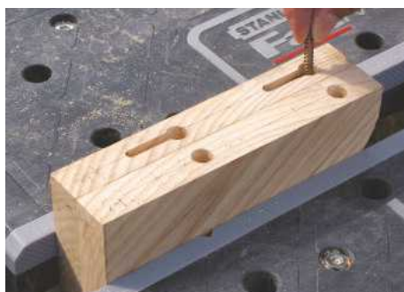
STEP 17. Starting from the hole, proceed to rout a 6mm wide slot. Follow with a dovetail bit set to the correct depth
