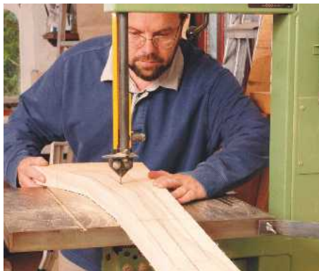
PIC 7. One of the main uses of the bandsaw is for cutting out curved and angled components
