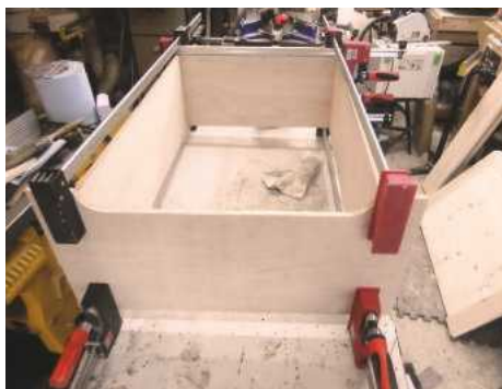
PIC 15. Glue-up of box frame
