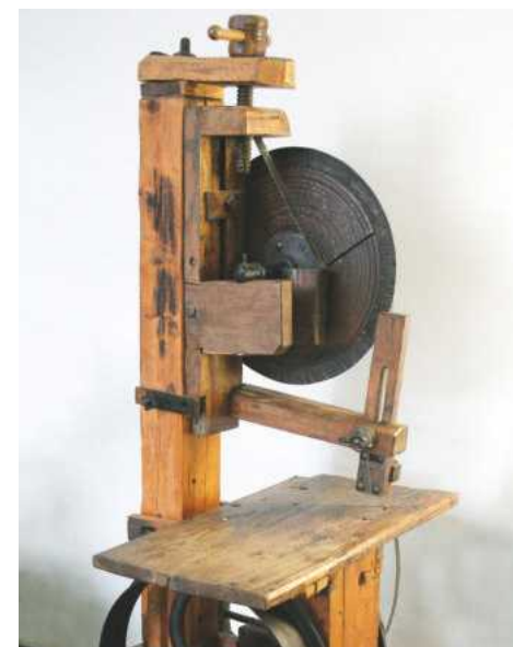
PIC 2. This treadle-operated bandsaw was built by a German village craftsman about 150 years ago while the first ever bandsaw was patented in England over 200 years ago
