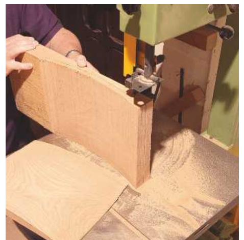
PIC 9. With a length of blade exposed the bandsaw can cut deep into the wood, such as when making wide curved components
