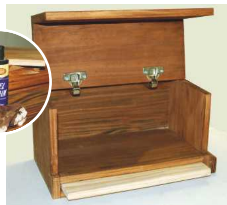
PIC 9. For the bread bin interior, use a stain in an antique oak colour, but check to make sure the one you use is food-safe
