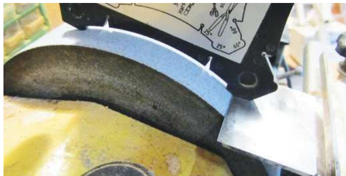
PIC 19. Plane blades demand a little more precision. Hence, here, a more determined attempt to repeat its 25° angle and to set it firmly in a blade-holding jig
