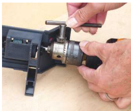
A spindle running through the jig is secured in the chuck, then you're almost ready for action
