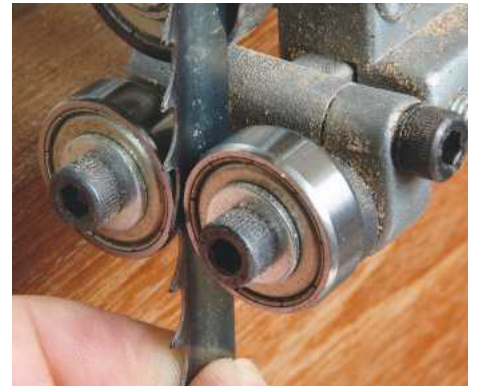
PIC 5. The blade is secured above and below the slotted table by a wheel each side and one behind the blade
