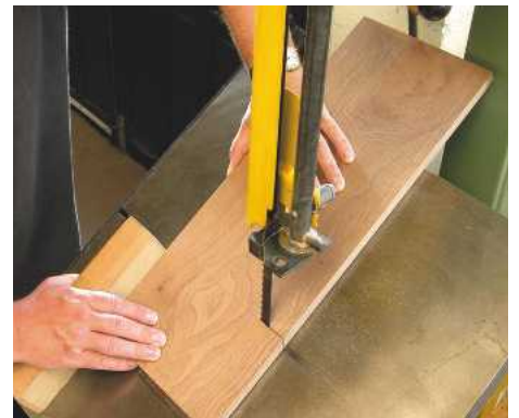
PIC 8. The bandsaw table can be tilted for making slanted cuts
