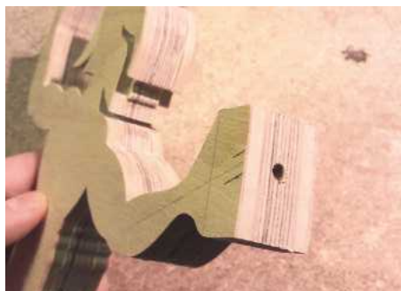
PIC 9. To make the second hand stronger, I drilled a 4mm hole and inserted a 4mm brass rod to strengthen it
