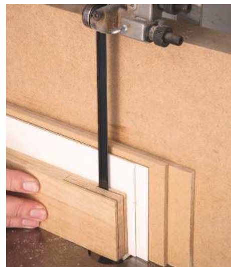
PIC 12. A set of two thin shims made from card and two thick made from MDF are used here to rip saw the second side of the slot
