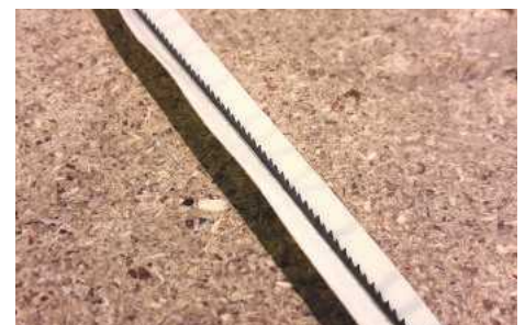
PIC 13. Taking a wide scrollsaw blade, cut off a strip of the abrasive with the adhesive tape attached, with a width of roughly six times that of the scrollsaw blade
