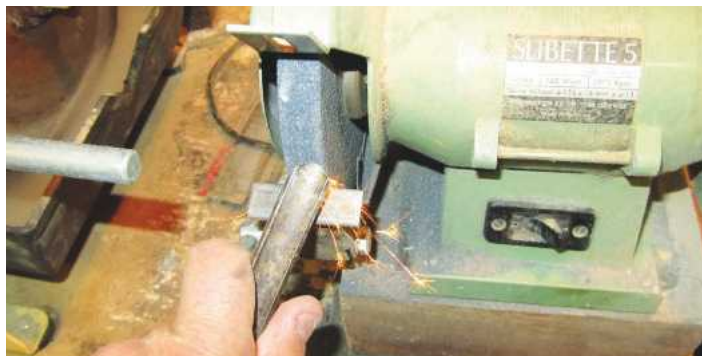
PIC 18. Turning tools aren't hard to sharpen freehand. Roll the bevel against the wheel until sparks just begin to fly over the nearside face. Lift the tool off frequently to let it cool and to check that the bevel is smooth. Finish the tool off on a felt wheel, but don't bother removing any wire-edges; the lathe will do that for you in seconds
