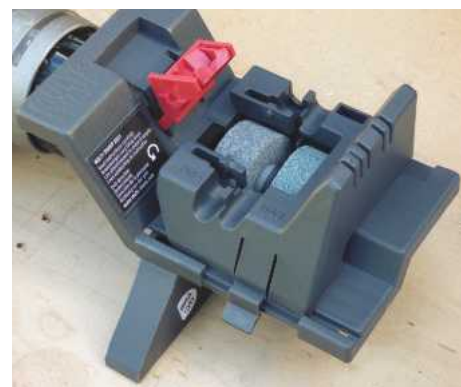
Both the grey aluminium oxide wheel and the green silicon carbide wheel are 15mm wide, with a diameter of about 35mm
