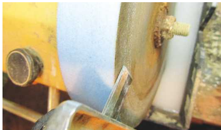
PIC 12. Purists say you shouldn't flatten the back of a blade on the side of a wheel; you should use a lapping stone or wet-and-dry paper stuck down on glass. I say it works well enough and it's much faster
