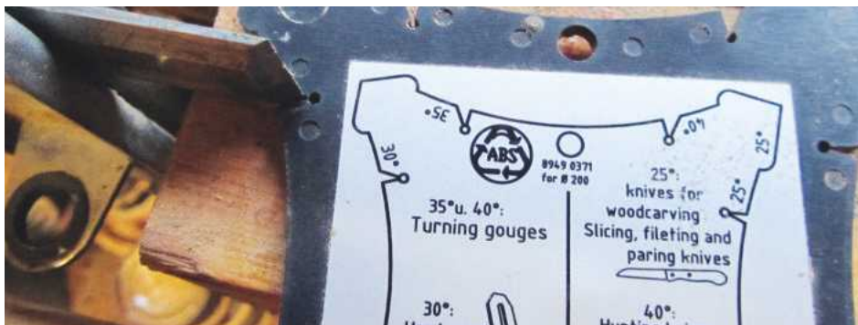
PIC 11. This angle gauge – like most of its kind – is too small to be reliably accurate, and I had to spend 20 minutes cleaning it to make it readable enough for a photo!
