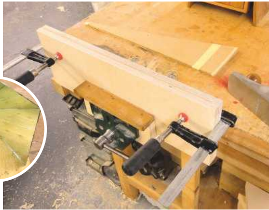
Shooting the balance veneers using a finely-set hand plane
