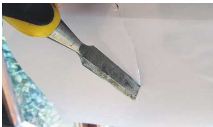
PIC 17. A smooth cut through paper is not a bad test of a blade. For my money, this edge is now ready to go back to work, not more than five minutes after starting
