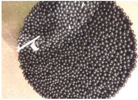
PIC 2. The lead beads in the base will aid stability
