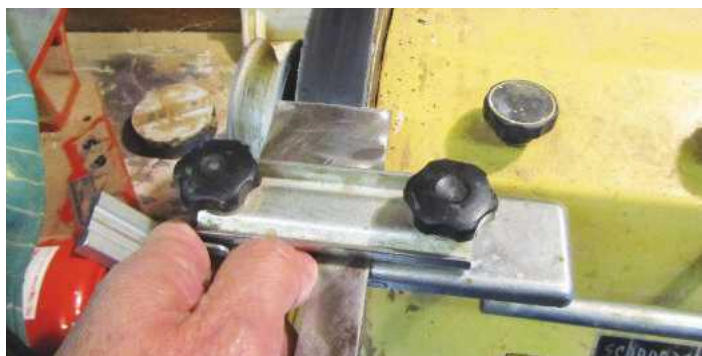
PIC 20. Once the plane was ready for polishing on the leather wheel, I was ready to finish it off by hand (you'll see that the jig is no longer riding on its bars)
