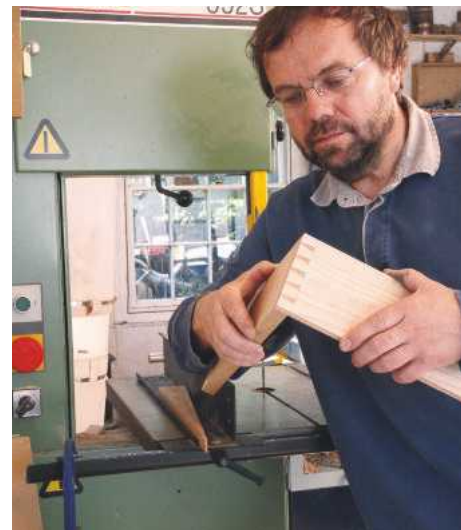
PIC 15. The tails and pins of a dovetail joint cut on the bandsaw are slotted together
