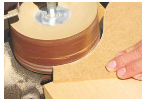
STEP 6. Transfer the outline to 6mm MDF; cut out and clean up the template on a sanding drum
