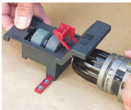
The locating foot is screwed down, enabling the jig to slide into place
