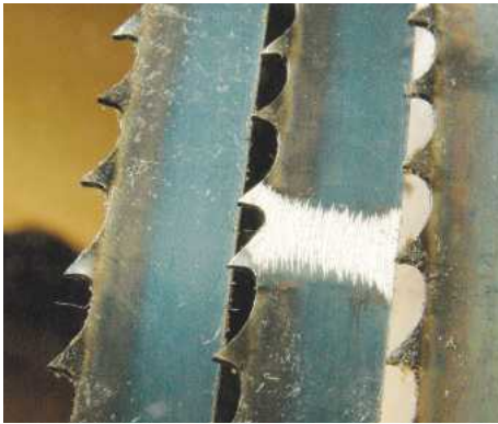
PIC 3. The toothed steel strip, which forms the saw blade, is welded together as a continuous band
