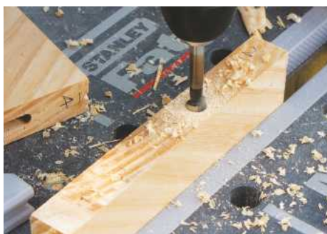
STEP 16. Drill a 13mm hole at the lower end of each slot. This creates the clearance needed for the screw head
