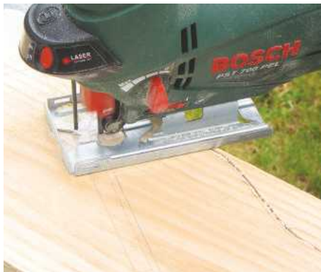
STEP 8. Cut out each bracket with a jigsaw fitted with a narrow blade. Allow 2mm waste outside the pencil line
