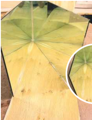
A pair of mirrors were used to visualise the fan design before any veneer was cut
