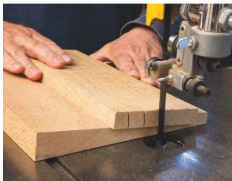
PIC 14. A wedge-sectioned block is used to support the wood while cutting the pins of a dovetail joint
