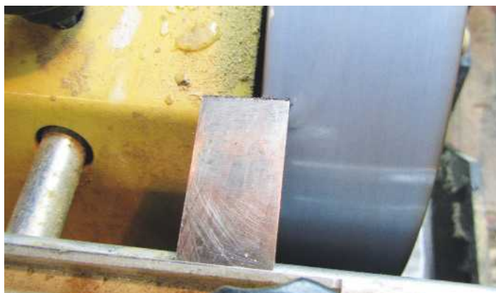
PIC 8. Two minutes of firm grinding remove the camber and raise a lumpy wire edge. The water in the stone stops the metal overheating
