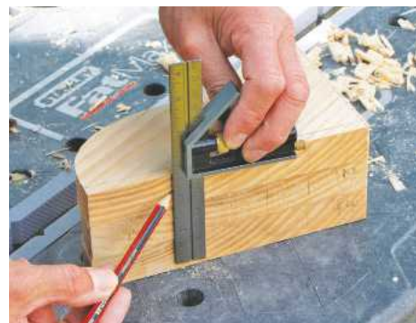
STEP 15. Using a square, measure and mark out the dovetail slot hole centres on the rear edge of each bracket
