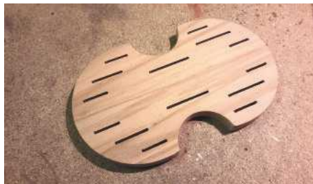
PIC 20. Use a 3mm drill bit to drill holes at each end of each of the slits on the front layer
