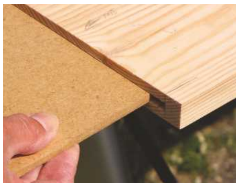
STEP 22. The two shelves meet in the middle, so rout a 6mm slot in each end for the loose tongue
