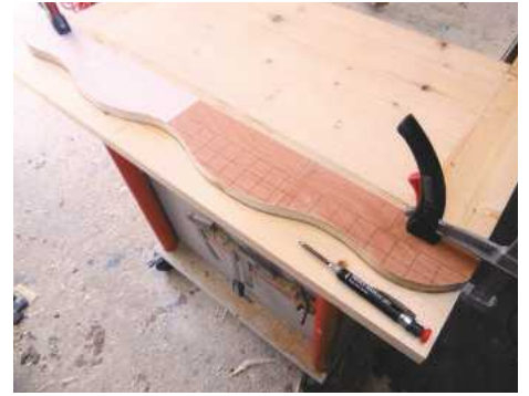
PIC 9. Top shape template from 1:1 printout
