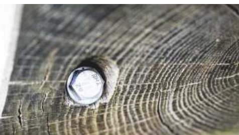
PICS 4&5. Visible fixings have been kept to the bare minimum; those that can be seen are discretely placed and neatly pocketed. This coach bolt ties the back of the arm to the seat; to avoid using a second bolt in the arm, however, the front is retained by an oversized button – the sort of thing you'd normally find fastening a tabletop to its apron – that keys into a mortise in the arm
