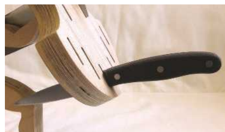
PIC 19. The slit length has been adjusted for this knife
