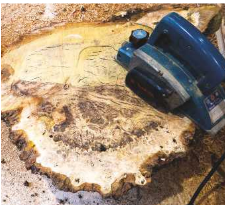
The cut left by the tree surgeons made flatter with a hand planer
