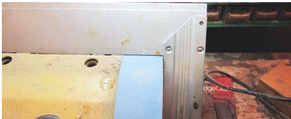
PIC 5. Cleaned, flattened, dressed and checked for square, the grindstone is ready to go back to work
