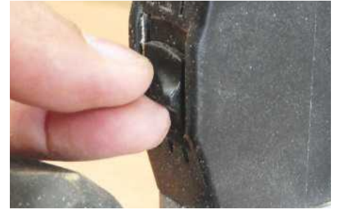
The side-mounted sliding power switch is easy to operate
