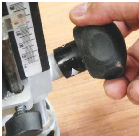
The simple twist lock plunge is great for fast, easy and controllable plunges
