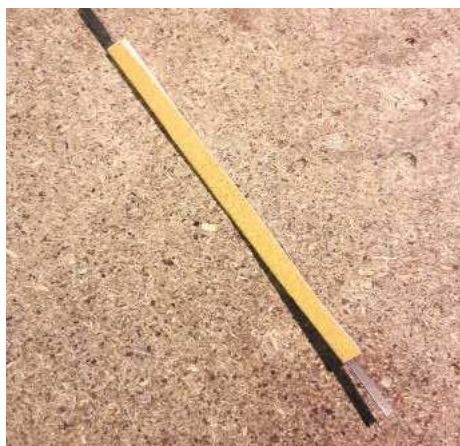
PIC 14. Fold the strip along the middle and then remove the back of the adhesive tape. Place the scrollsaw blade with the flat side into the middle of the abrasive and fold again
