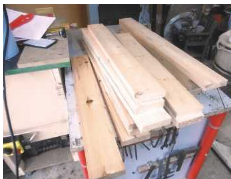
PIC 1. Head and footboard timbers ready to stick
