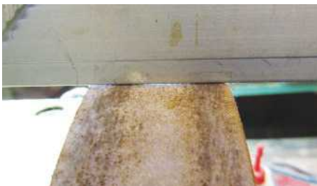
PIC 2. A straightedge reveals a hollow in the middle of the grindstone and a slope falling away on the left-hand side
