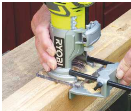
The Ryobi is a brilliant little tool for inlay work, adding chamfers or smaller edge profiles
