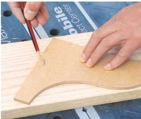
STEP 7. Draw around the template onto the timber selected for the brackets. You need to make sure the grain runs diagonally
