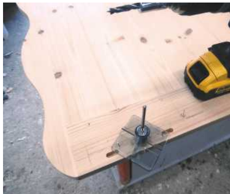
PIC 10. Drilling template for the leg bolt hole
