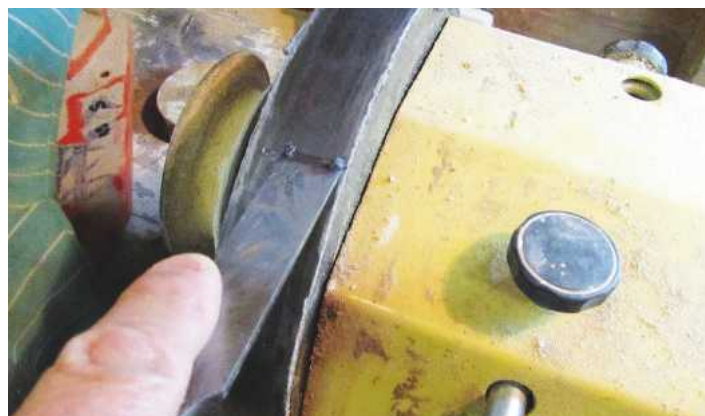
PIC 14. You can of course use a tool-holding jig when you hone a blade on a leather wheel, but I find it simpler to hold the bevel on the wheel by hand. The pattern of slurry build-up around the edge will tell you whether the wheel is getting right to the tip of the blade. So will the feel of the tool in your hand and the sound of the wheel against the metal
