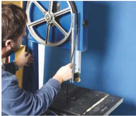
PIC 4. Changing the blade on a modern bandsaw with the power isolated, the covers opened and the upper wheel lowered to remove tension
