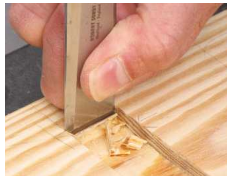
STEP 21. Square off the rounded end of each housing with a wide chisel. Each bracket should be a snug fit
