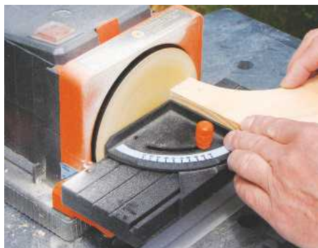
STEP 14. It's easiest to clean up the short end on each bracket with a disc sander. Alternatively, use a block plane
