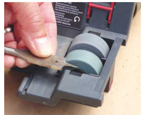
You can regrind flatbits, too, though results are less accurate as there's no guide as such
