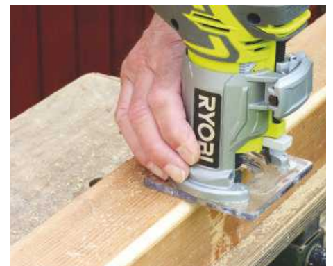
Testing the Ryobi with a (bearing-guided) roundover bit. Fitted with a 4.0Ah battery, an ogee bit cut 14m of softwood
