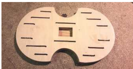
PIC 21. Use a scrollsaw to cut out the slits, by cutting along the lines and connecting the two holes at the end of each slit
