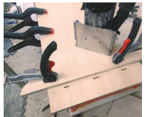
PIC 14. Dominos for the storage box front
