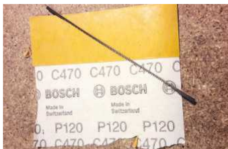
PIC 12. Apply double-sided adhesive tape onto the back of a piece of abrasive
