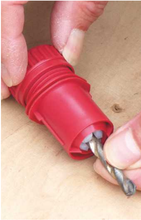
The bit is inserted into a vertical turret, which presents the tip at 118° to the wheel
