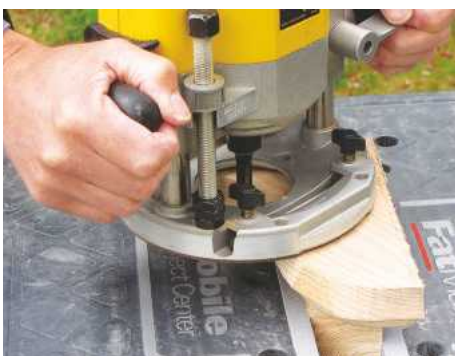
STEP 10. Grip the block in a vice and rout around the template. Use a long, straight bearing-guided router bit
