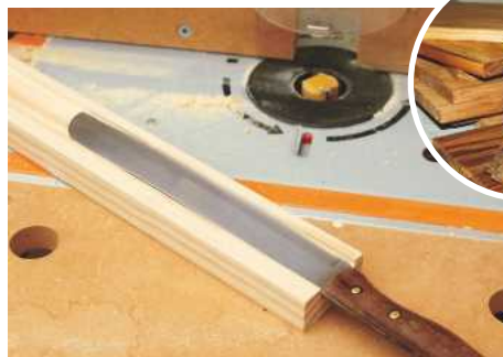
PIC 8. Use a router to cut a 4mm deep slot in the pine section
