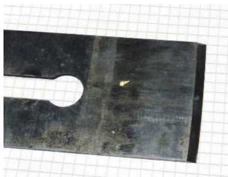
PIC 7. You can see that even with this brilliant device I have managed a less than brilliant result. It would take a little more practice to obtain an even curve
