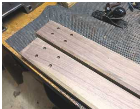
PIC 20. Pre-drilling and counter-boring screw holes to attach coat hook boards to the posts
