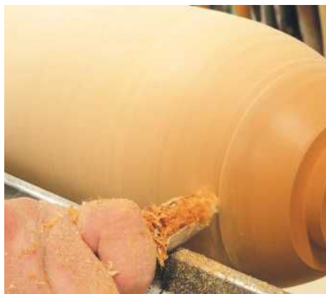
STEP 10. Turning of an egg shape is completed using the bowl gouge, all the time working downhill; this means you are working with the grain and will get the best finish off the tool
