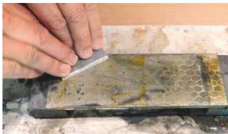
PIC 3. As always, the back of the blade must be flattened, at least at the cutting edge
