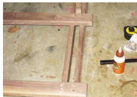
PIC 23. Plugging stretcher screw holes
