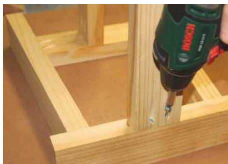
PIC 4. Attach the side rails with wood glue and pocket hole screws
