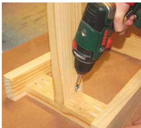
PIC 6. Use wood glue and pocket hole screws to secure the top and bottom rails to the sides
