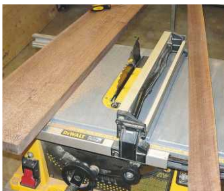
PIC 3. Ripping the posts (PLEASE NOTE THAT BLADE GUARD HAS BEEN REMOVED FOR CLARITY)
