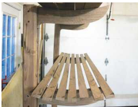
PIC 24. Finalising slat spacing
