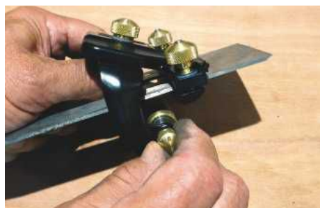
PIC 6. The clever little micro-bevel knob clicks at 90° increments. Rotating it brings the roller down just a little so that a finer edge can quickly and easily be honed
