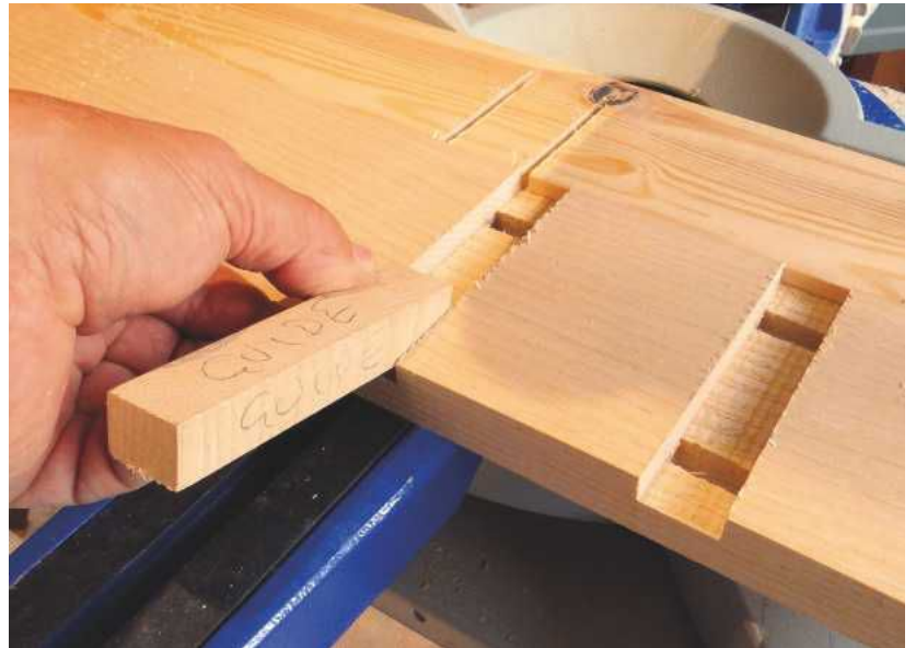
PIC 3. This trenching would be better done with a router in a jig so that the tenoned rails would fit uniformly snugly into it. Instead I used an offcut as a guide and trenched on a mitre saw. It is worth remembering to sand the rails first because this makes them thinner, but here, on the underside of the table, such refinement was not necessary
