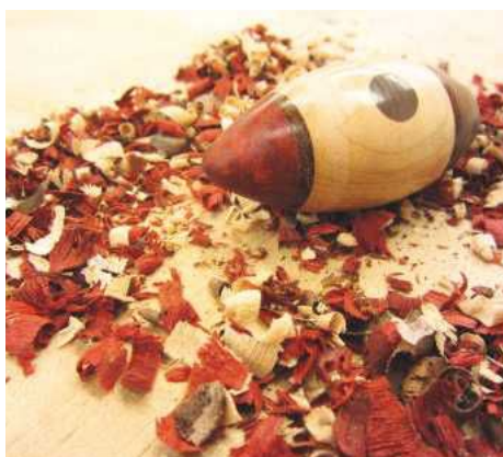
PIC 12. The rocket body all sanded and the window finished on the lathe using CA adhesive
