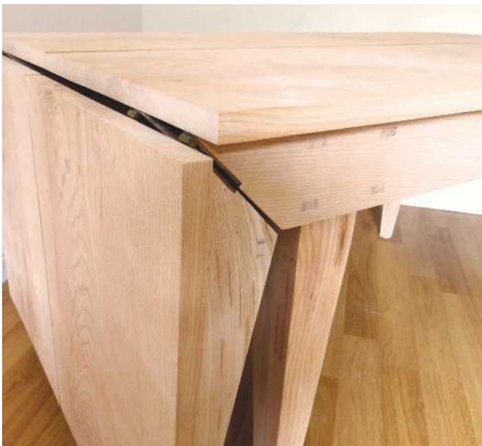
PIC 13. A silly error. Because of the centre of gravity of the flap, it doesn't fall fully vertically and so the 45° meeting doesn't close up. Ah well!
