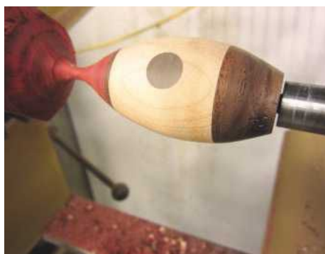
PIC 11. Once turned, the rocket body needs to be sanded through a range of abrasive grits until you've achieved a consistent, smooth finish
