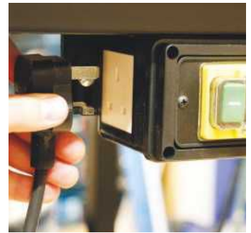
The router is controlled by plugging it into the NVR switch provided
