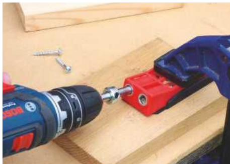
Some pricier pocket hole jigs have one built-in to anchor workpiece and jig together, though a standard quick-grip cramp will suffice here
