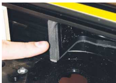
The sponge helps prevent dust ingress behind the fence when routing
