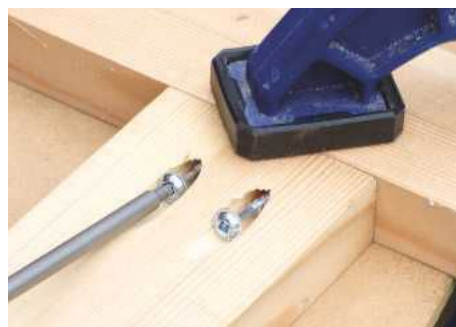
Ideally you'll need a face cramp when jointing same thickness components, such as framework
