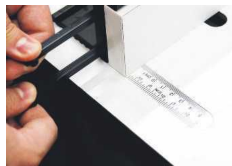
These two rods slide behind the outfeed fence to pack it off for planing functions
