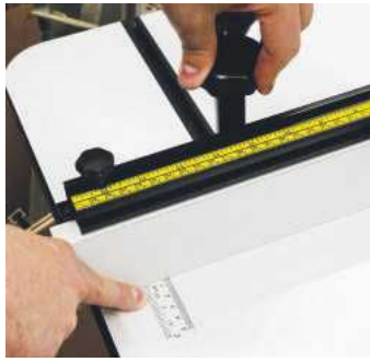
Two locking knobs secure the fence with twin scales on the table, thus aiding positioning
