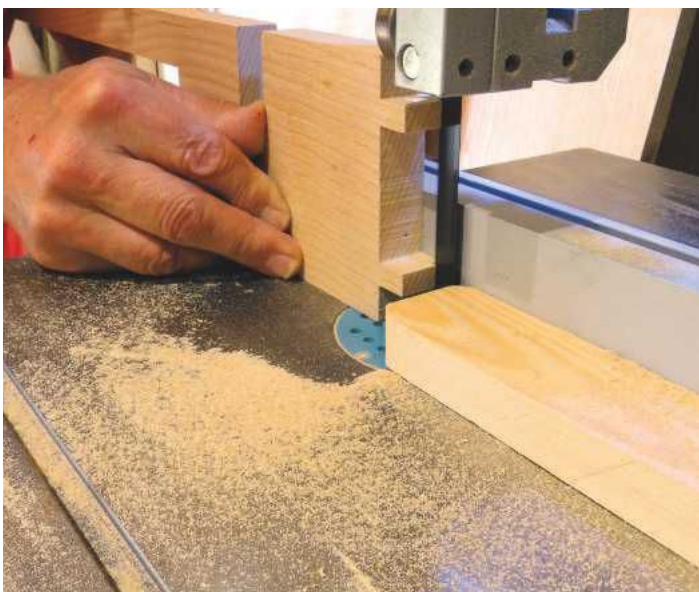
PIC 8. Wedging 1: Arguably the slots in the tenons might slope in a little towards the body of the wood so that there is no danger of the remaining sliver shearing under the strain of the wedge. Arguably also the mortise should be flared to accept the wedge and, in effect, create a dovetail joint. I did neither
