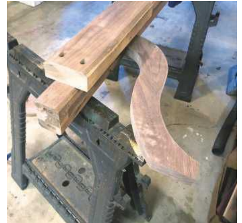
PIC 13. Attaching the posts and S-curve supports to the bases with 10 × 50mm Festool Dominos
