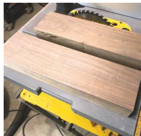
PIC 2. The two bases trimmed to correct length/width (PLEASE NOTE THAT BLADE GUARD HAS BEEN REMOVED FOR CLARITY)
