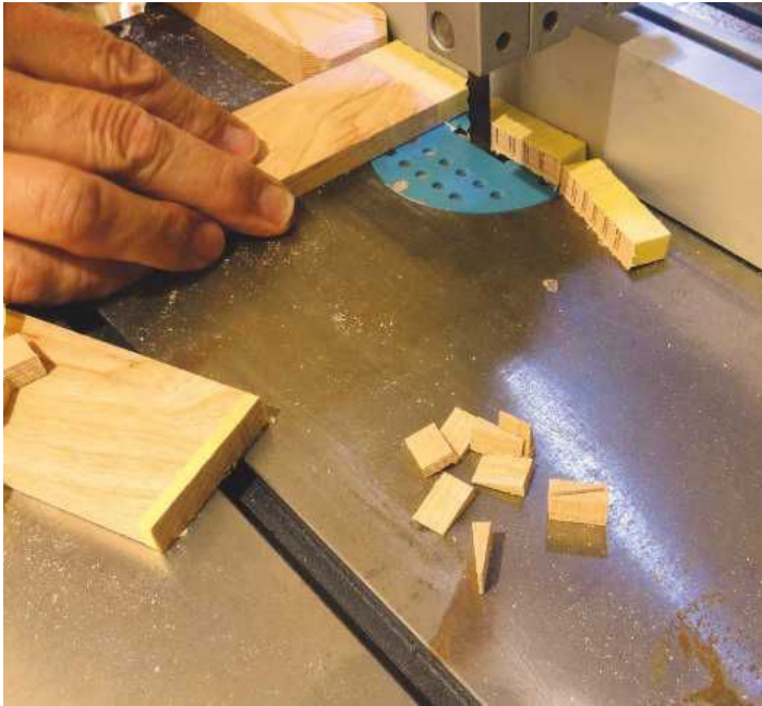
PIC 10. Wedging3: Before the wedges are sliced off, the cut end is wrapped in masking tape so that they don't fly everywhere or get caught by the blade. (I've shown a sequence in one shot: in operation the table should be clear)
