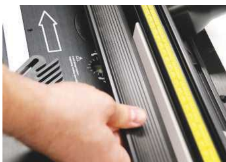
Checking the fence facings with a straight edge showed them to be smack on
