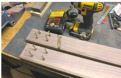
PIC 21. Starting the screws
