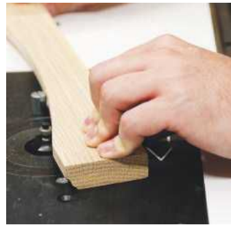
You can see the principle here, providing a pivot point to introduce the work to the cutter
