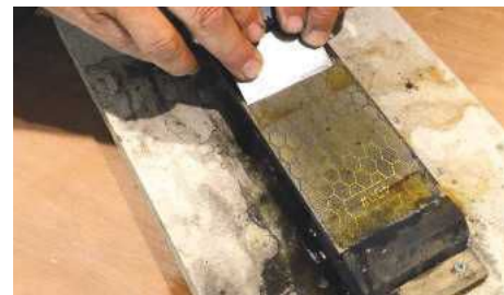
PIC 5. If you have to restore a badly sharpened blade it will take a little time, beginning on a stone such as this at 400 grit, then flipping it over to finish at 1,000 grit. Once the correct angle is established, it takes a matter of seconds and just half a dozen strokes to bring back a perfect edge. The Veritas guide is so accurate that the precise angle can be repeated, and work kept to a minimum
