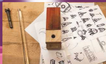
PIC 7. The hole drilled in the blank, ready to accept the acrylic rod
