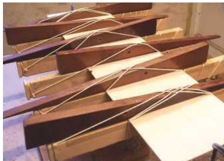
PIC 20. The soundboard in a wedge and lace jig
