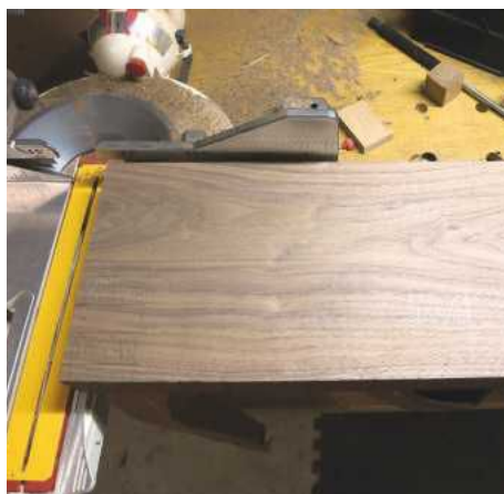
PIC 1. The two bases marked out on a single block of 50mm walnut – here you can also see marked the notional locations for upright posts
