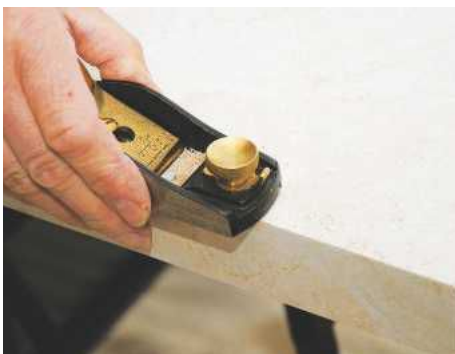
STEP 10. Carefully trim the lipping with a finely-set block plane, working down almost to the surface
