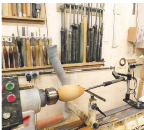
STEP 16. The rig is all set up on the lathe. It's important to get a good fixing to the lathe bed to avoid any chance of vibration. I do the initial hollowing without the laser attached
