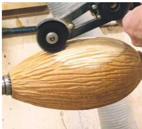
STEP 11. I wasn't going to texture this piece but I needed some way of hiding the unsightly split. The Arbortech with the mini industrial cutter was used to cut random grooves in the direction of the grain
