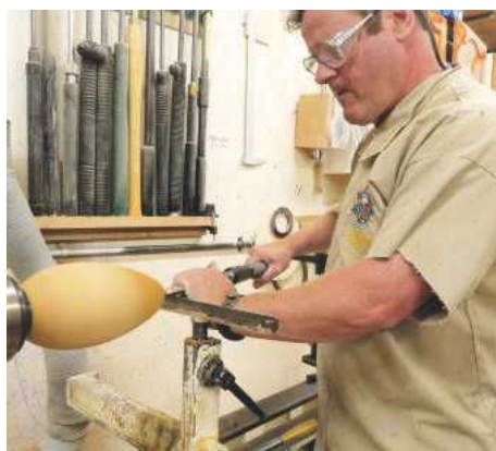
STEP 17. Not leaning over the lathe helps to make the whole process much more comfortable and enjoyable. The cutter is angled slightly down to take some of the force away from the cutting edge
