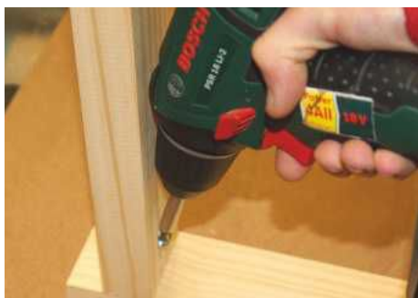
PIC 3. Secure the legs to the seat support using wood glue and 32mm pocket hole screws
