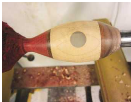
PIC 10. After some further turning and rounding over, the shape begins to look even better
