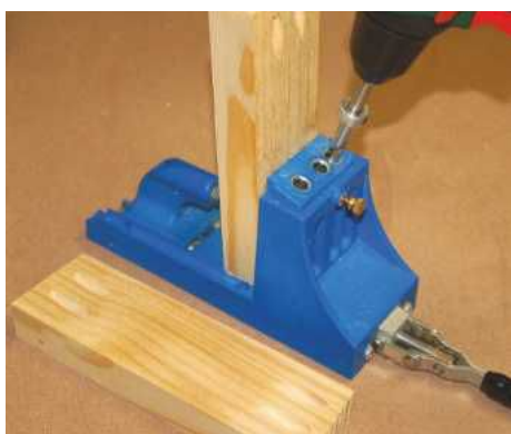
PIC 1. Drill pocket holes into the rails, cross-pieces and legs
