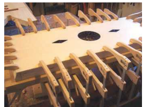
PIC 24. The soundboard is held in place with cam clamps
