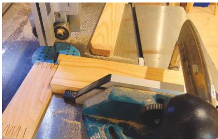
PIC 9. Wedging 2: I'm rather proud of this. Previously I've cut wedges on the bandsaw more-or-less by eye, but in this case I thought you (and I) deserved something better. The sliding guide is slewed at 7.5°, and a stepped stop is cramped to it. Another stop prevents this carriage moving too far. A strip of wood is machined to the correct thickness and then chopped into half a dozen small sections. Each of these is sawn, flipped over, sawn again, turned round and repeated. Then the stepped stop is adjusted for the next saw cut. This arrangement took a while to work out and set up, but once done, I could have cut a thousand identical little wedges while listening to the afternoon play
