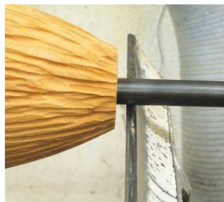
STEP 18. Keep the toolrest close to the work, and wherever possible, try to work over the stem of the rest as this will be the strongest part. I found it best to keep the tool presented horizontally
