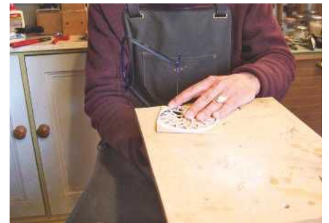
PIC 21. The sound hole rosette is first fretted out in the 2mm ply
