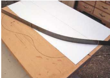
PIC 1. A steel ruler can help to create a smooth curve
