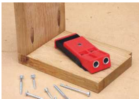
Once holes are drilled, swap to the screwdriver bit and assemble the joint
