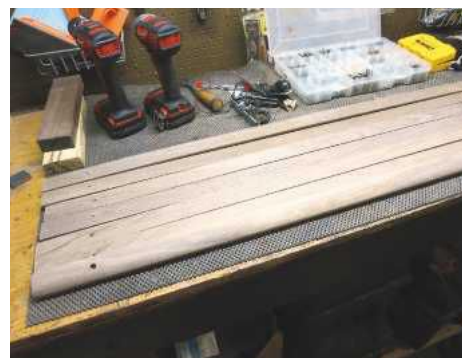
PIC 26. Slats sanded and pre-drilled
