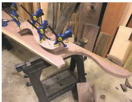
PIC 8. Once all the parts are cut to size, carefully glue everything up and clamp the whole stack in place
