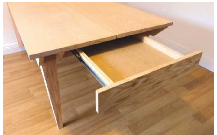
PIC 12. The drawer was given a secondary front so as to be invisible (which James fancied). The bottom of this front is pointed down so as to provide a hand-pull, and to relate to the slanting lines elsewhere on the table. I retained a gap between the boards to emphasise their width, though I concede that it is a little impractical as crumbs and spillage can fall through. If J & K wish to close it up, they can
