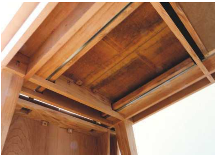
PIC 6. The drawer-runner idea seemed viable, but the frame of the flap was in the way. Square holes would allow the runner to slide through the flap frame to support it. And if I was going to all that bother, I might as well use runners at the other end and provide a drawer for place mats or suchlike. The drawer turned out to be shallow because my priority remained the structural integrity of that part of the frame. This was turning into quite a heavy structure and it needed to be strong. I couldn't think of a sensible alternative to an MDF drawer bottom (I had 9mm in stock) so that made it even shallower but still, I hope, useful
