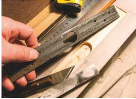
PIC 3. Heavy-duty keyhole brackets made from 30mm-wide lengths of 3mm steel
