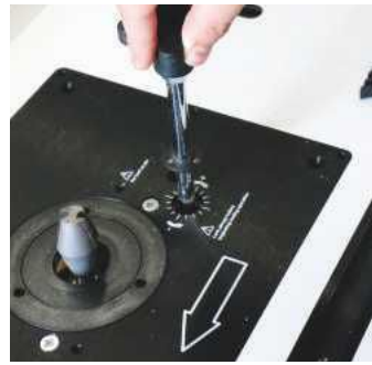
With a T11 router in place the cutter height can be easily altered from above the table
