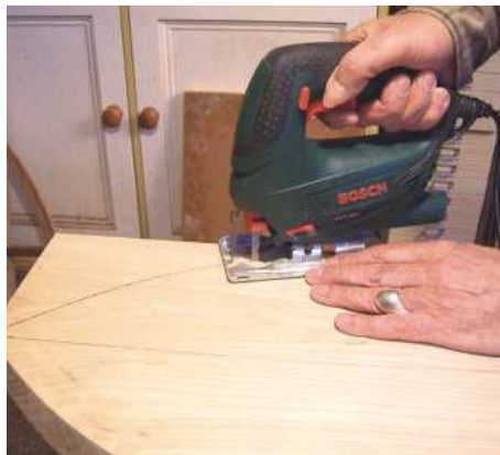
PIC 3. A jigsaw is used to remove waste wood
