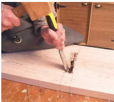
PIC 5. The mortise is chopped out with a chisel
