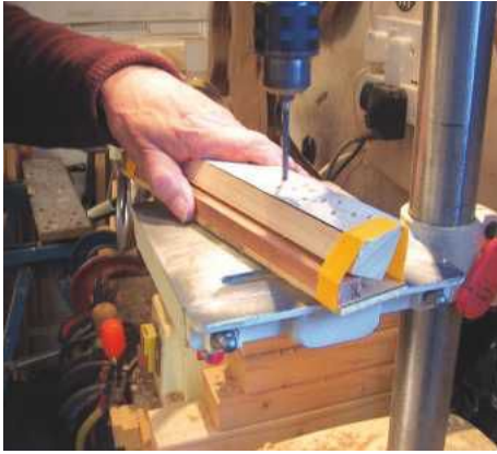
PIC 16. Taking the pin holes out on the pillar drill, helped with a simple jig
