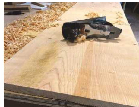
PIC 8. As a precursor to sanding, hand planing would be entirely appropriate, but as a final finish it is decidedly rustic
