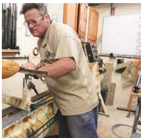
STEP 14. Here you can see my normal stance when hollowing on the big lathe. I could transfer the work over to one of my swivel-head lathes but they're not as powerful as this 3hp Oneway
