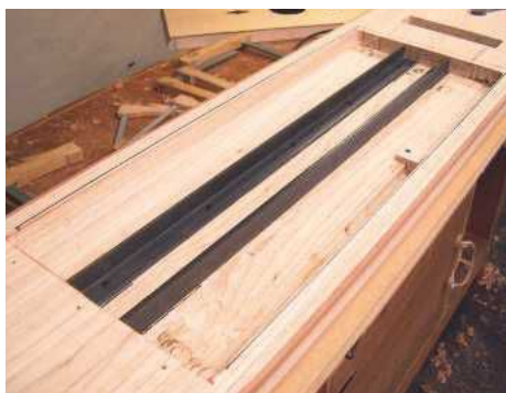
PIC 13. An angle iron is used to strengthen the back
