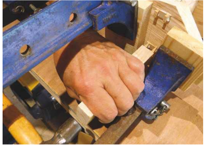
PIC 11. Wedging 4: What satisfaction little things can offer! Having jiggged up every stage of the way, each identical pair of wedges drove home simultaneously and perfectly, later to be sanded smooth
