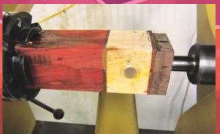
PIC 8. Chuck the rocket blank in your wood lathe and stabilise it using a live centre in the tailstock
