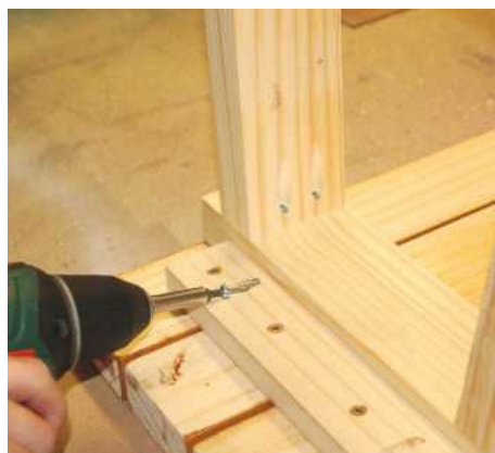
PIC 7. Mounting the bottom frame to the underside of the seat slats – push the frame in place between the two seat slat cross-pieces
