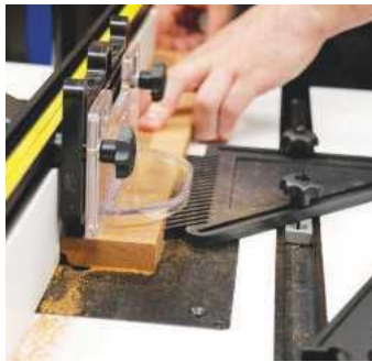
Once set up the featherboards keep the work tight to the table and fence for great results
