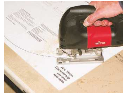
STEP 3. Stick the paper template to the underside with spray mount glue and proceed to cut carefully around the line
