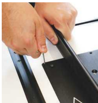
The insert plate has a series of levelling screws to get it flush to the table surface
