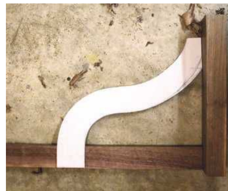
PIC 7. S-curve pattern in place between posts and base
