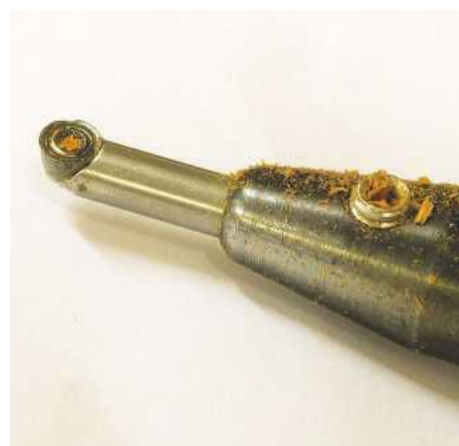
STEP 15. This hollowing tool with its small carbide cutter from Simon Hope is one of the best tools I've ever used. The combination of the big bar and small cutter is perfect for working blind
