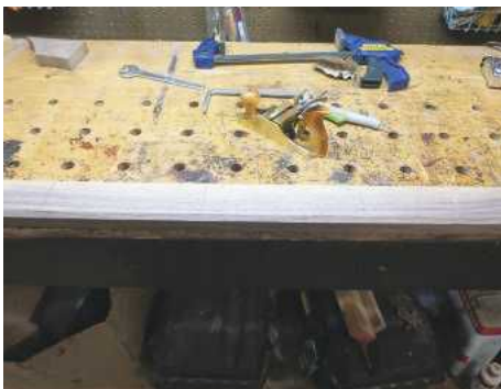
PIC 19. Final surface cleanup with an added chamfer
