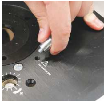
A lead on pin is provided for curved work; it stores on board when not in use
