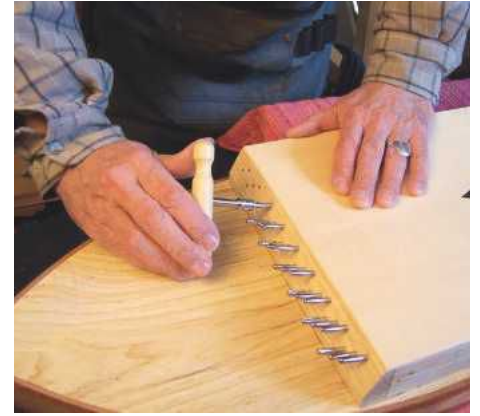
PIC 18. The tuners must be put into place with a wrench
