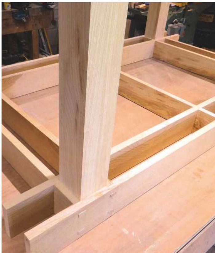
PIC 4. The basic frame jointed. I like this construction and I think I'll use it again on a simple table (more-or-less as seen here). The legs were later held in place by a single big screw. Being able to dismantle a table so thoroughly makes transportation easier
