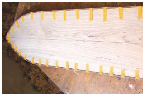
PIC 7. Masking tape holds the inlays in place as the glue cures
