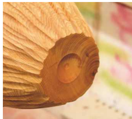
STEP 12. When hollowing in end-grain, it's an advantage to drill the centre out. I turned a small location hole in the end of the work using a spindle gouge, which ensures the drill will have a perfect start
