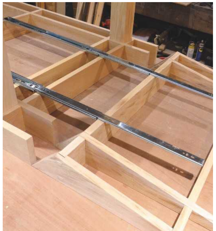
PIC 5. The drawer runners are beautifully engineered, telescoping out smoothly and remaining rigid in the vertical plane. Quite how rigid when put to such a task as this, I wasn't sure. No amount of theoretical design would have helped me here. I had to make the whole frame before I could know if it would work - albeit without the additional weight of the flap boards. On the other hand, I thought, how could it possibly not work? What would give way, buckle or break? Mmm
