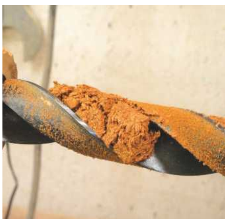
STEP 13. I used a twist drill as I like the way the shavings exit through the piece. You can see the way the shavings swell after they've been cut. Using a Forstner bit allows the shavings to back up behind it
