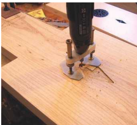
PIC 8. Sockets for the decorative lozenges are routed out
