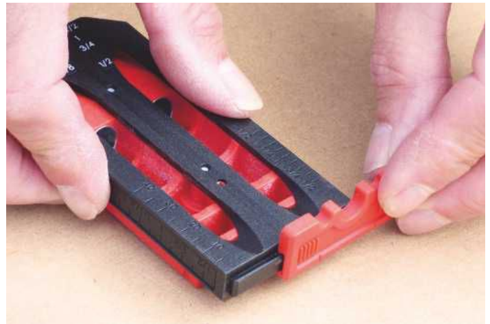
The end stop is simply reversed for drilling corner joints, for example
