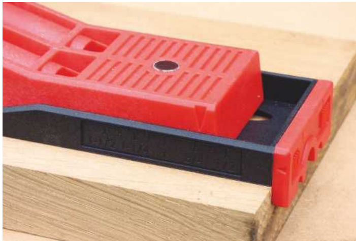
A 'V' symbol on the end stop indicates which side to use (they're slightly different) depending on the drilling task
