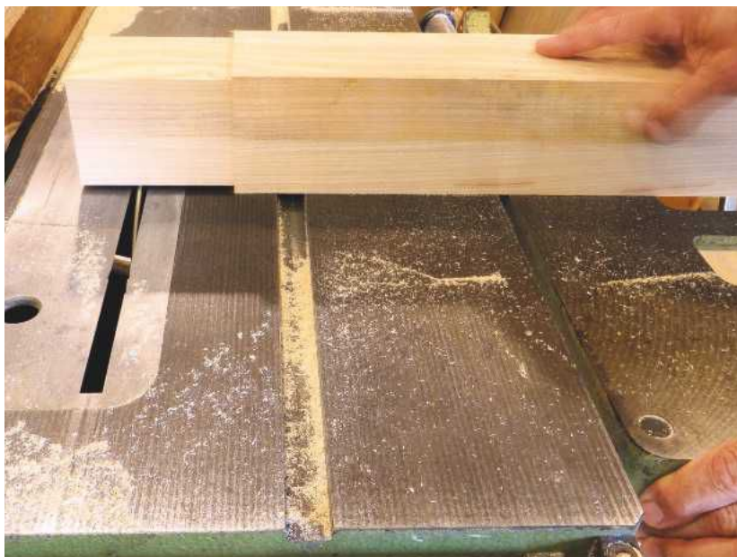
PIC 2. The shoulder is necessary to make the leg sit squarely and securely. No, it probably isn't conventional to cut it like this, sliding the timber across the saw blade, but how else would you effect this shallow step on the top of the legs? A router, perhaps, but this would be nowhere near as quick and efficient
