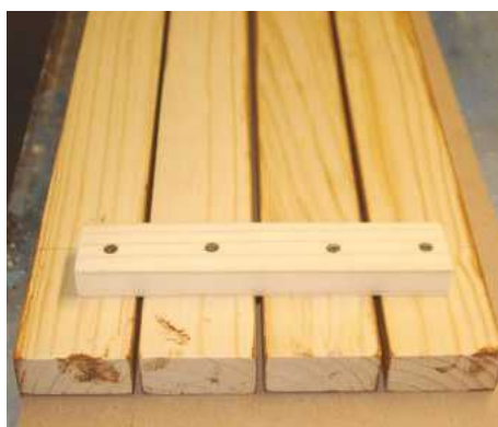
PIC 2. The slats that form the seat have 5mm spacers placed in between each slat
