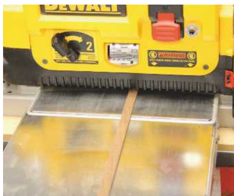
PIC 7. Put a long strip of walnut scrap through the planer several times to mill it down to the correct thickness
