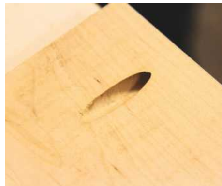
PIC 20. One of the completed pocket holes
