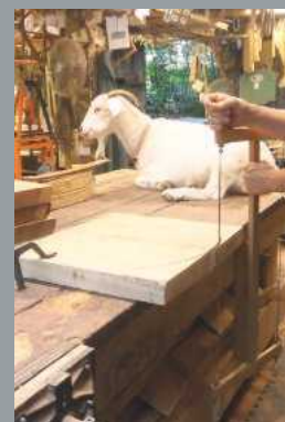
Frame sawing a seat out of 50mm curly maple
