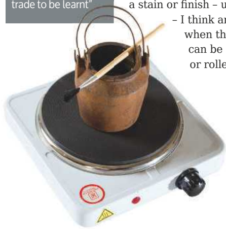
ABOVE: Cheap but effective: the inexpensive hot plate has enough oomph for warming glue; the cast-iron double-boiler has enough mass to avoid hot spots
