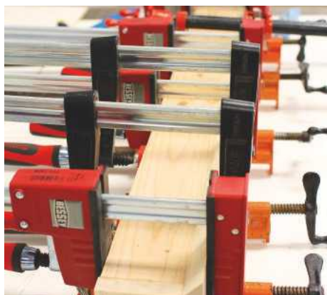
PIC 2. ... then glue, clamp or brad nail them into position
