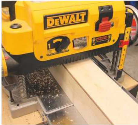
PIC 10. Plane the entire post in order to flatten everything out and make the inlay perfectly flush with the adjacent maple boards
