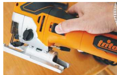
A side-mounted on/off slider on the left makes the saw better suited for right-handed users
