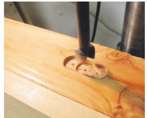
PIC 27. Load a Forstner bit into the drill press, set the depth so you don't remove too much material and drill holes to remove the wood inside the pencil line
