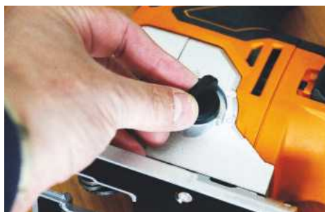
A three-stage pendulum controls the speed and finish of the cut and is also used for working different materials
