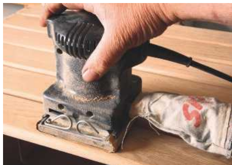
PIC 6. A little hand-held sander produces spiral tracks on the surface as the paper oscillates in a circular motion while the tool is swept across the surface
