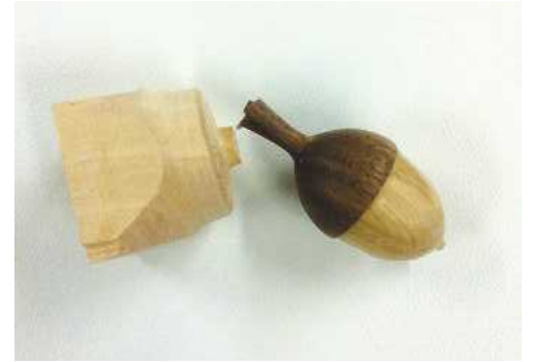
PIC 11. Remove the acorn from the spigot using a fine-bladed saw
