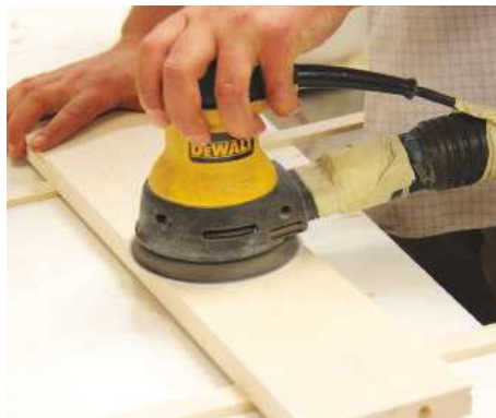
PIC 29. Now it's time to sand all surfaces with 120 followed by 220 grit discs mounted in a random orbital sander
