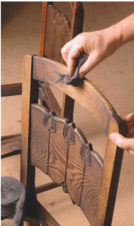
PIC 15. Steel wool rubbed in beeswax polish can be used to burnish a surface and to shade the colouring with a stained paste
