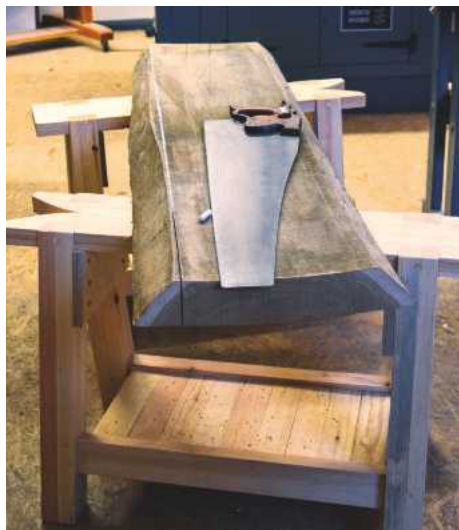
PIC 6. With a good saw and a couple of saw benches, hand ripping your stock doesn't have to be a pain
