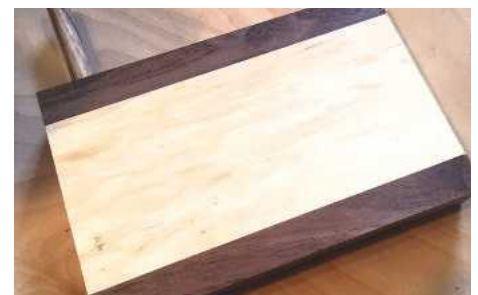
PIC 10. The camera body, once run through the joiner to ensure all the surfaces were smooth
