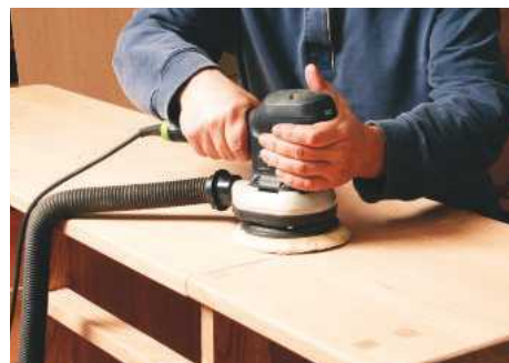
PIC 7. The random orbit sander also produces spiral tracks but each one is different from the last so that no pattern builds up and the effect is smoother
