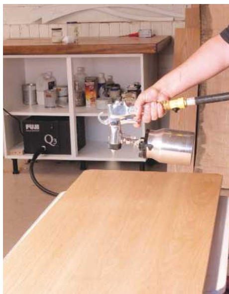
PIC 23. For spraying, water-based finishes are best applied with a high volume low pressure (HVLP) system, which provides an even coating with the relatively large water droplets
