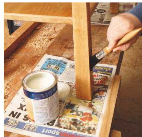
PIC 21. Water-borne varnishes use small amounts of solvent (low VOC) by suspending the varnish as a fine emulsion in water
