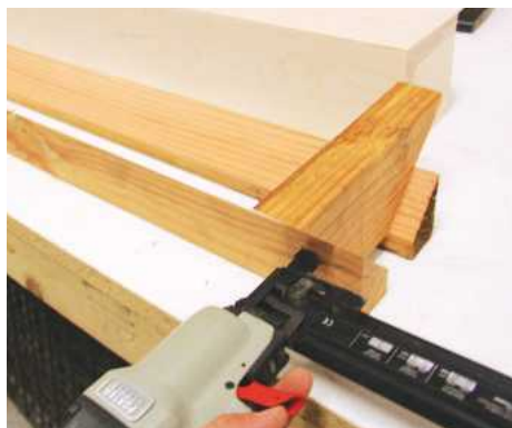
PIC 5. Use a brad gun to assemble the sled
