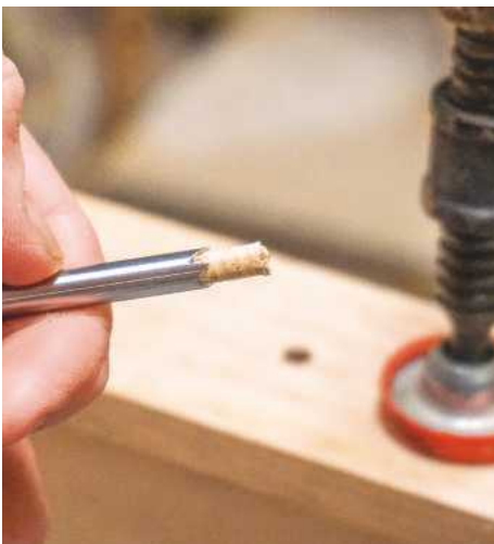
PIC 5. Removing the cylinder of wood with the embedded screw from the extractor
