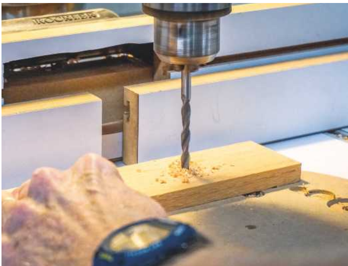
PIC 3. Preparing the guide with a 6mm hole
