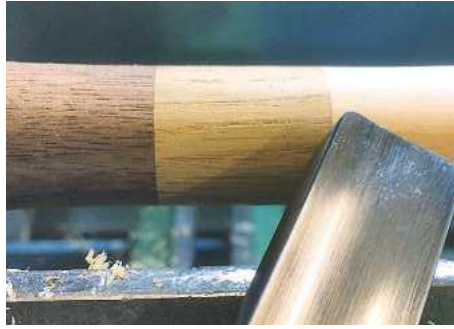
PIC 7. Begin to turn the glued-up blank to the round, using a suitable wide gouge
