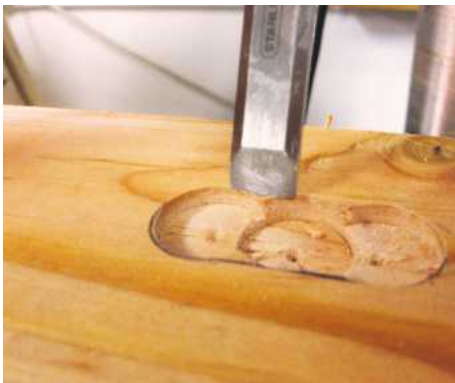
PIC 28. Clean up the hole using a chisel
