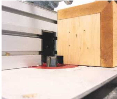
PIC 25. Using a straight \frac{1}{2} in or \frac{3}{4} in router bit, set the router fence and remove the back corner of the post, making several passes
