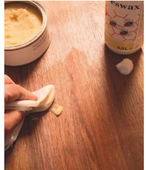
PIC 14. Smooth flat surfaces like this walnut can be treated with beeswax polish either in the form of a liquid emulsion (upper right) or a paste (upper left)
