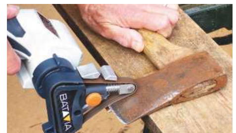
I tried the MaxxSharp on a small axe and it soon restored what was previously a pretty blunt tool
