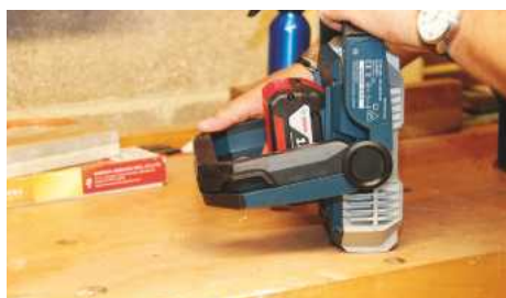
The light features a rotating stand, which allows the light to be fired in the direction required
