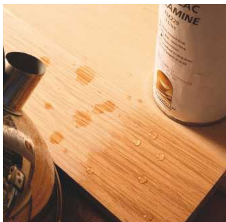
PIC 20. Synthetic lacquers such as melamine can briefly resist wetness or even boiling water as demonstrated on the bottom corner of this board
