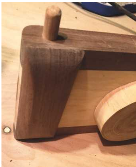
PIC 14. The grip added to the left-hand side of the camera body
