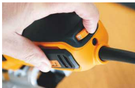
The variable-speed is controlled via the rear-positioned dial
