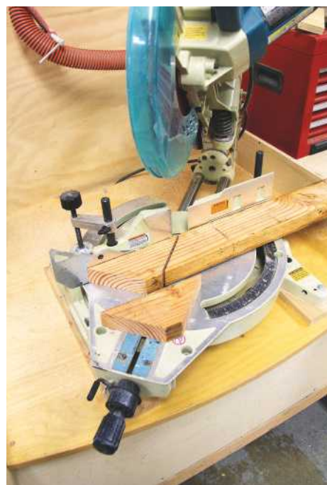
PIC 4. Use the chop saw to cut two triangular pieces of 50 × 100mm post with the saw set at 45° as before
