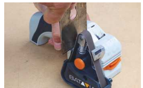
Although the angle is correct for grinding these there's actually not enough support for the blade as you move it across the belt
