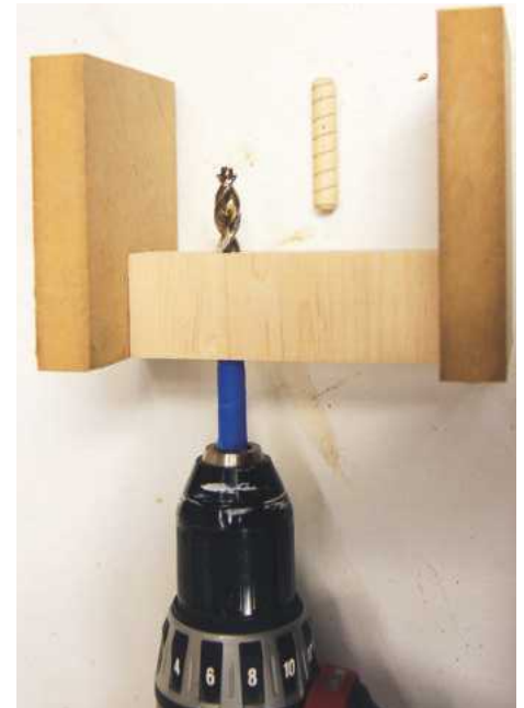
PIC 13. Mark the drill bit used to drill the holes for the wooden dowel pins with tape, to correctly show the depth to which it should be inserted into the jig
