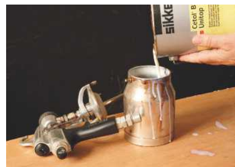
PIC 22. Spraying with water-based finishes is much less hazardous than traditional solvent-based spraying
