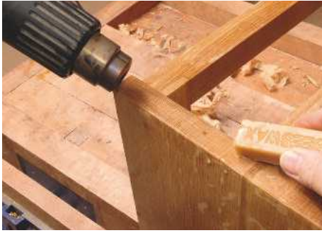
PIC 12. By warming the wood with a hot air blower the wax can be made to soak deep into end-grain and saturate between the wood fibres
