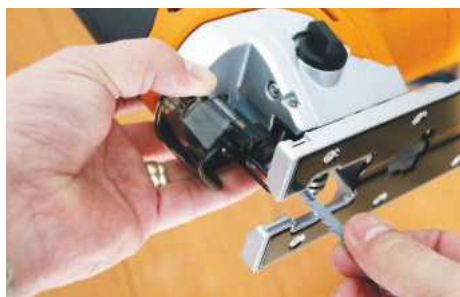
A plastic lever is used to release the blade clamp
