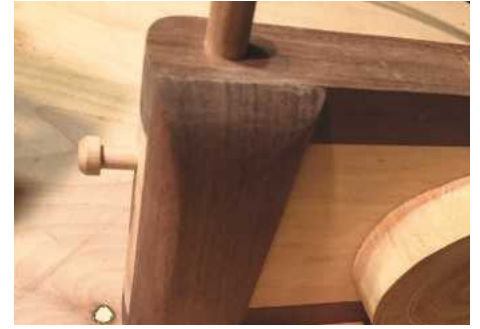
PIC 22. The hardwood peg in place, which the leather belt end will be placed onto
