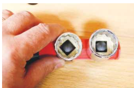
The socket on the right is secured; the one on the left can be removed
