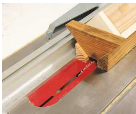
PIC 6. Push the corner post and sled through the table saw, cutting a 3mm wide inlay groove that runs vertically along the entire post ( PLEASE NOTE BLADE GUARD HAS BEEN REMOVED FOR CLARITY )
