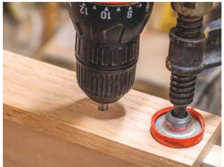
PIC 4. Drilling a cylinder around the screw
