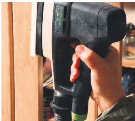
PIC 8. A linear sander is ideal for following the wood grain pattern, especially on edges
