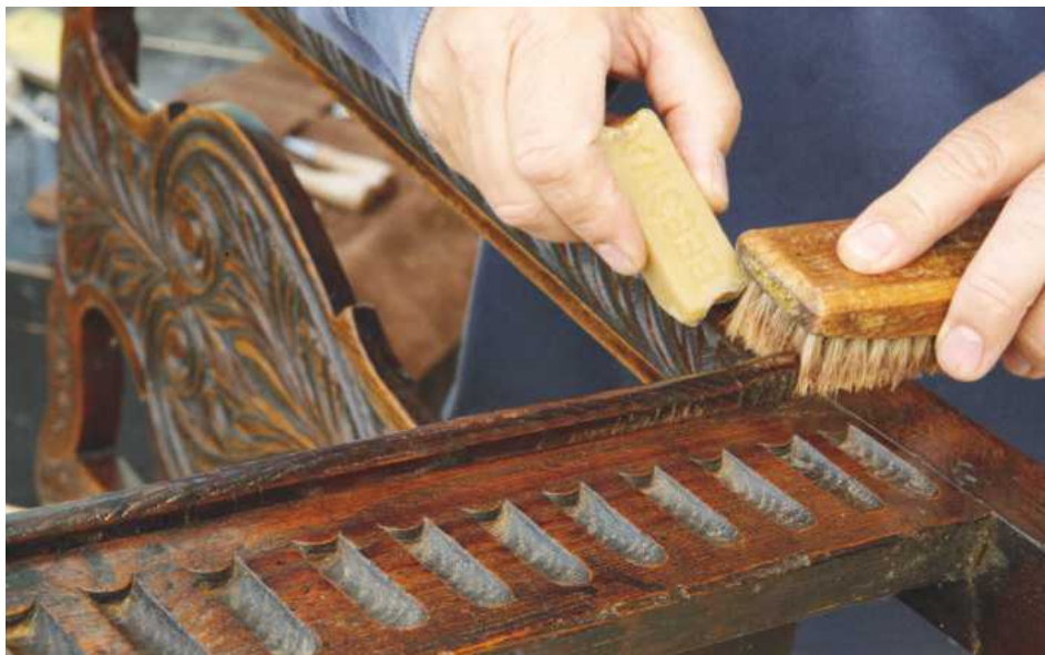
PIC 11. Pure beeswax can be rubbed onto coarse-grained and carved surfaces then worked in with a brush
