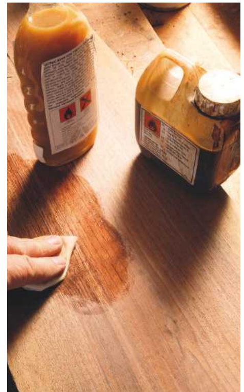
PIC 18. Ready-mixed shellac polish is supplied in a range of natural colours
