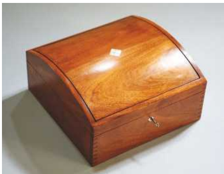
PIC 19. To prevent shellac taking too high a gloss it can be rubbed with waxed fine steel wool
