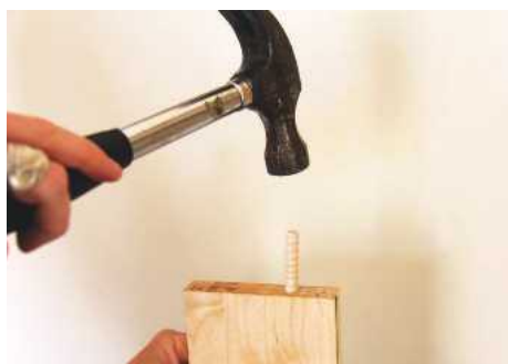
PIC 34. ... and lightly tap the shelf onto the corner post
