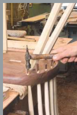
Wedging spindles and driving in walnut wedges
