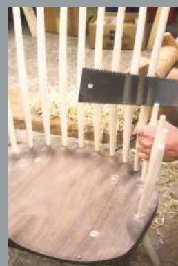
Cutting the kerf for wedges
