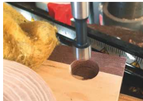
PIC 13. Drilling the hole for the viewer using a drill press fitted with a Forstner bit
