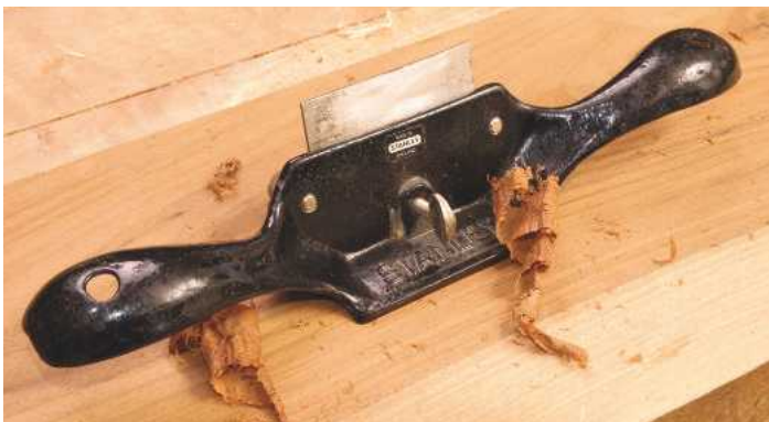
PIC 3. One of the most basic tools for flattening a wooden surface is the scraper blade, here mounted in a cast handle to take strain off the thumb
