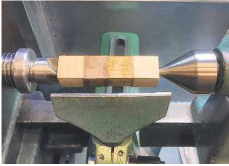
PIC 6. The cube structure, mounted between centres
