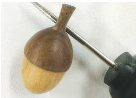
PIC 12. Mark the location of the hole using a bradawl
