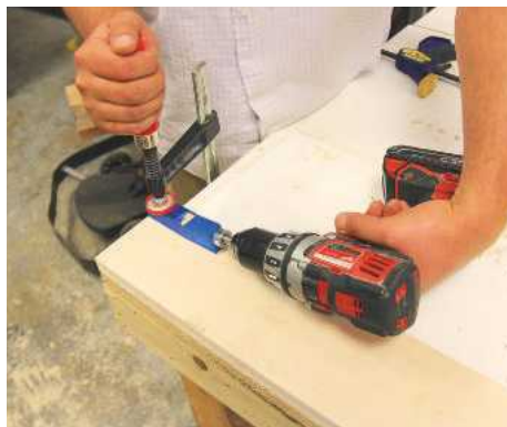
PIC 19. Drill one pocket hole in the end of each shelf
