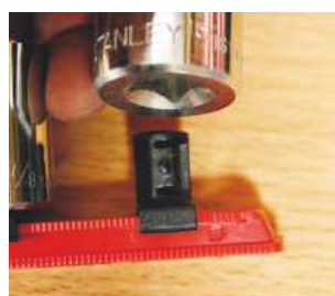
The rails feature a toothed profile, which allows the pegs to be held firmly in place
