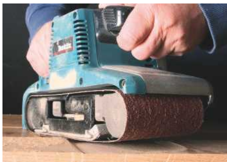
PIC 5. Although the belt sander is fast and powerful for removing wood, it is not widely used by fine furniture makers
