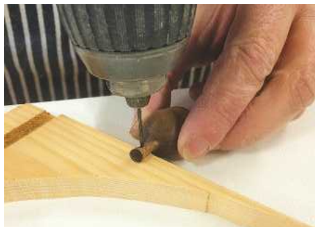
PIC 13. Drill the hole with a 1.5mm drill bit fitted in an electric drill
