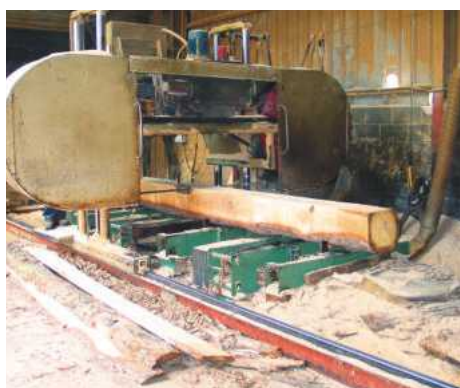
A horizontal band mill, with some slab wood in the front
