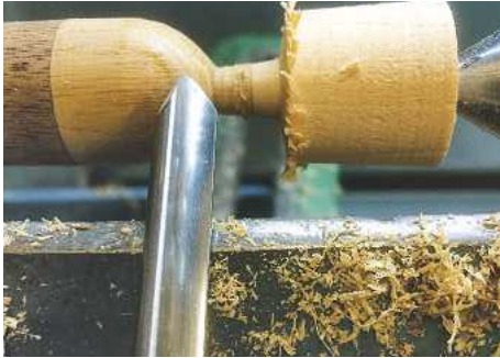
PIC 9. Start to create the desired shape, using a fingernail profile gouge
