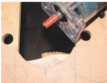
PIC 6. Template and yew clamped to workbench – note the pattern bit mounted in the router
