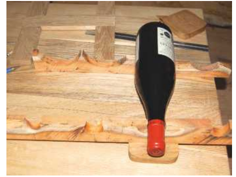
PIC 21. The rear member needs to be marginally higher than the front to ensure the bottle is level
