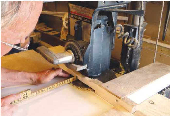
STEP 9. Now for the tenons. I have slung my radial arm saw over so that the blade is parallel to the table. It holds the coarsest blade because no blade likes cutting into end-grain, and this does it best, albeit with considerable noise. I move the saw in and out to set the depth of cut. The thickness of the tenon is controlled by the rise and fall of the saw and should be trialled so that it is a snug/easy fit into the mortise
