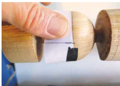
PIC 9. A strip of paper is used for measuring the circumference of a turned ball
