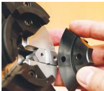
The jaws are located on a raised ridge and are secured with two set screws
