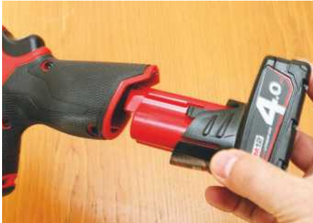
Batteries slide into the handle, which makes the grip slightly large
