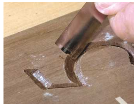
PIC 34. Change the angle of your chisel to do a final clean-up, in order to achieve smooth curves and edges
