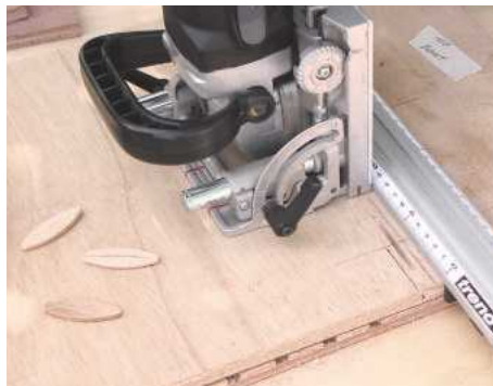
STEP 8. Cut slots in panels for No.0 biscuits, making sure you check the settings on plywood offcuts first
