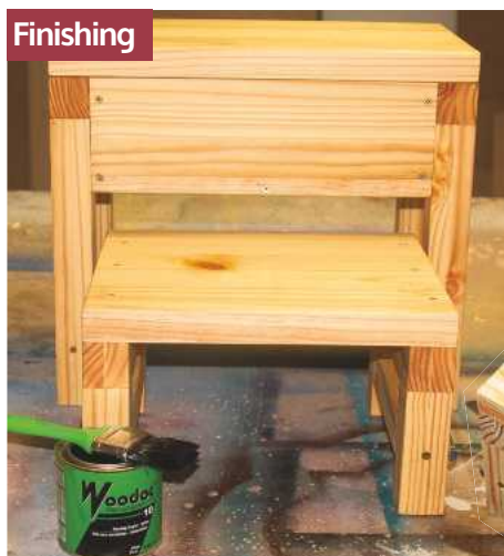
STEP 15. Apply wood sealer or varnish in accordance with the manufacturer's guidelines. I applied a clear sealer, but you can choose to tint the step stool in any colour you wish
