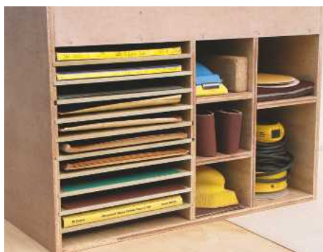
STEP 23. There's plenty of space for a random orbit sander as well as belts, discs, pads and sheets
