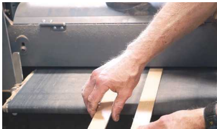
PIC 10. Running the cherry strips through the drum sander in order to get them to their final thickness
