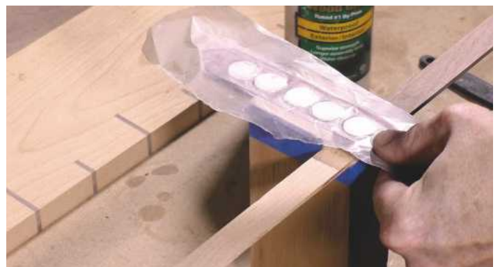
PIC 19. Gluing the horizontal bar into the other dado using regular wood glue
