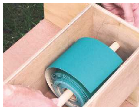
STEP 18. Pass the dowel through an abrasive roll and into the end holes. Check that the roll rotates
