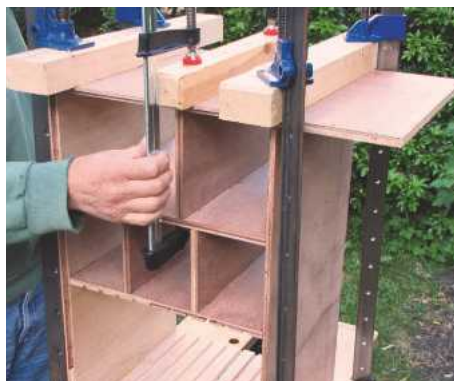
STEP 11. Use cauls to spread the pressure when clamping up the side panels, then check for square
