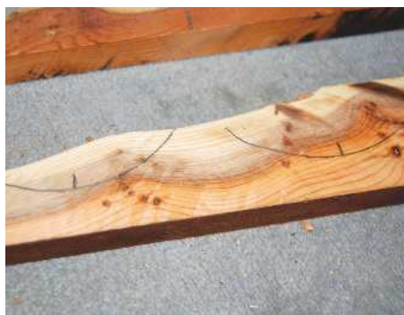
PIC 7. Marking out the segment
