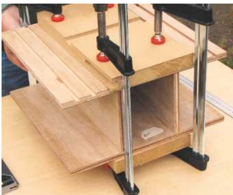
STEP 10. Assemble the box in two stages. This frees up clamps and it's easier to maintain square joints
