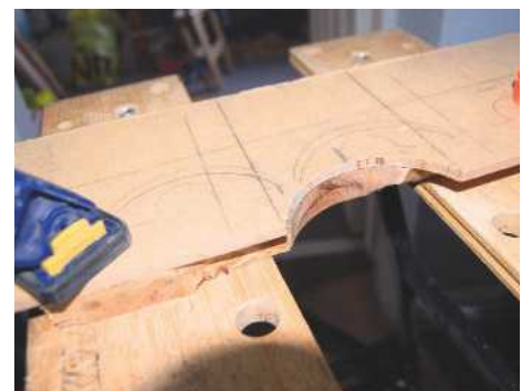
PIC 8. MDF template clamped ready for routing
