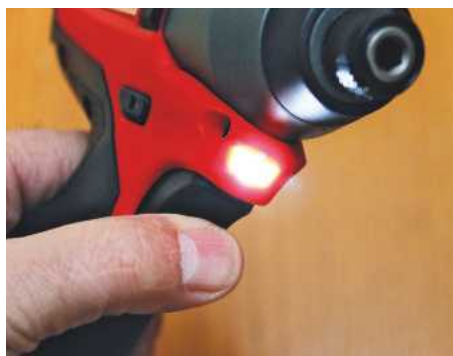
Likewise, they both have a trigger-operated LED worklight
