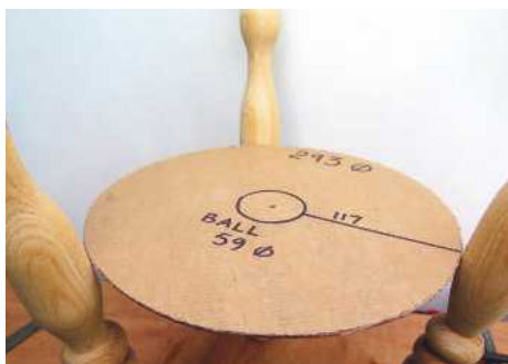
PIC 8. The circle gives a rough idea of stretcher lengths
