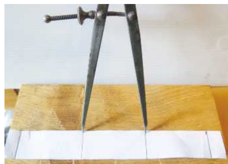
PIC 10. Dividing the circumference by three using a pair of callipers
