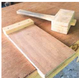
PIC 1. Hand-made mallet and bench hook, made using scrap materials
