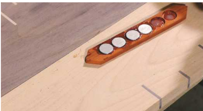
PIC 18. Epoxy was used to glue the magnets into the padauk strip
