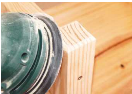
STEP 9. Sand all uneven edges with 120 grit abrasive and then sand smooth with 180 grit sanding pads. Wipe clean with a cloth lightly dampened with mineral turpentine. Use your orbital sander to give a chamfered (angled) edge around the bottom of the legs; this gives a nice finishing touch
