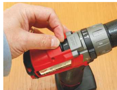
A top-mounted slider changes gears on the drill
