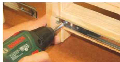
STEP 11. Place the small step stool underneath the large one and pull out the runners so you're able to secure to the leg rail of the small stool. Drive in two screws at the front end of the runner. Separate the runner from the track and drive two screws at the back end. You can then slot the runners back together
