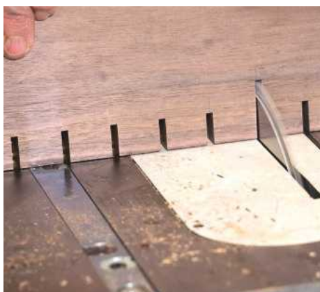
PIC 8. Cutting slots into the walnut
