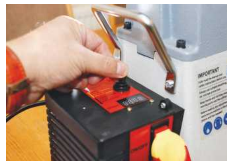
This switch also allows you to put the lathe into reverse for sanding
