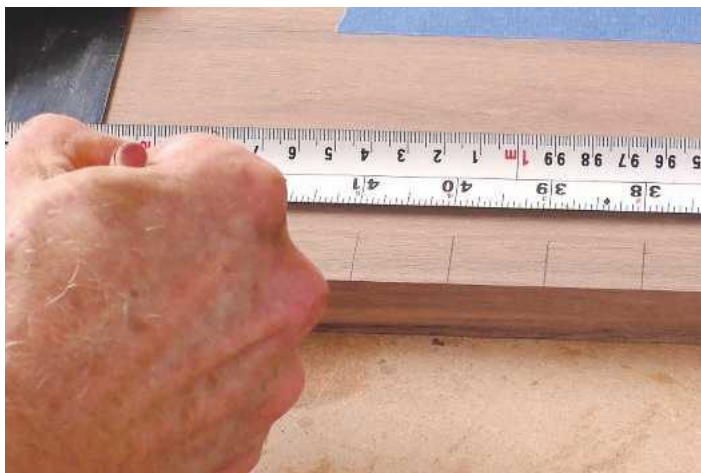
PIC 6. I marked an increment at every inch on the imperial side, and every 5cm on the metric side
