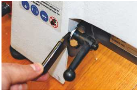
This simple two lever combination allows you to release the motor to make belt swaps
