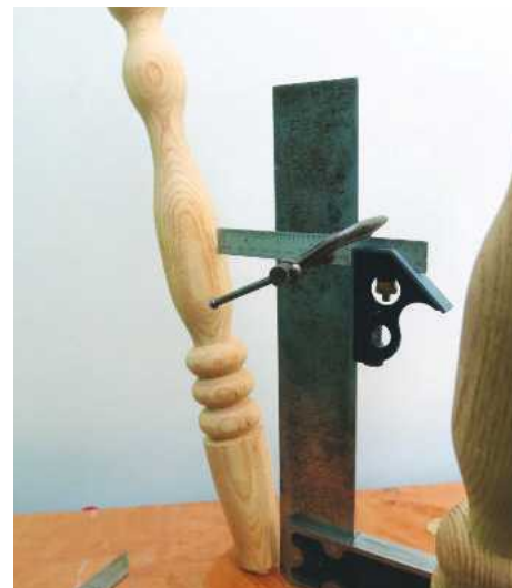
PIC 7. My setup for marking positions of the leg stretchers
