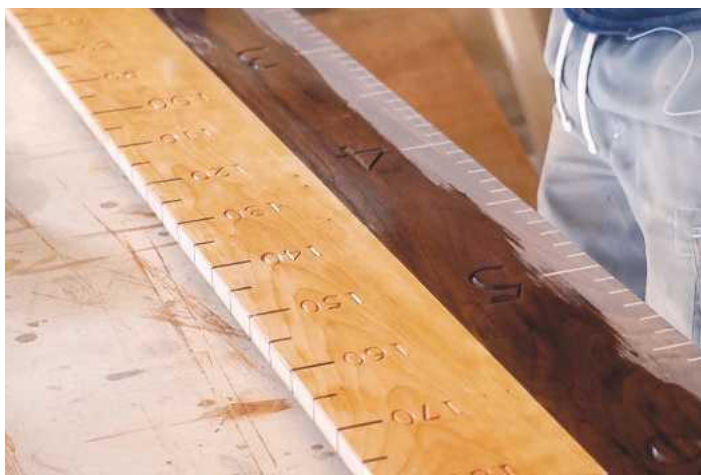
PIC 37. Applying a single coat of shellac to seal the wood
