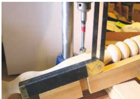
PIC 11. 15mm Forstner bit in the angled cradle jig
