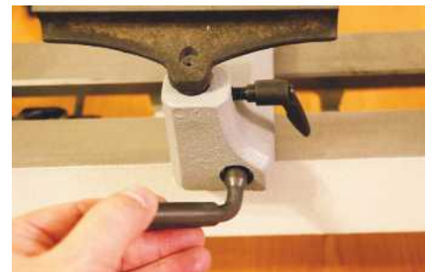
The banjo is held with a similar lever and holds firmly
