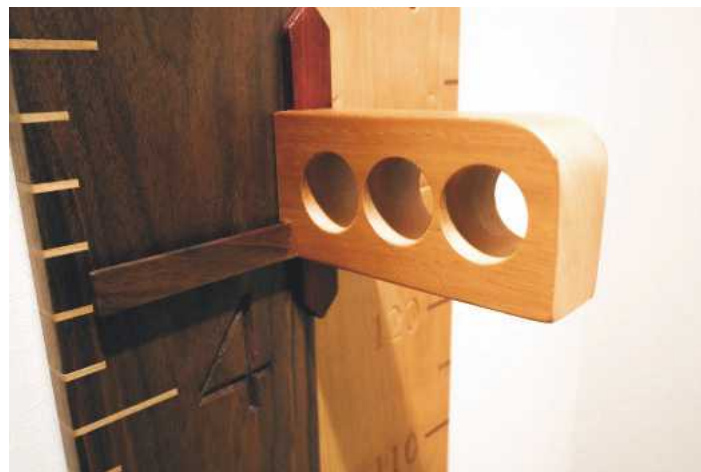
PIC 41. As a design modification, holes were drilled in the slider to reduce its weight
