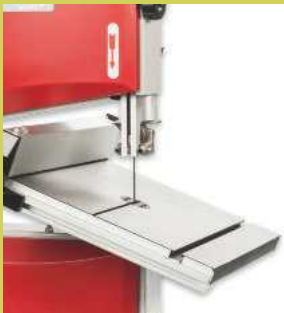
The cast-iron table tilts from 0-45°
