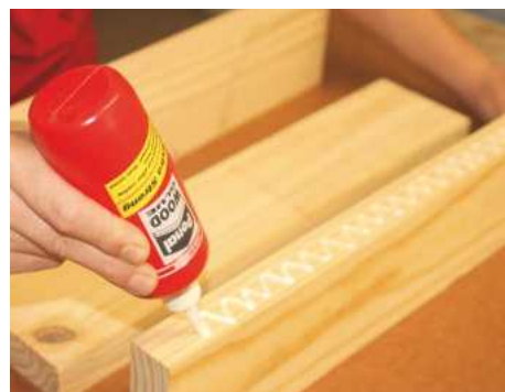
STEP 5. For both the small and large step stool, glue together the slats that form the tops/lid
