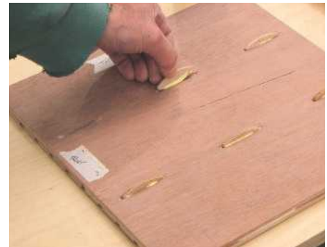
STEP 9. Work out an efficient clamping sequence, then glue components together with PVA glue
