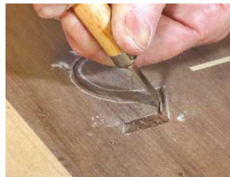
PIC 31. Using a straight chisel, approach the centreline at a 45° angle
