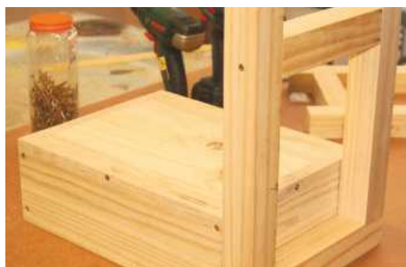
STEP 7. Turn the stool over to drive 60mm screws through the top and into the leg assembly on both sides
