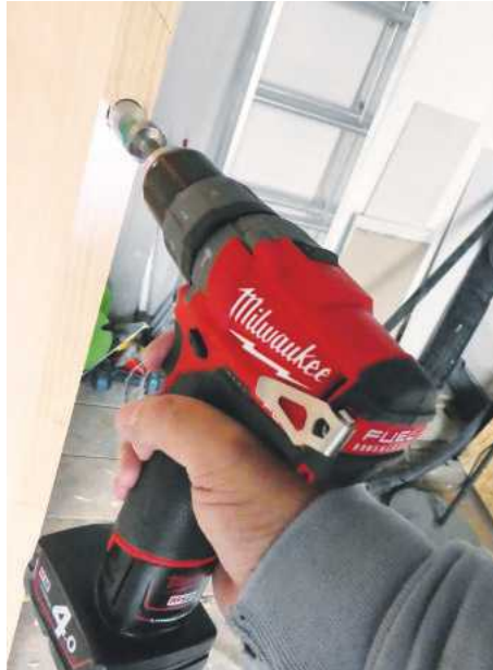
Drilling out oak with a 25mm auger was well within the drill's capabilities
