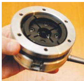
A faceplate ring is supplied, which traps with the jaws
