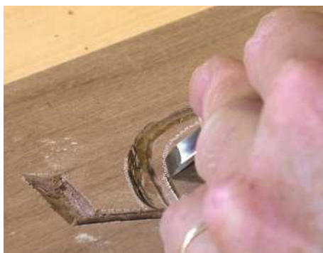
PIC 33. On the convex side of the curve, switch to a straight chisel and carefully cut inwards in small steps to create a smooth curve
