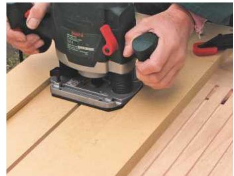
STEP 6. Cramp the jig to the ply and line up the pencil marks. Rout the grooves to a depth of 25mm
