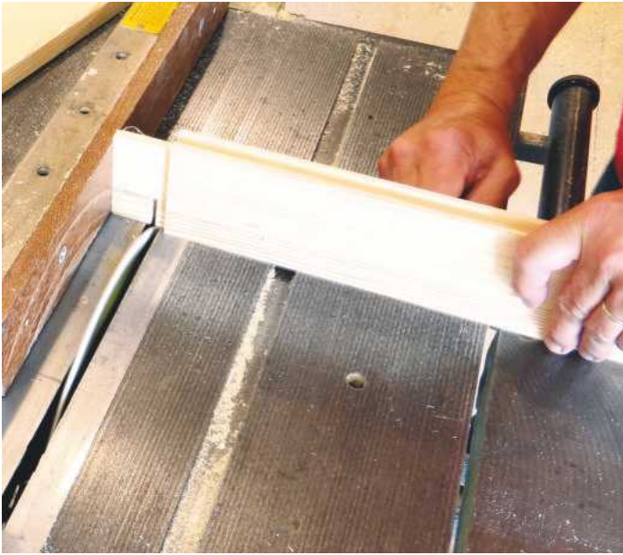
STEP 13. The tenon is haunched so as to leave a little piece to fill the groove in the stile. A radial arm saw would also accomplish this
