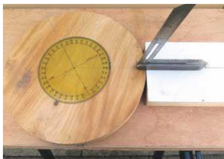
PIC 5. Marking out leg positions using a protractor
