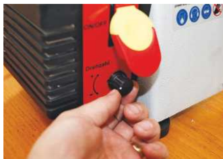
Variable-speed is very easy to control with this dial and digital readout
