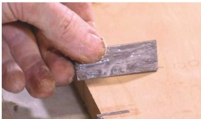
PIC 11. Gluing the inserts into place
