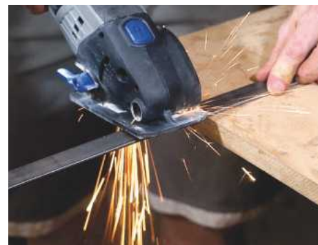
PIC 23. Cutting the steel bar to length so that it was just slightly shorter than the growth chart
