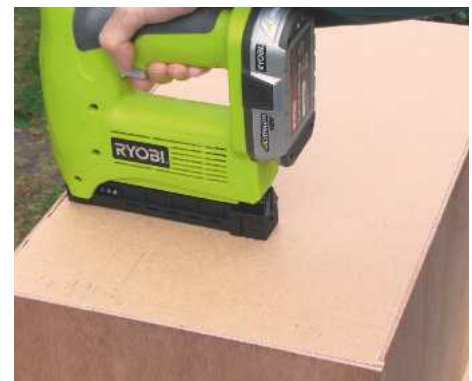
STEP 12. Trim the MDF back panel to size and attach with a nail gun, or simply pin and glue in place
