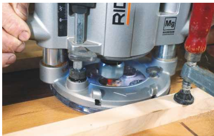
PIC 36. Using a router to cut a keyhole slot so that the growth chart can be hung on the wall
