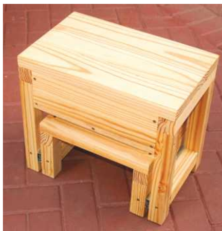
STEP 1. Arrange the pieces for the storage compartment and assemble using wood glue and 40mm screws
