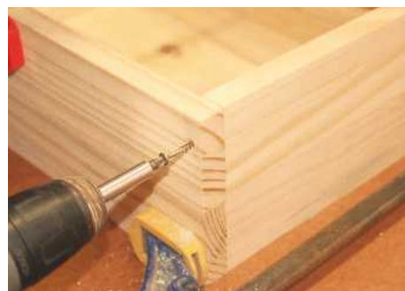
STEP 2. To assemble the small step stool, drill 3mm countersunk pilot holes through the side rail and into the legs, then join with wood glue and 60mm screws
