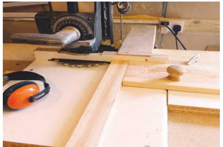
STEP 10. The first time I used this arrangement, I was a little wary. It looks dangerous, but it isn't. I've used it hundreds of times without the merest suggestion of a problem. The board with the knob on is to push the component with my right hand. My left hand holds the component to it, and to the melamine fence. It takes seconds to cut a perfect cheek. To ensure your safety, a guard should always be fitted over the blade, but here, I needed to see what was going on
