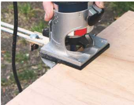
STEP 7. Rout a 7mm rebate around the rear edges of panels for the MDF back panel
