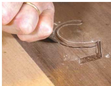
PIC 32. When you reach a curve, switch to a curved chisel on the concave side
