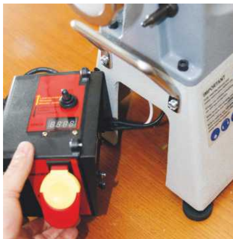
The switch box is hinged, which allows you to gain access to the bottom pulley for belt swaps
