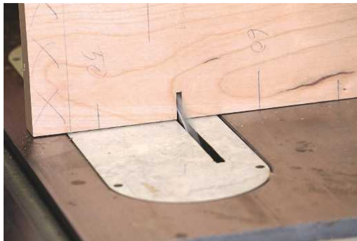
PIC 7. Cutting slots into the board at each increment mark. I cut these so that I could insert strips of contrasting wood to mark each of the increments
