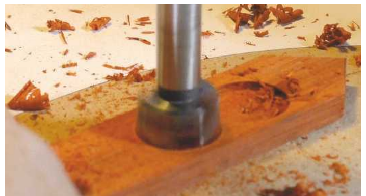
PIC 17. Drilling the recesses for the rare earth magnets, using a Forstner bit
