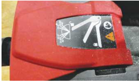
Features such as this large paddle for compound cuts are great for easy adjustment
