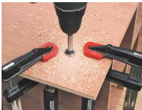
STEP 13. Mark 20mm dowel centres and bore end panels with a Forstner bit. Clamp an offcut to stop breakout occurring
