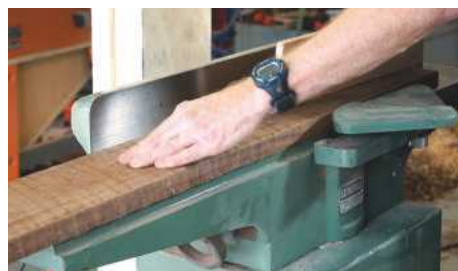
PIC 1. I started by jointing the walnut and cherry boards to create a flat face and a flat edge...
