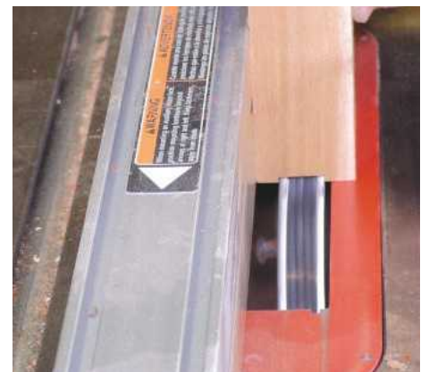
> PIC 15. Cutting the dado in the head piece
