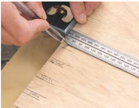
STEP 4. Carefully mark the positions of sliding trays. Space them equally apart by about 25mm
