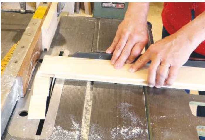
STEP 11. The sides are cut away from the cheeks. The secondary fence is to stand the workpiece off the saw fence so that the waste pieces won't get trapped between it and the blade. Perversely, this simple cut is more dangerous than the previous procedure because occasionally one of these waste pieces will get moved by the wind surrounding the saw; touch the blade and be whipped off the table at speed. As with all saws, keep hands well back!
