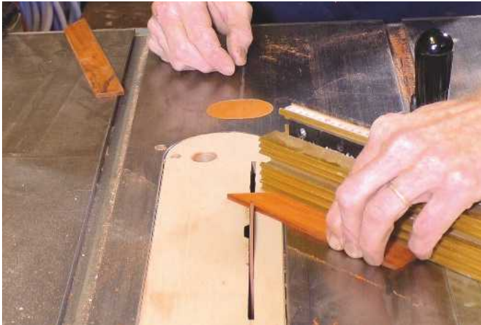
PIC 13. ... before cutting a 45° mitre to create a point on each end (PLEASE NOTE BLADE GUARD HAS BEEN REMOVED FOR CLARITY)
