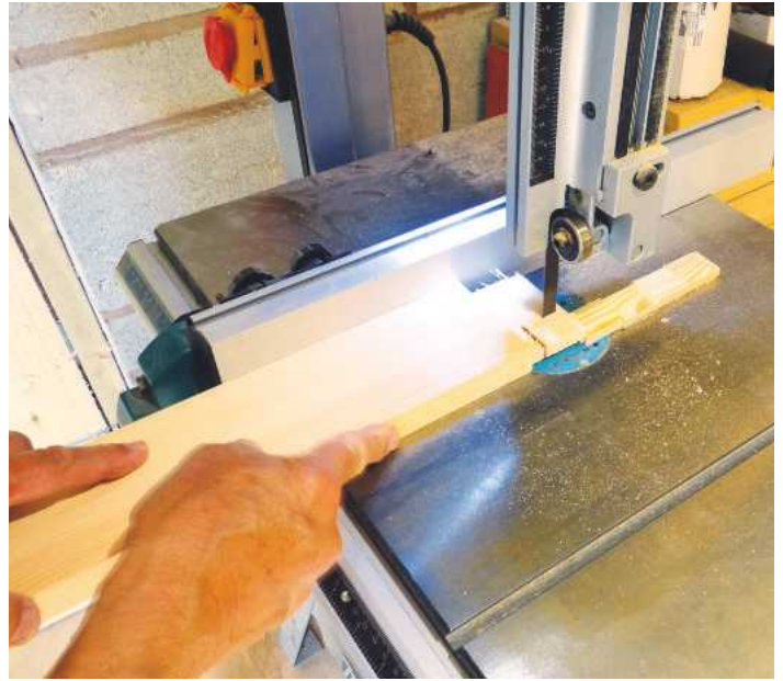
STEP 14. The haunch completed. Note that the waste is allowed to fall free on the right rather than becoming trapped between blade and fence
