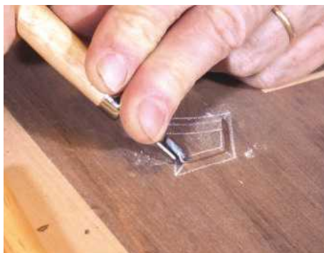
PIC 30. Using the V-parting chisel in the opposite direction along the angle guide
