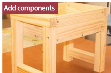
STEP 8. For the large stool, with the storage compartment upside down, glue the leg assemblies onto the side of the compartment. Pre-drill countersunk holes through the leg assembly, into the compartment, and secure with 60mm screws
