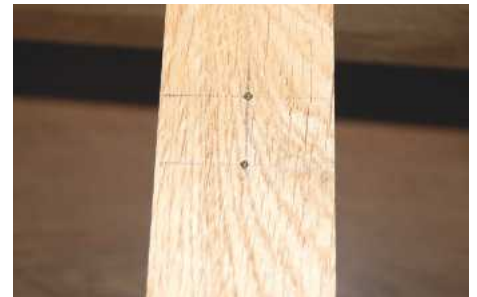
PIC 22. Drill positions are carefully marked using a bradawl
