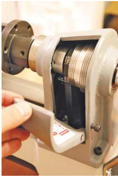
Access to the top pulley is via this hinged flap on the casing
