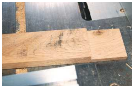
PIC 14. Top joint ready for trimming
