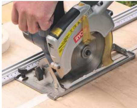
STEP 2. Cut the ply to size. A strip of masking tape along the cutting line helps to reduce splintering across the grain
