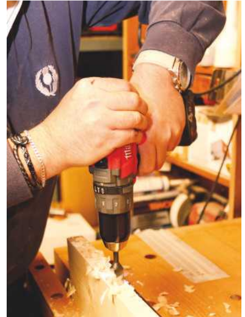
On its fastest speed it runs a 19mm auger in pine without a problem
