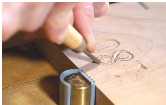
PIC 35. When carving the smaller digits, you'll need to use a much smaller curved chisel
