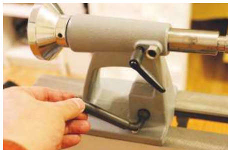
You lock the tailstock with this handle, which is positioned at the rear
