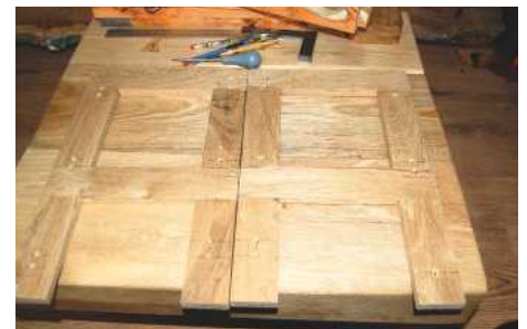
PIC 23. The side panels, pre-drilled and countersunk
