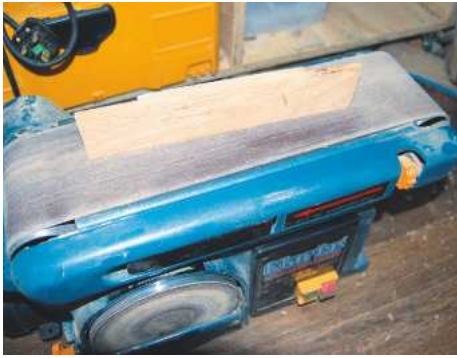
PIC 19. Sanding the internal edges
