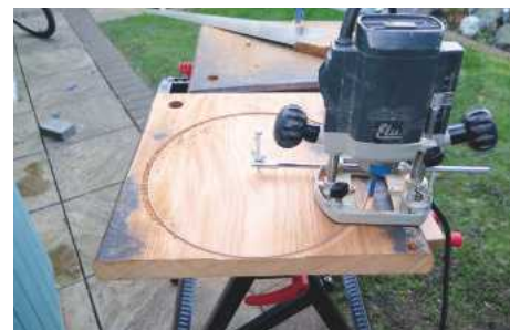
PIC 3. Using the router to create a circular top
