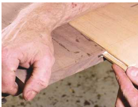
PIC 24. Inserting a small piece of the leftover strip to plug each end of the growth chart so that the steel bar won't slide out
