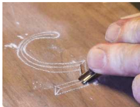
PIC 29. Starting with a V-parting chisel, cut along the centreline
