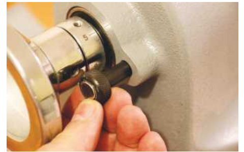
A neat magnetic tapered pin holds the indexes when needed
