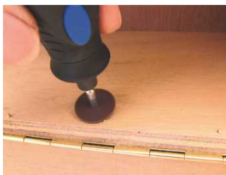
STEP 16. Using a Dremel tool or similar, cut off the ends of the protruding hinge fixing screws
