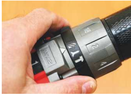
There's also a second collar that overrides it for drilling functions
