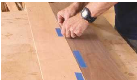
PIC 3. Marking the two jointed edges with tape so that I wouldn't lose track of which edges to glue
