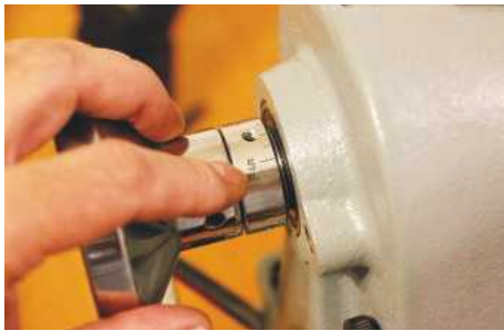
The indexing positions are replicated on the outer collar
