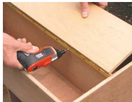
STEP 15. Supporting the lid, carefully mark and drill screw pilot holes. Screw the lid to the divider panel
