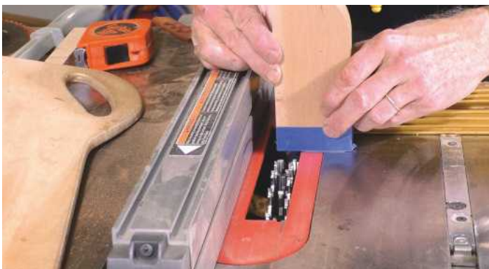
PIC 16. Cutting the dado for the horizontal bar – note tape added to the cedar, which helps to prevent tear-out when cutting the dados (PLEASE NOTE BLADE GUARD HAS BEEN REMOVED FOR CLARITY)
