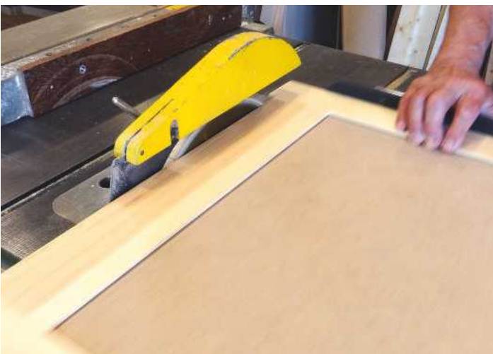
STEP 17. Finally, trim off the horns, finishing with a plane if necessary...
