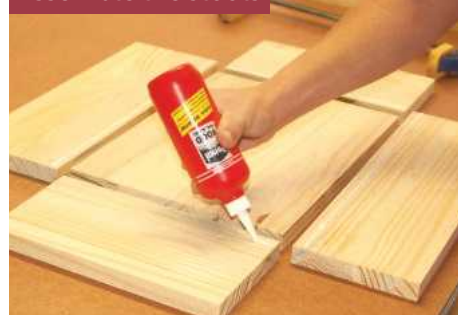
STEP 1. Arrange the pieces for the storage compartment and assemble using wood glue and 40mm screws
