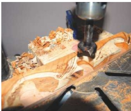
PIC 4. Cutting the part-circles on the drill press with the back of the yew referenced with a makeshift fence
