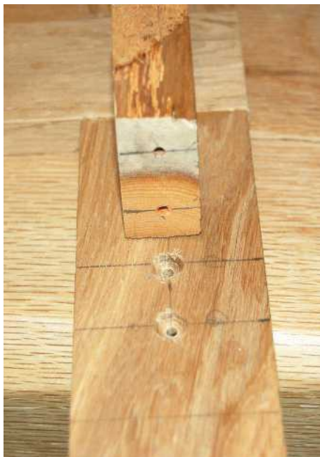
PIC 26. Matched holes are pre-bored on the side panel and horizontal members
