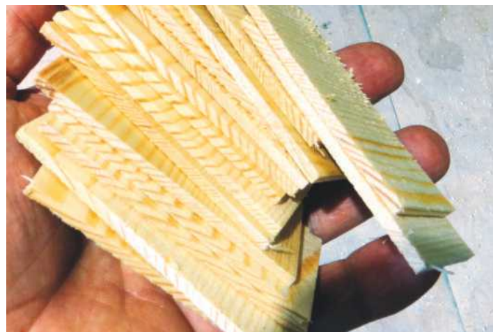
STEP 12. See how even these pieces of cheek waste are. It really is an efficient system. Before this I'd nibble the waste away face down on the table saw. This would leave a rippled surface, which I'd smooth off by moving it across the blade at right angles. It worked, but took very much longer and did not give such a uniform result. Again, a router could be set up in a jig to cut the cheeks. A well-tuned bandsaw would also work
