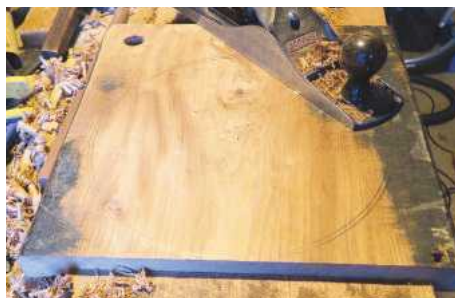
PIC 2. Flattening one half of the plank
