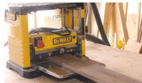
PIC 2. ... then I ran the wood through the thicknesser to ensure they would both be the same thickness
