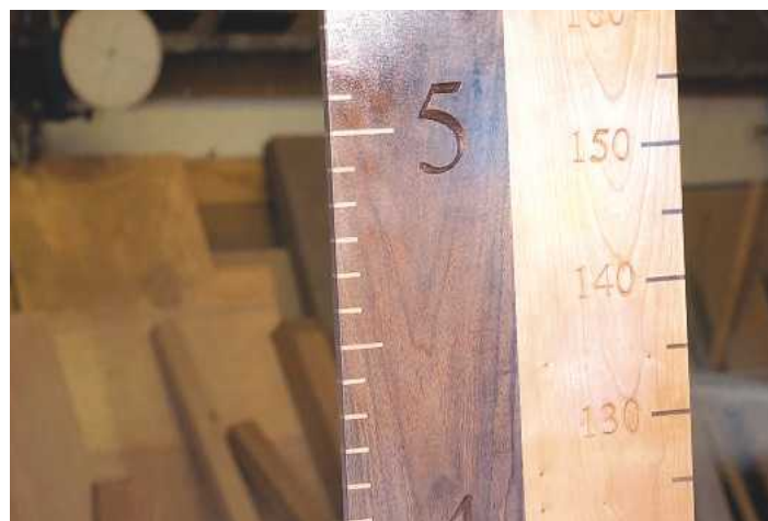
PIC 38. Spray on several coats of lacquer to give a satin finish
