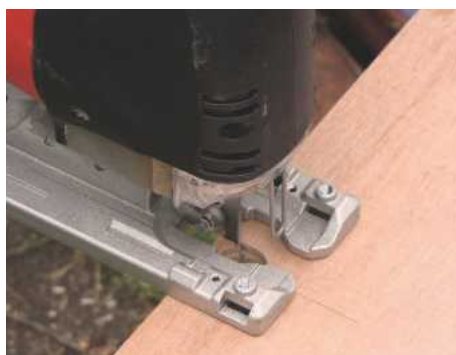
STEP 17. Drill a 20mm access hole in the centre of the front panel, removing waste using a jigsaw
