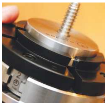
There is also a screw chuck that is secured with the chuck
