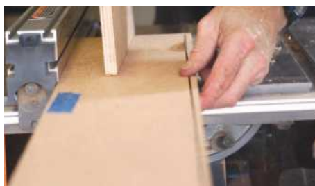
PIC 4. Ripping the walnut and cherry boards to their final width
