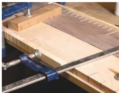
PIC 25. The boards are clamped up, making sure they remain absolutely flat
