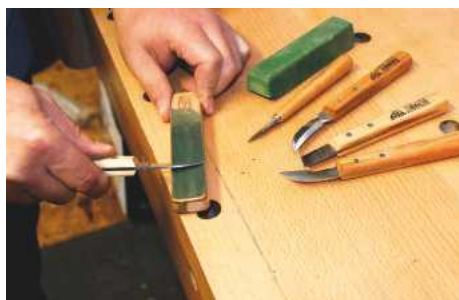
The knives benefit from a hone prior to use, and a strop keeps them cutting well as you work
