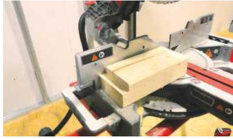
The mitre saw is easily capable of cutting through this 150 x 75mm softwood
