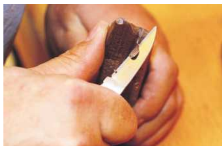
Some cuts are made by pulling towards bare flesh, so care is needed
