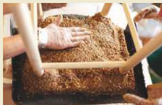
Applying thin layers of the material onto a mould for one of the chairs, which is exactly the same process as for the stool
