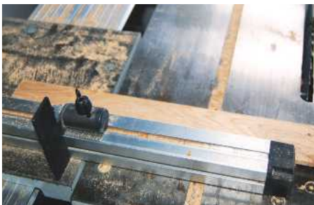
PIC 13. Using a sliding table attachment to make cuts
