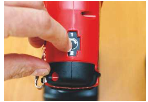
The impact driver has a toggle switch for changing speed and torque
