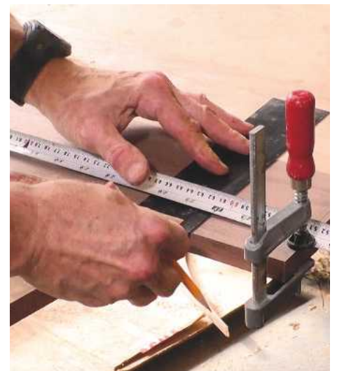
PIC 5. Aligning the two boards on the assembly table prior to marking the increments for the metric and imperial sides
