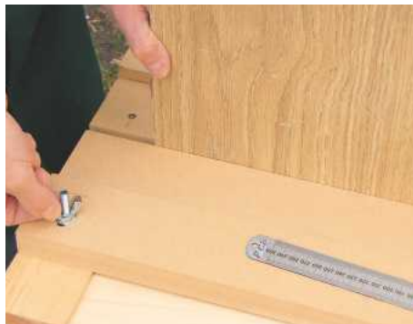
STEP 5. For routing a number of grooves the easiest method is to use a housing jig. Adjust this to suit the thickness of the tray
