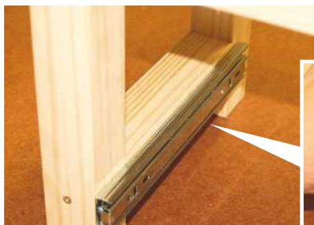
STEP 10. Secure the 250mm drawer runners to the leg rail on the large stool using 16mm screws
