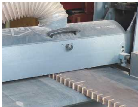
PIC 21. Running the growth chart boards through the drum sander to remove the excess from the inserts that had been glued into each increment mark
