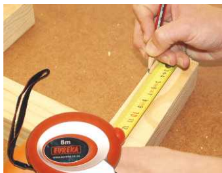
STEP 4. Measure up 41.5mm on the legs – for both the small and large step stool – and use this as a guide for mounting the leg rail
