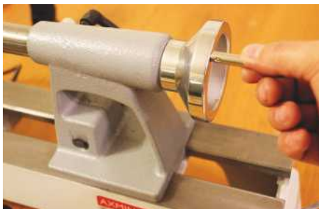
The tailstock quill adjustment is very smooth
