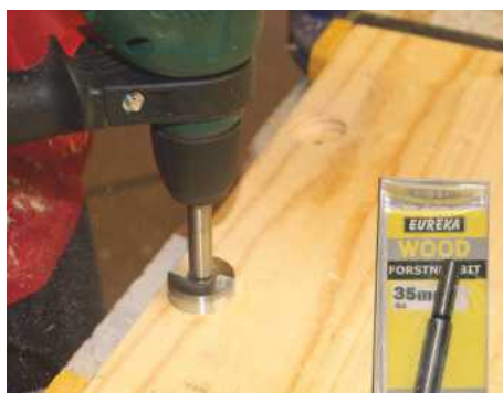
STEP 12. Draw a line 3mm in from the back edge of the slat top and drill two holes for the concealed hinge with a 35mm Forstner bit. Drill to a depth of 11mm
