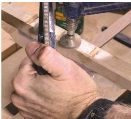
PIC 20. A piece of wax paper is applied on top of the magnets prior to clamping up
