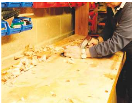
I had to flatten the top back as the leak in the roof had distorted my bench
