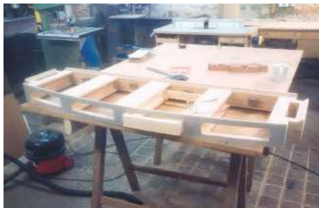
All the layers of the stack laminate construction have been veneered on their vertical faces. The drawers are fitted before the top and bottom of the carcass are bonded to the core
