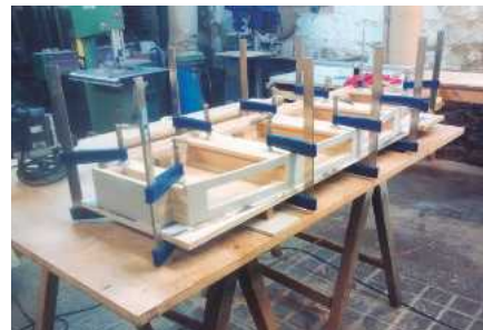
Here you can see the bottom of the table being bonded to the carcass
