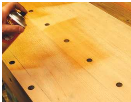
After cutting back between coats the lacquer is applied in the same way
