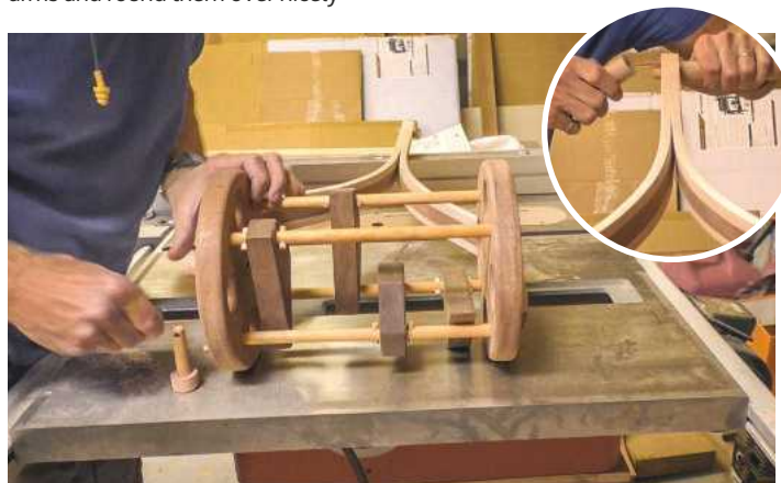
STEP 25. Now attach the arms to the wheels by inserting the little axles through each arm, then attach the handles at the other end. I attached the handles by inserting a 12mm dowel into the end of the handle, and putting the 12mm dowel through the end of the arm. In the inset photo, you can see a close-up showing how the pins are inserted into the 12mm dowel to hold things in place
