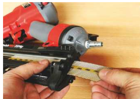
Fixings for the 15-gauge are loaded from the back of the magazine
