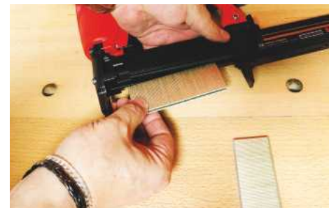
The stapler features a bottom loading magazine...
