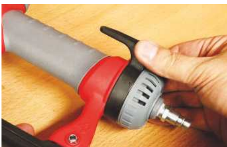
All three guns feature a rotating belt hook
