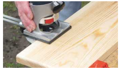
STEP 24. To soften the upper edges of the lid and fixed piece, rout with a bearing-guided round-over bit
