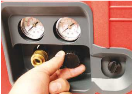
... while this one regulates the output pressure
