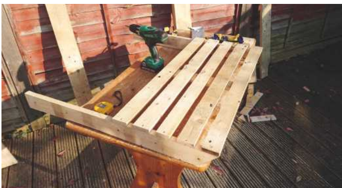
PIC 10. As the bottom shelf weighs a lot less than the top, I used the thinner planks as slats
