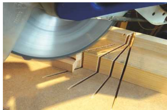
PIC 5. To achieve a clean cut, the workpiece must be held against a solid fence. I fitted the saw with a secondary fence standing some way out from the metal original so that the head could be swivelled round to cut at 45°, 30°, 15° and square without the cuts in the fence being so close that they'd destroy it. In this photo a little stop is added so that the 'foot' components can be chamfered identically
