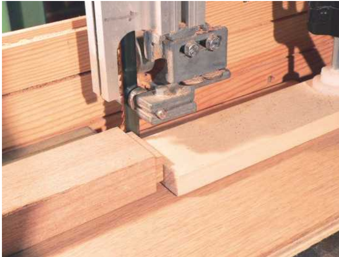
PIC 6. Cutting a tenon on the bandsaw with a guide and stop
