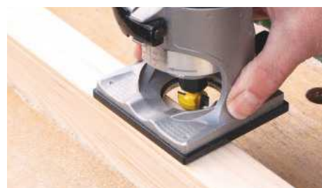
STEP 19. The lower edges of both rails feature a decorative bead. Use a bearing-guided router bit for this
