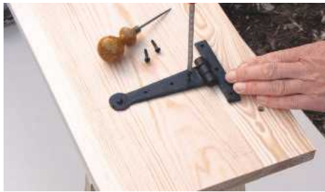
STEP 25. Position hinges and carefully mark screw holes with a bradawl. Fix in place and check that the lid opens smoothly
