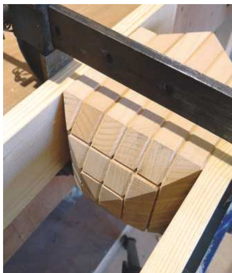
PIC 11. Emergency cramping was required! As long as not too much has gone wrong, it can be remedied while the glue is still soft, but set enough to keep the well-behaved pieces in place
