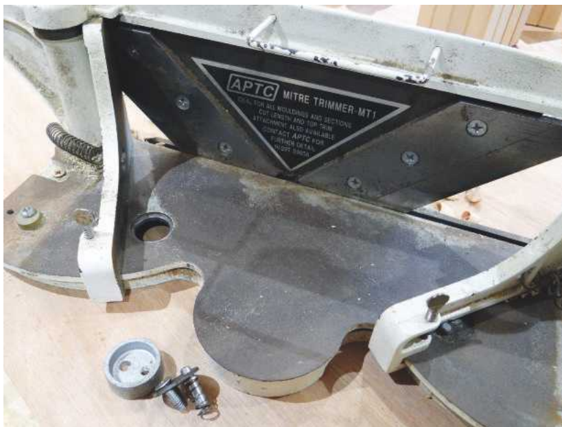
PIC 3. The cut from my chop saw, even with a fine blade, is not smooth enough, so important faces were trimmed on a guillotine. I already had a mitre trimmer when I saw this, the same model, rusty in the rain and missing its handle, at our recycling centre. I liberated it for £10. This allowed me the luxury of four angles permanently set up. A jig of any description should stay set up for the duration. Resetting only spells trouble. I removed the stop; it's useful for 45° cuts but gets in the way of 30°s
