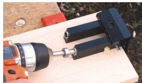
STEP 16. You can reinforce the joints between base and legs with central pocket-hole screws
