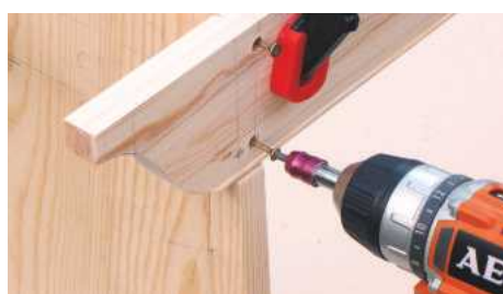
STEP 20. Drill and counterbore the rails, then glue and screw them into the notches at the top of both legs
