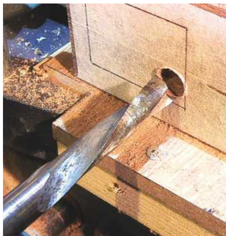
PIC 4. Cutting a mortise on the slot mortiser
