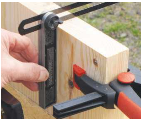
STEP 5. Cramp the legs together, secure in vice jaws and plane the ends. Check the angle with the bevel
