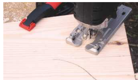
STEP 13. Saw the outline with a jigsaw fitted with a sharp blade. Reduce pendulum action for a clean cut
