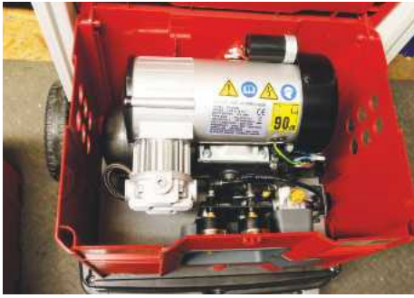
... and of course, the compressor itself
