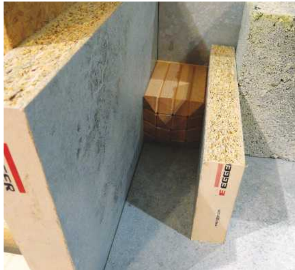
PIC 8. Never discard offcuts of kitchen worktop: they're solid, flat, stable and impervious. I cut these up on the table saw so they were square too, and set them in a frame of heavy chipboard that I'd made for this purpose before. And always have a concrete block handy. You just never know
