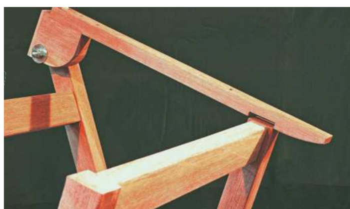
PIC 14. One bearer in place showing notches, raising block and M8 bolt
