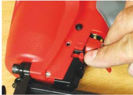
The guns all share similar attributes, such as switches for bump or sequential fire...
