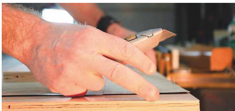
ABOVE: Laying wood veneer
