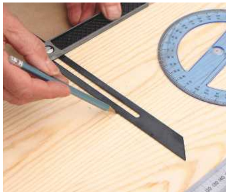
STEP 3. Both legs are splayed at 5°, so adjust the sliding bevel to 85° when marking out
