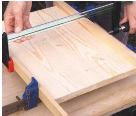
STEP 1. Glue and cramp boards together to make up the two legs. Plane the edges first if necessary
