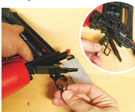
The two nailers feature a quick-release nose toggle for nail jams
