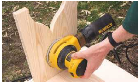
STEP 26. Remove the hinges and sand bench with 120 and 180 grit abrasives, ready for final finishing
