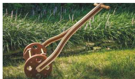
STEP 25. Now attach the arms to the wheels by inserting the little axles through each arm, then attach the handles at the other end. I attached the handles by inserting a 12mm dowel into the end of the handle, and putting the 12mm dowel through the end of the arm. In the inset photo, you can see a close-up showing how the pins are inserted into the 12mm dowel to hold things in place
