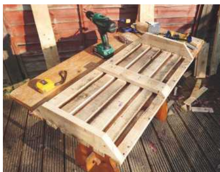
PIC 8. The shelves are 800mm wide, which is the length of the short planks from the pallets
