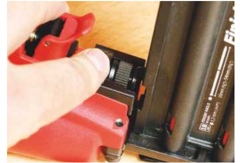
... as well as the depth of drive controls for setting the fixings in different materials
