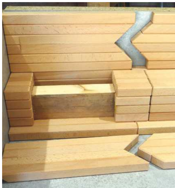
PIC 9. The softwood block is to maintain the nose cone in its proper place. The 16 loose blocks in the middle are to stop the sides collapsing in as they are glued. The little vertical line (top left) is where I scalloped out the four sides because over the course of the project, the beech had shrunk and the bottle became uncomfortably tight. The scallop was achieved by passing the sides over the table saw at right angles to the blade, guided, of course, by a fence
