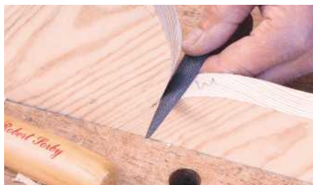
STEP 15. To get right into the apex of the curves, a combination of rasp and wide chisel does the trick
