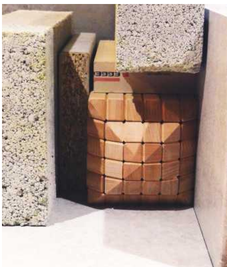
PIC 10. The final assembly was not entirely satisfactory. I want a massive iron cramping jig in three dead square axes. In its absence, a couple of concrete blocks have to do. I don't like the look of the strip one up from the bottom left-hand corner. I decided to leave this here for half an hour, which gave me the chance for some emergency sash cramping if required
