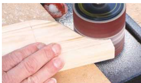
STEP 18. Saw rails to length. Mark and cut ends to shape with the jigsaw before cleaning up on the sanding drum
