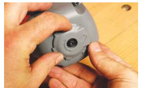
The bigger 15-gauge gun has a top-mounted rotating exhaust
