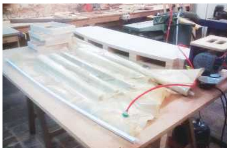
The interior faces of the legs are veneered in a vacuum bag press...
