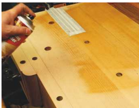
The Sanding Sealer is applied from around 150-200mm away and coats really quickly
