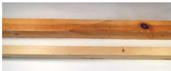
ABOVE: Two of Michael Huntley's practice scarf or bird's mouth joints, which are useful for sawing practice
