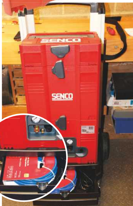
The trolley features a small drawer for storing the hose and power cord
