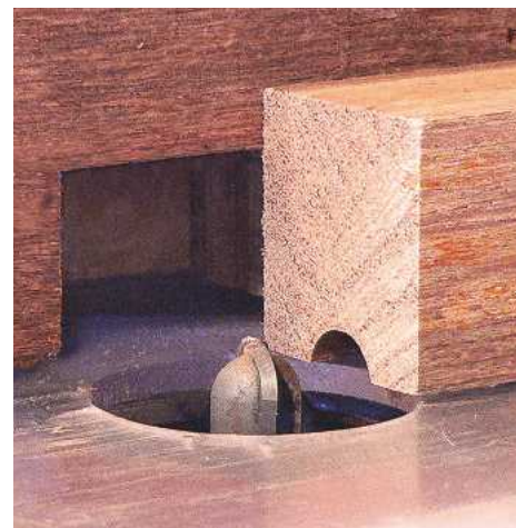
PIC 5. Routing the trough for the rod
