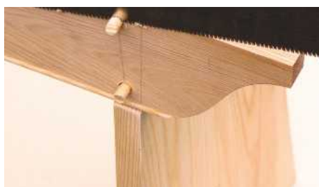
STEP 21. Glue matching plugs in the holes and saw off excess when dry, then trim flush with a block plane
