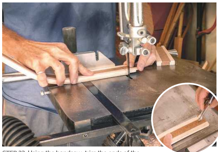
STEP 23. Using the bandsaw, trim the ends of the arms and round them over nicely
