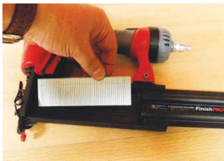
... while the 18-gauge gun is loaded into the side of the magazine channel
