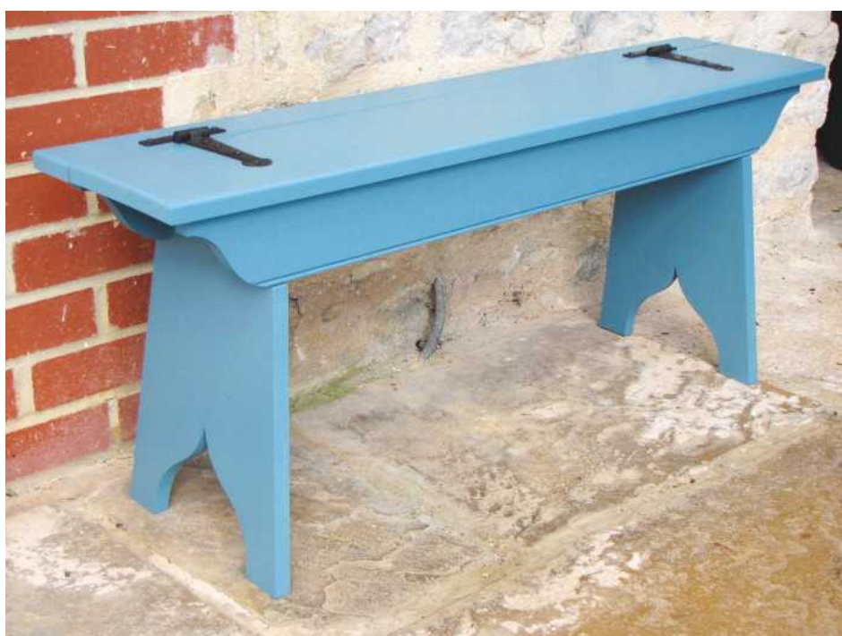
STEP 18. Saw rails to length. Mark and cut ends to shape with the jigsaw before cleaning up on the sanding drum
