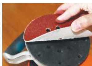
The sander requires standard hook-and-loop abrasive pads
