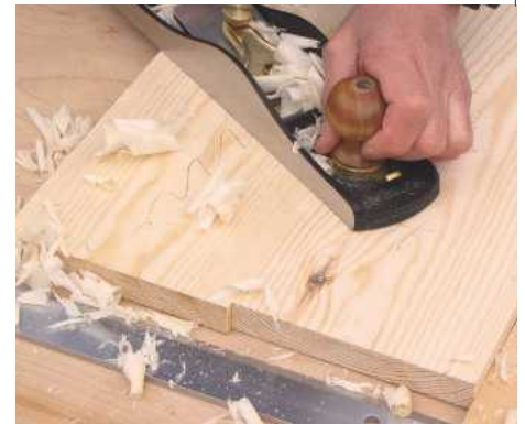
STEP 2. When the glue has dried, level the boards with a bench plane, checking with a straightedge
