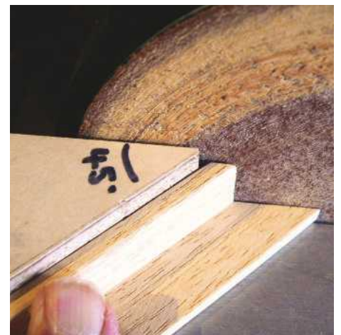
PIC 10. Trimming the mitres on lippings
