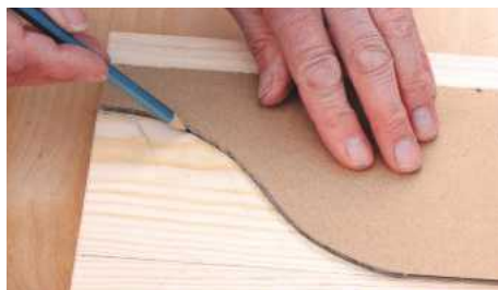
STEP 12. Cut the card with a craft knife. You only need a half template – simply flip on the centreline
