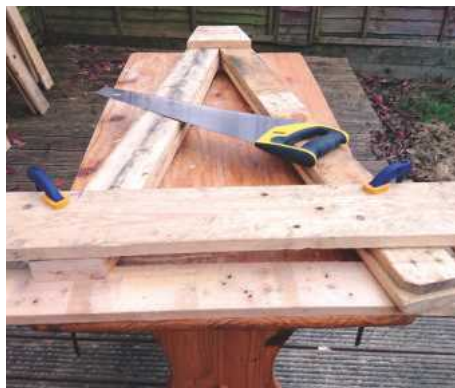
PIC 5. Sawing both legs as a pair
