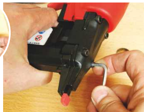
The stapler nose has to be stripped down with a hex wrench
