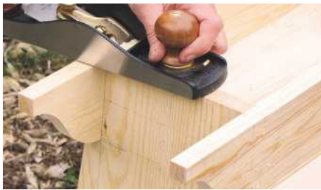
STEP 22. Plane legs and rails flush, working in towards the centre to prevent the timber splitting
