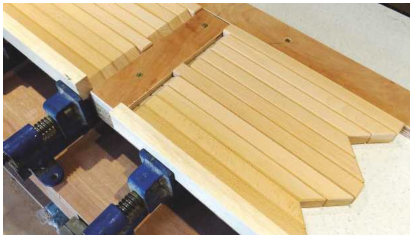
PIC 6. A pair of long sides and short sides cramped up. The PVA bottle recommends leaving assemblies cramped for three to four hours. Here, three to four minutes were enough. The strips are so flat that suction keeps them together. After that, if some error has occurred, it is actually quite difficult to get them apart. I cleaned away excess glue before it set
