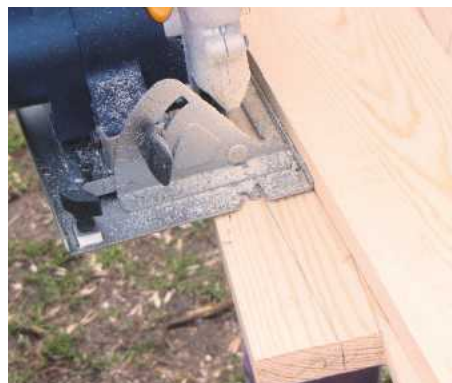
STEP 9. Cut the tapers on each leg using a baton cramped as a guide fence. Cut slightly oversize
