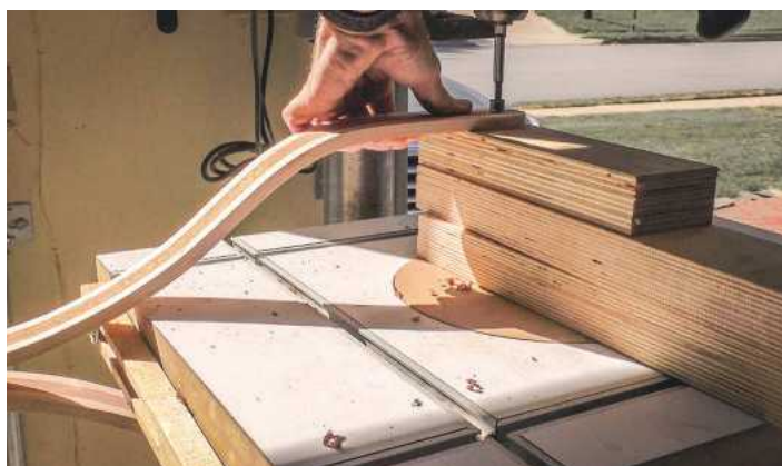
STEP 24. Drill a 16mm hole into the end of each arm at the point where they will meet the axle/centre of the wheel
