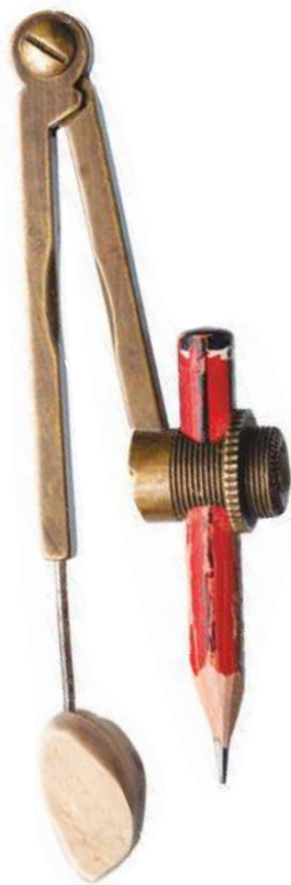
ABOVE: A simple schoolroom compass can be ideal for scribing
