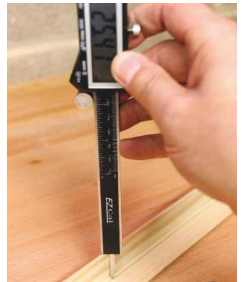
Checking the depth of rebates, internal corners, etc. is easy with the depth post
