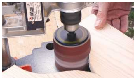
STEP 14. Use a large-diameter sanding drum to tidy up as much of the cut-outs as possible
