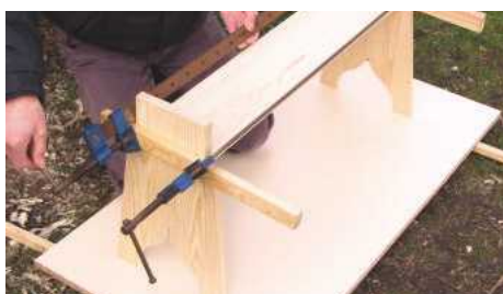
STEP 17. Glue biscuits into slots and assemble the bench with PVA glue. Use cauls to spread pressure when cramping
