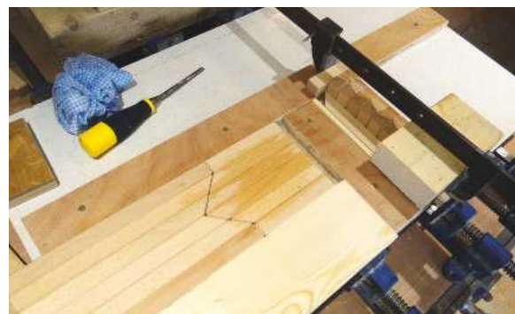
PIC 7. This is annoying. To ensure a good fit, the strips on the right are settled into the already glued assembly on the left, but here, and on all the assemblies, they would not mesh precisely. The zig of the zag (appearing almost vertical in this photo) won't close up. This is because the guillotine sliced fractionally off square, and two fractions make a gap. For the same reason, the zag of the zig was as snug as a bug
