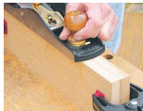
STEP 4. Saw both end pieces and plane them together, keeping them rectangular at this stage
