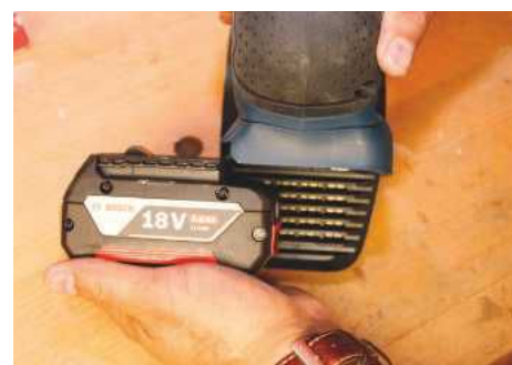
The battery pack slides neatly onto the back of the sander
