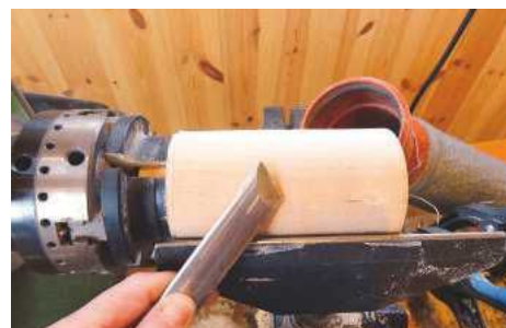
STEP 3. Turning to round using a skew chisel (note extraction close to the lathe)
