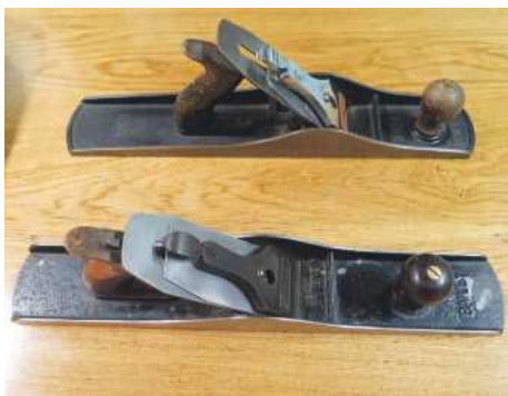
PIC 10. My cut down plane compared to a standard No.6 (notice proportions)
