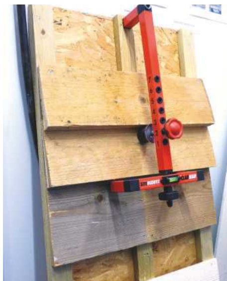
The Sitebuddyz Cladman offers a clever solution if you're cladding a workshop or outbuilding
