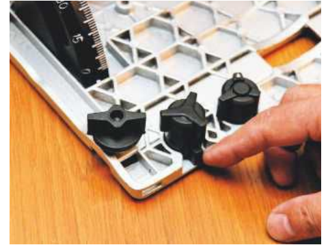
Two adjuster dials are used to snug the saw to the track
