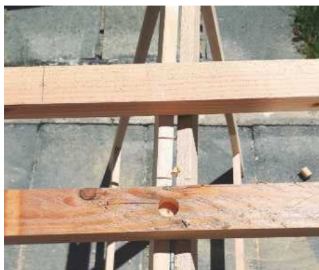
STEP 3. The pocket holes drilled to fit the ladder rungs
