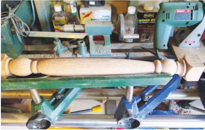
PIC 2. Turning before splitting
