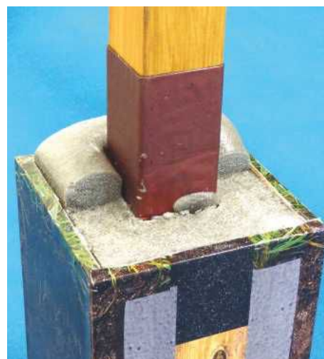
Quikset is a resin that's activated in a pouch, then simply poured into the hole, fully curing in around 90 minutes
