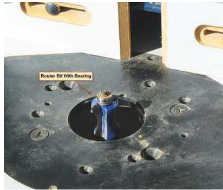
PIC 5. Close-up of the router bit with bearing attached
