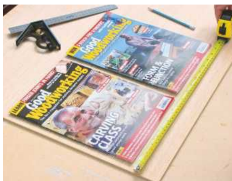
STEP 1. Measure a couple of magazines to help decide internal measurements, allowing space between them
