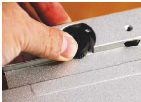
This serrated offset cam is the anti-kickback for safer cutting
