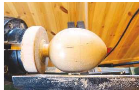
STEP 11. The completed plain egg, waiting to be parted off its sacrificial base
