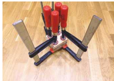
STEP 14. Once glued, each square needs to be cramped up and left to dry overnight
