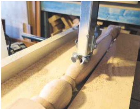
PIC 4. Splitting the turning on the bandsaw
