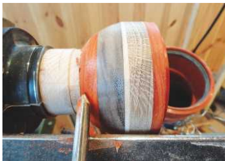
STEP 26. Working on the outside using a spindle gouge, prior to parting off
