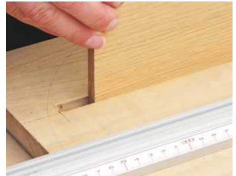
STEP 7. The groove is stopped about 10mm below the curved top edge. Check that the divider slides and is not too tight
