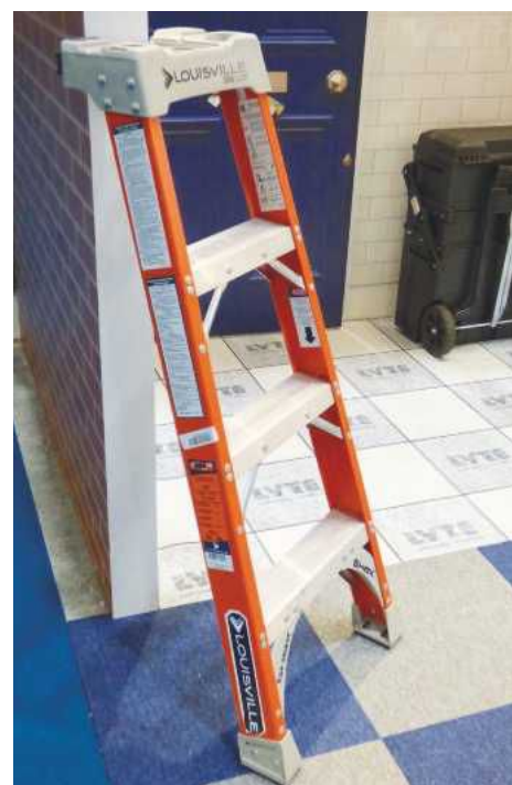
Lyte's rather unusual Louisville glassfibre ladder has cut-outs at the top, which enable it to be propped against an external or internal corner
