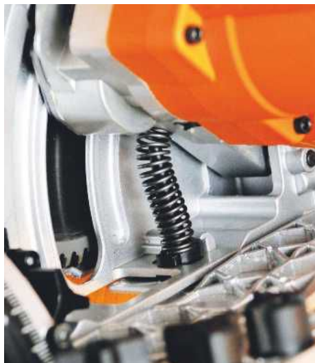
The plunge is controlled by this central spring, which is housed beneath the motor
