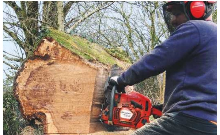
PIC 10. Embedded nails and barbed wire all but ruined one chain, and prompted repeated sharpening of others. After every cut we reassessed what we might do next, avoiding ironwork and making the most of the spectacular grain, which was only revealed chunk by chunk
