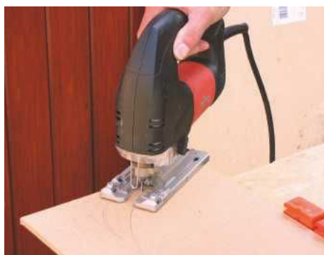
STEP 3. Cut the template with a jigsaw, then tidy up the curve with a block plane and sanding block
