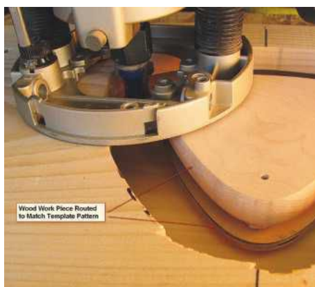
PIC 22. The finished wood workpiece is routed to match the template pattern
