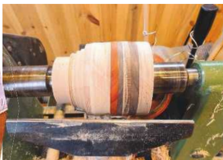
STEP 19. Mounted between centres and starting to look more like an egg
