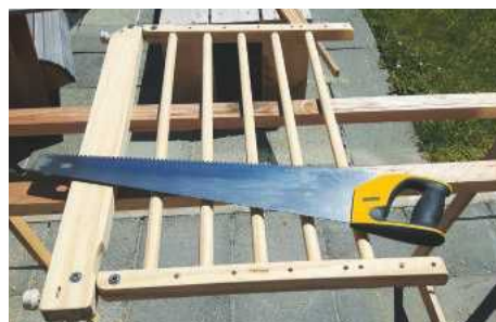
STEP 5. Use a hand saw to cut the remaining spindles from the safety gate
