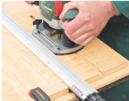
STEP 6. Mark the position of the divider panel along the centre of each end. Rout a 10mm groove to about half depth
