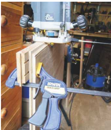
PIC 11. Carefully routing a corner bead on the rebated edge
