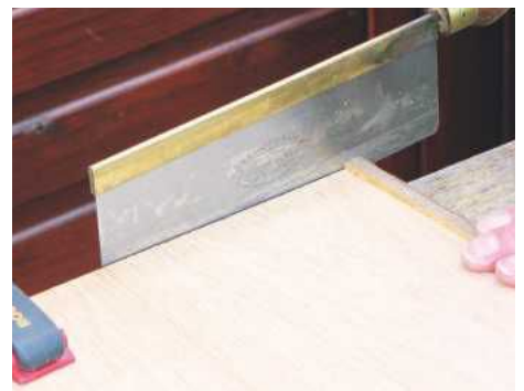
STEP 16. When the glue has dried, carefully cut the ends to length with a fine saw, finishing with a block plane if necessary
