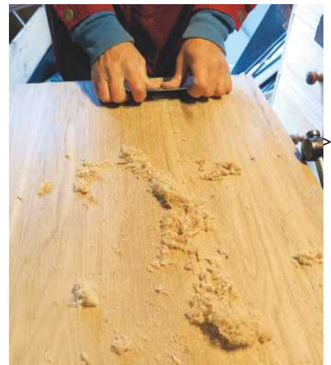
PIC 9. A cabinet scraper is used to finish the solid oak board
