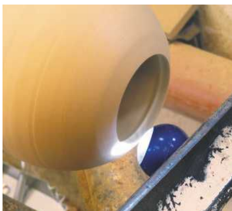
STEP 16. A couple of years ago one of my students gave me a small LED light that can easily be attached to anything. I have it on the toolrest so it shines inside the piece I'm working on but doesn't get in the way of the tool
