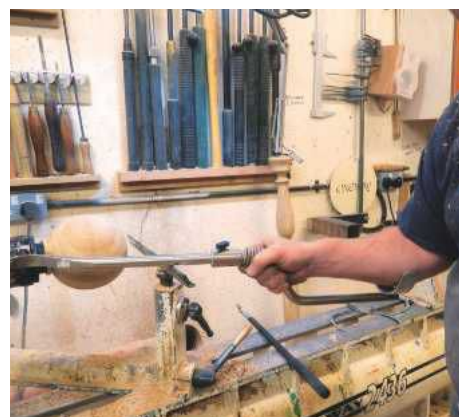
STEP 18. The tool has an armbrace attachment, which makes it easy to control. It also has a side handle, but I personally don't recommend this as I prefer to look for the areas inside the vessel where the tool doesn't twist
