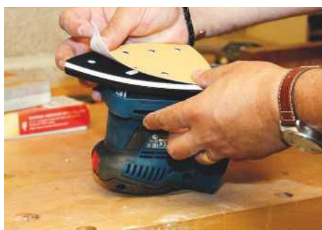
Hook-and-loop abrasives can be used on all three bases
