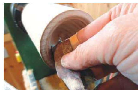
STEP 6. Sanding the interior of one half of the egg before moving on to buffing
