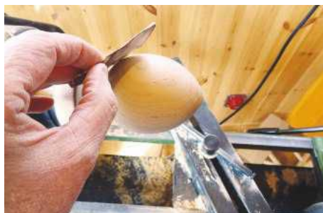
STEP 10. With the two halves together, sanding of the egg exterior can begin
