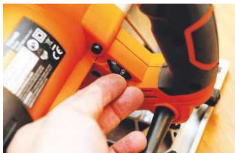
The variable-speed dial is used for cutting different materials
