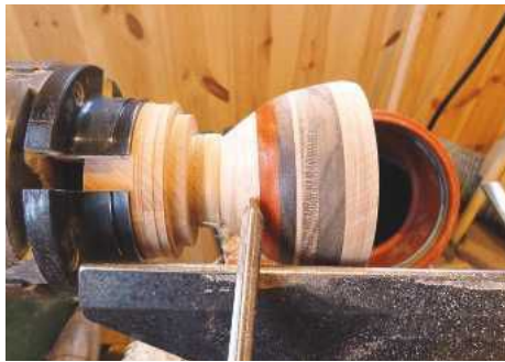
STEP 23. Using a spindle gouge to achieve the egg shape
