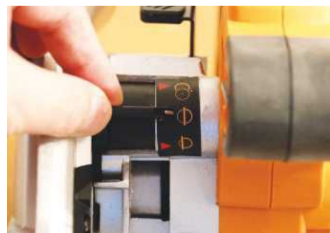
This lever controls the blade for plunge, blade change, or scoring cuts
