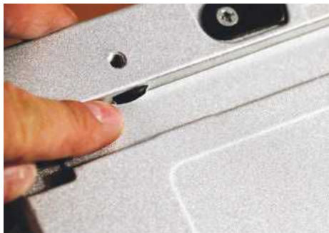
The dials micro adjust these small guides
