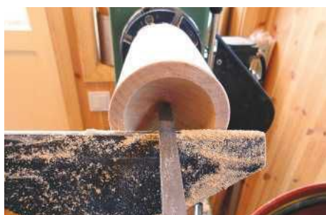
STEP 4. Starting to hollow out the blank to achieve the egg shape
