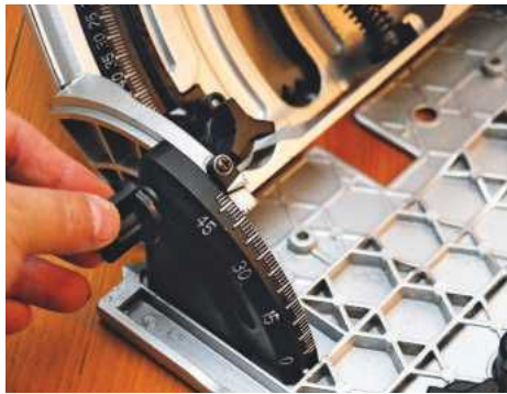
The blade tilt locks at the front and back with locking knobs
