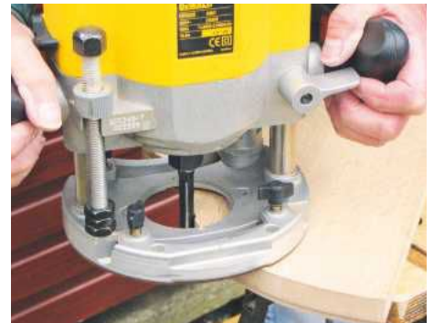
STEP 10. With a flush trim cutter fitted in the router, carefully cut the curve to shape, following the template
