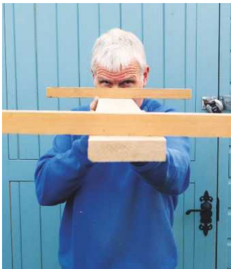
PIC 7. Checking for wind before running through the thicknesser
