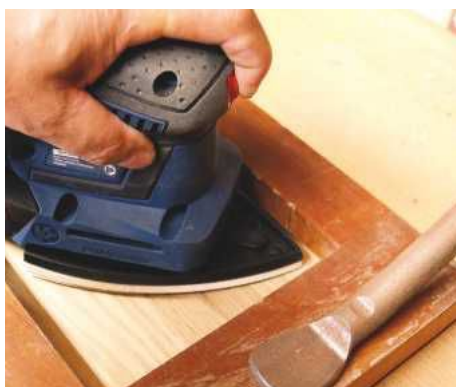
The delta base is ideal for getting into tight recessed corners
