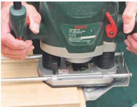
STEP 11. The bottom panel will be rebated into the end pieces. Ensure to rout these carefully along the lower edges
