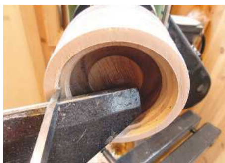
STEP 21. Turning the tenon so both parts of the box fit together
