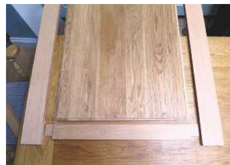
PIC 14. Main board components before gluing up
