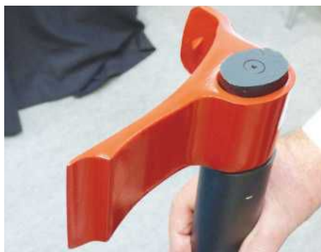
The Finnish Leveraxe relies on leverage force – rather than wedging force – to split the log and so requires less effort
