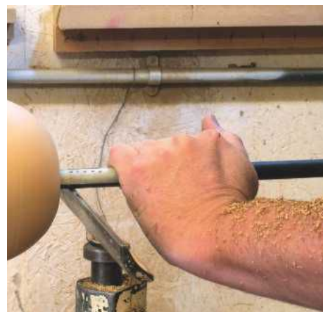
STEP 12. This tool is used horizontally with the toolrest close to the entrance. Work the tool using nice flowing movements with the shaft along your forearm to aid stability
