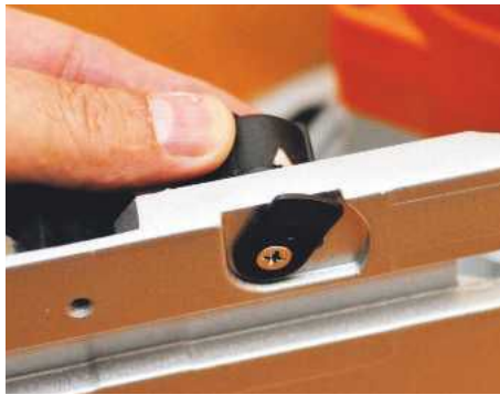
This tab rotates and links into the track when making bevel cuts
