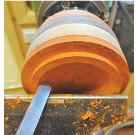
STEP 25. Turning the inside of the box's bottom as before
