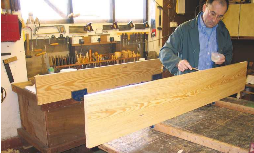
Coating the cut slots with glue
