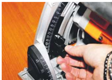
The plunge depth can be restricted with this adjustable stop
