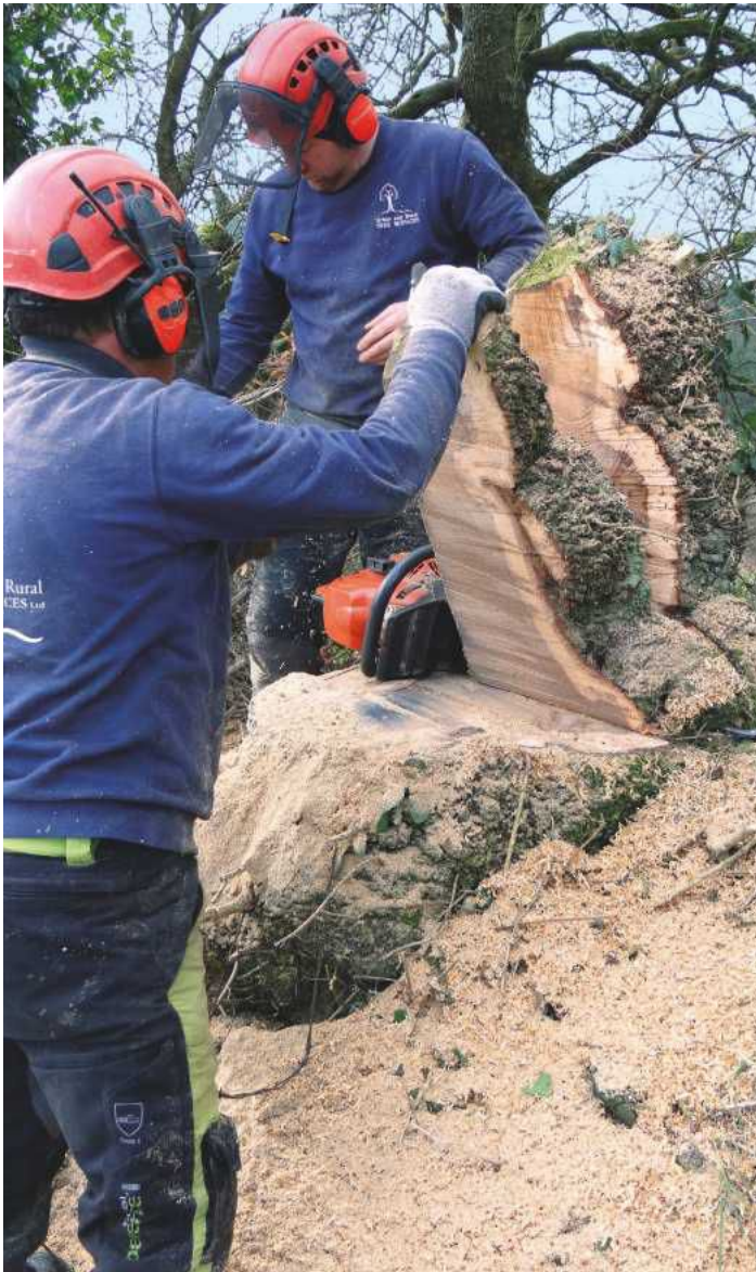
PIC 11. A sideways cut through the burr produced some stunning chunks. It'll take a few years airing these in stick in an open shed before bringing them in to season a little further. But they are destined for sculptures, not furniture, so bone-dryness won't be necessary
