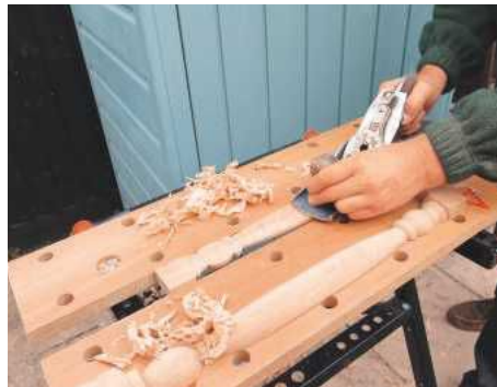
PIC 5. Planing the split turning while it is held in a portable workbench
