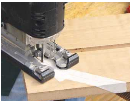
STEP 8. Saw curves, keeping about 3mm away from the pencil line. Masking tape will reduce splintering on the surface
