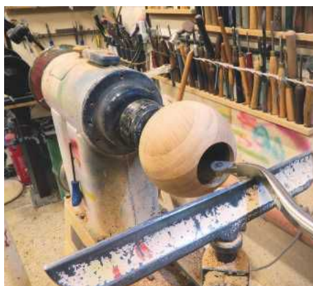
STEP 17. The final cuts around the piece are made using the Stewart scraper system from Robert Sorby; there is a small sharp teardrop-shaped scraper on the end. If the curved part of the tool is on the toolrest, it will twist in your hands
