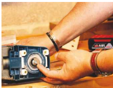
This metal oscillator sets the orbital action for the various bases
