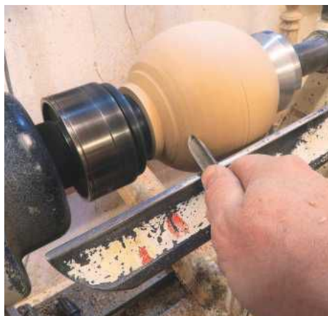
STEP 10. The tool is worked this way when coming around the left-hand side of the sphere. The bevel needs to be in contact with the wood as you traverse around
