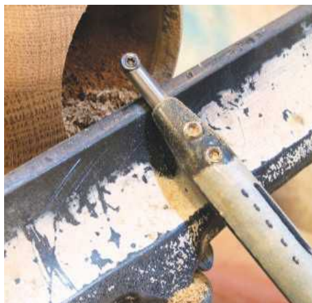
STEP 11. The hollowing is carried out using a Simon Hope hollowing tool – the small TCT cutter used with the big bar is a fantastic combination for easy cutting. The marks on the top show the best position for cutting
