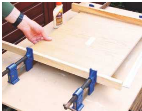
STEP 15. The ends of the front and back panels are lipped with solid oak. Cut slightly oversize and glue to the edges
