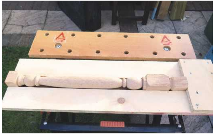
PIC 3. Simple cradle for use on the bandsaw
