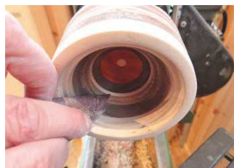
STEP 22. Sanding the interior before applying a finish
