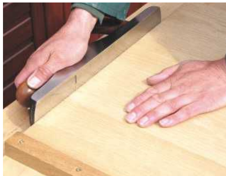
STEP 12. Saw the divider panel to size and trim the edges with a bench plane and shooting board. You can then check for square
