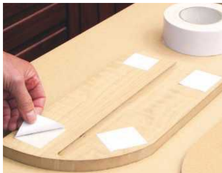
STEP 9. Stick double-sided tape to one of the end pieces. Firmly press the template in place, checking alignment
