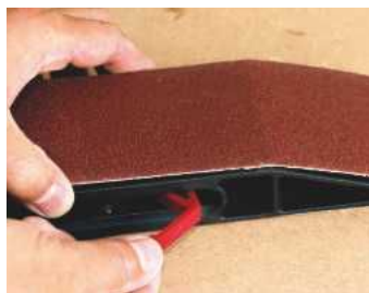
Belts are swapped using this tension lever, although it doesn't look to be overly durable
