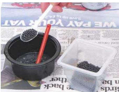
STEP 10. Mix the epoxy adhesive thoroughly and add enough lead shot for filling both holes in one core piece
