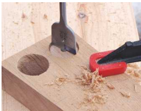
STEP 8. Mark hole centres at the bottom of the core timber. Drill a pair of 38mm holes with a flatbit mounted in a drillstand
