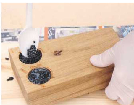
STEP 11. When fully mixed, spoon the lead carefully into each hole. Allow this to settle, but don't overfill
