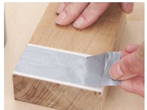
STEP 9. Cover the holes on one side with several layers of masking or gaffer tape, pressing this down firmly
