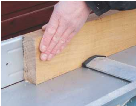
STEP 1. Plane faces of the inner core and make sure one long edge is square. The opposite one will taper
