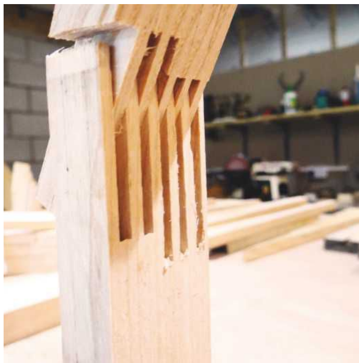
PIC 3. But if the components were rotated by 90°, they'd clasp each other, fingers interlocked with no stress or strain. This, I thought, was better. But then it disturbed me that I had not arrived at this obvious and profound conclusion by myself. Must I go round the houses in order to arrive? On the other hand, I quickly retorted; isn't it good to be working in a system that automatically corrects for human error?
