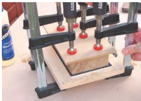
STEP 14. Brush PVA glue on to surfaces and stack up layers. Cramp together with cauls to spread the pressure
