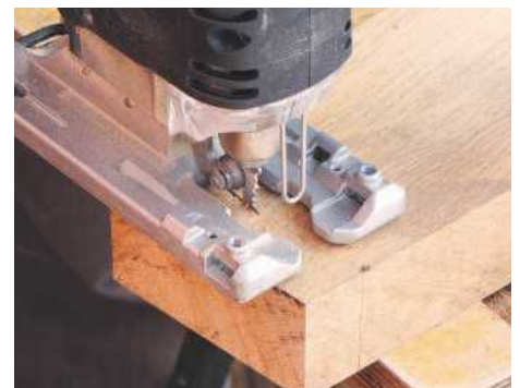
STEP 6. Carefully cut out the core timber with a jigsaw, ensuring to keep just on the waste side of the pencil lines
