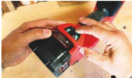
A toggle switch and a set of lights show the status of the gun, which also powers it on or off
