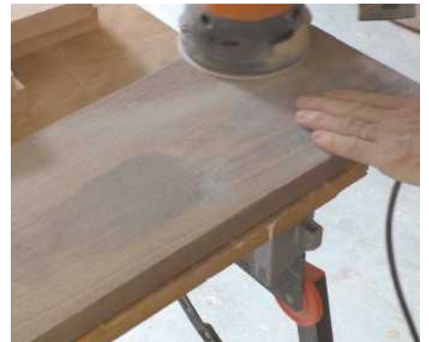
STEP 9. Sanding away the excess epoxy to make the surface nice and flat
