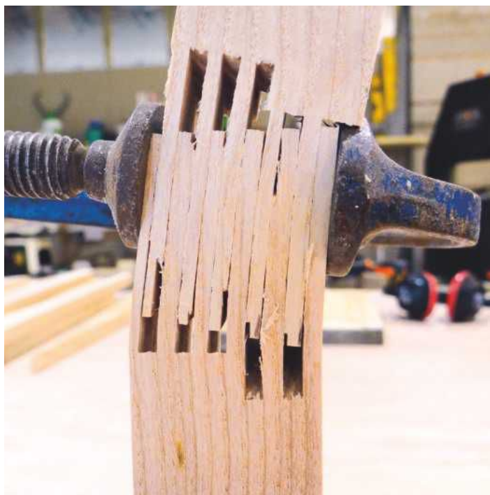
PIC 2. Inauspicious beginnings. What was I thinking of? If these rough-hewn combs were five times as long, they might invite a satisfactory curve with a radius of, say, 400mm. To laminate on that scale makes my modification (to have one end remaining in the solid) of little consequence/a bit of a nuisance
