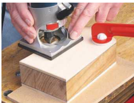
STEP 17. Finish edges with a light chamfer or rounding-over bit. Alternatively, use a block plane
