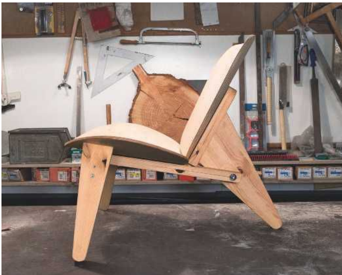
STEP 10. Screw the back chair leg into place with a large machine screw (M12 x 120mm), countersinking it with a Forstner drill in order to recess the screw. You can also use a longer screw, of course
