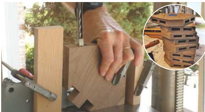
STEP 21. For drilling the mortises into the seat pieces, I used a mortising attachment with a 10mm bit on my drill press
