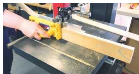
Deeping is often safer on the bandsaw, using a gripper to hold timber against the fence
