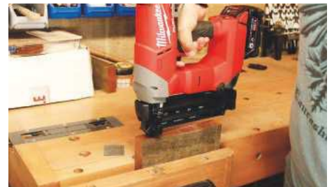
Firing 54mm brads into sapele posed no problem for the gun in either mode
