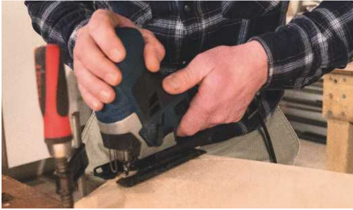
STEP 8. Carefully saw the shape of the surfaces and then sand the edges. Round off the edges by sanding them manually
