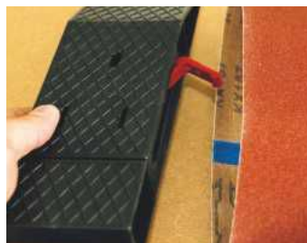
The Sand Devil 3.0 takes standard off-the-shelf 533 × 75mm belts
