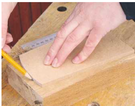
STEP 5. Cut out the template and clean up edges. Align the 90° corner on the core timber and draw the outline
