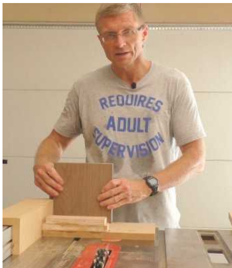
STEP 13. I decided to make a jig that fits over my table saw fence so that I could make cuts with my dado set
