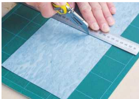
STEP 13. Cut veneer and outer facings to size. These should be at least 3mm larger all round than the core
