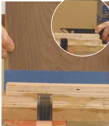
STEP 14. Rather than making the full cut of 25mm high × 24mm wide in a single pass, I made the cut in two passes
