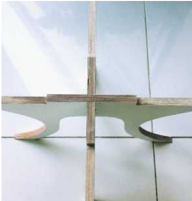
PIC 15. Assembling the side panels
