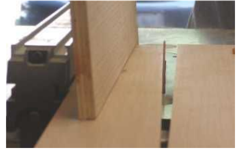
STEP 3. Cutting the legs to be 75mm wide using the table saw
