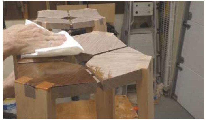
STEP 31. To finish, I applied a tung oil followed by paraffin oil mixed with some medium coarse pumice stone after the final coat had dried
