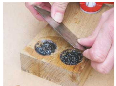
STEP 12. Leave to cure overnight, then clean off excess glue with a cabinet scraper or using a sanding block
