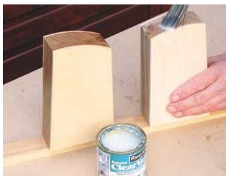
STEP 18. Fine-sand surfaces and brush on a couple of coats of satin varnish, denibbing between coats
