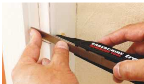
It will transfer the line if the lining has stops fitted – an area where a gauge may struggle
