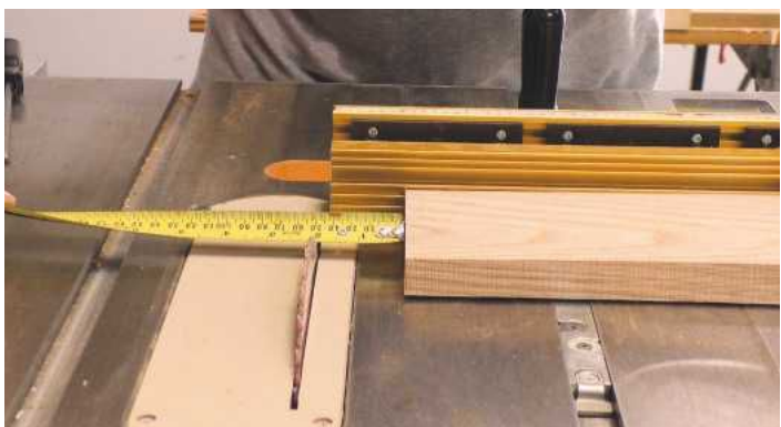
STEP 23. Cutting the tenons to length using a stop block
