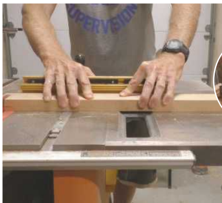
STEP 26. Set the table saw blade to have a 5° bevel and then trim the legs to length
