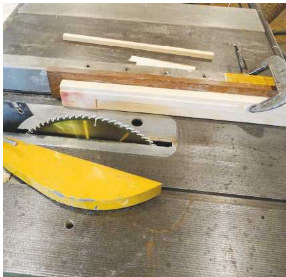
PIC 4. A second fence is cramped on to the existing one. The thin, shaped strip, which is glued to it, allows the component to be stopped precisely. The strip is thinner than the first tooth of the comb so that the first gap can be cut
