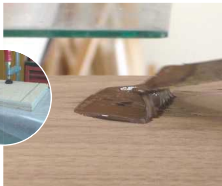
STEP 8. To fix the grain separation, I decided to use dark brown epoxy, added wax paper, then clamped it with a board to join the wood together
