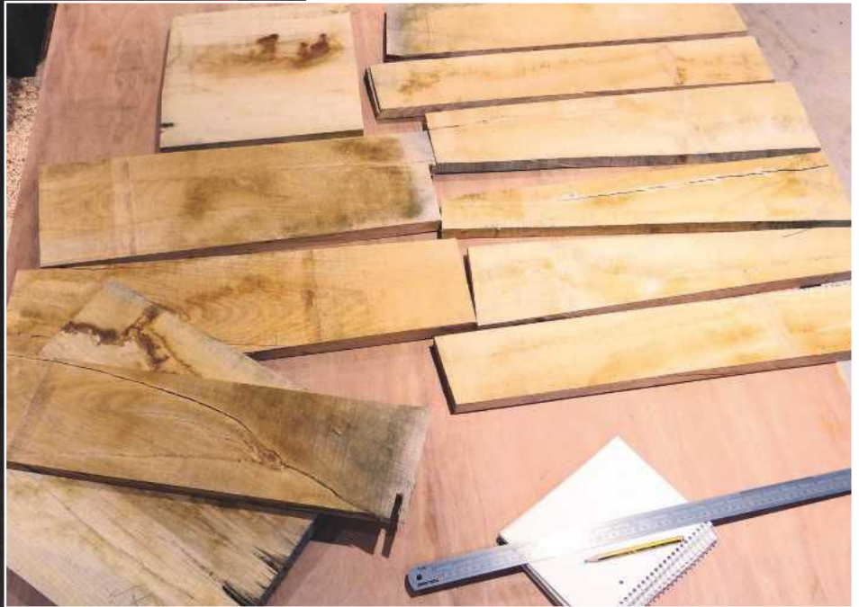
PIC 1. The ends, seen bottom left, had no worthwhile timber in them and will, sadly, end up on the fire. Top left is a better piece whose main fault is in being short – but, critically, not too short to go through the thicknesser. I had already sawn down existing shakes. There are more cuts to make. With each necessary cut, the amount of usable timber dwindles
