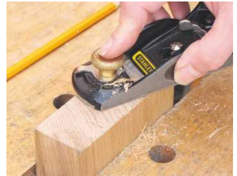
STEP 3. Trim one end of the core timber square with a finely-set block plane or on a disc sander
