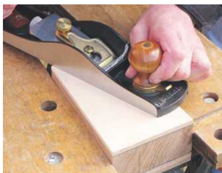
STEP 16. Using a finely-set bench plane, carefully clean up facings and edges, checking the grain direction
