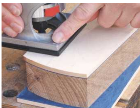
STEP 15. When the glue has dried, use a bearing-guided straight router bit to trim facings flush with the core
