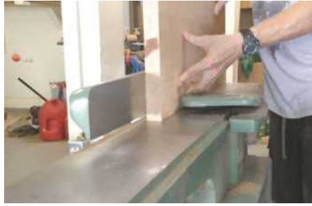
STEP 2. Jointing one edge of the cherry to make sure that it is straight prior to cutting the legs on the table saw
