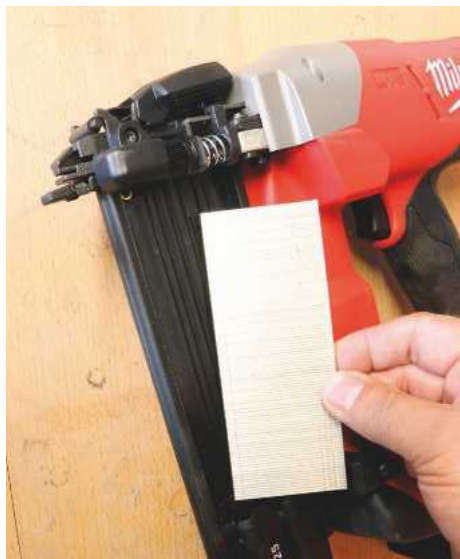
Fixings drop easily into the magazine – the total capacity is 110 nails
