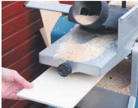
STEP 2. The outer facings can be of any thickness. Here sycamore is being reduced to a thickness of 6mm
