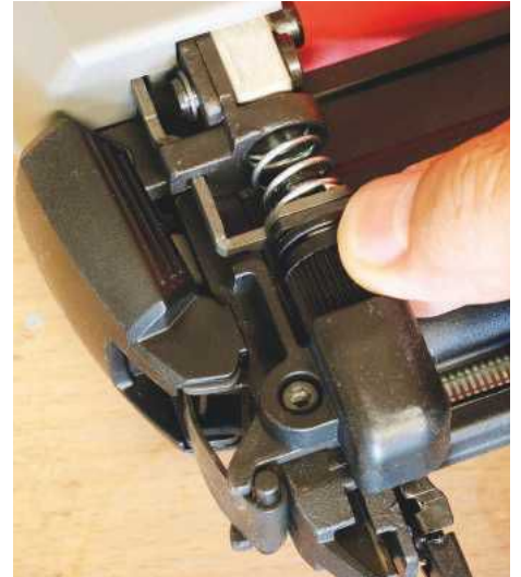
A simple dial adjuster sets the depth of drive for the fixings
