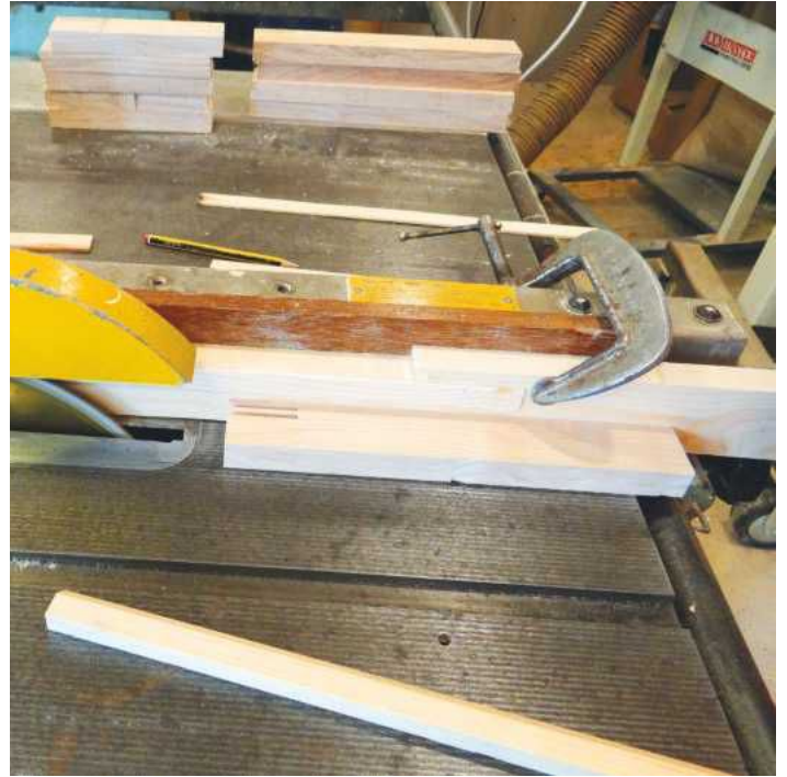
PIC 7. Cutting the second gap. A push-stick is necessary though largely as a pull stick. When the component is stopped by the fence, it has to be drawn back. The stick makes this safe and controllable
