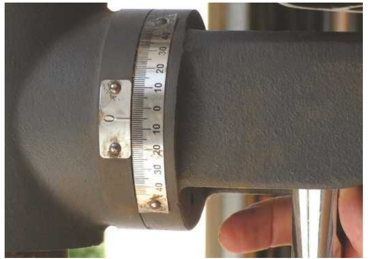
STEP 20. The angles are going to be set at a 5° angle (i.e. 85° to the floor)
