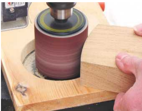
STEP 7. Plane tapered edges to the line, then shape upper curves with a sanding drum. Check against the template
