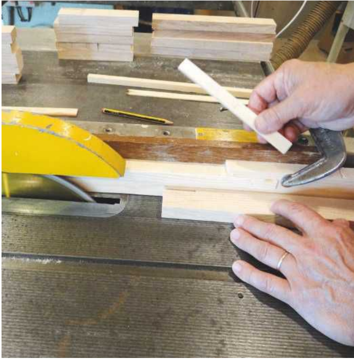
PIC 6. Holding the component firmly to the table; releasing the fence and winding it out, then back in with a spacer in place; locking the fence; removing the spacer and repositioning the component for the second gap. This spacer is a vital part of the procedure and determines the tightness of the joint by affecting the thickness of the comb's teeth
