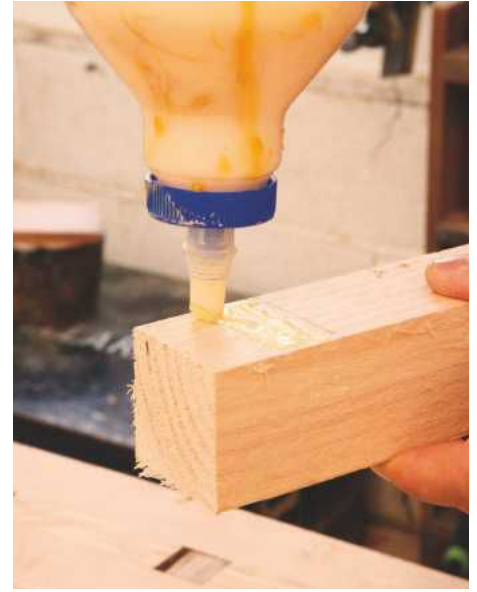
PIC 3. PVA-type glues are among the commonest and most easy to use for general furniture work
