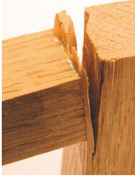
PIC 2. Two pieces of oak were glued in a right-angled butt joint, then force applied to snap the joint. Again, the wood broke before the glue showing that even an end-grain glue joint is strong
