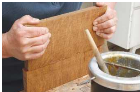
PIC 20. Instead of clamping, the glued edges are rubbed together for a few seconds until the joint grabs
