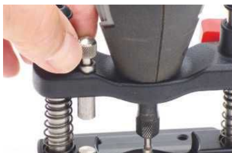
PIC 7. Beneath the depth stop is a steel insert set into the base, so the rod does not mark the aluminium
