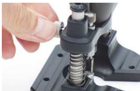
PIC 6. To set the plunge action there's a steel depth stop located in the bridge, with thumbscrew locking and built-in fine adjuster
