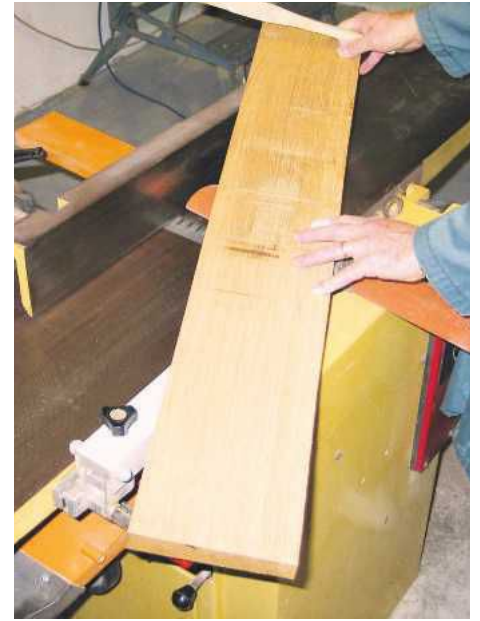
STEP 3. 'Hit and miss' is OK at the facing stage; this can be removed later on
