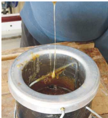
PIC 9. Pearl glue mixed with water is heated until it forms a thin gel that thickens within a few seconds of cooling
