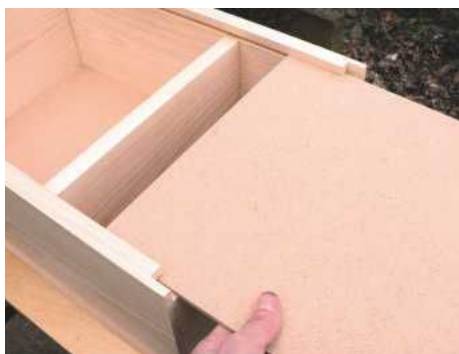
STEP 17. Cut a piece of 6mm MDF to size for the front panel. Check it slides neatly, then glue on a small block for a pull grip
