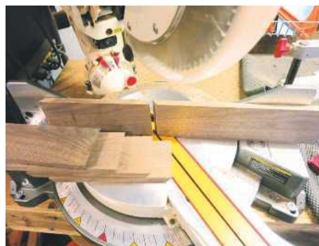
STEP 3. Once ripped to length and resawed, the pieces for the top need to be mitred to match the pentagon top
