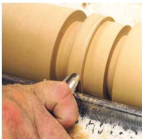
STEP 8. Let the shaping begin! This is great fun as you can pretty much make it up as you go along. The spindle gouge is used for shaping the half beads, which will sit above and below the shelves
