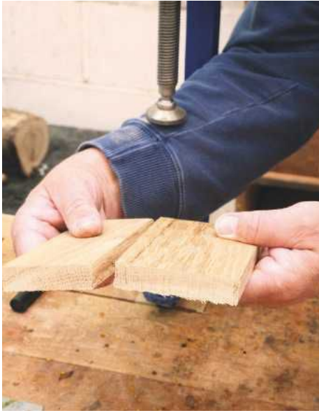
PIC 1. Oak boards were glued edge-to-edge and then snapped using clamps. The break occurred 10mm to the left of the glue line so the glue was clearly stronger than wood!
