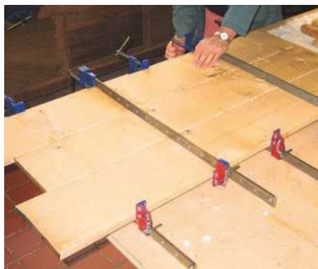
STEP 21. Rub the joints and clamp the top up from both sides to keep it flat
