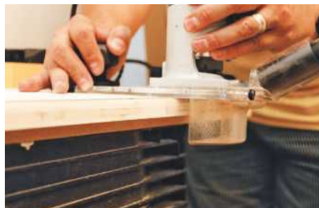
Dust control is excellent with the edge dust collector kit fitted
