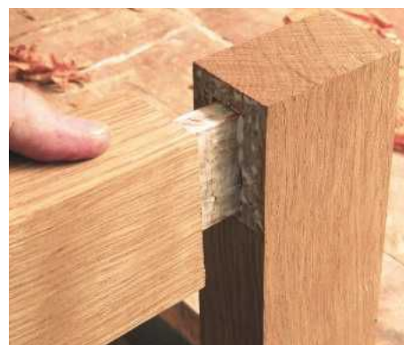
PIC 22. Pin and socket joints, such as this mortise & tenon, can have glue applied to some or all contact surfaces
