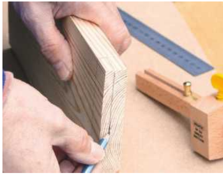
STEP 2. Set your marking gauge to one-third of the timber thickness. Running a pencil along the line helps it to show up clearly
