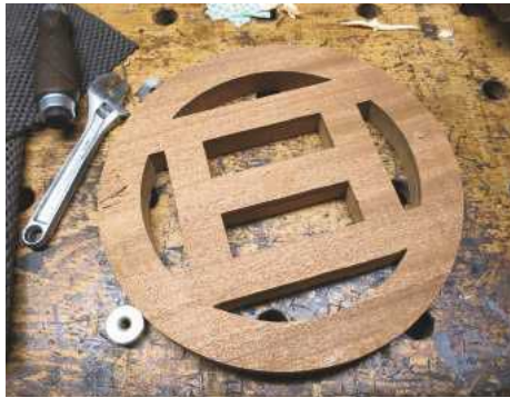
STEP 12. The symbol after pattern routing and due to the thickness of my stock, scrollsawing. This was later resawn by hand
