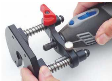
PIC 3. In the case of Dremel, you remove the nose end cap to reveal its threaded collar and screw the tool into the housing
