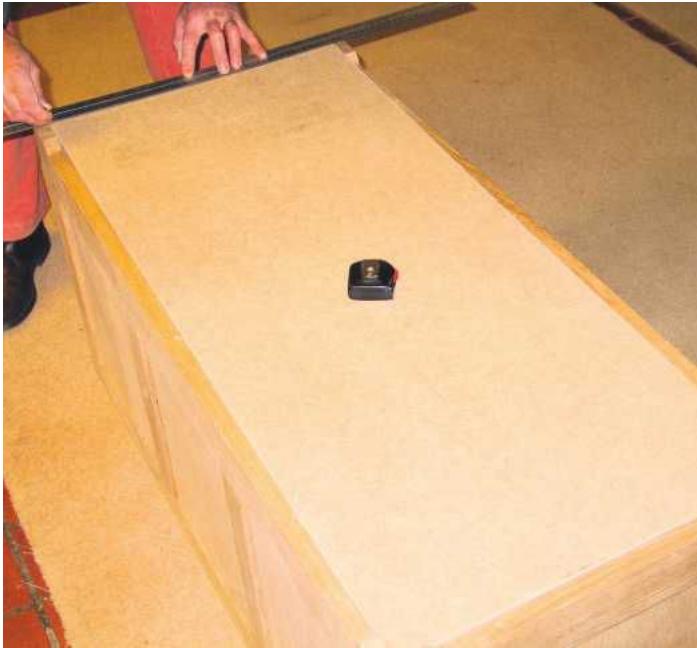
STEP 18. Measure and finish to size the bottom from underneath
