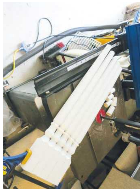
STEP 1. I used reclaimed banisters for the table legs. Once laid out, depending on the size of the skirt you'd like to use, stack cut the square ends on a mitre saw
