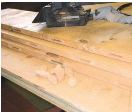
STEP 20. Joining the top from a number of pieces using biscuits
