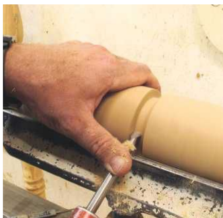
STEP 7. You want to try and keep the piece as strong as possible during the turning process, so finish each short section before moving along. If you're confident, then support the timber with your fingers to stop any vibration
