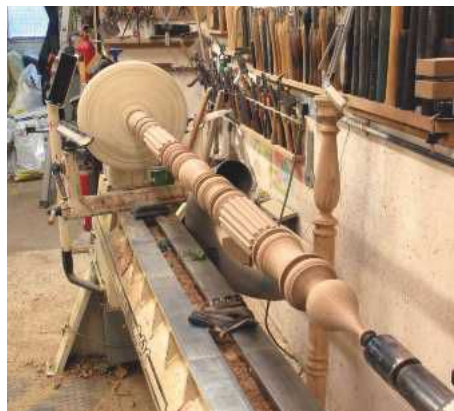
STEP 35. The length of the lathe allows me to use it as a clamp. I used PVA, but in hindsight I may have been better off using polyurethane. This whole project has given me lots of ideas for future display stands I can make in the future
