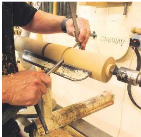
STEP 5. The slots are cut with the 10mm multi-purpose tool using a pair of Vernier callipers to gauge the size. This needs to be accurate, as if there's any slack in the joint, the shelf could fall out
