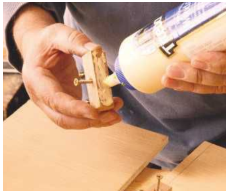
PIC 14. Adhesive is applied to pre-drilled and counter-sunk blocks, which are positioned along the line
