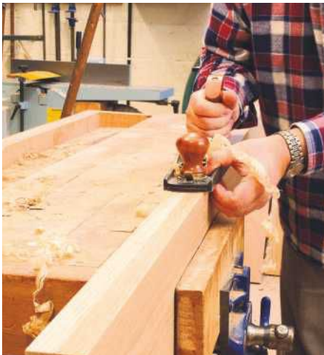
PIC 16. When preparing an edge joint the two boards are clamped face-to-face, then the edges are planed as a pair
