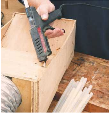
PIC 11. Hot-melt glue sticks are handy for temporary fixings and for sealing gaps, such as in a dust extractor
