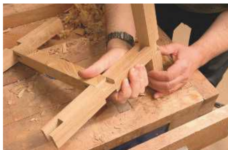
PIC 23. It is helpful to rehearse by fitting joints dry before gluing them, but it's best not to fully fit them as they may be damaged by pulling apart
