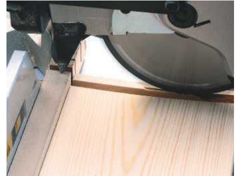
STEP 3. If using a sliding mitre saw, set the blade depth to cut rebates that form the lap joints. Check the depth on scrap timber first
