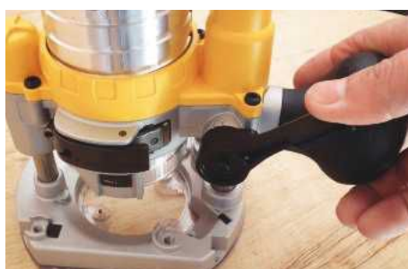
DeWalt have fitted an excellent oversized plunge lever to their base
