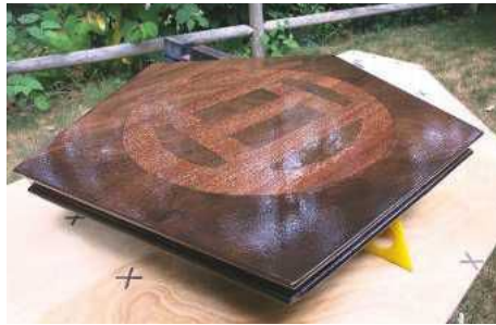
STEP 15. I used a wipe-on polyurethane through a spray gun to apply the top coat
