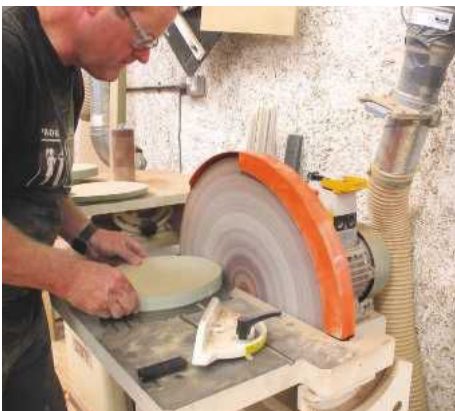
STEP 34. Having access to all the kit in the workshop next door is a huge bonus. The big disc sander makes short work of smoothing off the edges before applying the limestone effect, which is also used for the base
