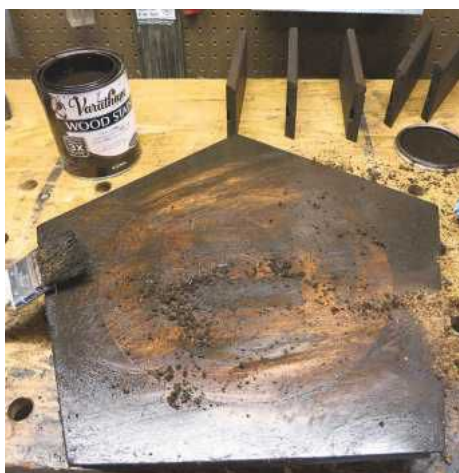
STEP 14. For the top, I used a few layers of filler followed by a thick layer of gel stain. With it still sitting on the top, I dropped a load of sawdust onto the top and worked it into the crevices
