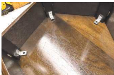
STEP 18. To attach the legs to the top, I used a ring of metal L-brackets on the inside to hold everything together
