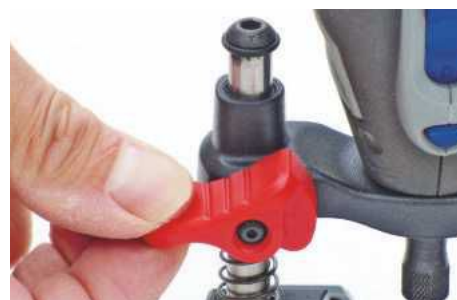
PIC 8. The red plunge locking lever is flipped up (rather than down) to lock the cutting depth
