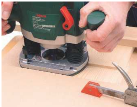
STEP 8. Mark out the shelf housing on both side panels. Rout out to the same depth as the groove for the lid
