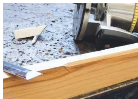
STEP 14. A bearing-guided bevel cutter in a router cuts the chamfers
