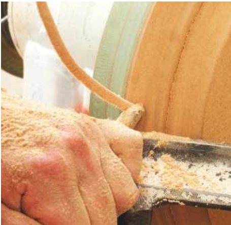
STEP 28. MDF turns really well and produces long, streamer-like shavings. Here you can see the dust on my hand so do always protect yourself from the dangers of fine dust, especially MDF
