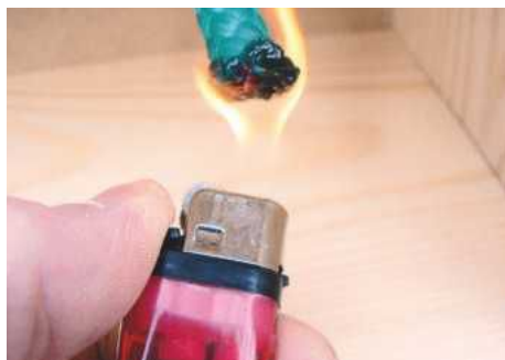
STEP 20. Cut the rope to length, then very carefully melt the ends with a flame to prevent fraying and pulling through the box
