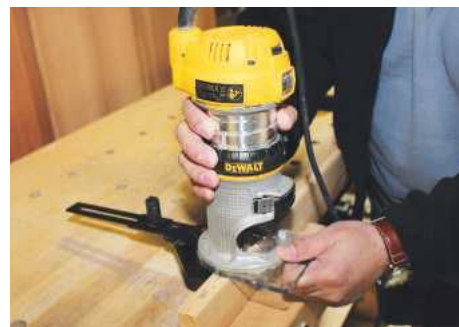
Fitted with the fence and steadying the base keeps it stable for edge mortising or grooving
