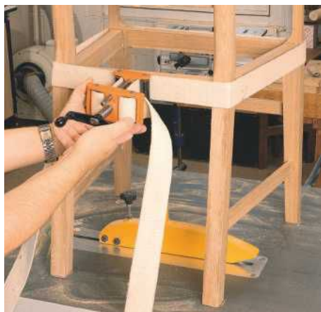
PIC 26. Awkward and irregular shapes like this chair seat can be pulled together with a strap clamp
