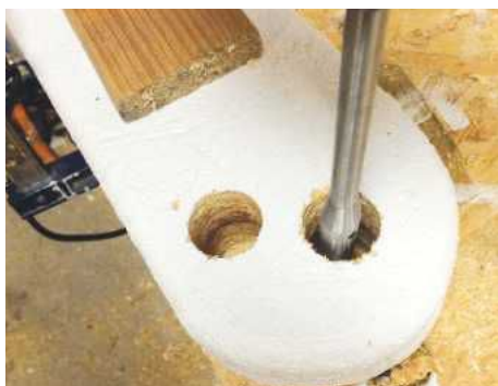
STEP 11. The best piece of equipment for drilling the holes is a pillar drill
