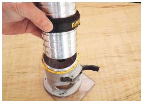
The motor simply drops into the bases for very easy engagement
