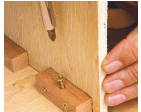
PIC 15. With glue applied to all the contact surfaces the joint is screwed together
