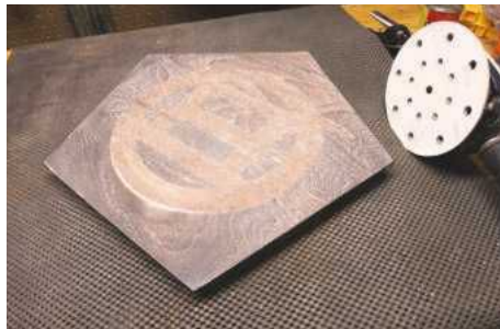
STEP 16. Sand the top between each layer at 400-800 grit to remove the last few dents and separations between the top and the symbol
