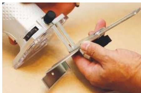
The supplied fence only fits to the fixed-base but is easy to adjust
