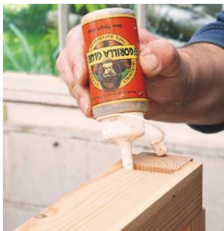
PIC 4. Polyurethane glues are particularly useful for joints with gaps as well as where a lot of seasonal wood movement is expected
