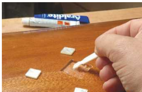
PIC 7. Two-part epoxy resins are ideal for fitting small decorative features or for embedding metal reinforcements into joints
