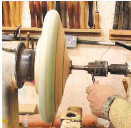
STEP 29. A sawtooth machine bit is perfect for drilling the base. The drill bit is mounted in a Jacobs-style chuck in the tailstock. The bar fitted into the hole in the chuck stops it twisting
