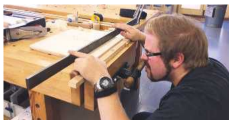
PIC 3. Checking flatness with a Veritas straightedge
