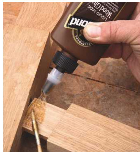
PIC 10. Modern solvent-treated hide glue avoids the need for heating and allows a much longer open time
