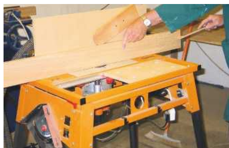
STEP 10. A straight cutter is used on the router table to cut the grooves for the panels
