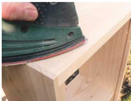
STEP 18. Fill the pin holes and sand the outside of the box, then remove any sharp edges with a sanding block
