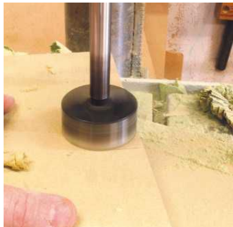
STEP 32. Use a 60mm sawtooth bit to make the initial hole in the shelf. Clamp the board securely and remove the drill frequently to clear out the build up of shavings
