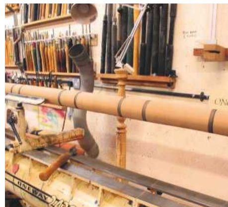
STEP 3. I am lucky to have a lathe that allows me to fit long lengths between centres. The first step is to rough the wood to the round using the spindle gouge and then mark up where the shelves are going to be placed
