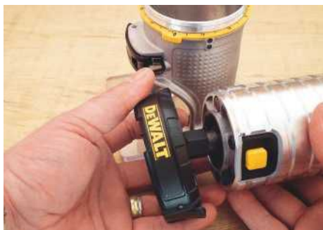
This collar screws onto the router body on a slow helix thread
