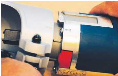
Align these arrows and twist the body in to fit the fixed and tilt bases
