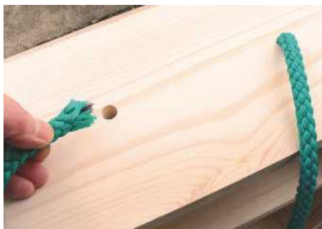
STEP 19. The handle is a piece of 12mm diameter polypropylene rope. Drill two holes in the top for it to pass through
