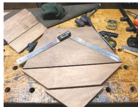
STEP 5. In order to maximise material, the top will be made from several glued-up boards
