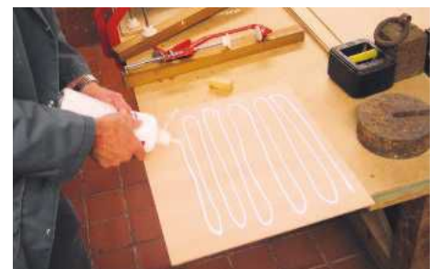
STEP 11. The two-part panels are then prepared and glued
