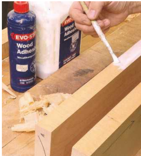
PIC 17. The planed edges are evenly brushed with a layer of white PVA-type adhesive
