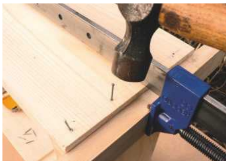
STEP 13. Pin the joints together, having pre-drilled holes first to prevent the wood splitting. Punch below the surface
