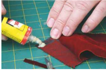
PIC 12. Rubber-based glues can be useful for highly flexible joints, such as fixing soft fabric linings in furniture
