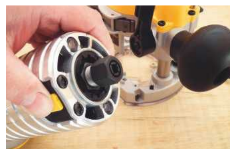
Multiple indexing points for the collet nut makes swapping cutters simple
