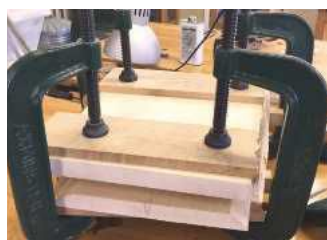
PIC 4. After initial planing the boards are cramped to keep them flat
