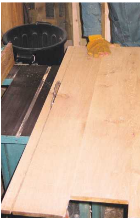
STEP 23. Cutting the top to width freehand on the bench saw
