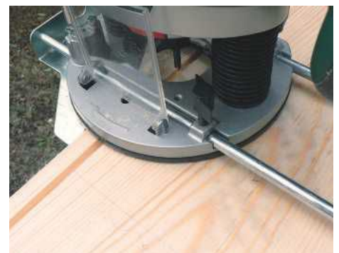
STEP 6. Rout a groove for the sliding lid, which is made from 6mm-thick MDF. Set this about 12mm down from the top edge
