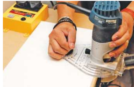
There's excellent support for the router with the tear-drop base fitted
