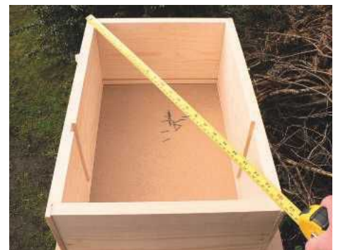
STEP 12. Check the carcass is square by measuring across the diagonals, adjusting cramps if necessary
