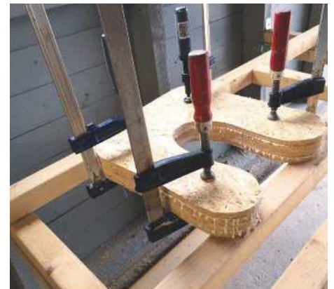
STEP 8. Glue them together, two pieces on top of the other, to give a total thickness of four pieces, before securing with several clamps
