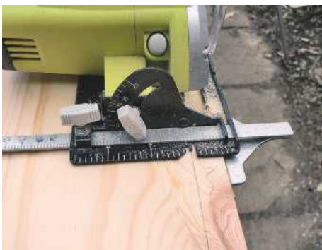
STEP 10. Saw the shelf to the same depth as the end panel cut earlier, cleaning up the edge with a bench plane
