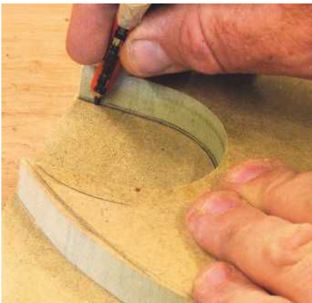
STEP 31. The shelf template seemed to work well so I marked out the position of the hole on eight pieces of MDF. The balloon shape is a perfect addition and doesn't over-balance the stand
