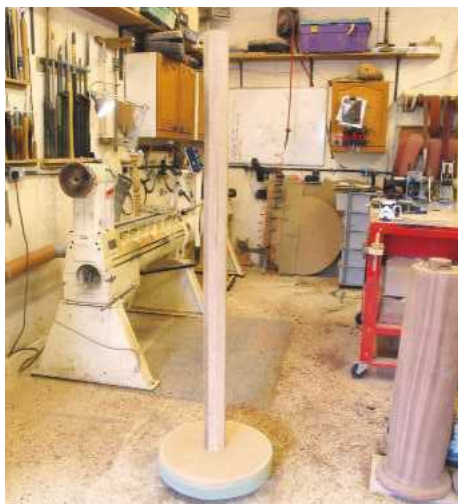
STEP 1. Oak and MDF: the stem is around 1,700mm long and 75 x 75mm. In hindsight, I could have done with it being a little bigger in section
