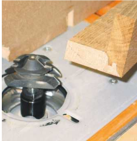
STEP 5. A multi-form router jointing cutter was used to make the leg joints
