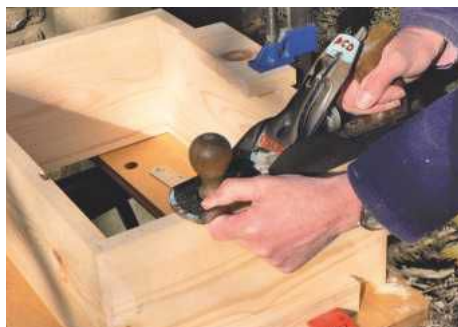
STEP 14. Plane excess end-grain, working from each side towards the centre, then plane the upper and lower edges
