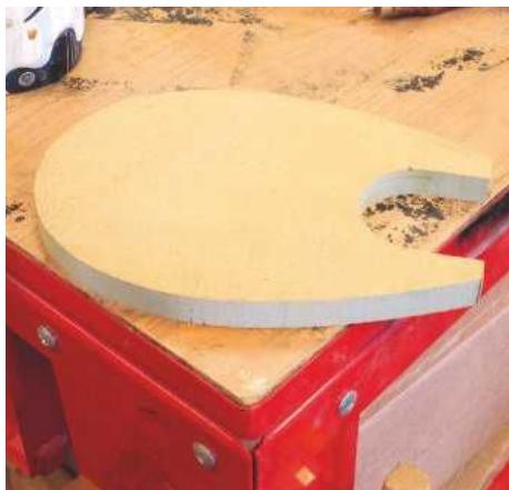
STEP 4. The shelves are made using 15mm MDF and I made a sample one to try in each slot. I could have used plywood or even real timber, but as they are going to be sprayed, MDF is fine
