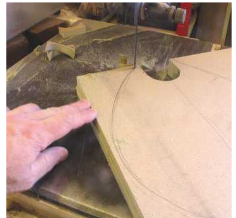
STEP 33. Carefully cut out the shape using the bandsaw. I decided to do this freehand as I quite like the fact that they're not symmetrical. If the stand is perfect, then people may not look at the turnings displayed on it
