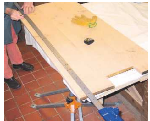
STEP 22. A long straightedge is handy for marking the top's finished size
