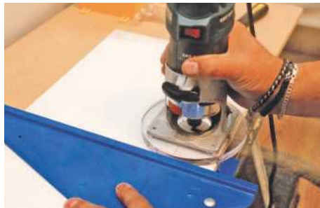
The round base takes guidebushes and is useful against straight edges
