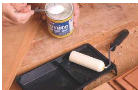
PIC 5. Glues made from powdered synthetic resin are good for spreading over large areas
