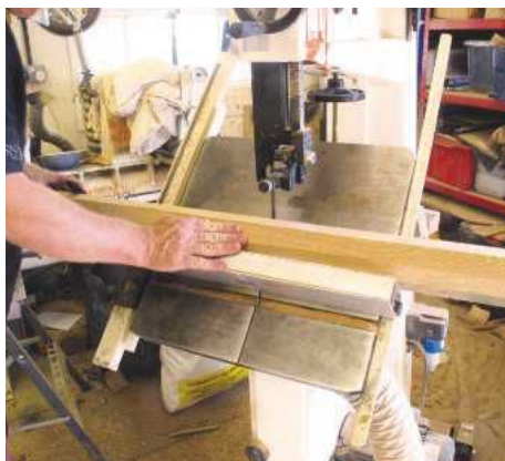
STEP 2. Turning a piece this long to round, straight from the square, will cause problems so I am taking the corners off on the bandsaw. When I bought my bandsaw many years ago, the speed at which I could tilt the table was a major factor in deciding which one to buy
