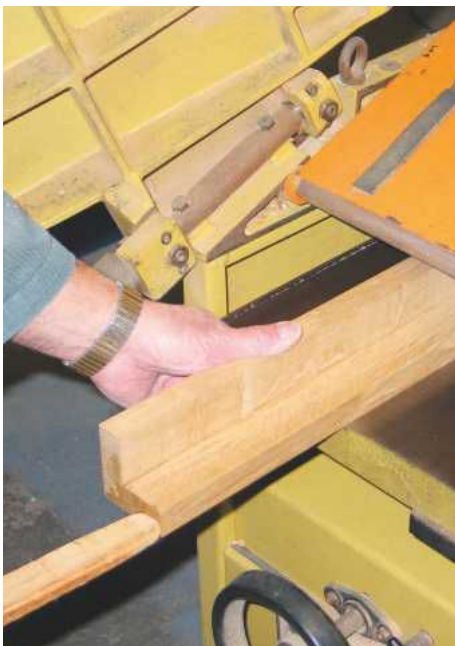
STEP 7. The legs are planed to their finished size along with the rest of the components
