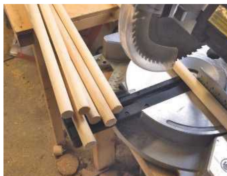
STEP 12. Next, cut the dowels to length using a mitre saw
