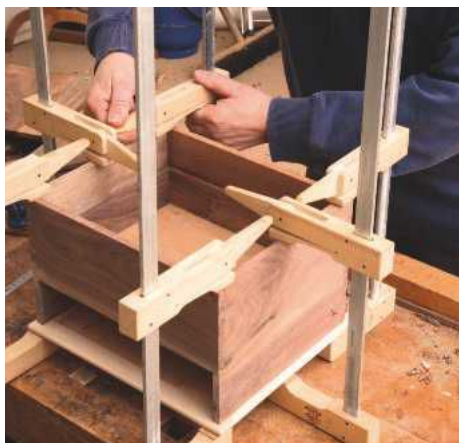
PIC 25. Sometimes a large number of clamps is necessary to pull evenly in both directions
