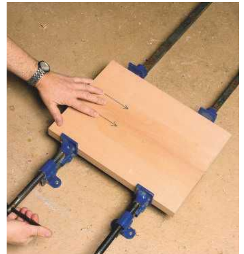
PIC 18. The boards are clamped edge-to-edge while the glue sets
