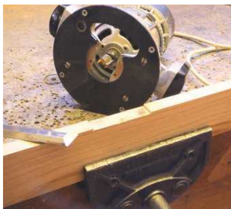
STEP 25. Rout out the bulk of the waste and finish by hand
