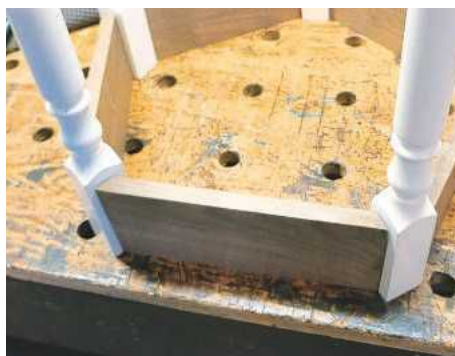
STEP 4. Test fitting the side skirts and estimating the size before cutting Domino joints
