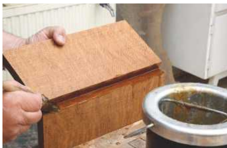
PIC 19. Traditional edge joints made with hide glue need to be quickly worked and do not require clamps
