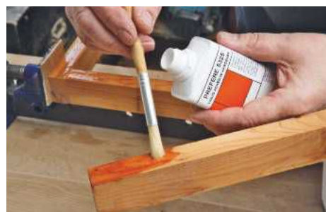
PIC 6. Resins with a separate liquid hardener are immensely strong for close-fitting joints where a long open time is needed
