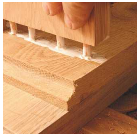
PIC 21. Dowels are versatile components for making simple glued-up joints without specialised knowledge or equipment
