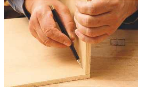
PIC 13. A screwed and glued joint is started by marking the position of one board against the other with a pencil line
