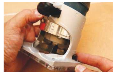
A fine adjustment wheel on the tilt and fixed-base read against the etched scale
