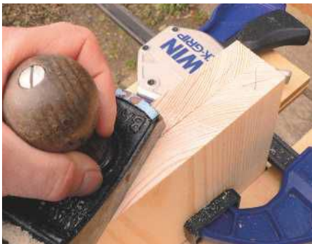
STEP 4. Cramp the two end boards together and place in a vice or Workmate. Plane the end-grain and check for square
