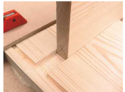
STEP 9. Make sure the shelf is a sliding fit in the housing. A tight joint will add strength to the box when glued
