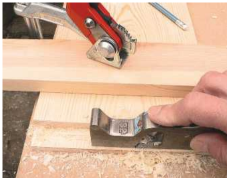
STEP 5. Cramp side panels down to a board and clean up rebates with a shoulder plane. Work from each end towards the centre
