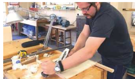
PIC 2. Jack planing to flatten the board
