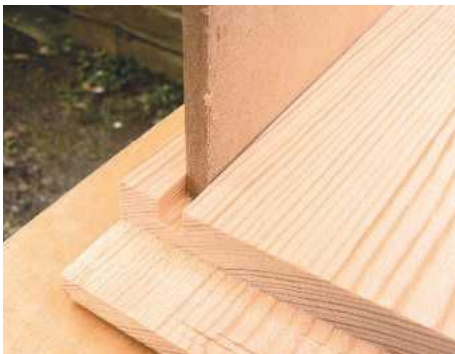
STEP 7. Check the MDF fits in the slot snugly and adjust the groove if necessary. Cut one end panel down so the lid slides over it
