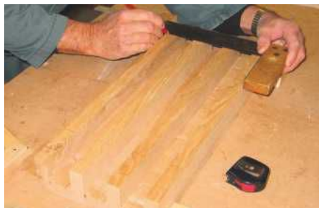
STEP 8. Marking the mortise holes on the legs
