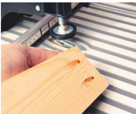
The resulting pockets are clean and uniform
