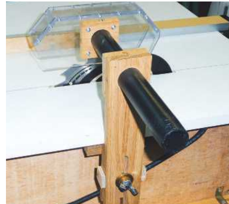
PIC 8. Height adjustment and extraction for the guard
