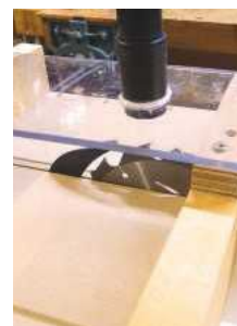
PIC 6. Cross-cut sled in place showing extraction and safety block on the rear
