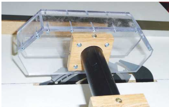
PIC 9. Close-up showing guard construction
