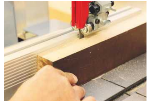
Thin repeat veneer cuts are accurate and consistent
