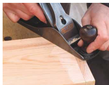
STEP 10. When the glue has dried, plane the end-grain flush at the top of both side panels
