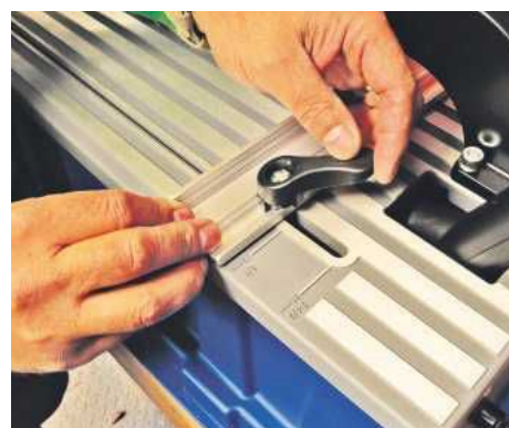
Common timber dimensions are marked to help set the fence
