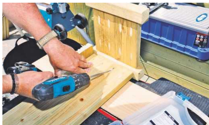
STEP 12. The long boards are now screwed to the end panels
