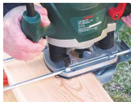
STEP 7. Rout rebates along rear edges for the matchboard. Rebates do not run full length on the side panels
