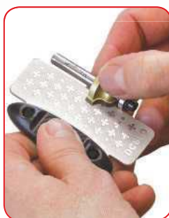
Specialist stone designed for router cutter sharpening.
