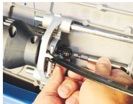
The drills are held in a sleeve chuck for quick changeover
