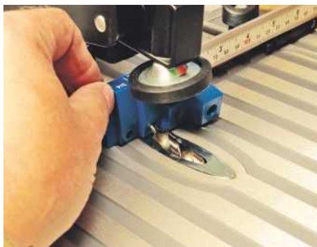
You set the drill depth against this setting block...
