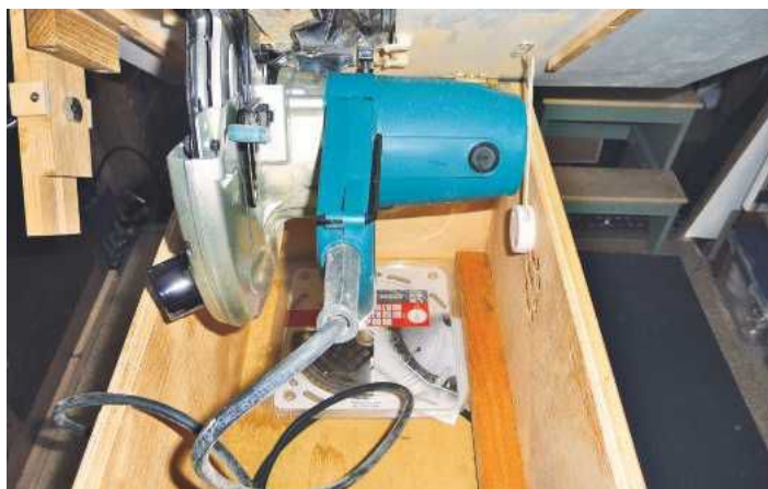
PIC 5. Inside of the box showing the stay and cable router
