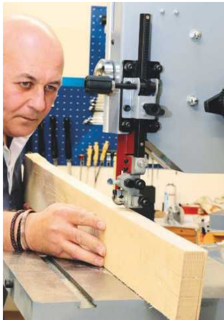
The saw is equally powerful for deep ripping of timber
