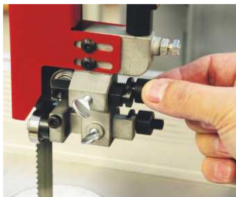
The upper guides are adjusted without the need for tools
