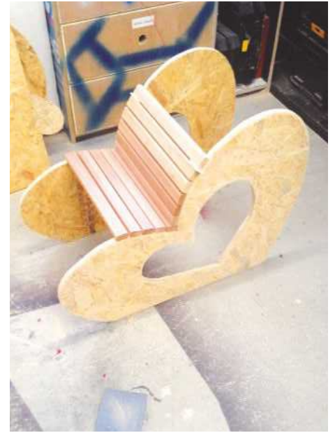
STEP 3. Take two OSB hearts and space them 400mm apart; you can then start nailing down the cedar ribs
