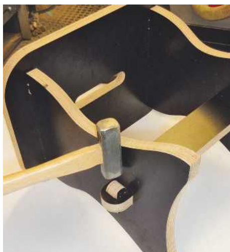
PIC 10. The tenons are tapped into position
