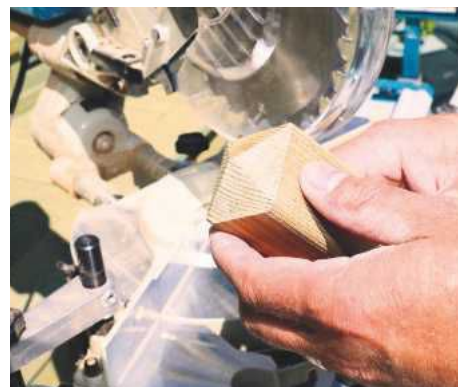
STEP 6. Once all four cuts are made, you should end up with a pointed top
