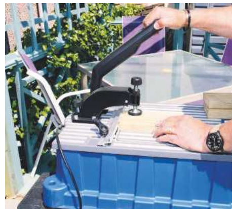
STEP 8. The pockets are made in pairs and applied to each piece
