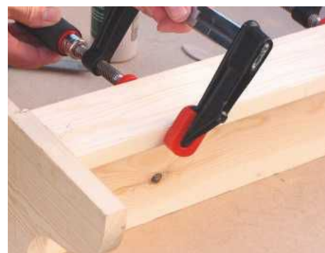
STEP 13. Upper and lower aprons are also fitted with biscuits. Sand the face sides before gluing in place
