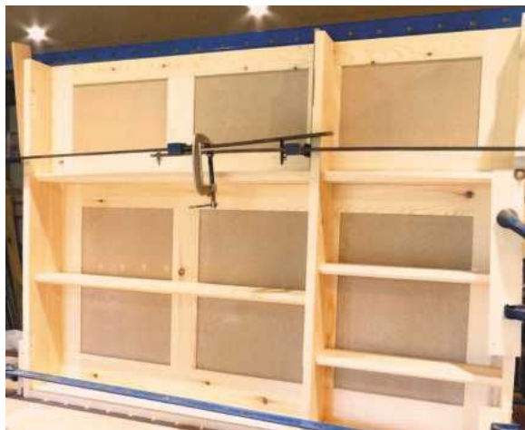
PIC 1. Where's another long clamp when you need it? With time ticking and the glue expanding, I had to act quickly. The little G clamp holds two sash clamps pinned together just enough to pull that left-hand side in tight
