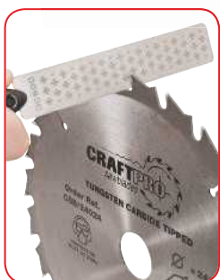
5" file with handle for sharpening sawblade teeth.
