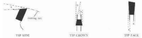
FIG 5. The supporting body of the cutting tip is 'relieved' or ground back (X) so that only the cutting edge itself makes work contact
