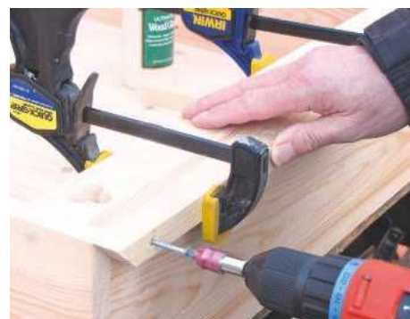
STEP 16. Mitre, glue and screw 20 x 20mm blocks around the top of the carcass to support the coving
