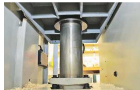
A substantial central ram controls the rise and fall of the table
