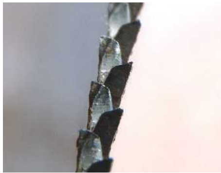
PIC 13. Disposable saws are rather coarse for fine furniture making and because of the hardening the teeth cannot be adjusted
