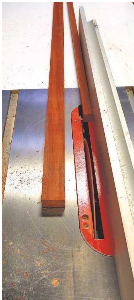
STEP 4. Placing the previously jointed edge against the fence, cut strips of random width
