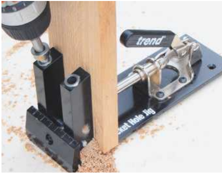
STEP 5. Using a pocket hole jig such as the one shown here, drill both ends of the top and bottom rails for the fixing screws
