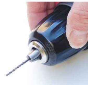
The triple jaws will grip a 2mm bit but nothing smaller
