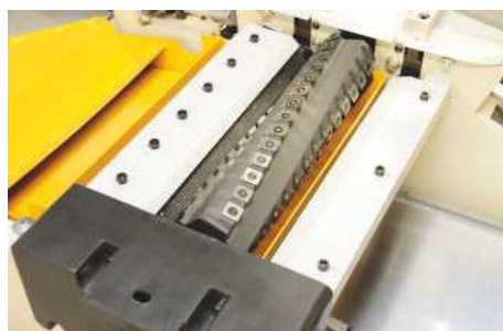
Individual cutters are arranged in a slow spiral to give a sheer cut
