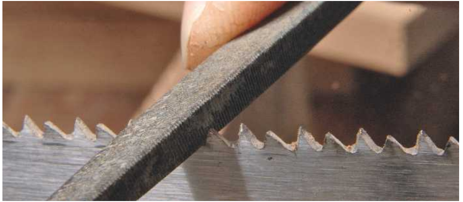
PIC 11. A traditional saw can be sharpened with a three-cornered Swiss file, being careful to maintain the angle and height of each tooth
