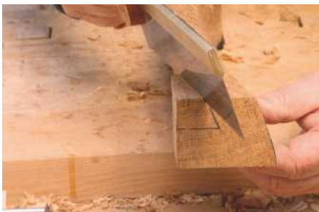
PIC 4. Tight, awkward cuts may require the saw to be tilted sideways as well as cutting down to an angled baseline. This takes a good deal of concentration to keep both angles in control
