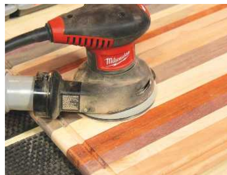
STEP 12. Sand the board using a random orbital palm sander and work through the grits
