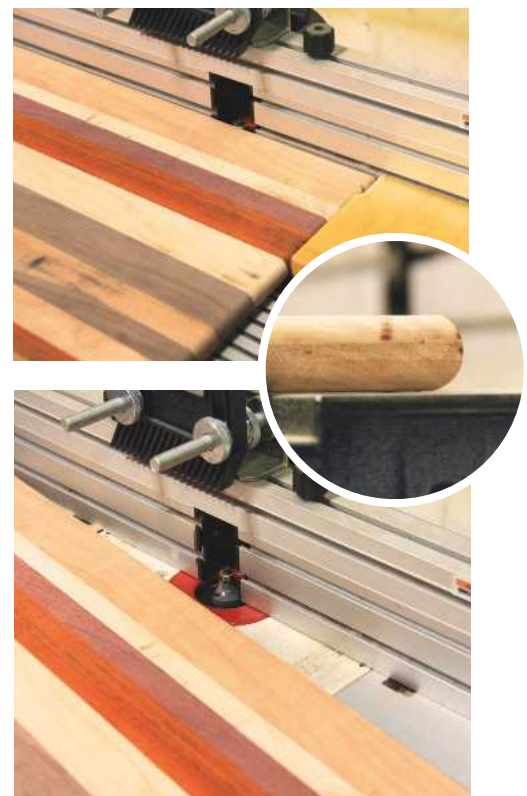
STEP 10. Round over the top and bottom edges with a roundover bit fitted in the router table
