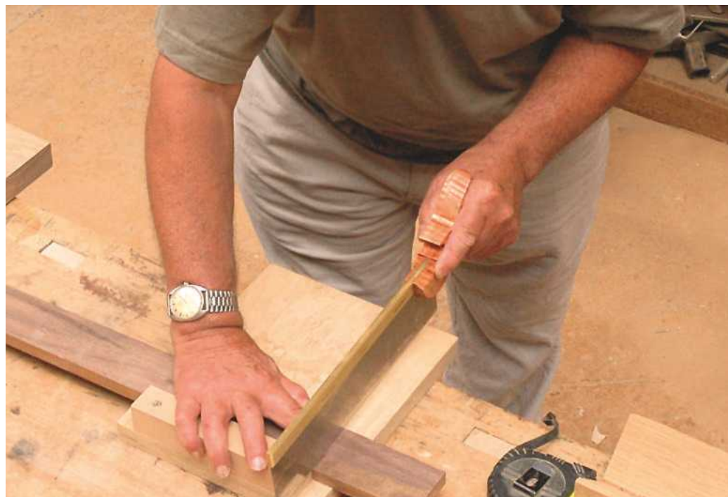
PIC 2. Here a left-handed furniture maker uses a bench hook to guide a wide saw cut. The hook is designed to be used on either side while the saw is held in the left hand and the right fingers are used to guide the start of the cut
