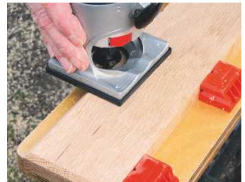
STEP 10. Rout 5mm chamfers around the lower ends of the stiles and along the top shelf
