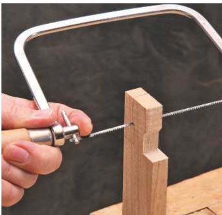
PIC 19. Frame saw blades can be guided to follow tight curved or complex joints like this or on decorating features
