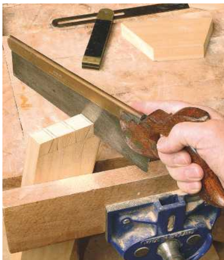
PIC 8. Sometimes it can be helpful with complex joints to clamp the wood at an angle so the saw cut remains vertical
