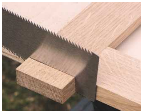
STEP 12. Once the glue has dried, saw off any protruding horns and trim flush with the aid of a bench plane
