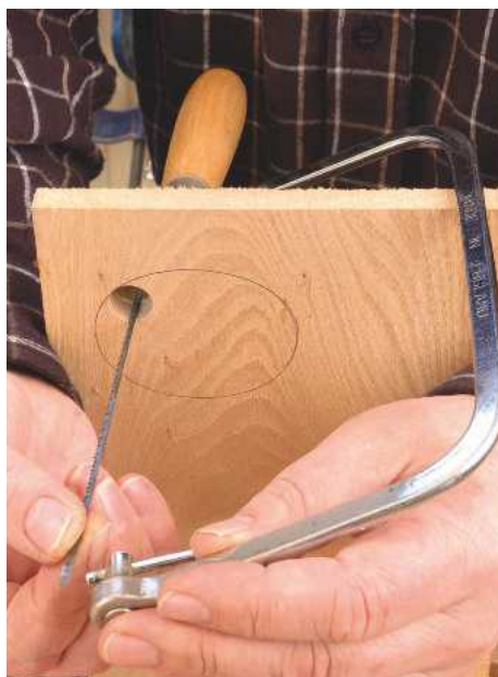
PIC 17. The blade can be removed from a frame saw to pass it through a drilled hole
