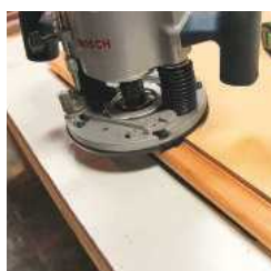
STEP 11. While there are many ways to cut a juice groove, the easiest way is to fit the router with a simple pattern bushing and follow a rectangular piece of masonite cut to size as a template
