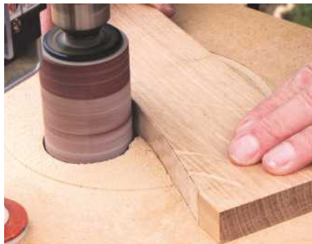
STEP 9. Saw the curve just on the waste side of the line and clean it up on a sanding drum
