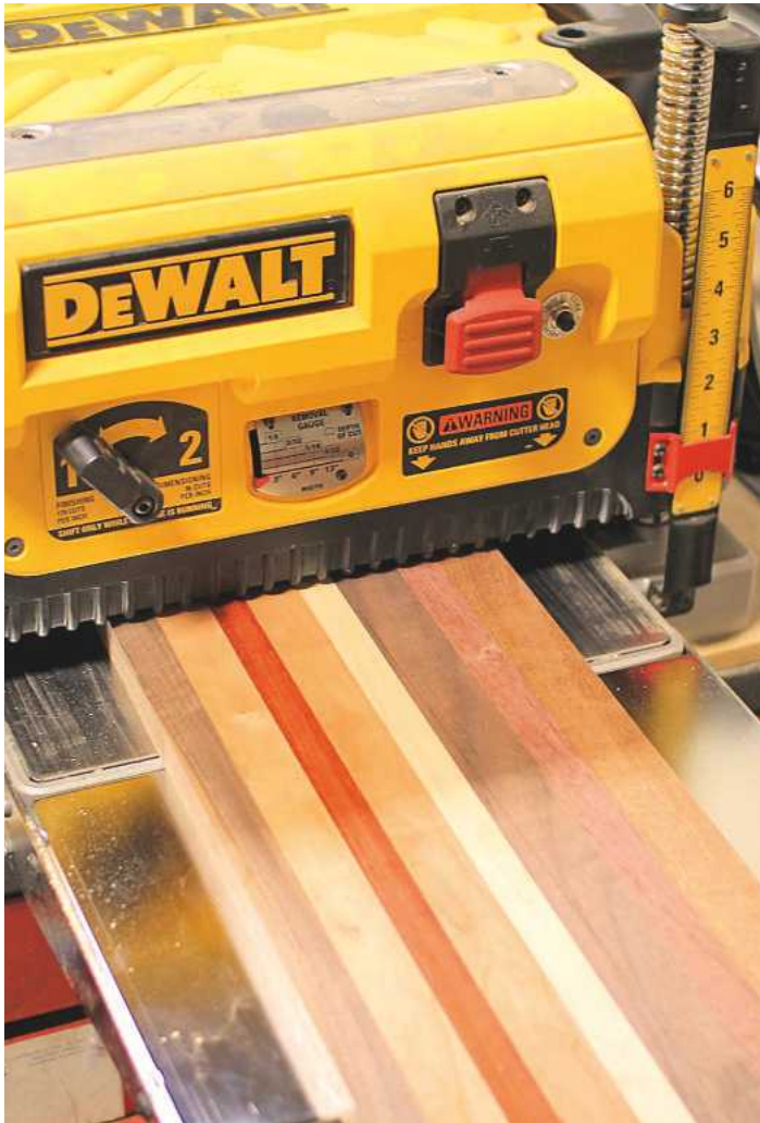
STEP 7. Run the two boards through the planer, taking off as little as possible on each of the faces
