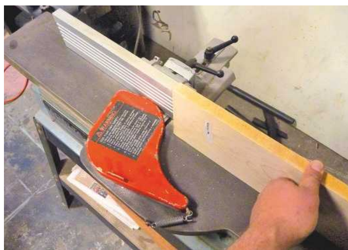
STEP 2. Use a jointer to prepare one edge; this creates a straight edge, which you can use later to push against the table saw fence to make a straight cut
