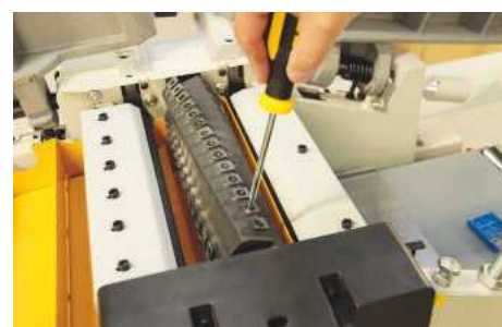
Cutters are self-setting and swapped with a Torx driver
