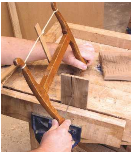
PIC 16. Frame saws are the traditional cabinetmaker's tool for making curved saw cuts. Moving on from this rather crude looking string-tensioned wooden device, steel framed coping saws and fine fret saws will fit into places no other saw can reach
