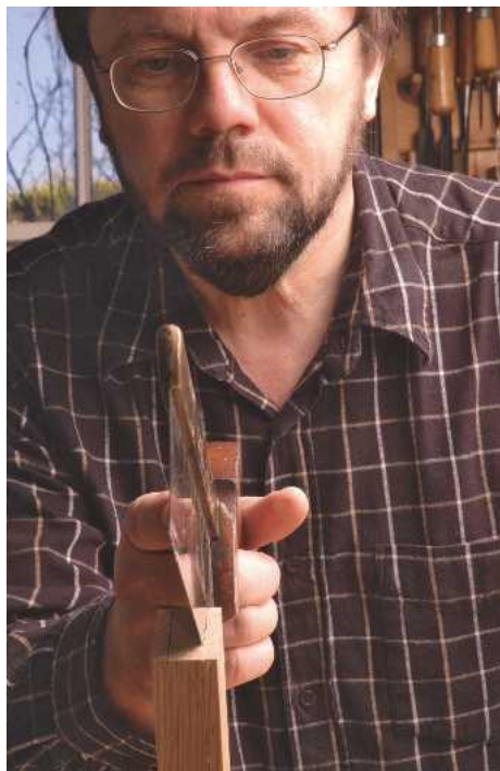
PIC 5. By keeping the head centred with one eye above either side of the blade, you can watch that the saw does not deviate from a straight line
