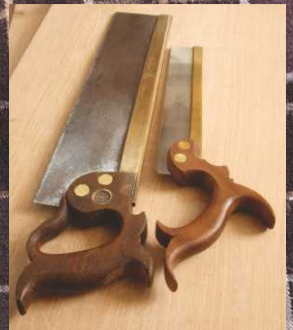
These two 'back saws' have heavy gauge brass backs on top of their fine steel blades. On the left is a 'tenon saw', on the right a 'dovetail saw'
