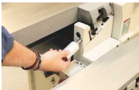
The surfacer depth of cut adjuster is at the back of the machine
