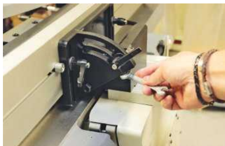
Adjustments can be made to the fence stops for 90 and 45° positions
