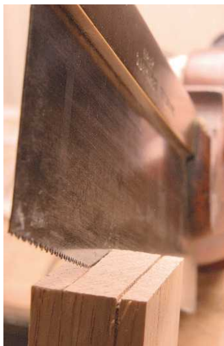
PIC 6. When making deep cuts, such as for this joint, the saw blade is continuously guided to stay tight against the waste side of the marked line
