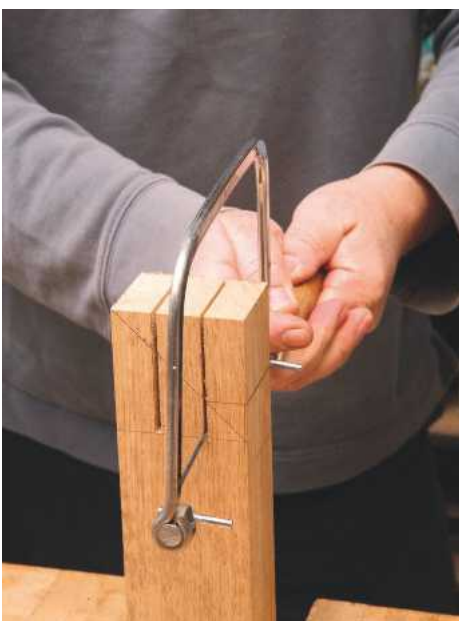
PIC 20. Even on simple joints the coping saw provides a useful way of removing chunks of waste
