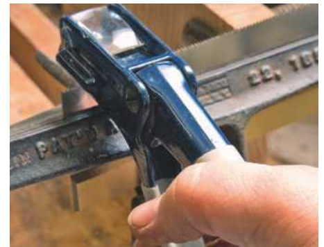
PIC 14. The saw-set is a tool designed to keep the teeth slightly bent over to alternate sides; this prevents the blade from jamming in its own cut
