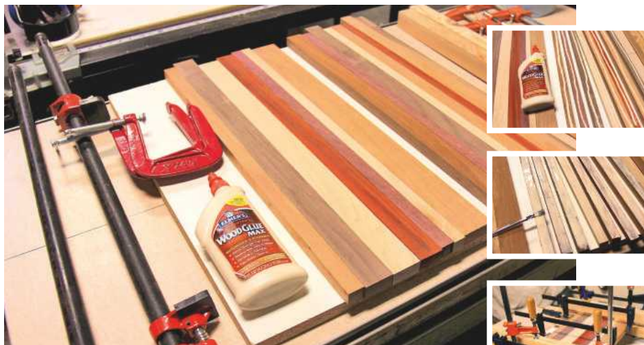
STEP 6. Separating your cutting board strips into two groups, no wider than the maximum capacity of your planer, glue the strips together
