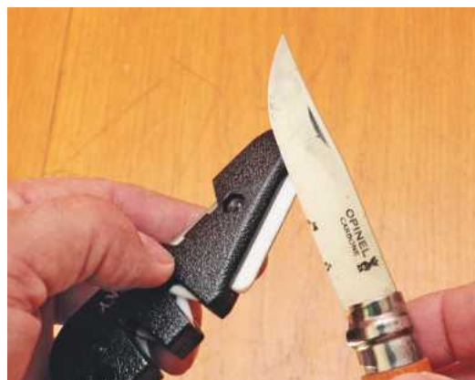
The ceramic rod keeps a fine cutting edge on the blades
