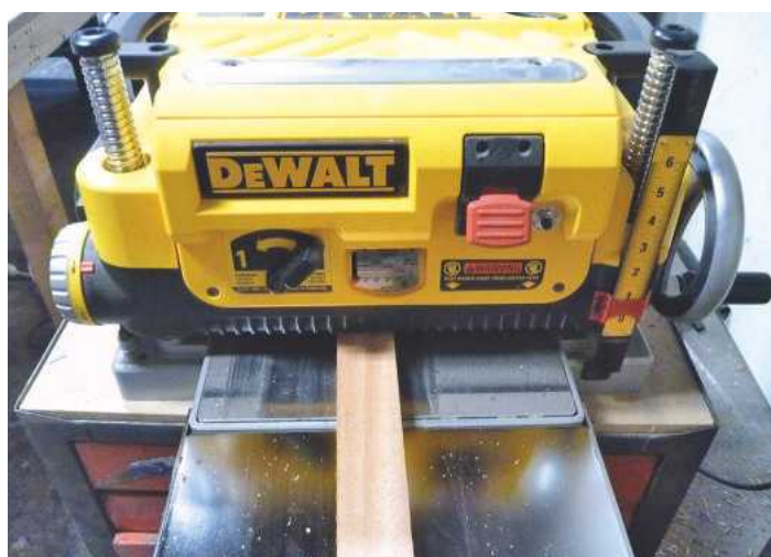
STEP 3. Take the already dimensioned face and place it face down onto your planer bed, then run the piece of wood through the planer
