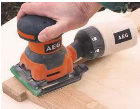
STEP 14. Check stiles and rails are flat with a straightedge, then sand the frame
