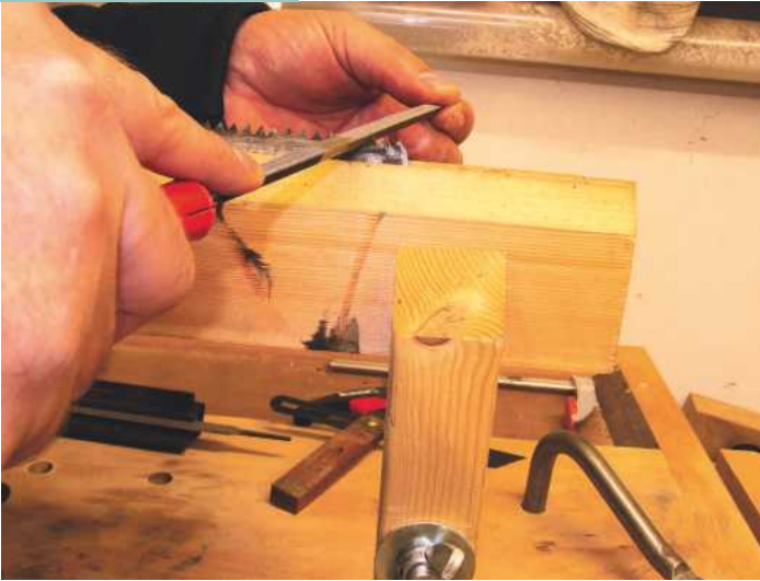
⬆ This photo demonstrates the way most saws are filed nowadays, with the file at 90° to the blade but skewed to give a crosscut profile
