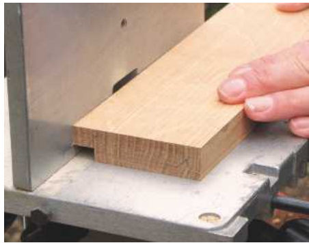
STEP 6. It's easiest to cut the 8mm deep rebates for the glass with a router mounted in a table
