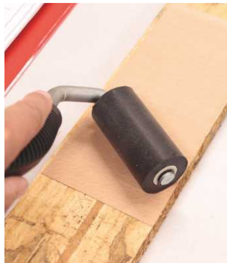
LEFT: ... and once on the substrate, pressure is applied with a 'J' roller for a good bond
