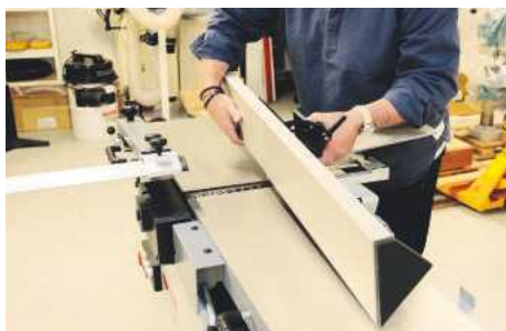
You have to remove the fence to use the thicknesser function
