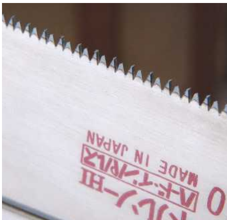
PIC 15. The teeth are hardened to keep their sharpness while making them brittle and the blade disposable
