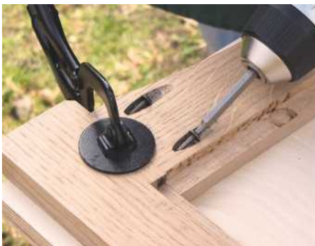
STEP 11. Brush on PVA glue, cramp to a flat surface and screw rails and stiles together
