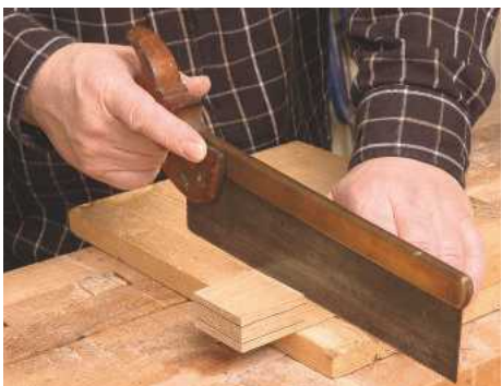
PIC 7. Here the wood is held down on a simple guide known as a bench hook while making a wide saw cut for the shoulder of a joint
