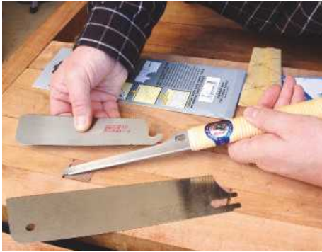
PIC 10. Japanese back saws have a different construction from European and American ones. The blade is hooked into a slotted back, which has a wooden handle bound on
