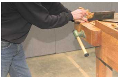
PIC 3. Once the cut is under way, the furniture maker stands back from the bench, providing room for the arm to sweep back and forth in a straight line
