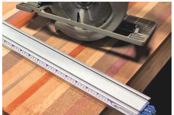
STEP 9. Alternatively, you can use a circular saw and straightedge instead of a sliding mitre saw to cut off the uneven edge
