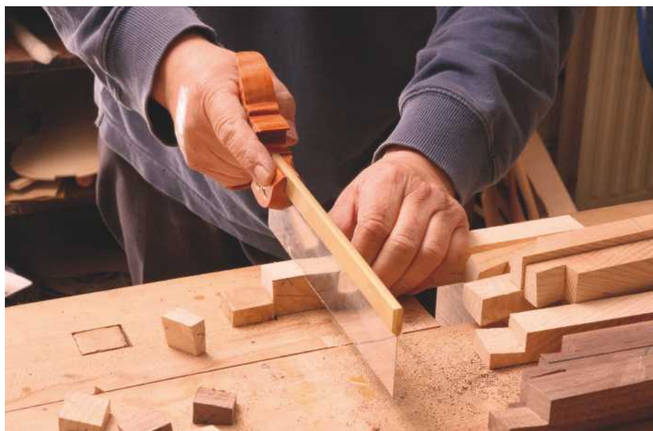
PIC 21. Where a large number of similar saw cuts need to be made, lining them up as a batch saves time and improves accuracy
