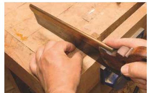
PIC 1. The way a saw cut starts is most important – it needs to be clean without any judder, in the right position and at the correct angle
