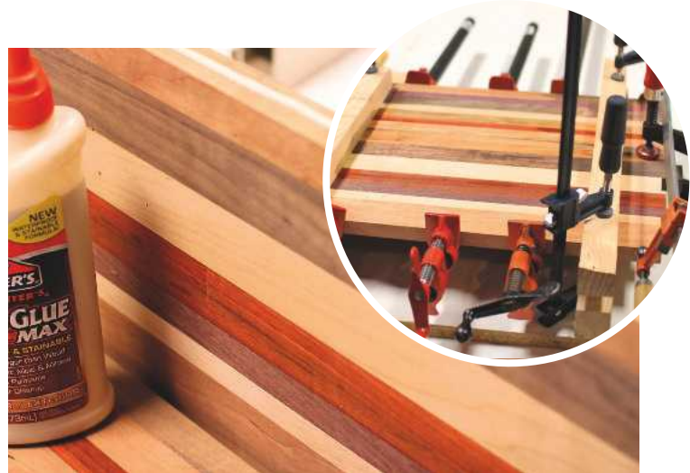
STEP 8. Glue the two boards together and clamp up overnight using cauls to keep everything aligned
