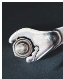
In its working position the spanner sits around the nut to apply pressure
