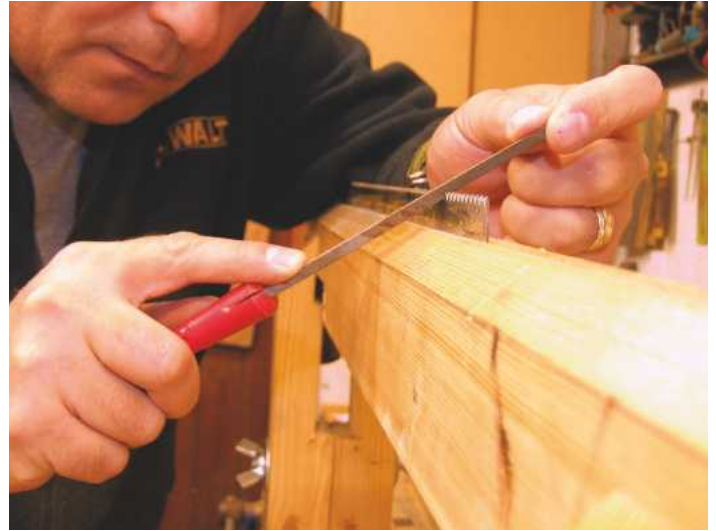
⬆ Here the file handle is dropped to file uphill and make a needlepoint tooth for a cleaner cut, but this involves more work and tends to blunt easier when it hits harder knots, etc.
