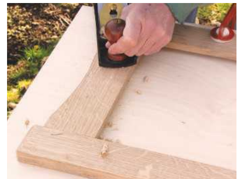
STEP 13. True up the surface of the frame, checking for grain direction. If the wood tears, switch to using a cabinet scraper
