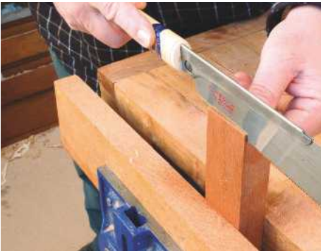
PIC 12. The Japanese back saw blade is thin and very suitable for sawing fine joint details
