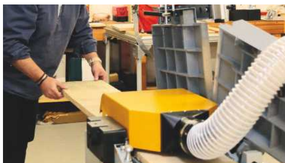
With the beds up there's excellent access to the thicknesser
