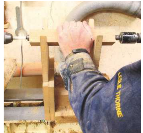
▲ Pic.3 Due to regulations, the candle can't come in direct contact with the timber. The brass candle cup requires a 22mm hole – 'V' blocks will allow you to drill an accurate hole, just wind the wood onto the spinning drill
