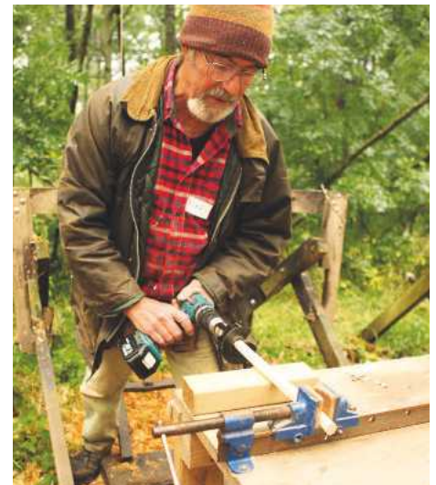
The Veritas tenon cutter in action
