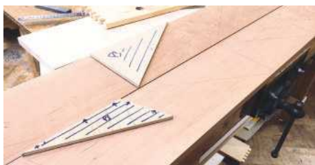
▲ Pic.9 I then re-planed my timber after having given it some time to settle. It was then on to marking out the cutting list on the planed timber for the carcass, using the templates I'd prepared and finally, cutting the components using the bandsaw
