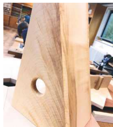
▲ Pic.36 The drawer handle is a hole. There is also a smaller hole in the back panel to allow the drawer to open freely and not get stuck due to vacuum. I thought the figuring of the rippled sycamore worked really well here. I then used a pillar drill and a hand-held router to round off the edges
