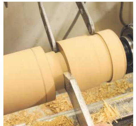
▲ Pic.27 In the past, before I had these fingers, I had to have lots of callipers set to different sizes. The worst thing that happened was when you picked the wrong one up!
