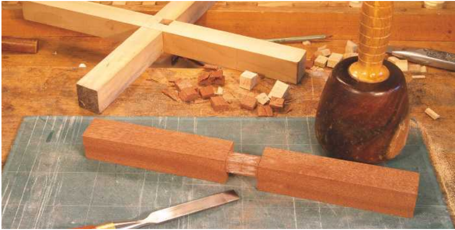
▲ Pic.13 The waste chopped out leaving the chalked squares
