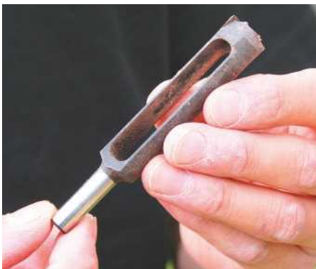
▲ Pic.12 To hide the visible pocket holes and screws on the underside of the cover, I used a pocket hole plug cutter to cut some plugs
