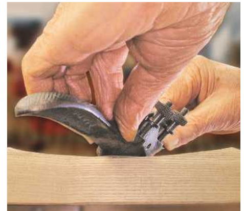
▲ Pic.7 The metal spokeshave resembles a very short plane
