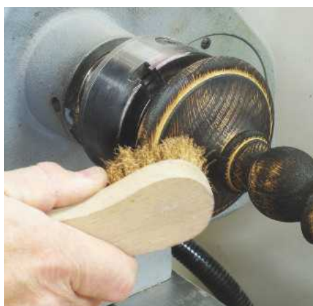
▲ Pic.32 The use of a liming or soft brass brush will remove all the leftover carbon deposits. I have two of these brushes so I don't mind one getting contaminated with black
