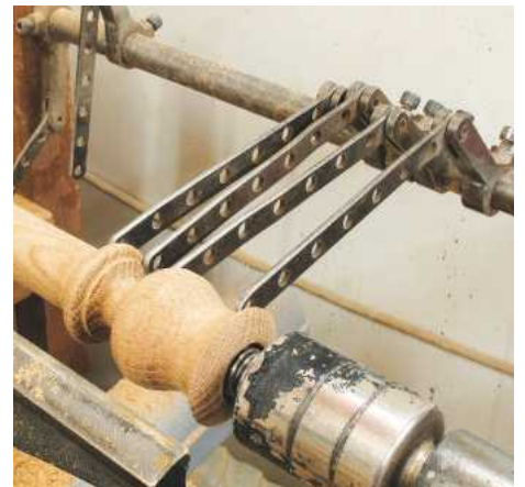
▲ Pic.24 When the first one is finished set the copying fingers up onto the major sizes; this makes the whole turning process much more efficient. Just keep removing wood until the fingers fall off
