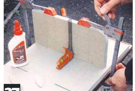
27 Apply glue to the edges and insert biscuits. Cramp each shelf for at least an hour, checking they're square to the panel
