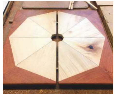
▲ Pic.43 As a standard, when oiling, I massage the oil into the timber rather than applying lots of it and having to dry off the residue after a while. I was really pleased with the end result
