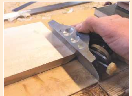
▲ Pic.26 Once dry, I laid the structure onto the carcass and marked out the corner angles, making sure the structure was precisely centred. Once I had marked it off, I began to place the ends
