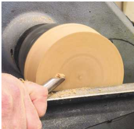
▲ Pic.4 Now the hole is drilled you're ready to start turning. The base is held on a screw chuck. True up the bottom with a pull cut or use a scraper to remove any ridges left by the gouge
