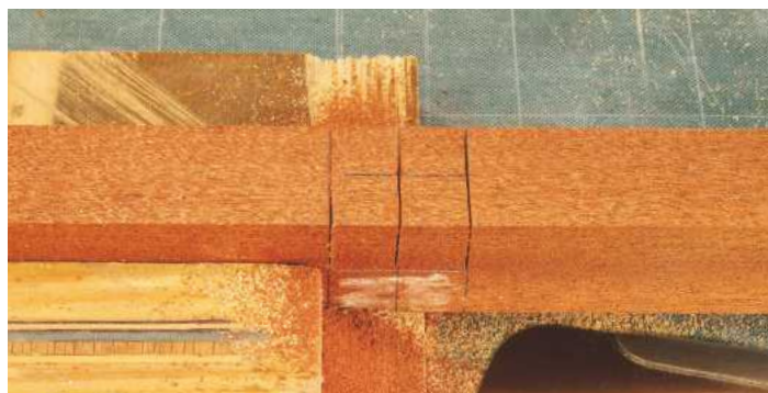
▲ Pic.12 Sawing the third stick down to the chalked squares
