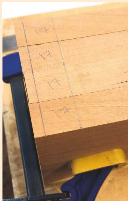
▲ Pic.19 It was now on to cutting the 'SunRay Dovetails'. I marked out the shoulders on all four pieces, measuring from the centre of the panel where the components meet, as this was where the carcass and the door panels would have to line up when assembled
