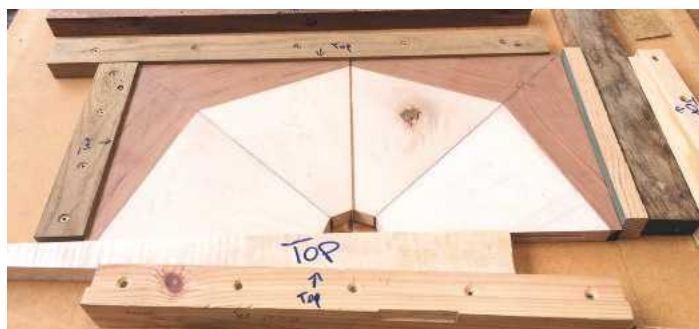
▲ Pic.16 To achieve absolute symmetry, I imitated the gap between the two door panels by laminating a strip of cherry veneer in between every eighth. Once dried and trimmed, the veneer looked very neat
