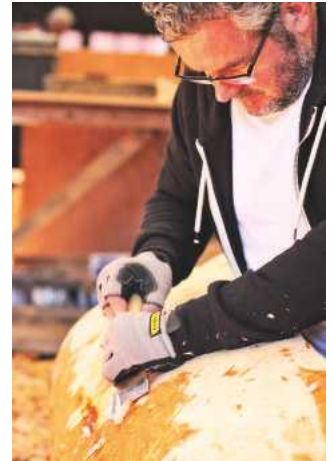
▲ Smoothing with a chisel
