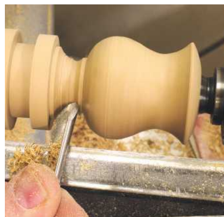
▲ Pic.18 Let the shaping begin. Always design a piece within your capabilities: a simple design turned well is always better than an ornate shape turned badly. Keep your detailing crisp and smooth
