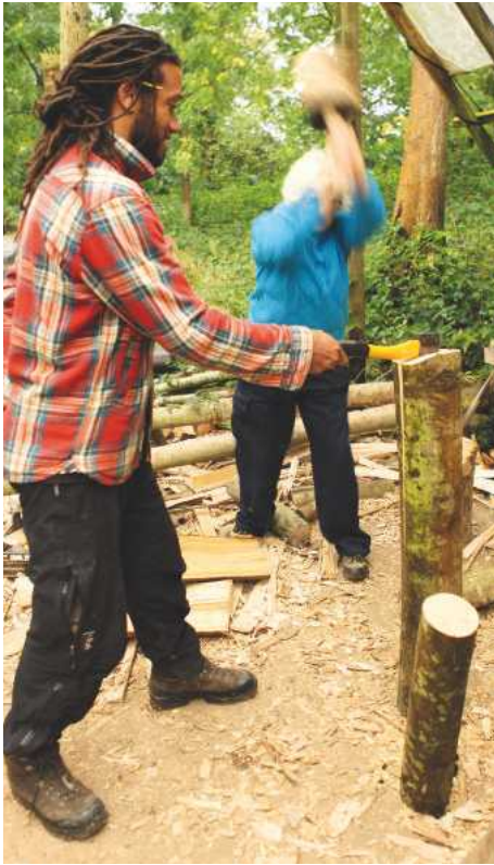
A student making the beginning cut to insert the froe to cleave the log
