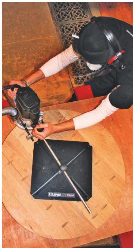
▲ Pic.14 Routing the perfect circle using Trend's ellipse and circle cutting jig
