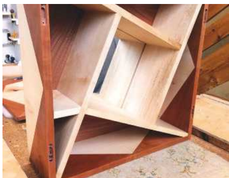
▲ Pic.44 To fit the star I just dabbed a bit of glue into the corners, since it just needed to be held in place
