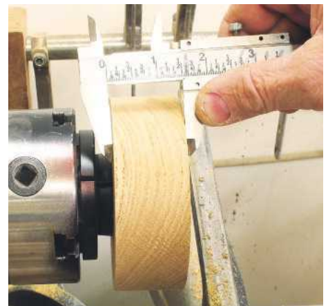
▲ Pic.9 To achieve good copies the sticks will need to be the same height. Measure the thickness of the base so that measurement can be transferred to the other one(s)
