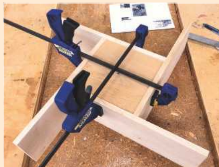
▲ Pic.25 It was then time to shoot down the doors to make them fit. To glue and clamp the inner square structure, I had to build a box to clamp around it. I used biscuits to join them, then dry-clamped and glued everything up
