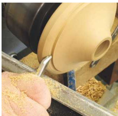
▲ Pic.14 Rounding over the bottom section of the base will be aesthetically pleasing. The grain of the timber is going in a different direction than spindle work so the tool works up the bead rather than down; this will give you a superior finish
