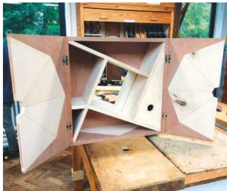
▲ Pic.41 I decided to assemble it, then fitted the back panel and the hanging plates, before moving on to shooting the doors to size. I sanded them followed by the whole cabinet
