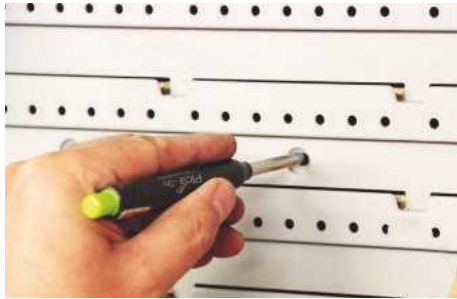
▲ The extending lead also proves useful for marking through fittings for hole positions
