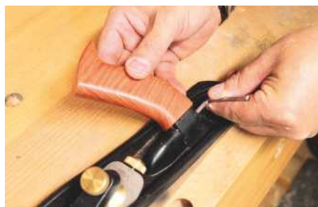
▲ You can pivot the rear tote to gain a better position when doing bevel work
