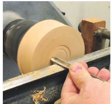
▲ Pic.6 To be able to turn the top detail you need a way of turning it around. Turn a dovetail chucking recess in the bottom to suit your chuck. If you make this 3mm deep, it can be filled with a piece of hardboard before you apply the baize
