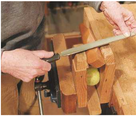
▲ Pic.4 The carver's chop: handy for holding irregularly shaped workpieces...
