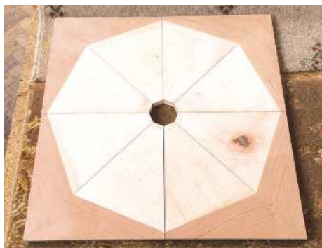
▲ Pic.18 Here you can see the four quarters all joined together to make a whole. My teacher, warned me about solid wood movement. I tried to change the structure, but it wouldn't work, so I stubbornly went for what I had in mind
