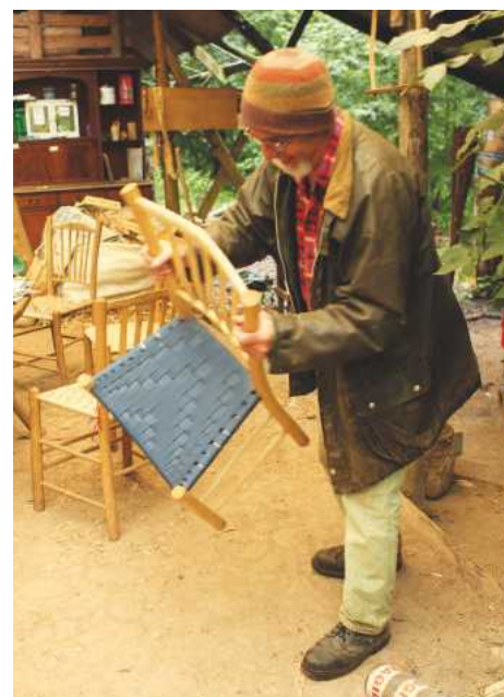
Mike Abbott demonstrating the 'bounce' quality test
