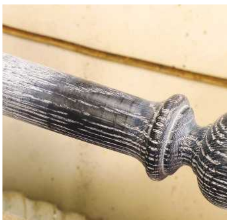
▲ Pic.34 Using a shoe brush with a little paste wax on, remove the excess liming wax. Work across the grain; this will stop you from removing too much of the white
