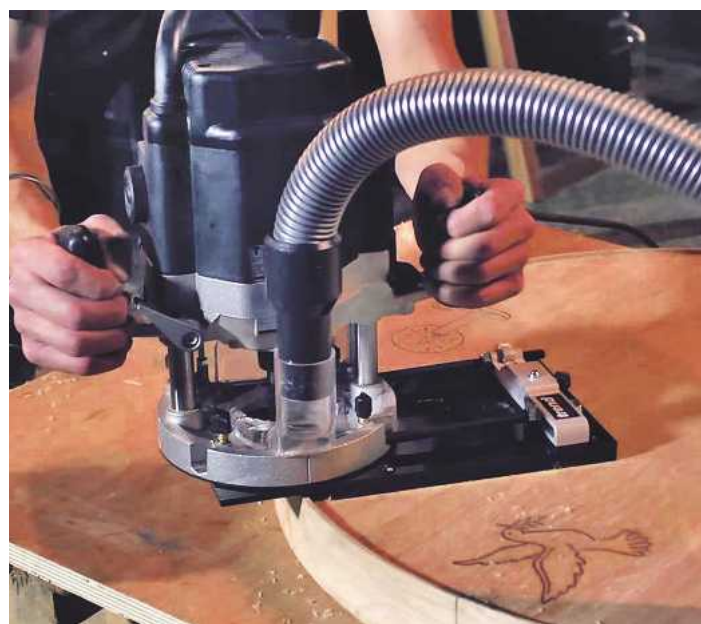
▲ Pic.18 Creating a high quality finish on the lath using Trend's multifunctional CRB combination router base
