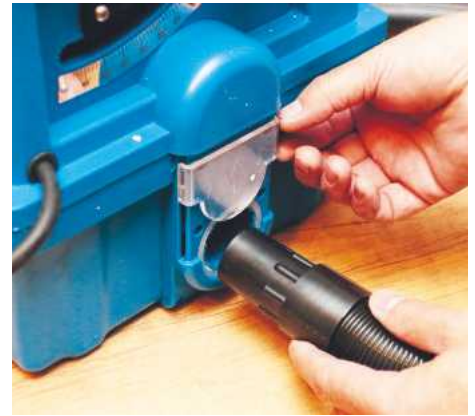
▲ Lift this cover and the supplied hose can be used for general cleaning
