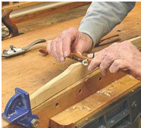
▲ Pic.8 I held the rail between cramp heads, while the 'shave was pulled
