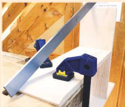
▲ Pic.27 Another way to check if the angles were correct was to line up every corner with the straightedge
