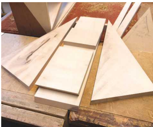
▲ Pic.34 I then moved on to making the triangular drawer. Originally I wanted to combine timber types for the drawer but I ran out of cherry, although this didn't matter because it looked better in sycamore anyway
