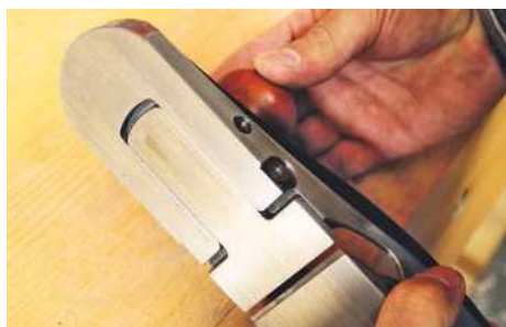
▲ The enclosed mouth slides freely. An adjustable stop restricts the opening
