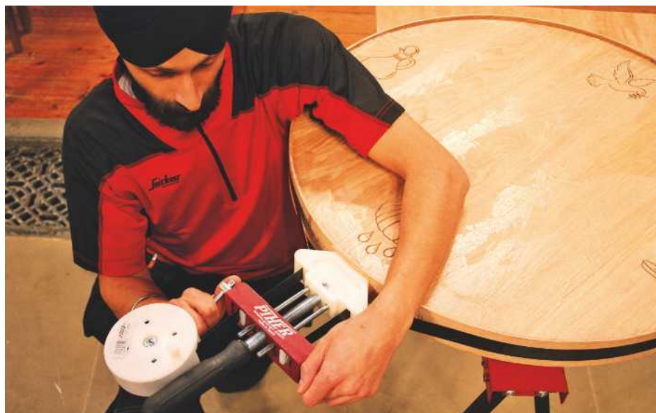
▲ Pic.16 Securing the lath in place using a band clamp
