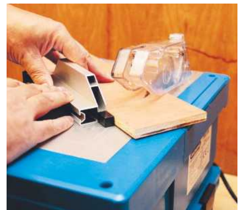
▲ The cross-cut fence on the TSV150 is basic but works as it should
