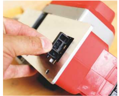
▲ The parking shoe can be locked in flush if not required
