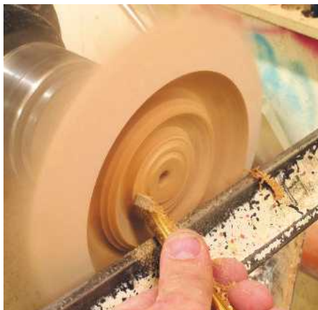
▲ Pic.26 Approach the hollowing out just as you would when working on a normal bowl. Work the shape down in steps with the majority of the cutting coming from larger to smaller diameter
