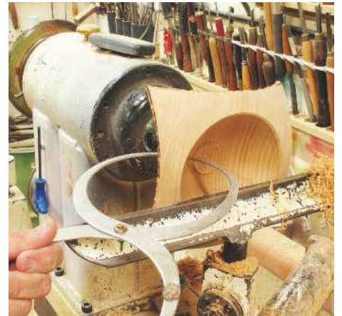
▲ Pic.30 Take the wall thickness down to a fairly even 5mm. Using hour glass callipers will allow you to measure this easily as they basically repeat on the end nearest you the thickness of the bowl
