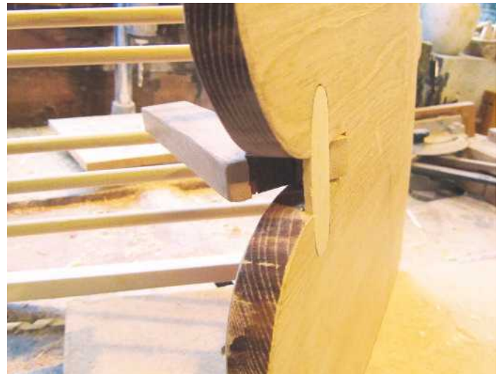
▲ Pic.9 The post supporting the tray was prevented from swivelling beyond the vertical by gluing a slim pine stop into a routed recess on the underside of the seat
