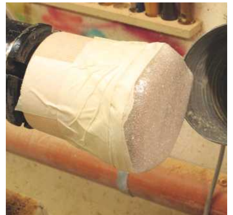
▲ Pic.33 The bowl now needs to be remounted to enable you to remove the marks left by the chuck. A dolly made from a piece of wood covered in bubble wrap and secured with masking tape will act as a friction chuck
