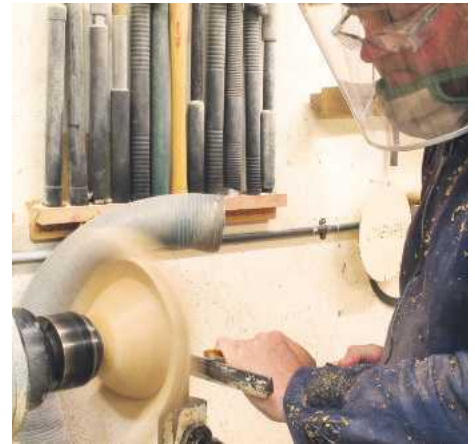
▲ Pic.21 It's absolutely imperative that you wear personal protection equipment when turning, especially on pieces such as this. Place a firm grip on the tool and make sure your hand is always behind the toolrest
