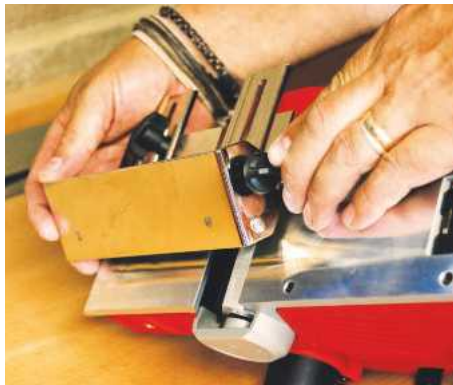
▲ The fence is a great addition and can tilt for angled work
