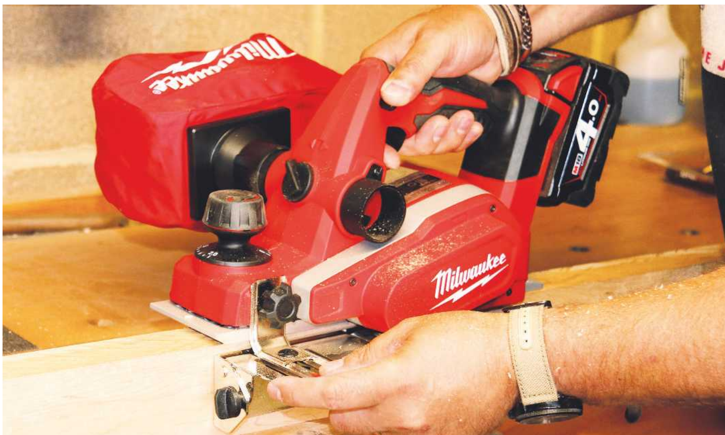
▲ Using the fence helps support the planer on edge work
