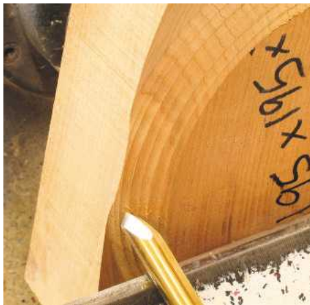
▲ Pic.5 The shape will need to be worked in two ways, hence the need for the long-grind bowl gouge. Work the tool in from left to right to form the shape on the wings
