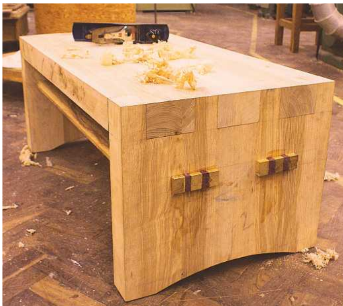
▲ Pic.6 The tenons were left over-size...
