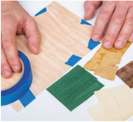
▲ Pic.1 Once you have made a line drawing of your intended marquetry image and glued it down, tape the background veneer onto another piece of cardstock
