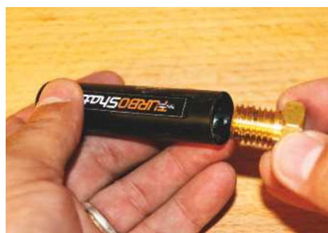
▲ This brass adaptor is supplied for altering the thread diameter
