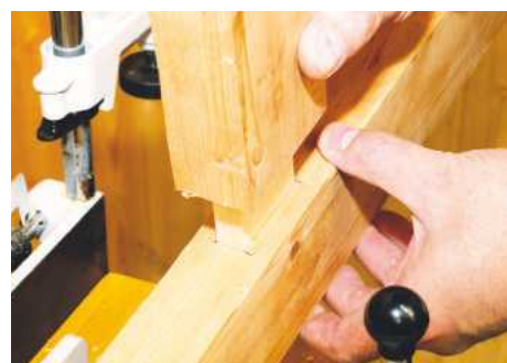
▲ The resulting mortises are clean and square
