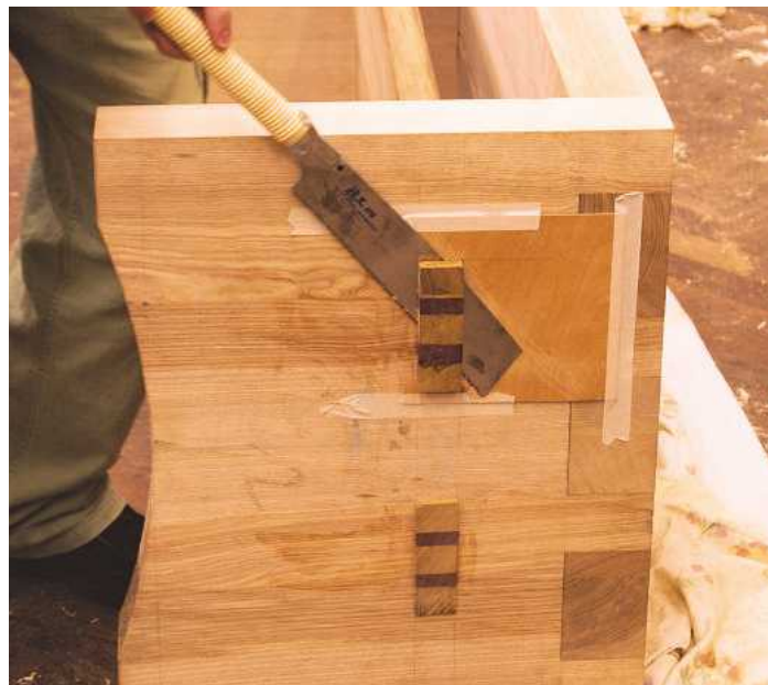
▲ Pic.7...and cut flush with a Japanese saw
