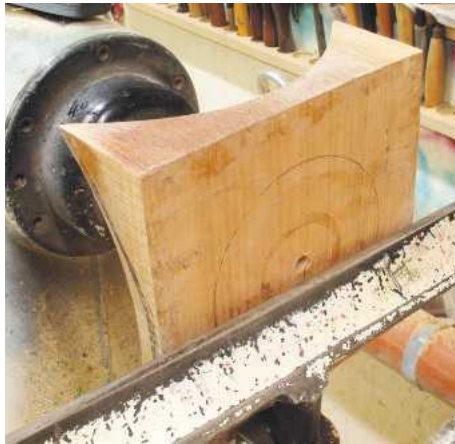
▲ Pic.20 Next, mount the bowl in the chuck jaws. Mark the diameter of the bowl and position the toolrest so it is straight across the front – this acts as a guard
