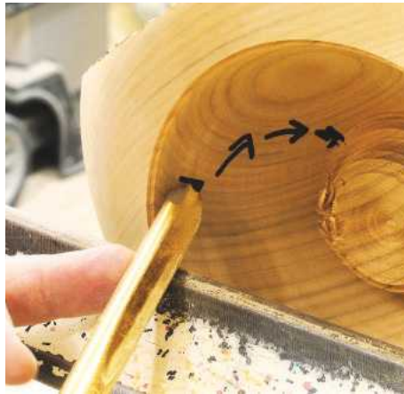
▲ Pic.29 Keeping the bevel in contact with the wood requires the tool to be passed through the wood in this way. Start horizontal and as you go through the shape, raise the tool tip higher, then lower down as you get to the centre
