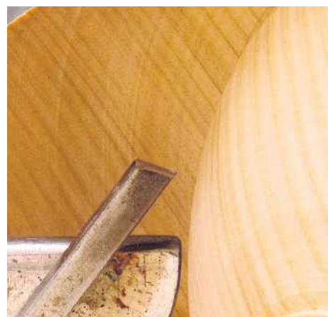
▲ Pic.18 I couldn't quite get the correct angle to do the final bit of turning with the gouge, so I changed to a diamond-shaped point tool. You only have one chance at this so be positive
