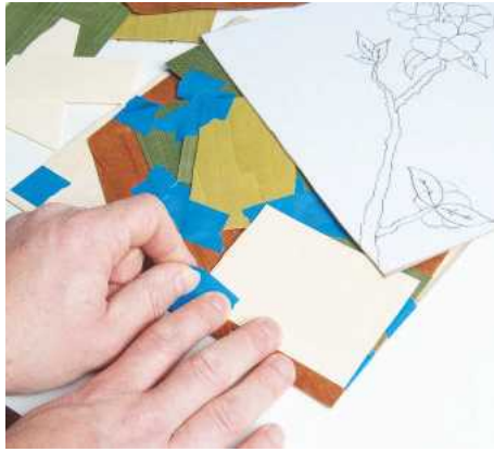
▲ Pic.2 Make sure the small pieces of veneer you use are larger than the piece you're cutting – go for a rule of 25mm larger
