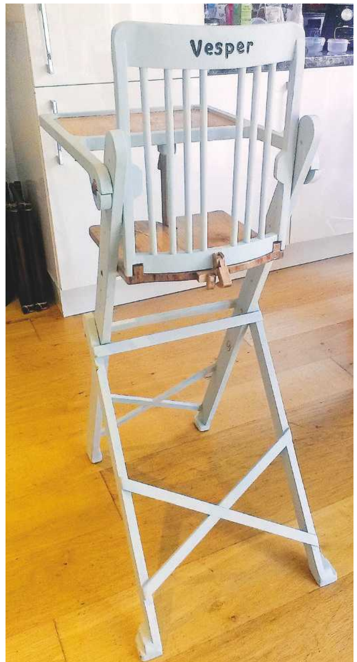
▲ Pic.9 The post supporting the tray was prevented from swivelling beyond the vertical by gluing a slim pine stop into a routed recess on the underside of the seat
