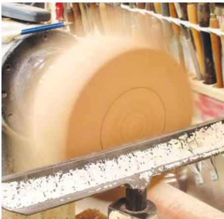
▲ Pic.4 Watch those fingers! The lathe speed is set at around 1,000rpm so anything finger-wise that you put over the toolrest is liable to be injured, so be careful!
