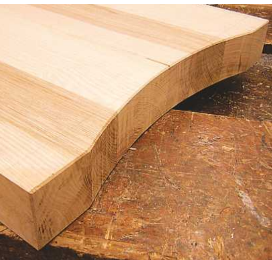
▲ Pic.8 The bottoms of the ends were curved to soften the angular lines
