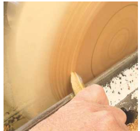
▲ Pic.6 When you have clearance you can work the bowl shape from the right to the left using the bevel of the tool on the wood; this is just like forming a normal bowl and the secret here is to forget about the square bit
