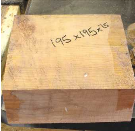
▲ Pic.1 Choose a piece of American cherry or similar, measuring just under 200mm square and cut it dead square. Any curly grain on the corners may cause a problem during the turning – we will have to see
