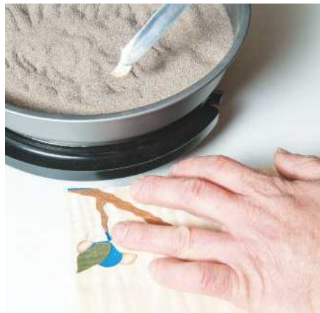
▲ Pic.5 To add depth to the picture, sand shading can be used. Carefully dip the edges in the hot sand, one at a time
