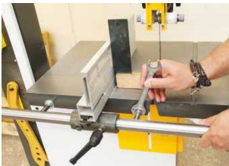
▲ The deep fence is easily set for square by minor adjustments to the running bar
