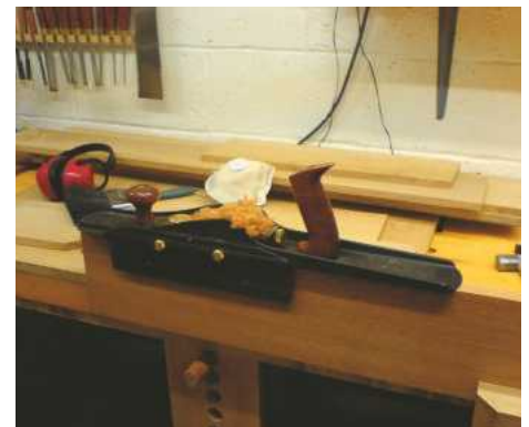
▲ Pic.3 After a pass through the planer/thicknesser, the edges and faces were finished with a jointer
