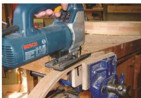
▲ Pic.13 Cut the beading to width with a jigsaw, cleaning up the surfaces with a block plane
