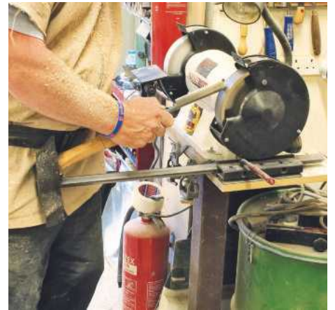
▲ Pic.12 Constant sharpening means that you will get the optimum cut. The Oneway jig makes touching up the edge of the roughing gouge simple
