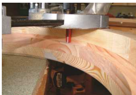
▲ Pic.11 Mark the frame position, remove and mount upside down. Rout the rebate for the glass
