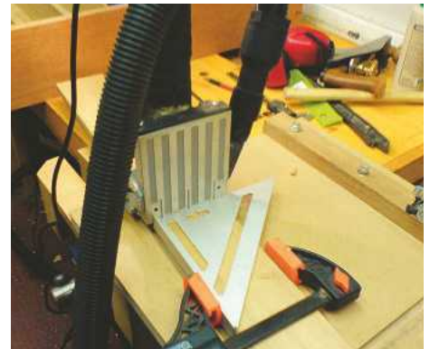
▲ Pic.13 Use a square to register the biscuit jointer when cutting the slots in the faces...
