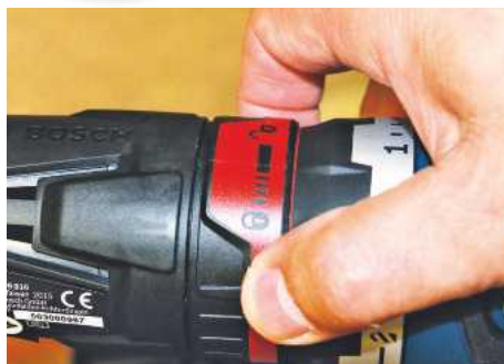
▲ The chucks are secured with a twist-lock collar
