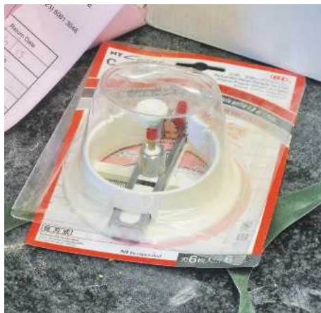
▲ Pic.35 The lamp bases do need to have baize on the bottom. The circle cutter will give you a perfect circle; scissors will not cut the baize clean enough
