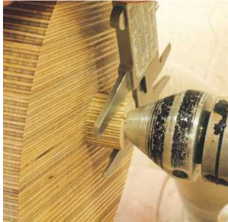
▲ Pic.20 The waste area at the top of the lamp is turned down to the diameter of the brass plate that will hold the lamp fitting. Watch out for the plywood splitting at the top
