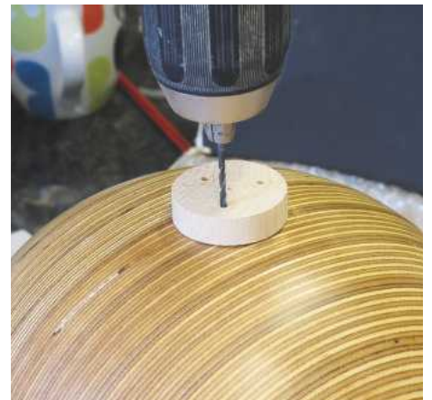
▲ Pic.33 Les made a little jig to allow him to drill the holes in the top for the brass plate. For strength he chose 25mm-long screws
