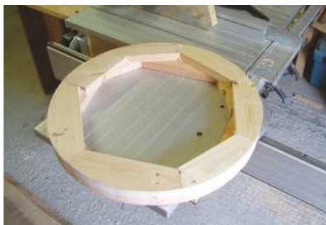
▲ Pic.5 With a jigsaw cut around the outside, leaving some waste. Repeat for the inner circle
