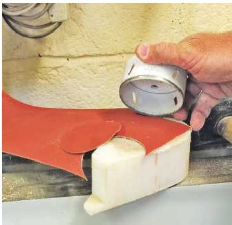
▲ Pic.22 Power sanding is not confined to bowl work and can be used on larger-diameter spindle work like this. Les cuts his 75mm discs from sheet with a hole saw with the teeth ground off
