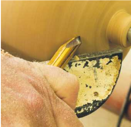
▲ Pic.19 Les doesn't like sharpening a tool that still has one of its cutting edges sharp, so will use a pull cut around the top so as to utilise both edges
