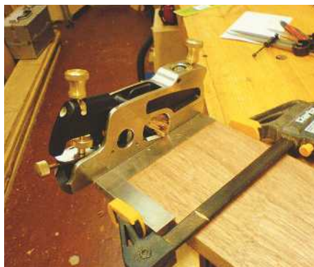
▲ Pic.6 Planing a shallow rebate in the pin board makes it easier to align the boards later
