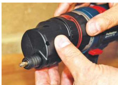
▲ You can rotate it to any position around the drill for different applications
