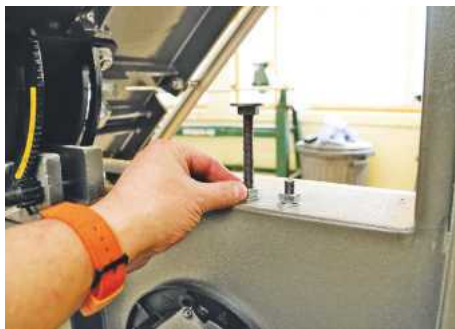
▲ This adjuster sets the table square to the blade
