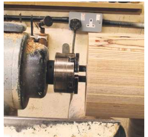
▲ Pic.15 Les has turned the base round. He likes to support the work on pin jaws, and these will hold the piece as he thins down the top. With increased tailstock pressure you could just drive off a cone
