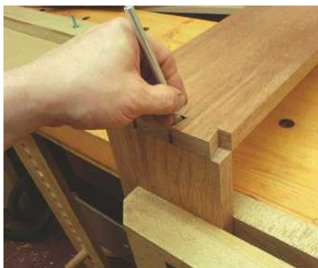
▲ Pic.8 ...after which you can use the tail board as a template when marking out the pins...
