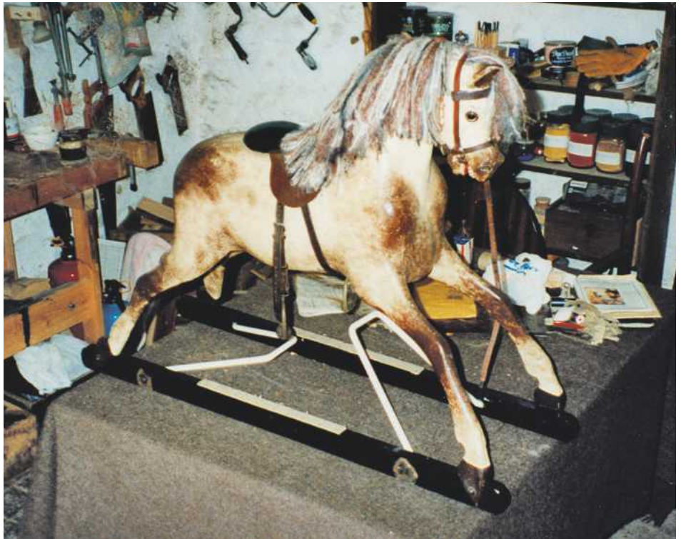
▲ Pic.3 Keep it stable: it's best to remove the horse from the rockers when working on it
