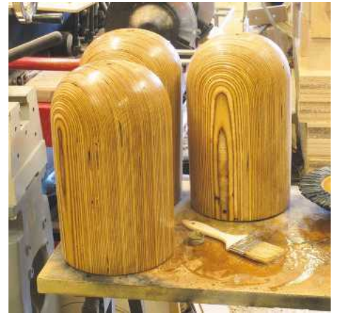
▲ Pic.30 Les experimented to find the best finish. Lacquer wasn't good on the end grain so he opted for hard wax oil, applying two coats with a light cut back between them
