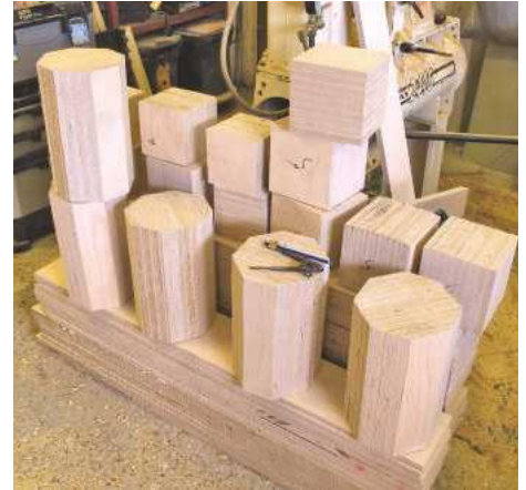
▲ Pic.3 This is about a third of the blanks needed. Les cut them to length on the bandsaw. He found that a narrow kerf blade cut the plywood better
