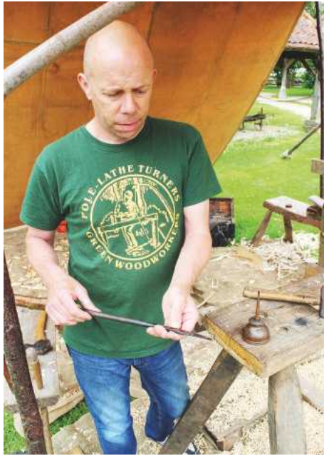
James Pumfrey turns bowls at speed using only this tool he fashioned from an old spring
