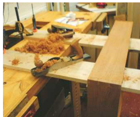
▲ Pic.10 Clean out the corners of the stopped rebates and the pin joints
