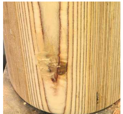
▲ Pic.27 Larger holes will need to be filled in in two goes. This one is a remnant of a knot in the birch. Apply the filler by hand with the abrasive on a cork block
