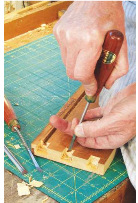
▲ Pic.12 Cleaning into the corners: you will need both a right- and a left-handed skew
