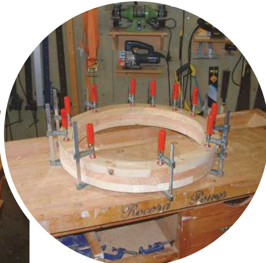
▲ Pic.7 Apply glue to all surfaces and cramp the third layer to the frame. Clean up when dry
