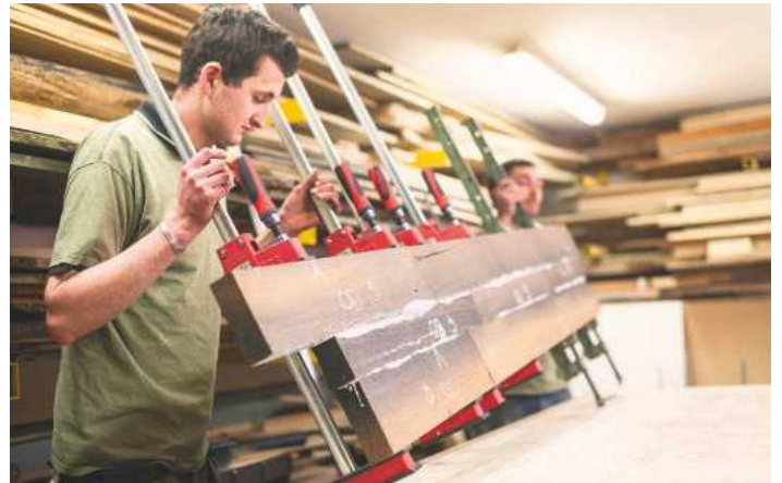
The prepared boards are glued up to create the desired appearance in the end-grain top surfaces
