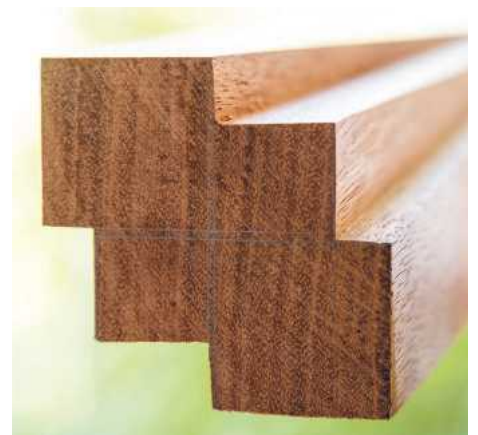
You get the idea: the cross section of one of George's table legs showing the 3-dimensional 'sunburst' of its stepped tapers
