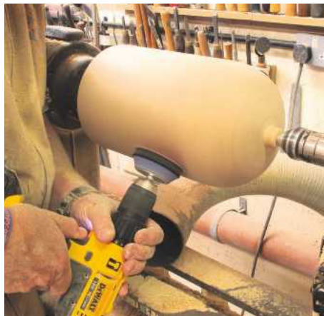
▲ Pic.23 Keep the drill down low. Sanding on the lower quadrant with a small gap at the top of the pad means that the drill will be easier to control
