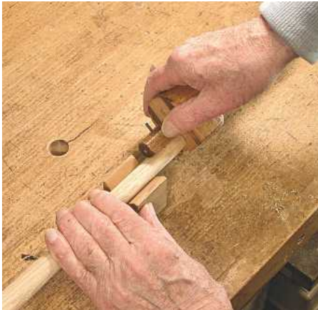
▲ Pic. 4 Using the marking gauge, scribe the tenon shoulder
