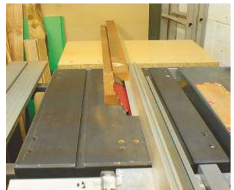
▲ Pic.19 Cut the French cleats on a table saw, then clean them up before cutting to length
