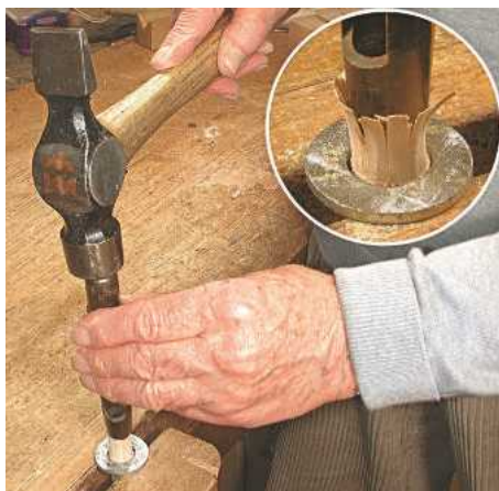
▲ Pic. 8 Jeff drives a leather punch to form a perfectly round tenon
