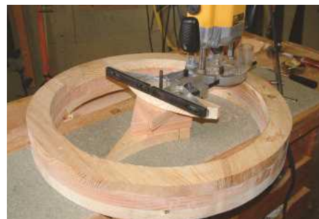
▲ Pic.10 Trim the inner and outer circumferences gradually with a long straight router bit
