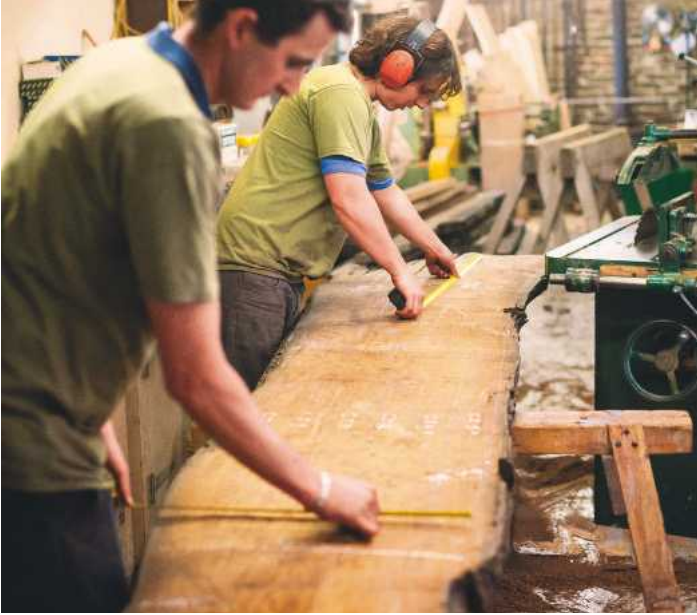
Each board is carefully surveyed to ensure maximum yield
