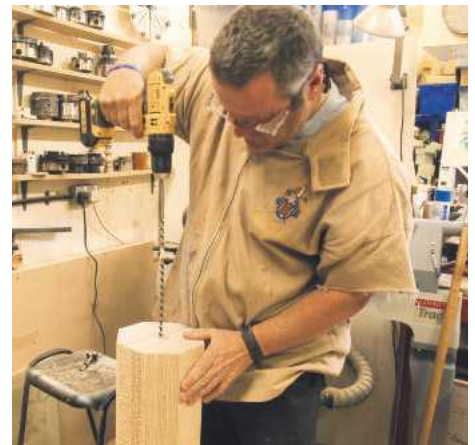
▲ Pic.6 Use the drill press to part drill a 7mm hole in from each end and then complete the through hole with a beam drill. For greater accuracy use the usual long-hole boring method
