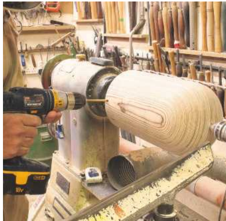
▲ Pic.29 The general consensus of a straw poll was that these lamps look best with the side grain facing you. Pick the best side and then drill a 7mm hole into the opposite side for the flex
