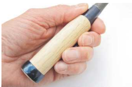
The two handle diameters depend on blade width
