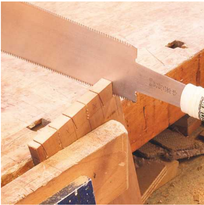
▲ Pic.6 Cutting the tails with the board angled so that the saw line is vertical
