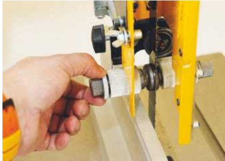
▲ All the guides have tool-free adjustment and can be finely set
