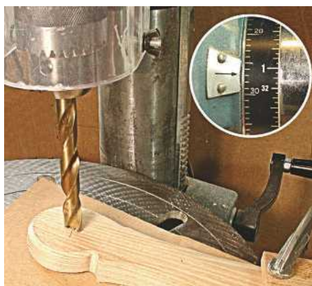
▲ Pic. 2 Here Jeff is preparing to start with a blind hole for the leg's tenon
