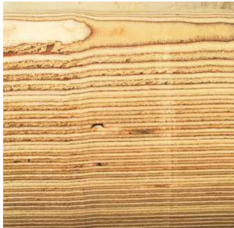
▲ Pic.11 You can see the difference between the roughing and the smoothing cuts. It will always tear out, you just have to make the best cuts to minimise the timber tear out
