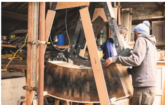
Once created, the curved sections are uniformly cleaned up with an ingenious pendulum router cradle
