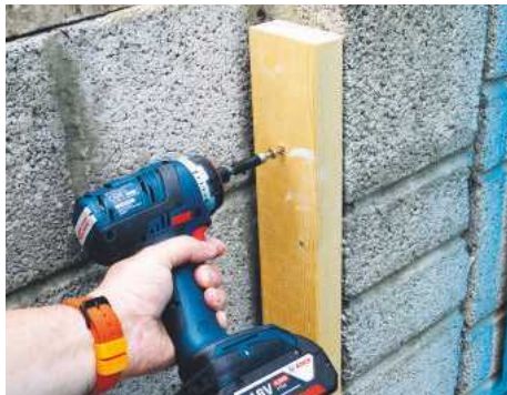
▲ As a direct-drive screwdriver it powers in concrete screws with ease...
