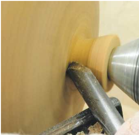
▲ Pic.28 Les prefers to remount the wood and turn the last bit of waste away, but you could just cut this off with a saw. The small section needs to be flat for the brass plate to fit properly
