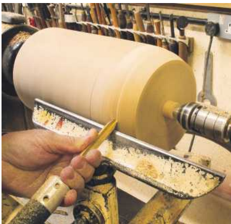
▲ Pic.16 The design calls for a curve about a third from the top, executed with the Robert Sorby bowl gouge that will keep edge longer than a normal M2 high-speed steel one
