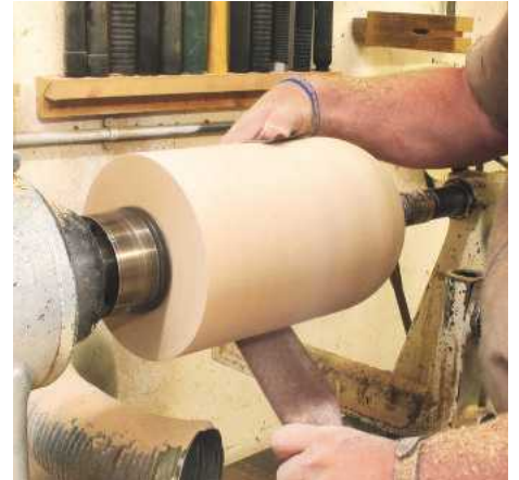
▲ Pic.21 You will find it very hard to get the desired finish off the tool so use the jokily named 60-grit gouge to finish off the shape. Plywood does sand remarkably well
