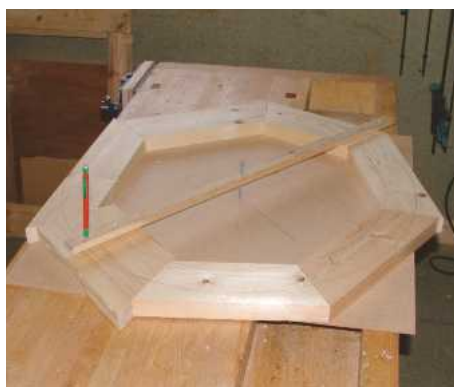
▲ Pic.3 Glue the segments together. When dry, clean up the surface and redraw both circles
