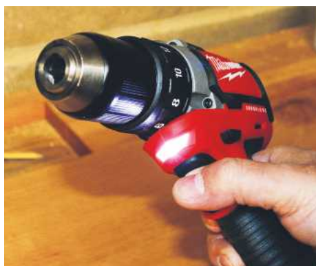
▲ A worklight is activated by pulling the trigger
