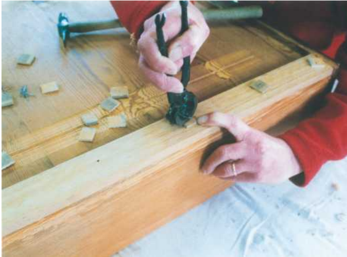
▲ Pic.4 Simple but effective: bent pins make excellent mini-clamps and after removal...
