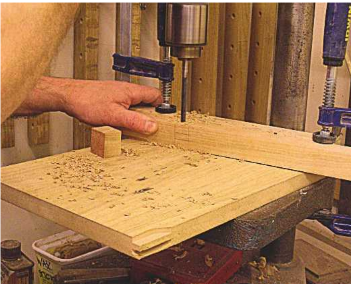
▲ Pic.6 Although the mortises are quite small, the bulk of the timber was removed with a drill
