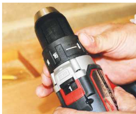
▲ There's a single collar to switch between drill and torque control
