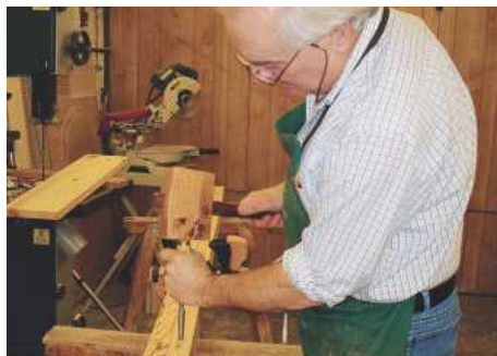
▲ Pic.4 ...to cut the wedge from the outside of the mortises by hand
