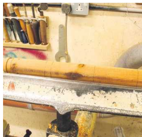
▲ Pic.18 Les has now marked on the fixed areas, like the overall length and where the small lower arms come out
