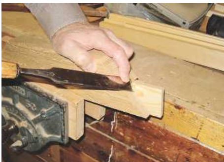
▲ Pic.16 ...when cutting the ovolo profile on the window rails
