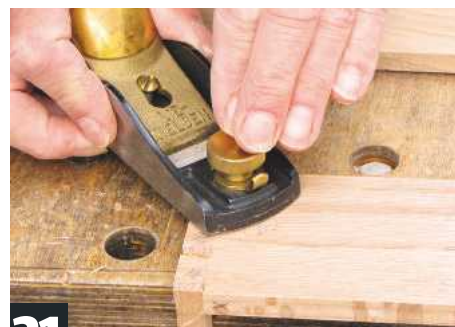
21 Once glue has dried, trim protruding dovetails flush with finely set block plane
