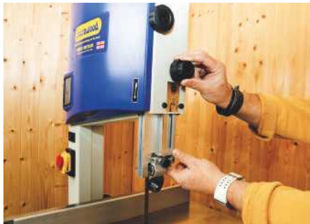
▲ The height post is set with the double-function knob
