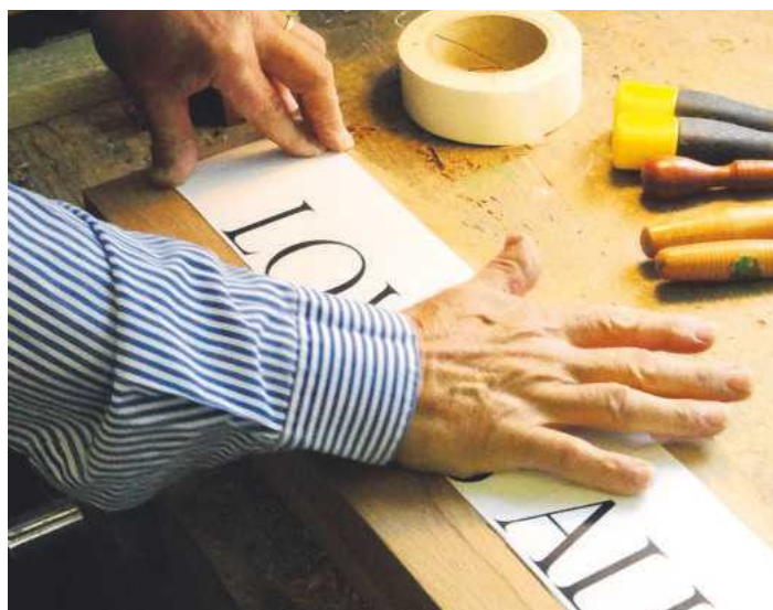
I laid double-sided tape on the back of the lettering and pressed it down firmly. The tape gripped well and, at the end of play, could be peeled away leaving no residue
