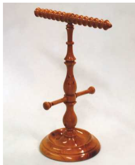
▲ Pic.35 For a glossy finish Les omits sanding sealer on this dense timber, and applies lacquer followed by burnishing cream when the lacquer is dry
