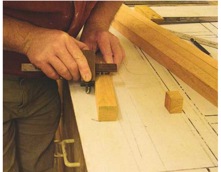
▲ Pic.5 The positions for the mortises were clearly scribed out with a mortise gauge
