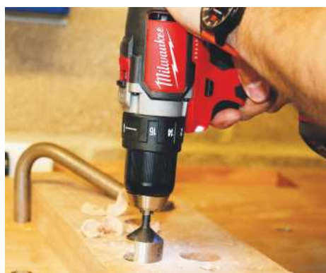
▲ An auger into beech didn't stall the drill but it needs a side handle!
