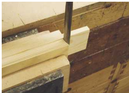
▲ Pic.17 The job is finished with a short scribing cut, which...
