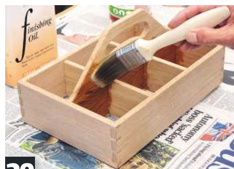
30 Brush on two coats of finishing oil, wiping off after a few minutes. Alternatively, add wax if for indoor use
