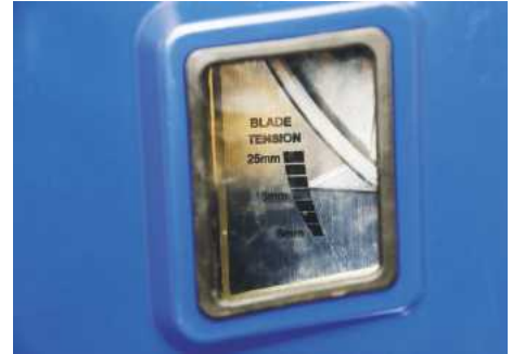
▲ You can check the setting through the viewing window in the top door
