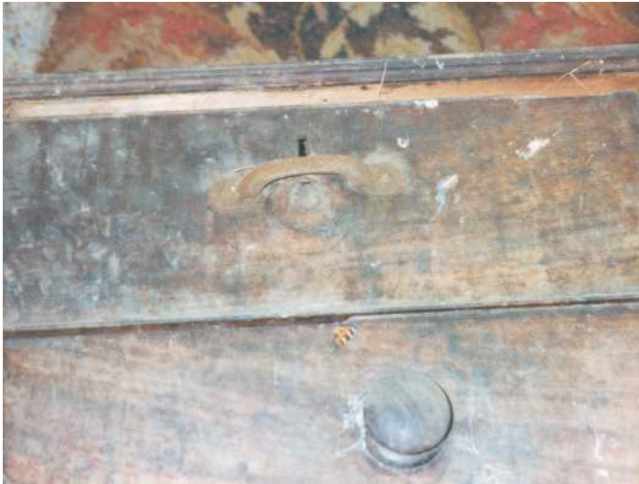
▲ Pic.6 Utilitarian as well as decorative: there's a missing section of cockbeading to the left of the dead butterfly...and note the ghastly handle botch
