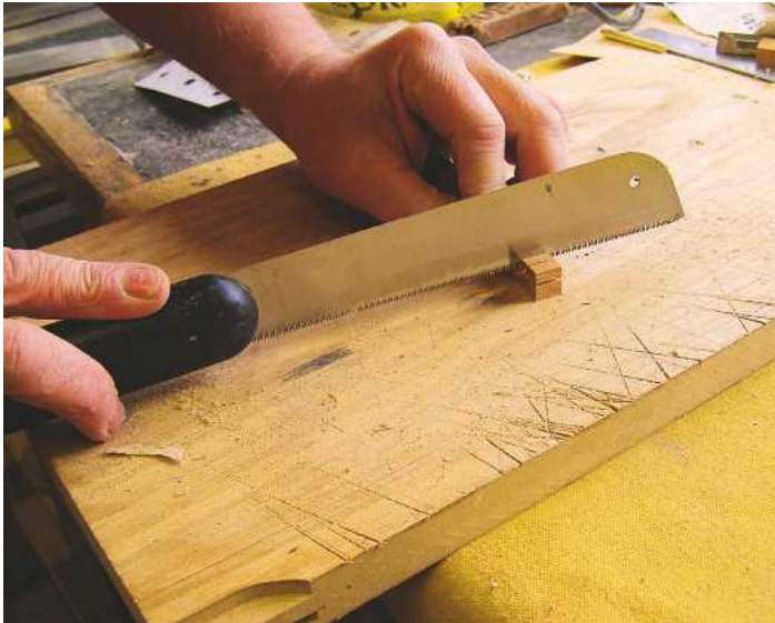
▲ Pic.13 The buttons to hold the table top were prepared from square sections of timber. A small pull saw makes a neat job of removing the waste
