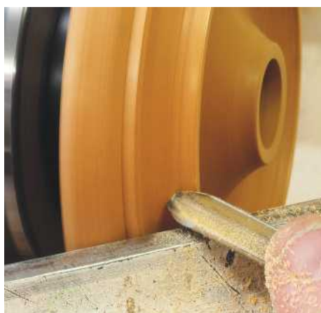
▲ Pic.14 He has swapped to the small Signature gouge because the bevel of this tool will fit perfectly in the tight curve on the edge of the base
