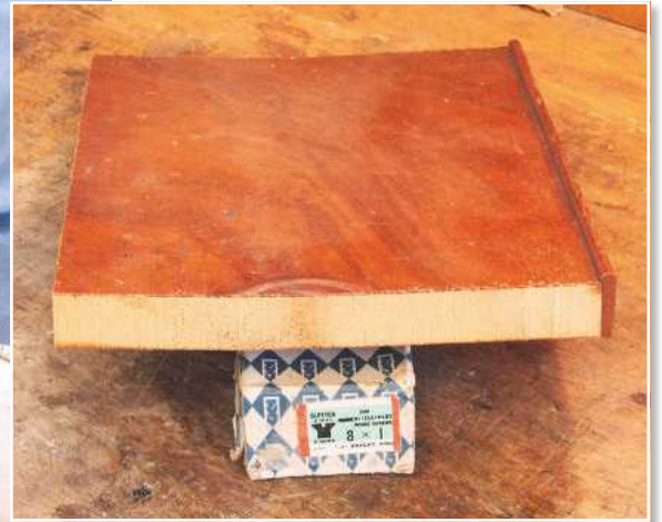
▲ Pic.1 Planing edges square on shooting board and, inset, showing bowed timber
