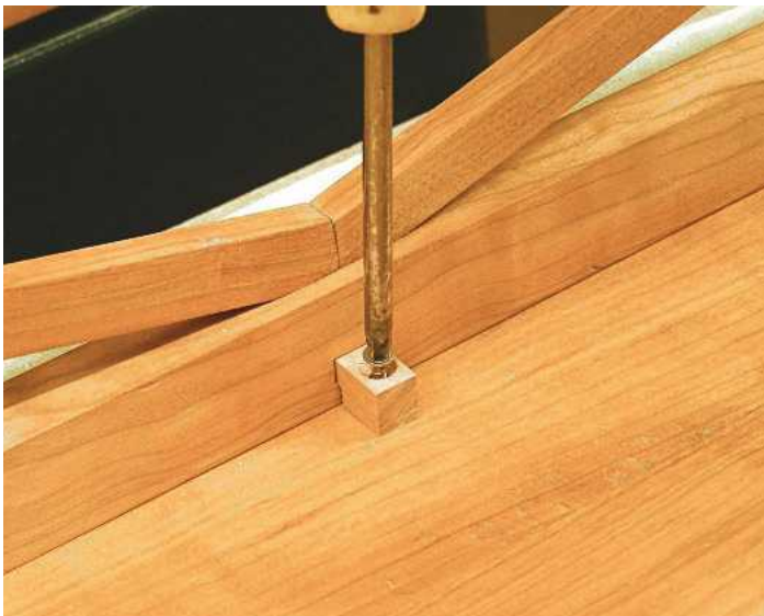
▲ Pic.15 The buttons fit into mortises cut into the inside faces of the rails. Eight are used to hold the table top
