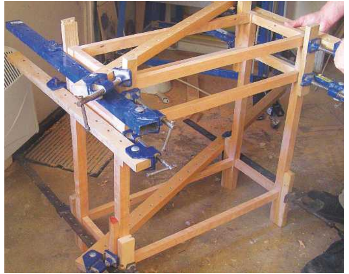
▲ Pic.9 Join the front and back rails together with end rails. Use a cramp across the diagonal to keep the frame square
