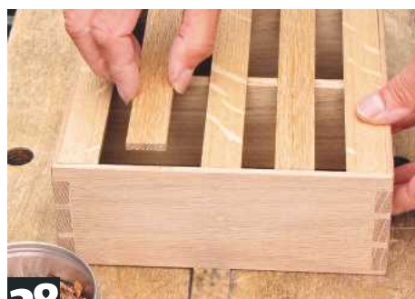
28 Thickness slats to 24 x 5mm and saw to length. These can be pinned or screwed into rebates
