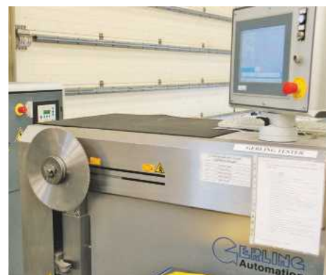
Blades go onto this machine to check them for true after tensioning
