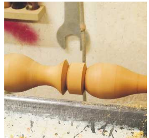
▲ Pic.24 The flat left in the shaft is for the arms to come out of. I thought about putting a cove here and in hindsight I should have – Mark II will have one
