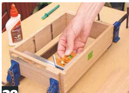
20 Clean up inner surfaces and check for fit. Glue and cramp up tray, checking for square
