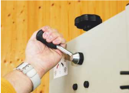
▲ A tensioning lever allows fast blade swaps
