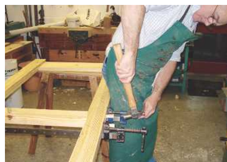
▲ Pic.9 The frame is now glued up, assembled, and the wedges are driven home
