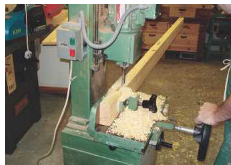
▲ Pic.3 ...which Mike cut on the mortiser using a 12mm chisel, saving his chisel and mallet...
