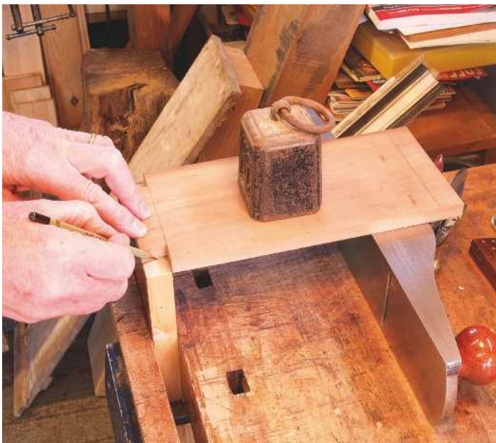
▲ Pic.6 Marking pin board
