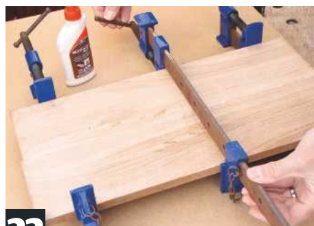
22 If required, glue boards together to achieve sufficient width for carrying handle. Thickness when dry
