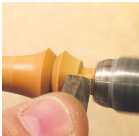
▲ Pic.26 He is turning the top spigot down to 10mm to fit into the top cross member. It can be worth taking a little tailstock pressure off at this point to prevent splitting
