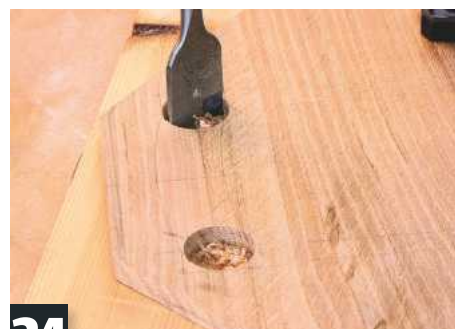
24 Mark hole centres and cramp board to backing material. Bore ends of cutout with 25mm flat bit
