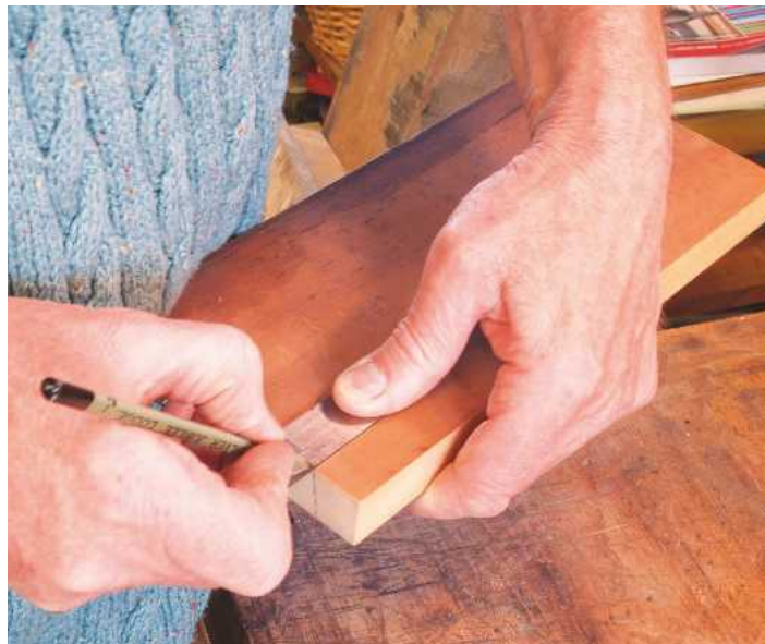
▲ Pic.9 Marking perpendiculars on pin board
