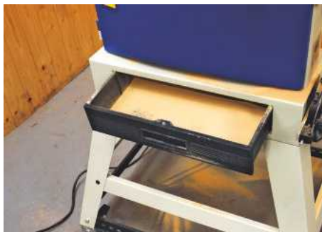
▲ As an indication of the collection feature, this is from one rip cut
