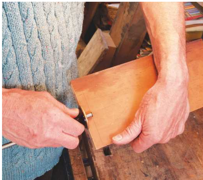
▲ Pic.7 Measuring thickness of tail board
