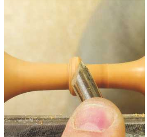
▲ Pic.21 When you have a large cove like this you can break it up with a bead in the middle. As the piece gets thin you can support the spindle with your finger as you are turning
