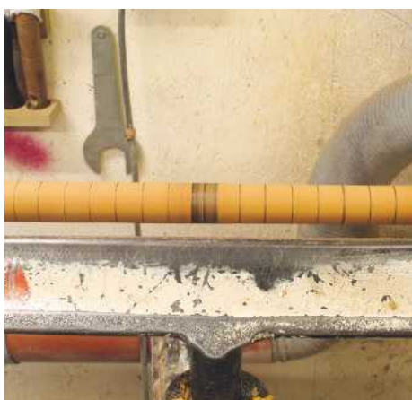
▲ Pic.31 The top cross member is mounted up last. The dark area in the centre will be where the hole will be drilled. He marked out a series of coves by eye
