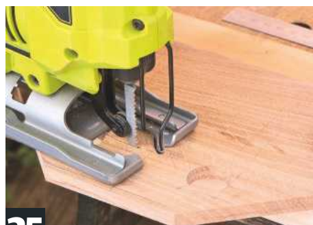
25 Remove remaining waste between holes with jigsaw. Use this for sawing tapered edges of handle
