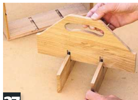
27 Handle and dividers are slotted together. Mark out halving joints and carefully cut away waste
