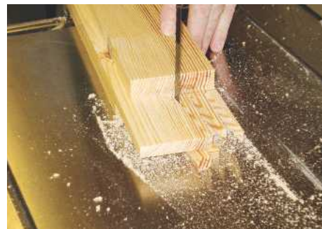
▲ Pic.5 The wedges themselves were cut from the waste material
