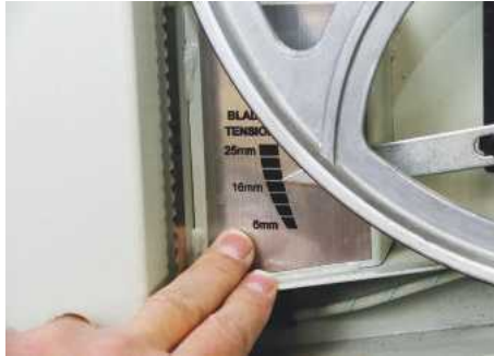
▲ Tensioning can be assessed with the indicator
