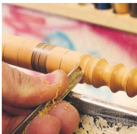
▲ Pic.32 Cut a series of coves along the length, working from the tailstock end towards the headstock. Not only do they look decorative but they will also stop the jewellery falling off
