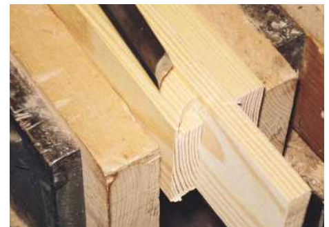
▲ Pic.18 ...produces the correctly shaped rebate for the moulding on the stiles
